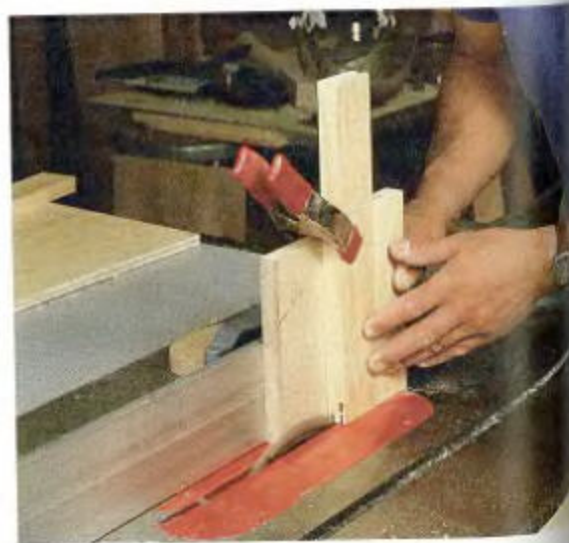
TENONING JIG FROM SCRAP. A stick of pine nailed to a square of medium-density fiberboard makes a jig to produce reliable tenons.
