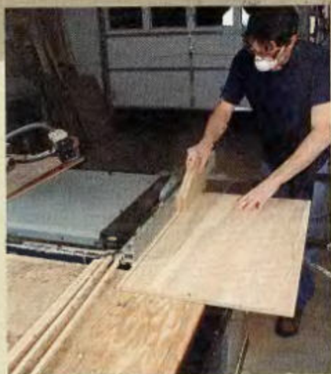
CUT THE SLATS. After applying backing veneer to one side, rip the panel into slats. A double-width push stick and a slow, steady feed rate help keep the slat tight against the fence.
