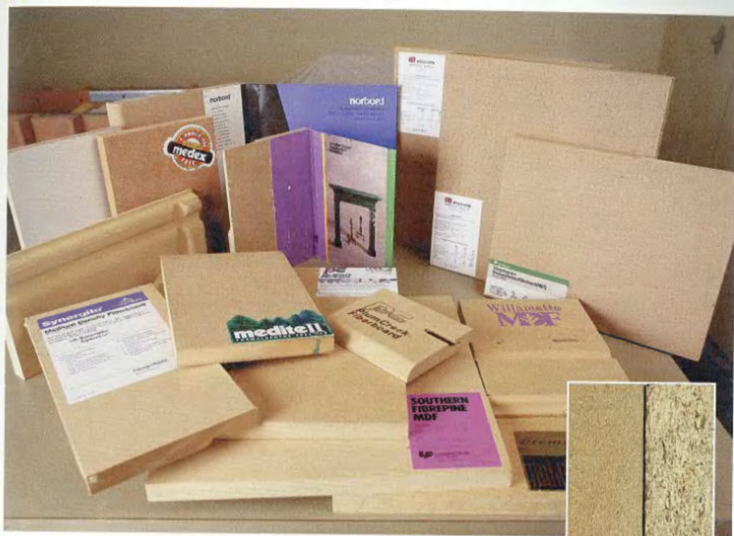
A VARIETY OF DIFFERENT TYPES OF MEDIUM-DENSITY FIBERBOARD (MDF) are available from nine companies that manufacture the material. Although it has been used in industry for 28 years, MDF is just now becoming more available to consumers and small shops. The difference in density is obvious when comparing MDF, left side, to common particleboard, right side.
