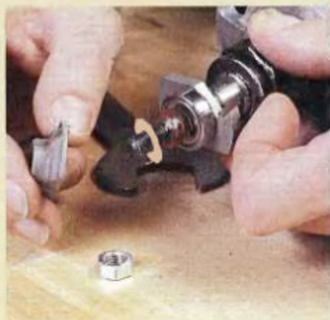
REVERSIBLE BITS ARE ADJUSTED BY USING SHIMS. A good-fitting coping and snug-fitting stub tenon require some trial-and-error when adjusting the distance between the cutters.
