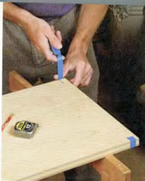
RIPPING CUTS TEND TO BE CLEAN , but crosscuts are prone to tearout. Raise the blade well above the sheet and put the most important face up. Then wrap blue tape across the bottom and around the ends.
