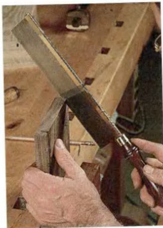
1. CUT THE TWO HALF-PINS at either edge of the drawer-front end, taking care not to cut past either scored line.
