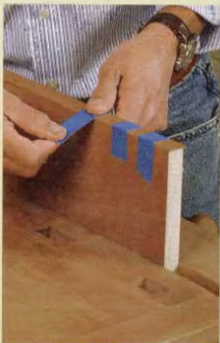
MASKING TAPE MAKES A GOOD CLAMP. Numerous short pieces of masking tape provide plenty of pressure for gluing wood edging.
