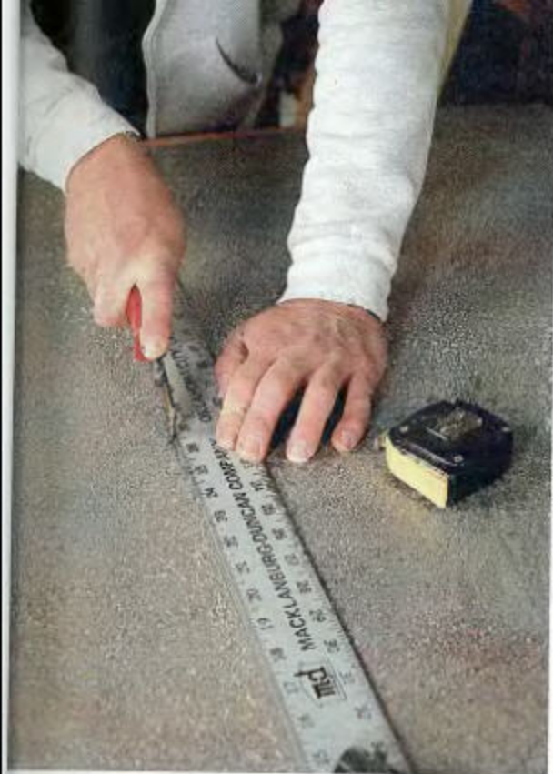
A CARBIDE-TIPPED SCORING TOOL MAKES CUTTING LAMINATE QUICK WORK. When cutting a sheet of plastic laminate down to rough size, use a light touch for the first couple of passes. Increase pressure gradually until you're through the top layer.
