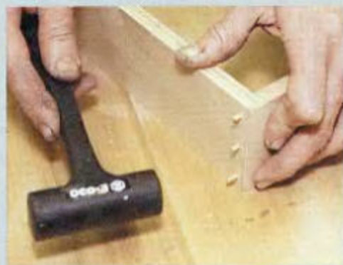
PIN A RABBET JOINT WITH DOWELS OR NAILS. Fasteners keep the joint from breaking apart when the drawer is yanked open.
