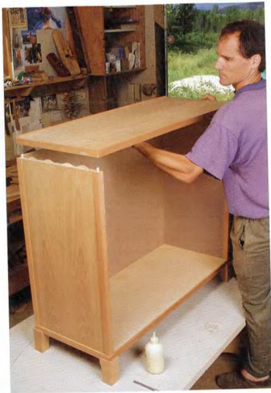
ATTACH THE TOP. Like the bottom, the top is located and attached with biscuits and dowels. The biscuits locate the panels side to side, and the dowels lock in the front-to-back alignment.
