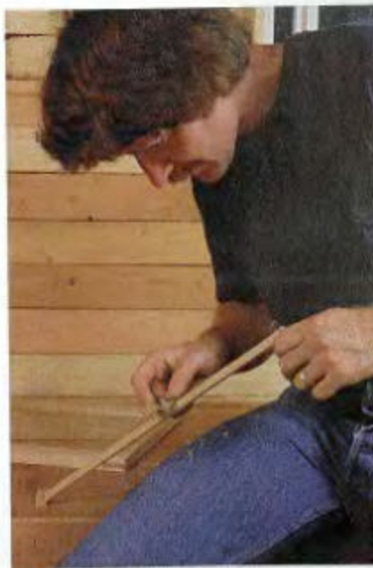
CHAMFERING THE BEVELED STRIPS relieves any sharp edges.
