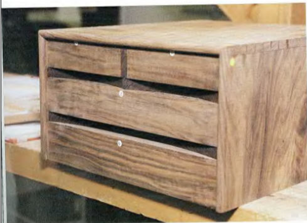
FRONTS ARE FITTED. With all drawer parts fit to their openings, the drawers can now be dovetailed together.
