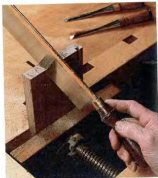
3. VISUALLY DIVIDE THE REMAINING SPACE in half for a drawer with two full pins, in thirds for a drawer with three full pins, and so on. Make all cuts at one angle first (see the drawing on the facing page for sequence), and then cut all the opposing angles. Also cut the pins for the drawer back at this time, using the same method. For the strongest dovetail joint, through- or half-blind, pins and tails should be approximately the same size.
