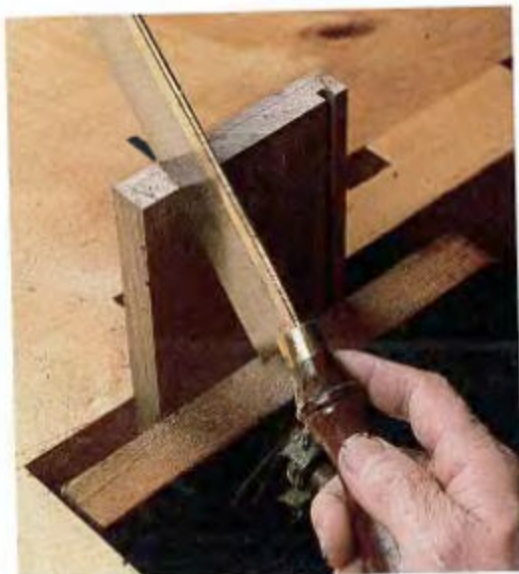
2. NEXT, JUDGE ANGLE AND SPACING BY EYE, without laying out the dovetails, and cut a full tail.
