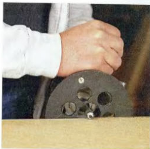
FOR A LESS-CONSPICUOUS SEAM when using conventional plastic laminate, glue the edge on first, and then trim it flush with the top using a laminate trimmer or small router. That way, the top sheet of laminate will cover over the strip along the edge, making the seam less evident.
