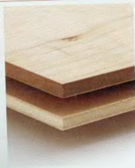
MDF- VS. VENEER-CORE PLYWOOD. Veneer core tends to run a little undersized, while MDF core is usually right on.
