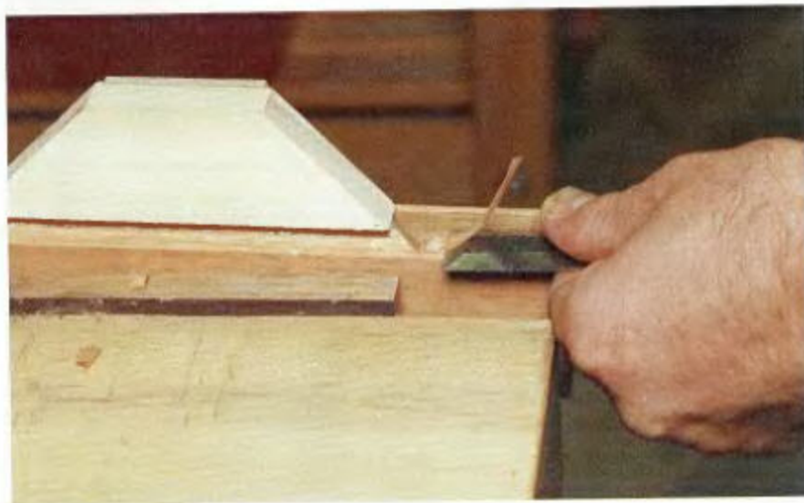
MAKE FINAL ADJUSTMENTS USING A CHISEL. The back wall of the groove on the stiles must be removed up to the miter. On both rails and stiles, use a guide block—a piece of scrap cut at 45° and clamped to the stock—to miter the inside corners of the profile.
