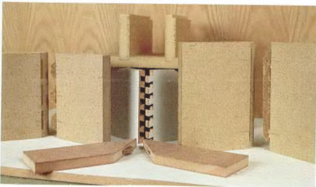
A WIDE VARIETY OF JOINERY is possible with MDF. Examples shown here surrounding a routed dovetail joint are, clockwise from left, biscuits, dado, rabbet and dado, spline miter, and biscuit miter. The background is a sheet of factory-veneered MDF.
