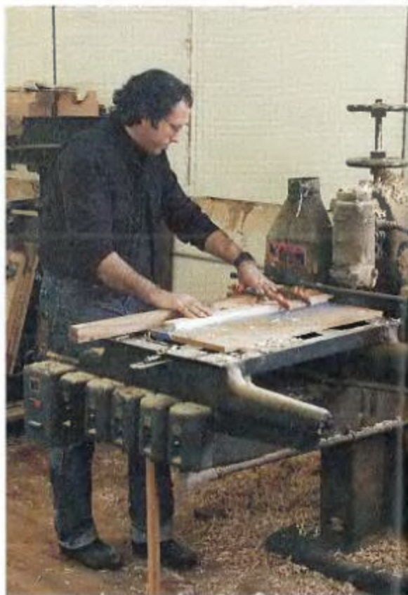
AN ANCIENT MACHINE IN A LOW-TECH SHOP. The author uses a 60-year-old single-end tenoning machine to mill cabinet parts. Aside from this machine, his shop is decidedly low tech. Good materials, solid joinery, and quality hardware make his cabinets bulletproof.
