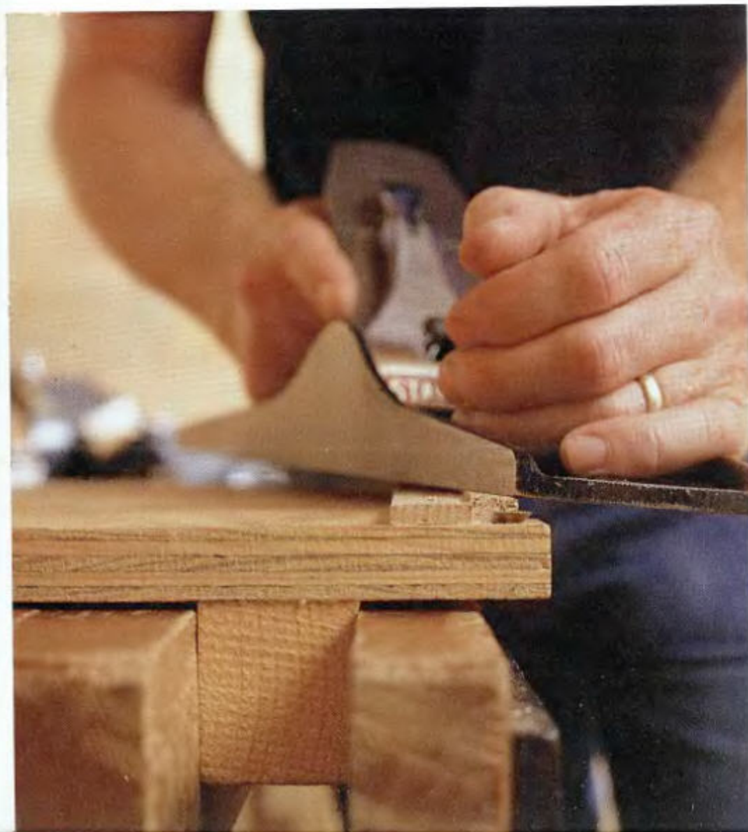
USING THE MINI-BENCH. A screw keeps the strip in place while the author planes a 5° to 8° bevel.
