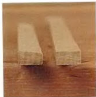
THE STRIP ON THE LEFT IS READY TO INSTALL. The bevel and chamfers, though small, are obvious when compared with the rectangular strip on the right.
