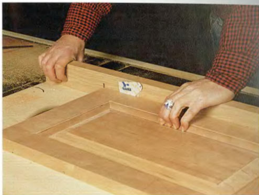
CUTTING DOORS DOWN TO SIZE. A sliding-crosscut box for the table saw makes it easy to trim doors accurately to size. A paper shim between the fence and the door produces a tapered bottom rail to fit an out-of-square opening.
