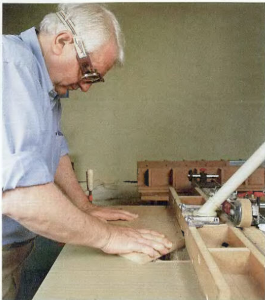
SHOP-BUILT ATTACHMENTS HANDLE MDF'S DUST on the author's router table. Built as an extension of his table-saw table, the router table houses a shop vacuum and sound baffling, which makes for quiet, dust-free operation.
