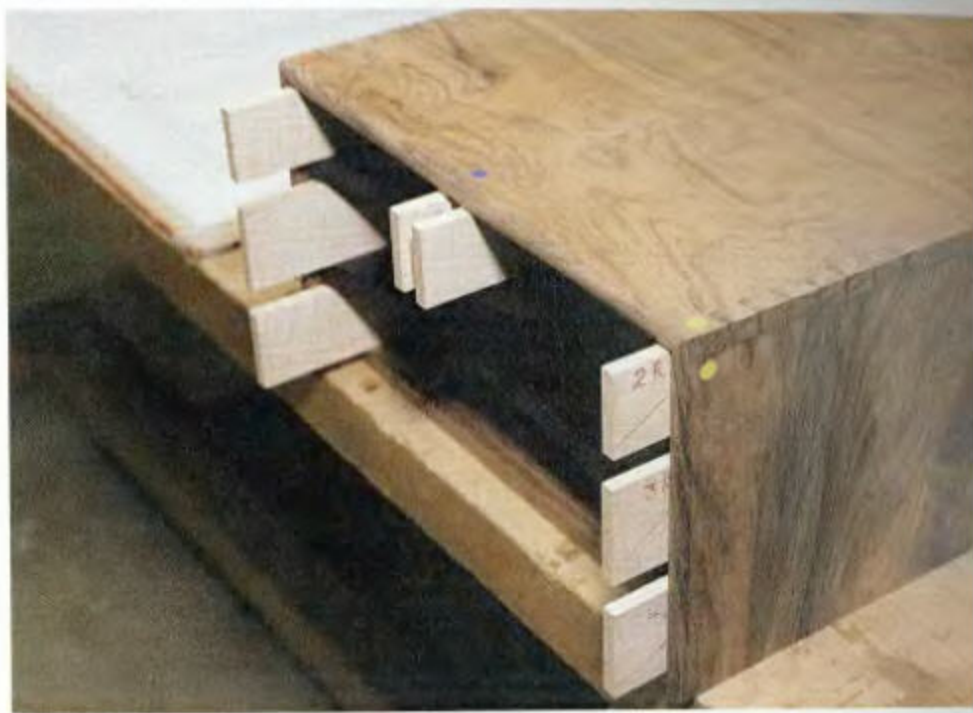
THE SIDES HAVE BEEN FITTED. The drawer backs are next. Colored dots at the corners of the case piece identify mating edges and indicate the front of the case.
