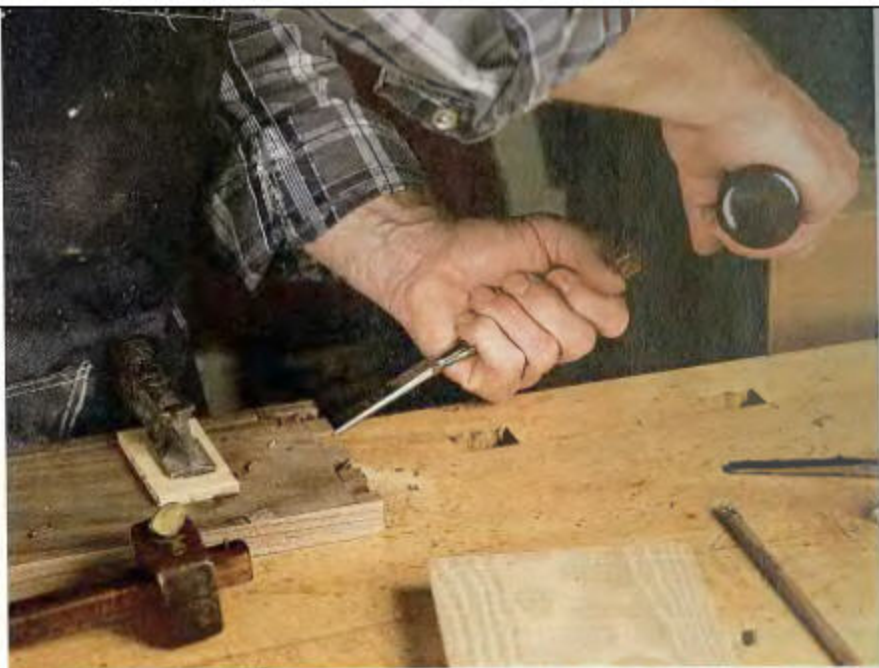
5. POSITION YOUR CHISEL 45° AWAY FROM YOUR BODY, about halfway between baseline and the end of the board, bevel up. Whack the chisel with a mallet, gradually moving the chisel back to the end of the board, working down through the waste between the pins.
