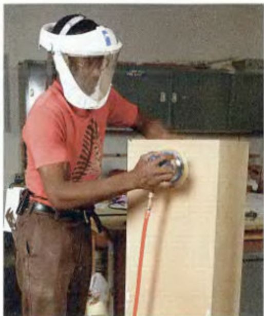
DEALING WITH DUST. A worker in the Sackler Gallery cabinet shop at the Smithsonian Institution avoids the fine dust produced by MDF by wearing a Racal powered respirator while finish-sanding a display cabinet.
