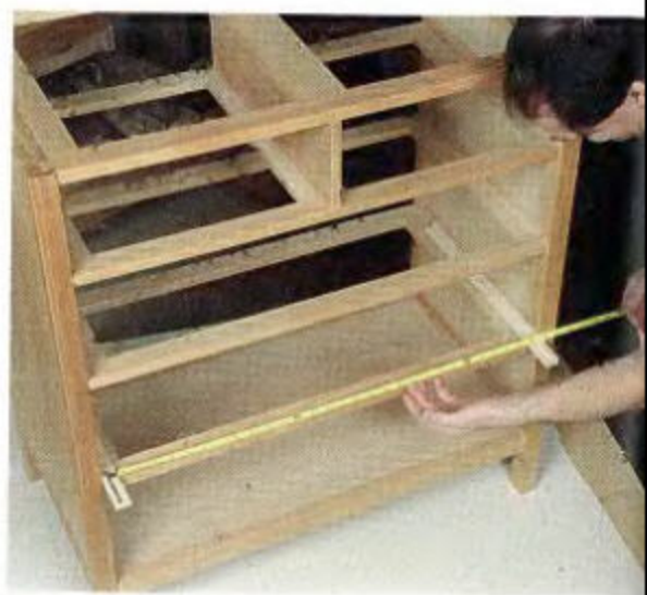
START WITH THE BOTTOM ASSEMBLY. With the runners in place, determine the width of the plywood bottom. Cut the bottom a bit wider than necessary. Then trim it to fit.
