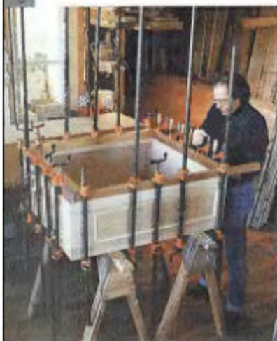
CAULING ALL CLAMPS. Strips of wood, called cauls, are placed between the clamps and the face frame to prevent marring. The author uses numerous clamps when gluing the face frame to the cabinet's plywood carcass.
