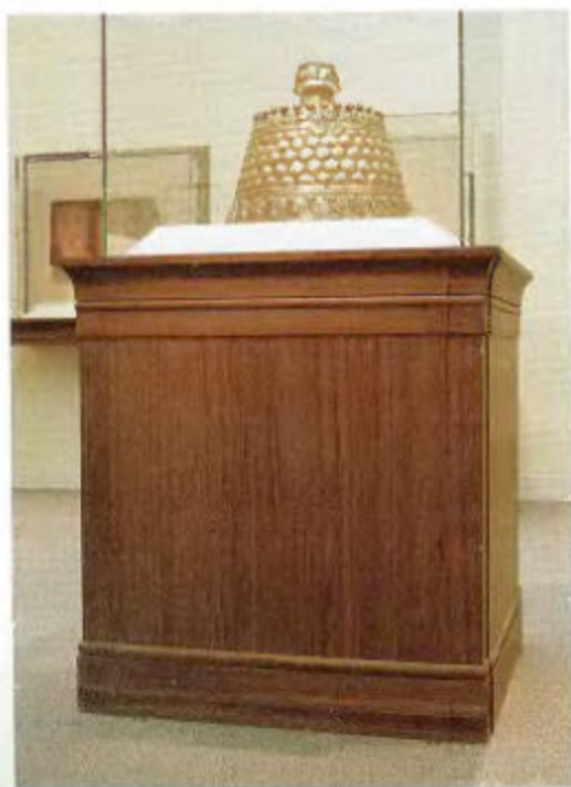
MUSEUM-QUALITY MDF. These display cases at the Freer Gallery of the Smithsonian Institution show off some of MDF's versatility. The case pictured above shows the crisp edge-holding ability of MDF in a painted piece. The case shown below makes use of walnut-veneered MDF with solid-wood moldings.
