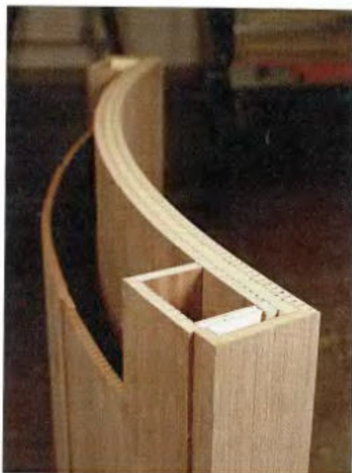
KERFS FOR A CURVE. Woodworkers at the Sackler Gallery cabinet shop in the Smithsonian Institution kerf-bend veneered MDF to make a curved museum bench.
