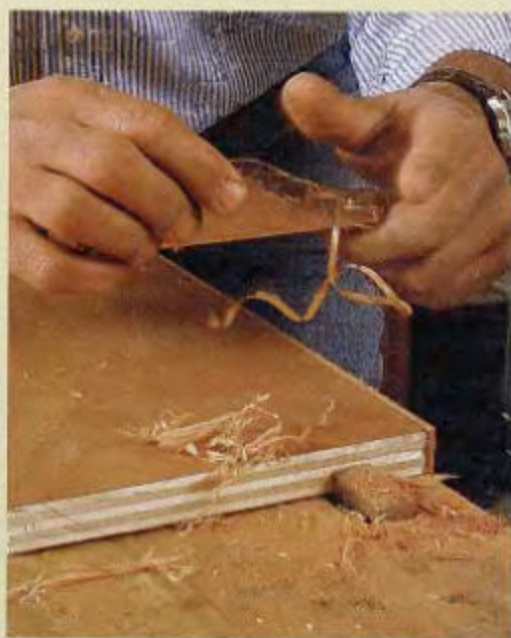
TOOLS FOR TRIMMING. Use a block plane to trim most of the excess edging flush to the plywood surface (above). Angle the sole of the plane to achieve a cleaner cut. A cabinet scraper finishes the job (right).
