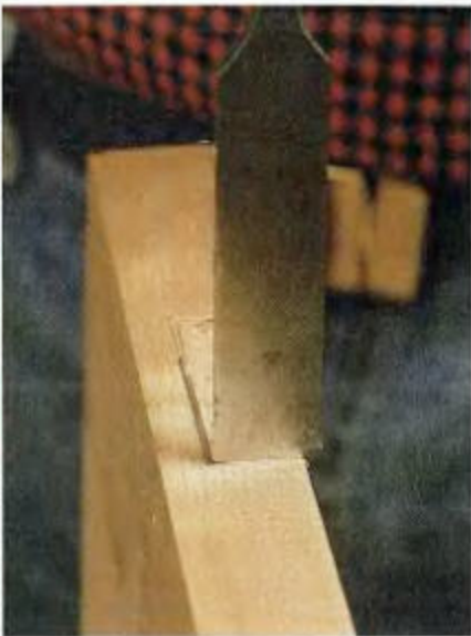
PAVE MORTISES GRADUALLY to the scribed line, alternately cutting down and from the side. Be patient, and work slowly for best results.
