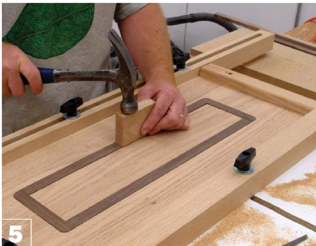
5 Apply glue in the grooves and lightly tap the strips to seat them.
