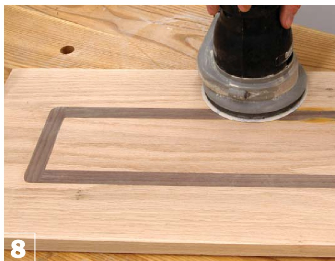
8 Sand the inlaid strips and door panel until you achieve a smooth surface.
