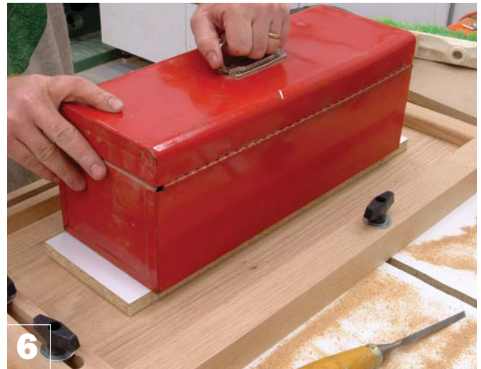
6 Use a heavy weight (a fully loaded toolbox works well) on top of a flat board to hold the strips while the adhesive sets up.
