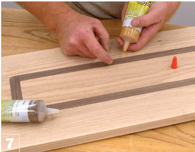
7 Once the glue has cured, fill any voids with the appropriate color of wood filler if required.
