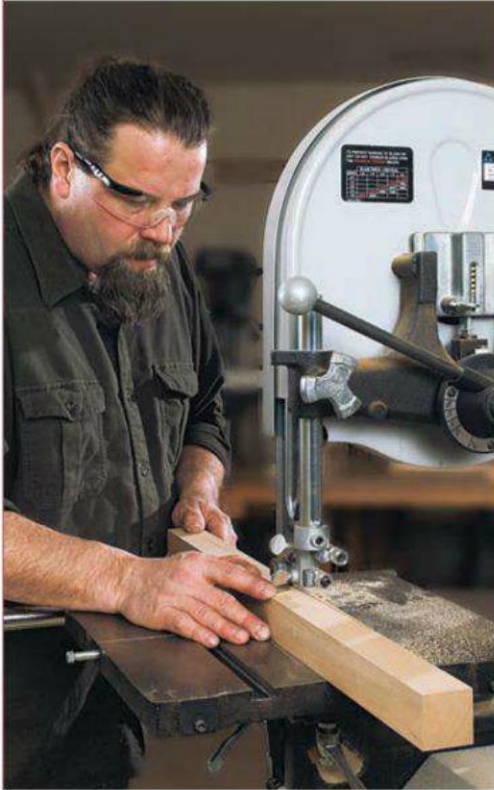
The author used a cabriole leg-cutting technique to form the simple tapers on two faces of the glued-up maple legs.
