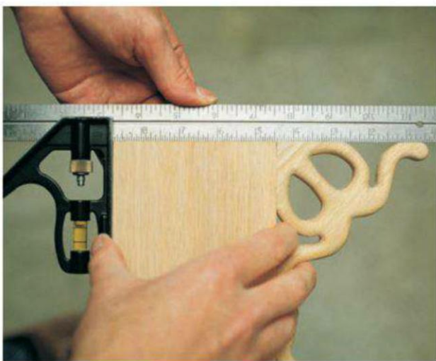
Figure 4: When gluing the brackets to the aprons, a combination square helps line up everything while the glue is still wet.
