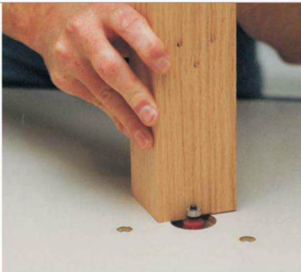
Figure 2: Ease the bottom edges of the legs with a 1/8" round-over bit. At 31 1/4" long, these legs are short enough to perform this operation while holding each leg vertically on the table.
