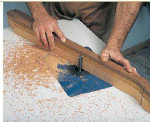
After band sawing the front and back profiles to within 1/16" of the cutline, attach the side template and rout to the cutline using a flush-trim bit.
