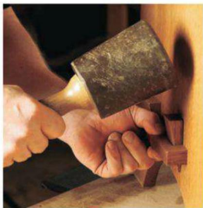
Using a plane inverted in a bench vise (photo at right), the author carefully fits the wedges in their mortises. During final assembly (above), the wedges are coaxed home with a few gentle taps from a rubber mallet.
