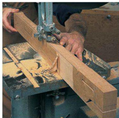
Reattach the offcuts to the front and back of the leg with hot-melt glue, then band saw the side profiles to within 1/16" of the cutlines.
