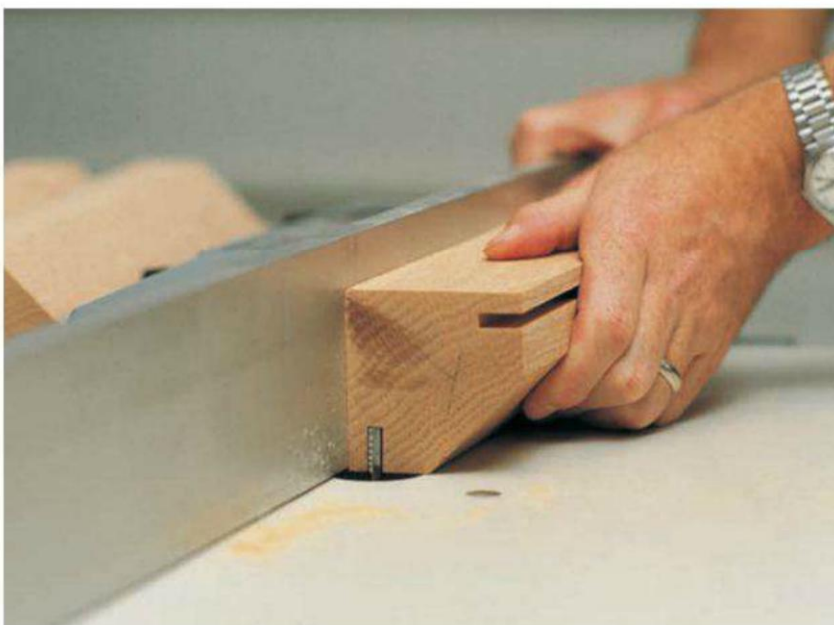
Figure 1: Mortises in the legs (they house tenons on the brackets and aprons) are cut on a router table using a 1/4" spiral-fluted straight bit.
