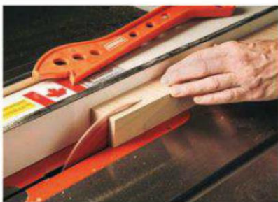
Once the roughed-out blanks were trued up, the author cut out the actual turning blanks on the table saw, as shown above.
