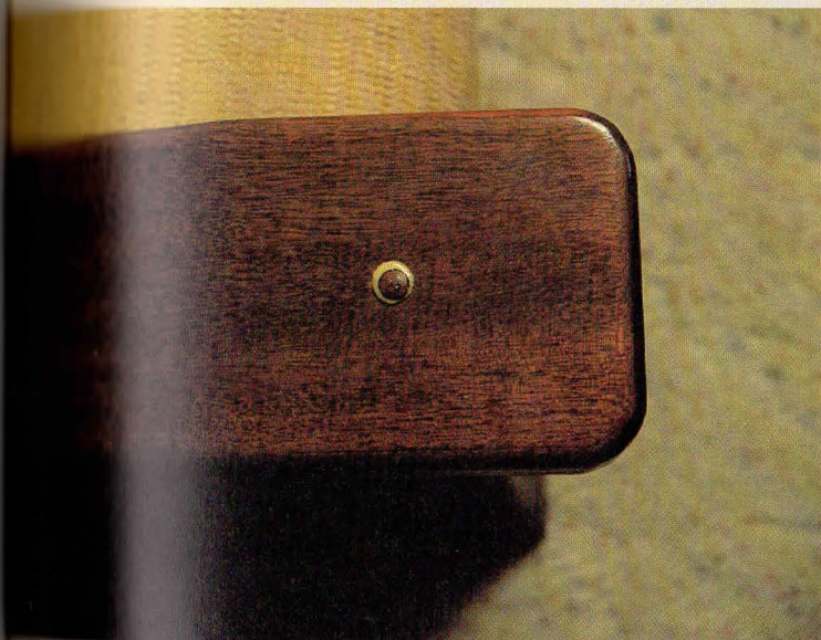
Glue in mahogany buttons with polyurethane glue.
