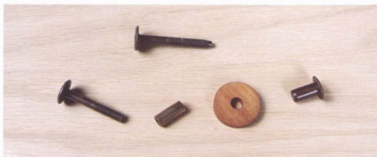
PHOTO J: The pivot is put together from stuff I found at my local hardware store. One of the connector bolts is cut shorter so that it can be tightened down all the way.
