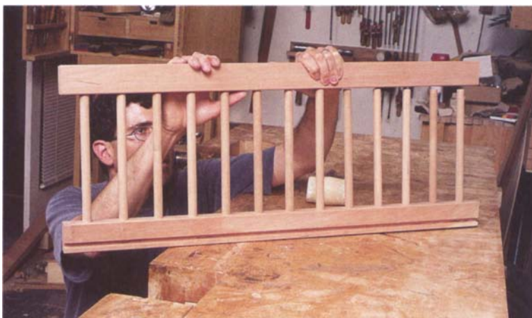
PHOTO F: The upper rail goes on to the lower rail and dowels one dowel at a time, starting at one end. Once the dowels are all in place, clamp the rails to be sure the dowels seat all the way.
