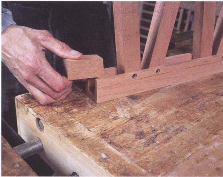
PHOTO E: The filler blocks at the bottom of the legs are necessary for strengthening the leg at this crucial point.
