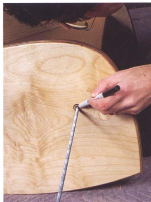
PHOTO I: Slip the threaded rod with one of the cap nuts all the way through the holes in one side and mark where the rod comes out the counterbore on the other side panel of the rocker.
