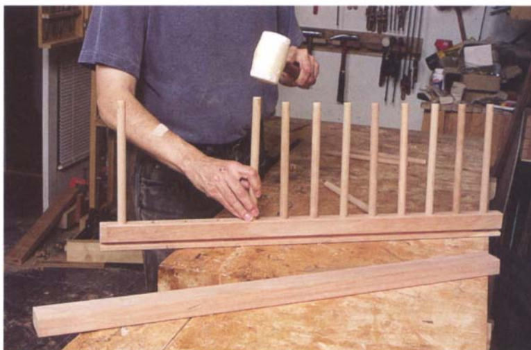
PHOTO E: Insert all of the dowels into one of the lower side rails first.
