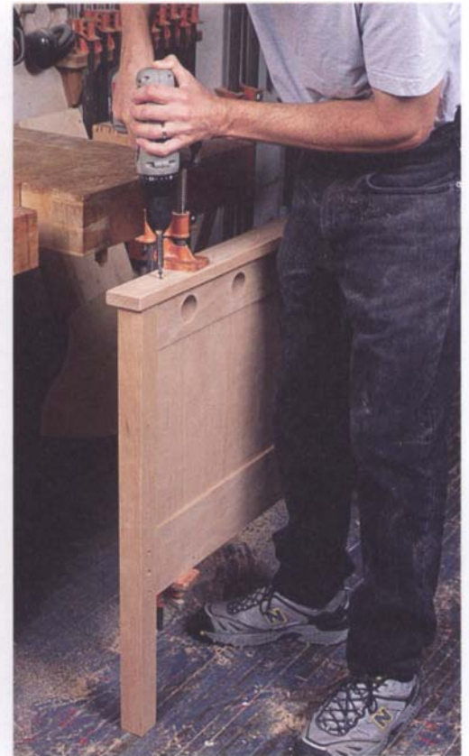
PHOTO H: With just a little bit of glue on the top of the upper rail, position, clamp, and then screw the cap into place.
