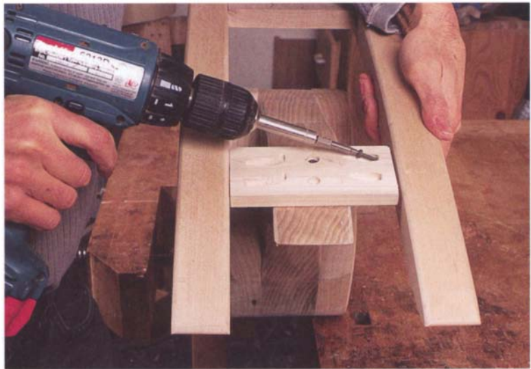
PHOTO I: Screw the crosspiece in place after attaching it to the tail.
