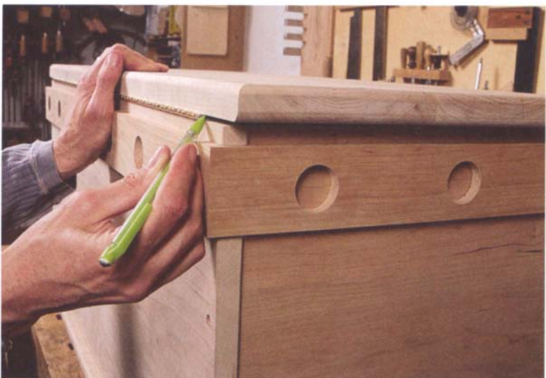
PHOTO H: Mark the hinge location on the underside of the lid after centering the lid on the chest.
