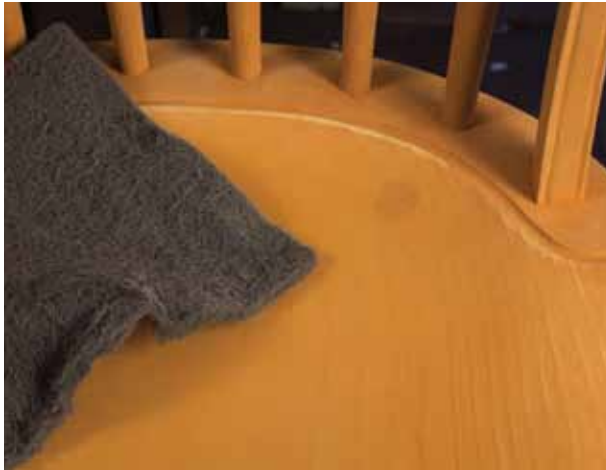
FIG. 25.22 The goldenrod paint after being rubbed out with a Scotch-Brite pad.
