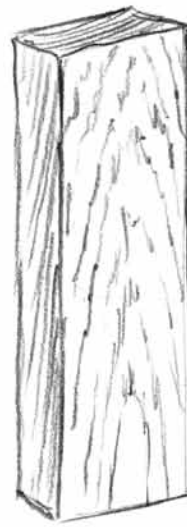
A highly figured board is a sign that the fibers are not parallel to the surfaces.
