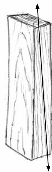
Inspect the edge of the board to ensure that you follow the fibers.
