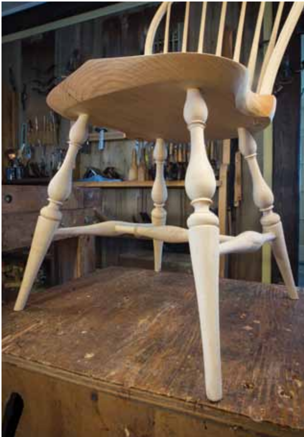
FIG. 25.10 Inspect the legs for grime or glue and sand accordingly.
