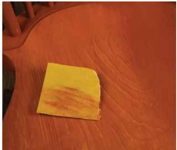
FIG. 25.17 The seat sanded after the first coat of red paint.
