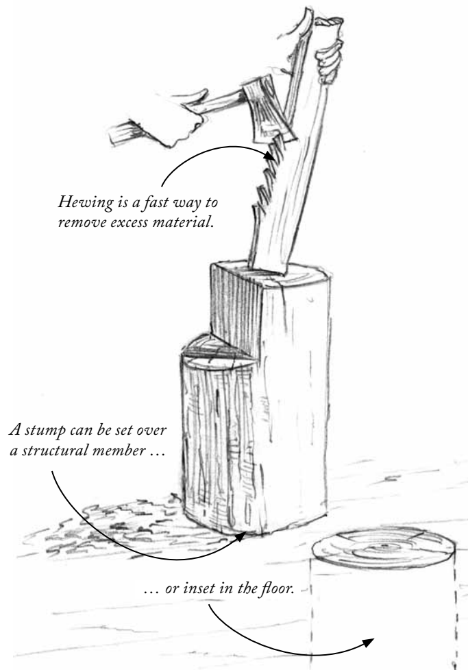
FIG. 4.4 I like to keep a stump handy for hewing away material from workpieces with a hatchet.
