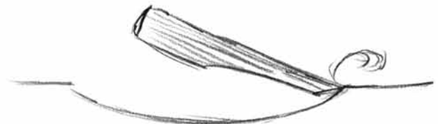
... while the high clearance of the bevel-down drawknife can carve with ease.
