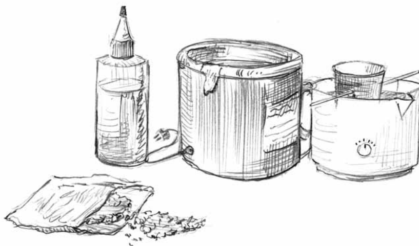
FIG. 2.7 Glue pot options: premixed liquid hide glue, a dedicated glue pot (center) and an electric pot (right).
