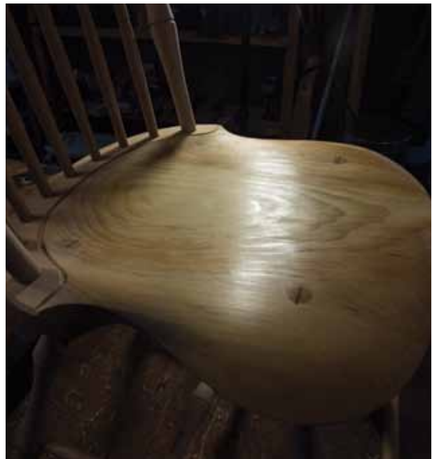
FIG. 25.11 Rinsing the seat with naphtha cleans the surface and can reveal surface quality.
