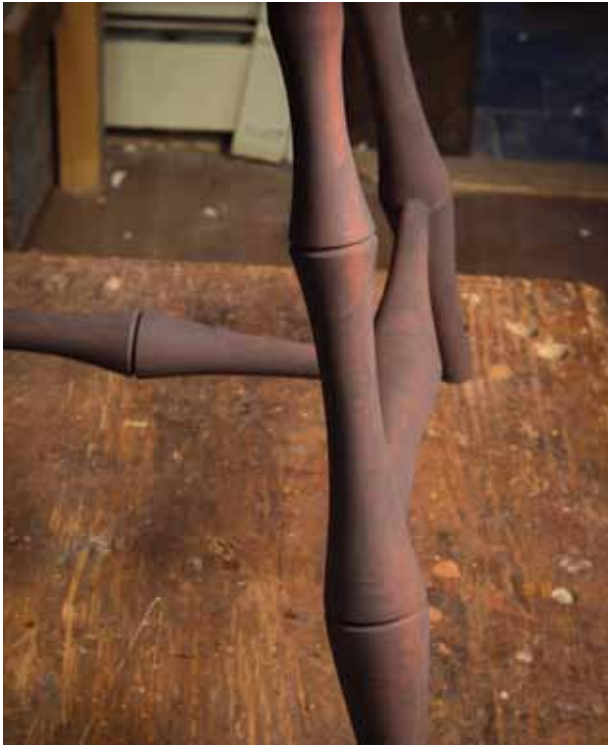
FIG. 25.19 The pinkish tones of the undercoat show through after the first coat.
