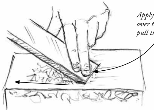
FIG. 5.12 Good honing relies on holding the stone and the blade in a stable position.
