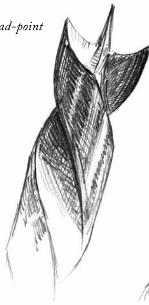
FIG. 16.11 Shop-made brad-point and Bismark bit.
