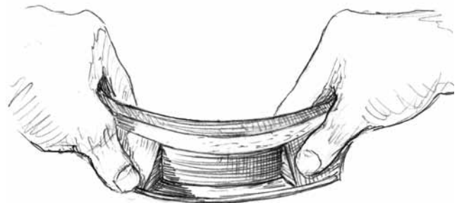
FIG. 19.24 Hand position and pressure is essential to travisher technique.
