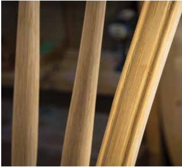
FIG. 25.6 Wetting scraped and sanded areas raises the compressed fibers.
