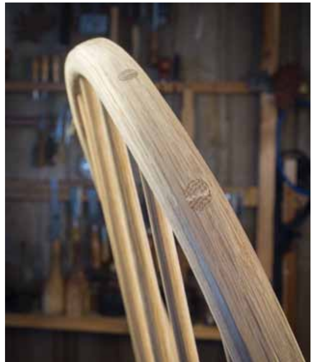
FIG. 25.9 Most surfaces on the oak can be finished with spokeshaves, leaving an inviting faceted surface, ready to finish.
