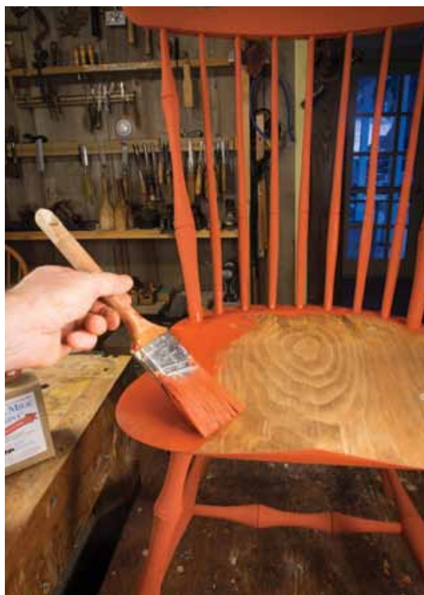
FIG. 25.15 Be sure to work the paint back along a wet edge to keep from painting over the paint that has begun to dry.
