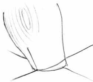
FIG. 17.12 Orienting a leg's tapered tenon with the tapered mortise in the seat.
