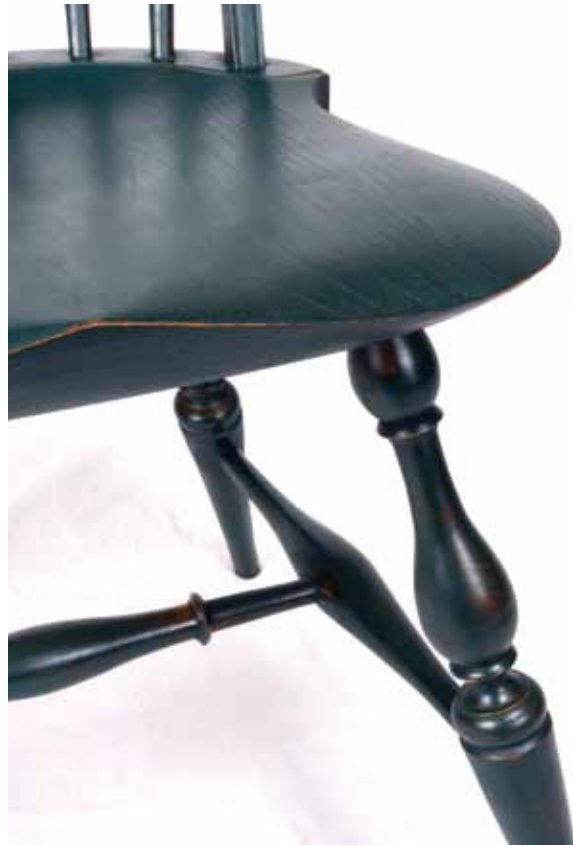
FIG. 25.27 The process of burnishing and oiling tends to reveal the undercoat, which adds visual interest when viewed close up.
