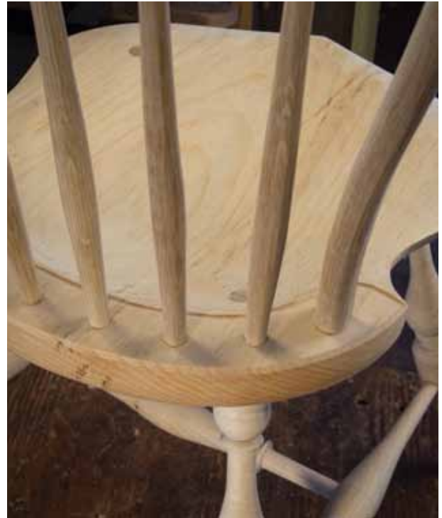
FIG. 25.7 Check every joint for glue residue, especially in the highly visible areas.
