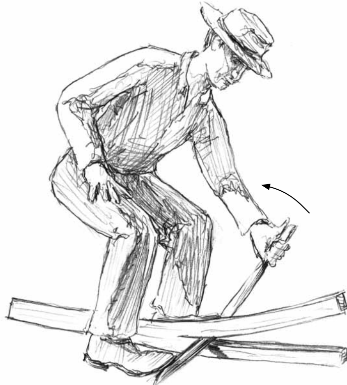
Then set the light side on the ground and stand on both sides of the froe to finish the split.
