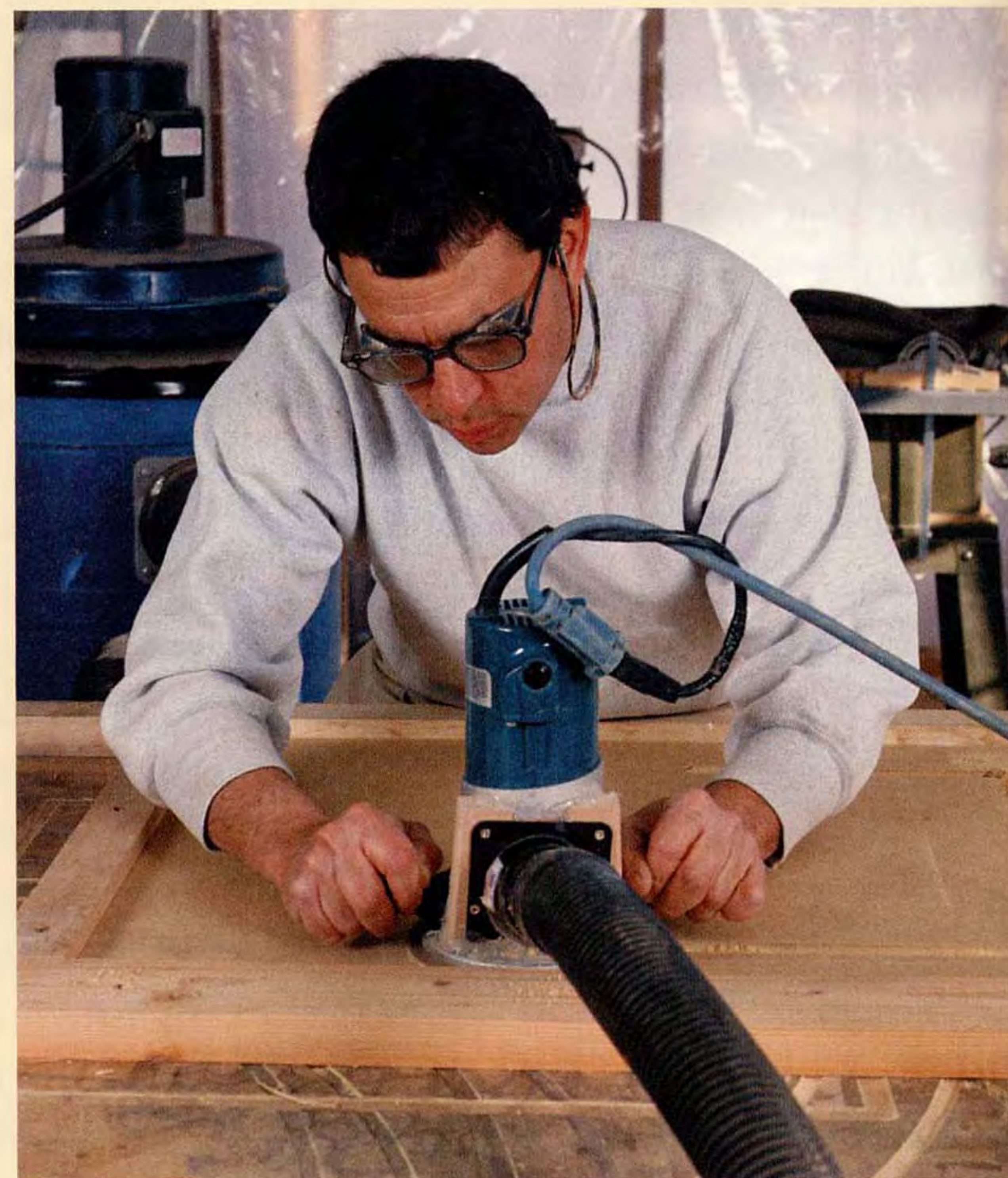
Routers turn MDF into cabinet door. Straightedge boards hold the panel in place and serve as guides for the routers.
