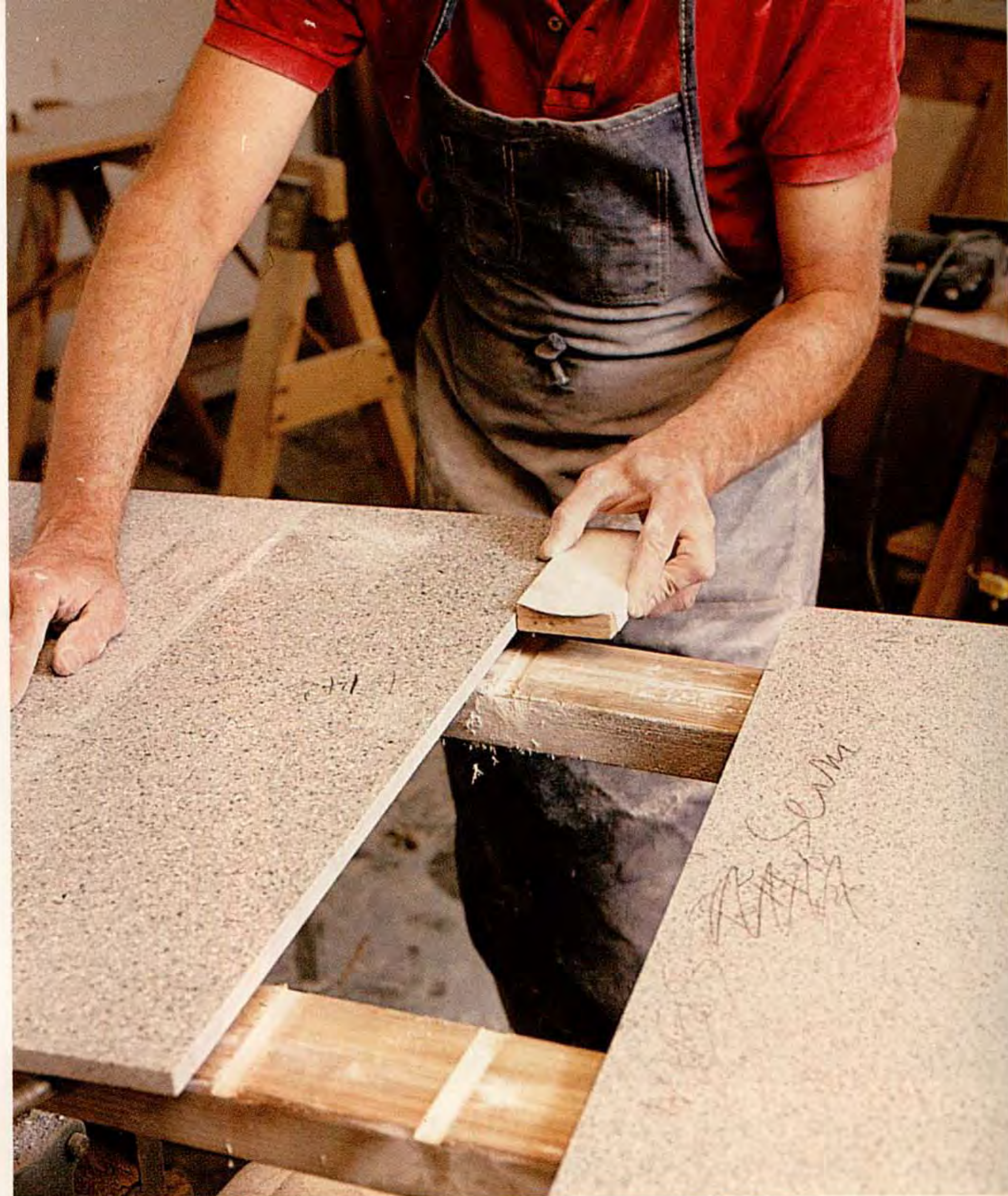
Edge treatment. Prior to glue up, mating edges are cleaned up with a sanding block. This block is made with a sticky-backed disk stuck to a hunk of plywood.
