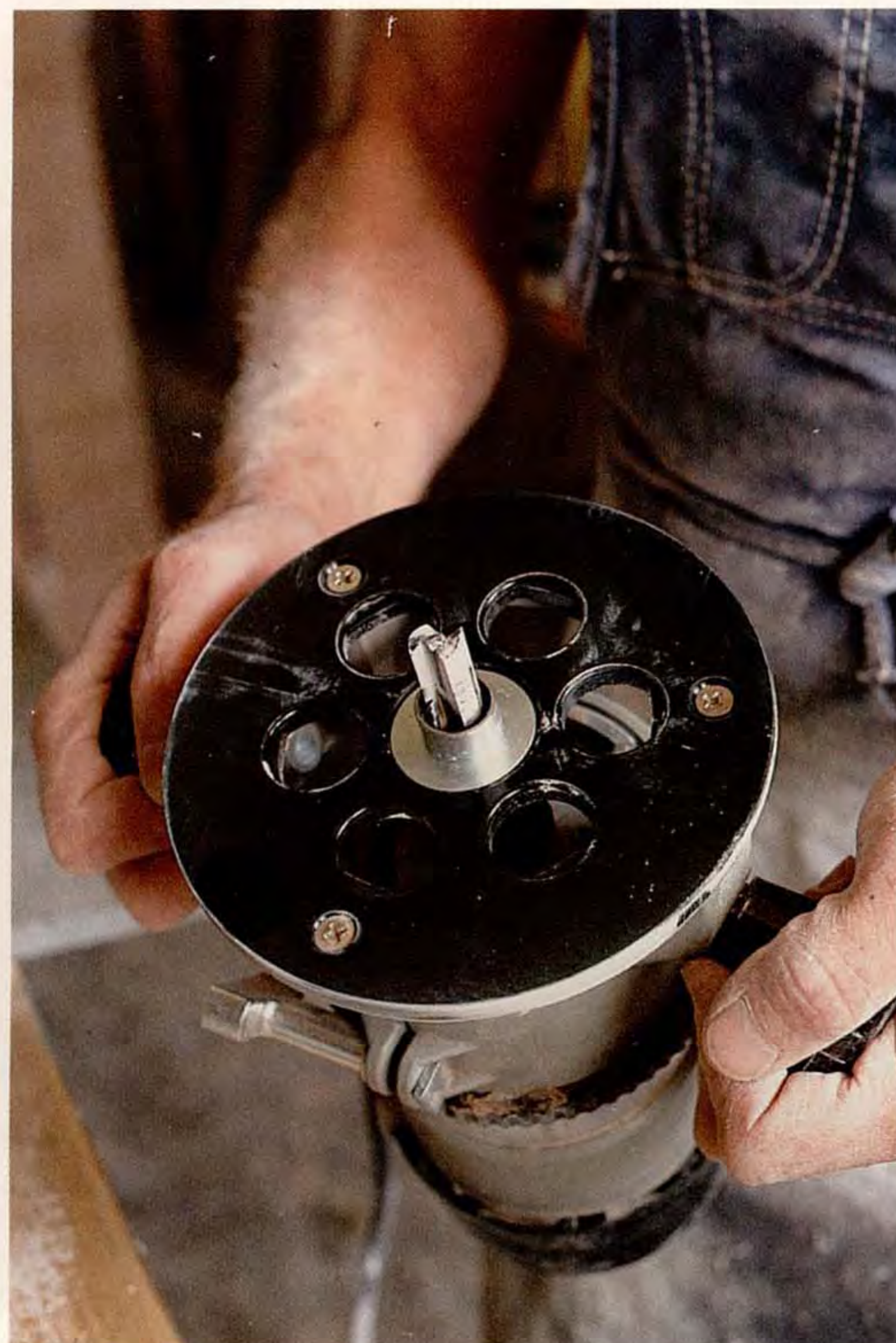
Collar and bit. A metal sleeve called a collar, or template guide, rides along the edge of the cutting guide and separates the guide from the 1/2-in. straight-flute bit.
