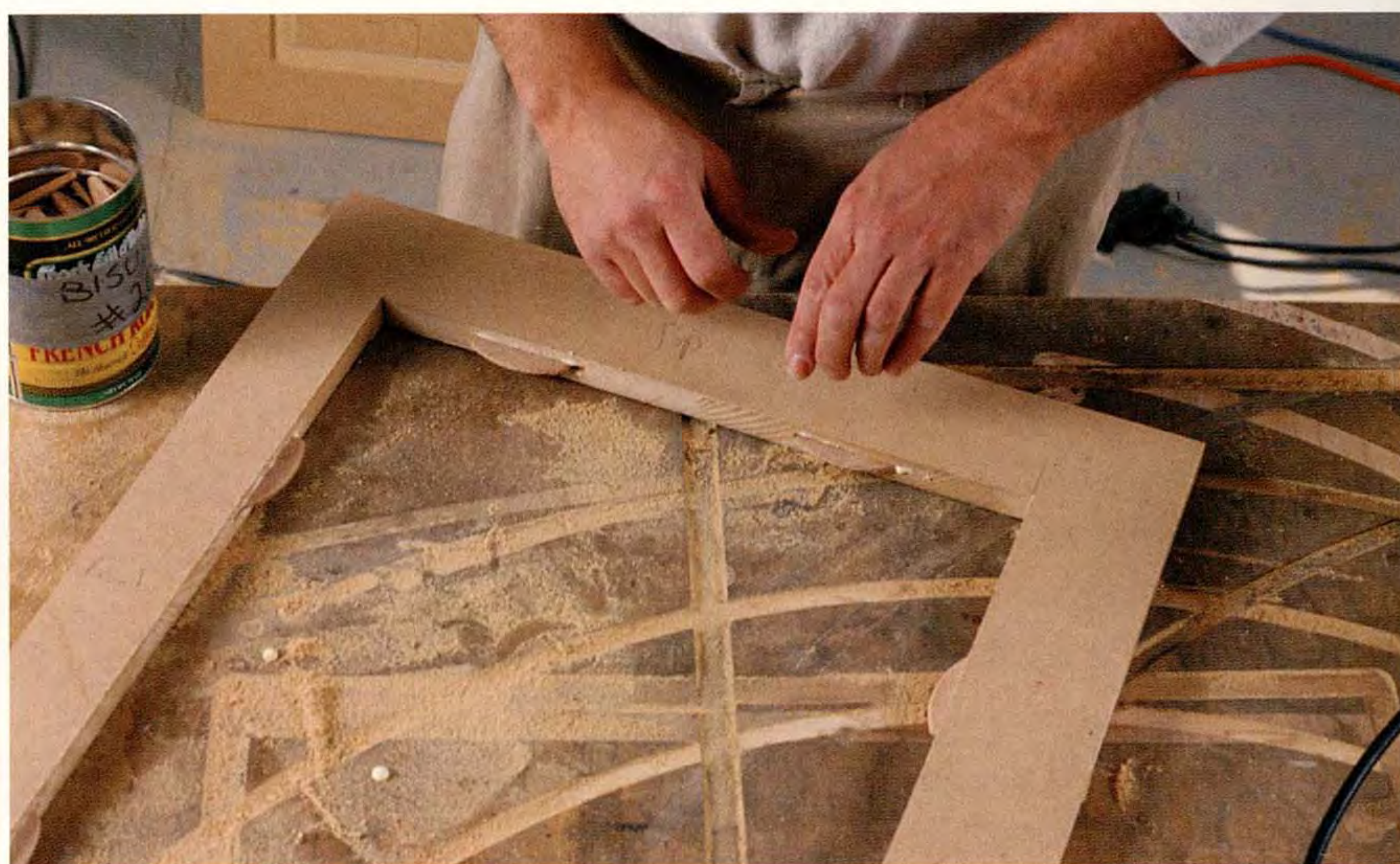
Biscuits act as stops for raised panel. The raised panel will be supported by biscuits inserted in the edge of the face frame. The biscuits hold the field of the panel proud of the frame.
