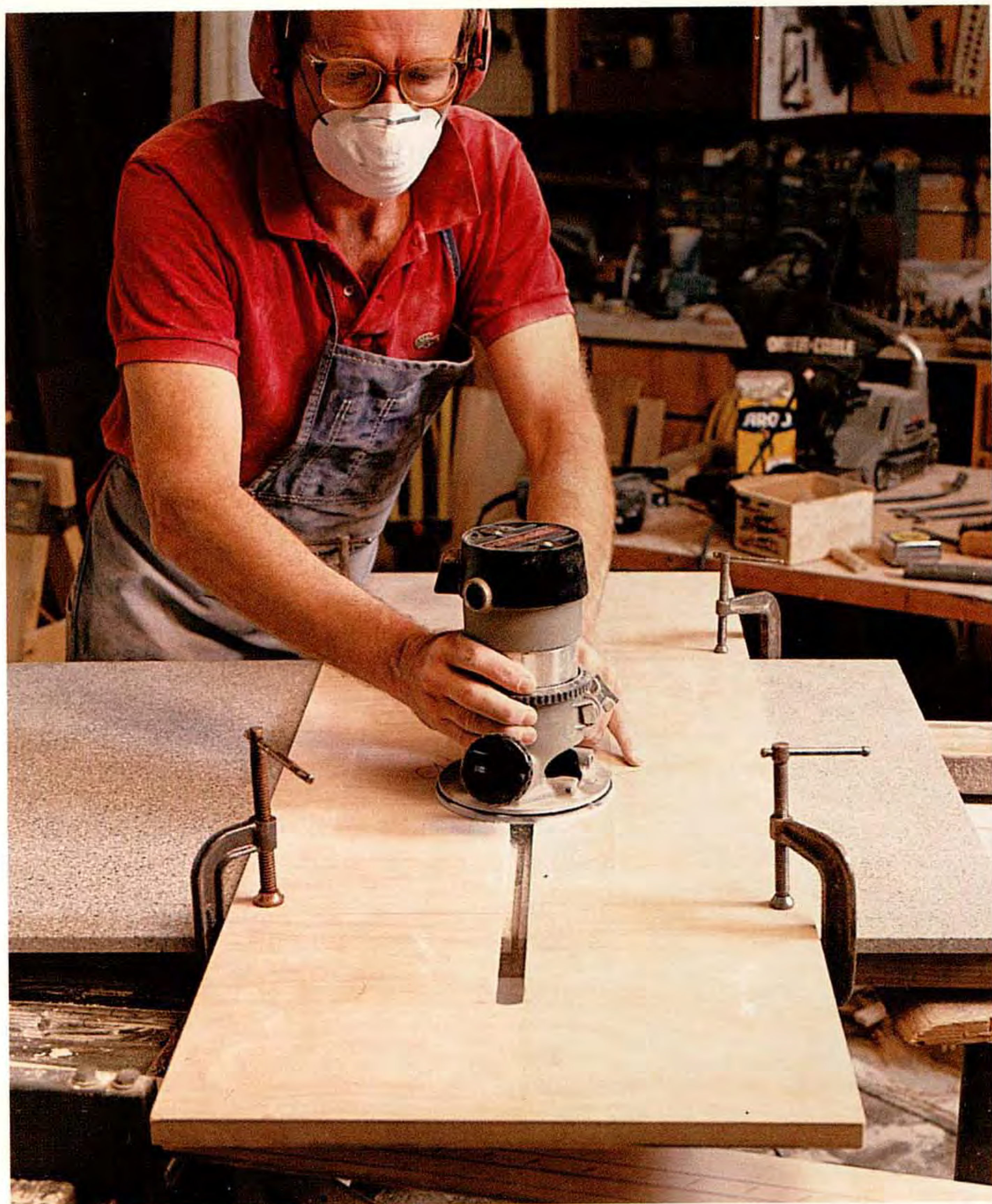
Mirror jig. A slot down the center of the mirror jig guides the router's collar as abutting pieces of counter are jointed simultaneously.
