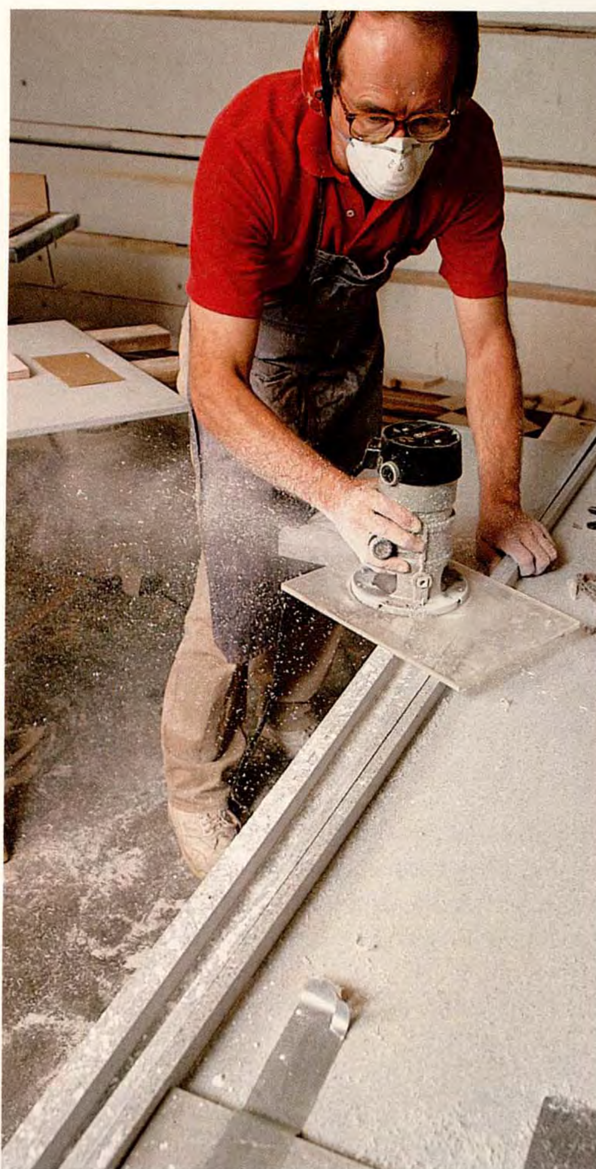
Bullnosing. As he rounds the inside corner, the author supports the router's custom base on edging strips. A dusting of cornstarch greases the track.
