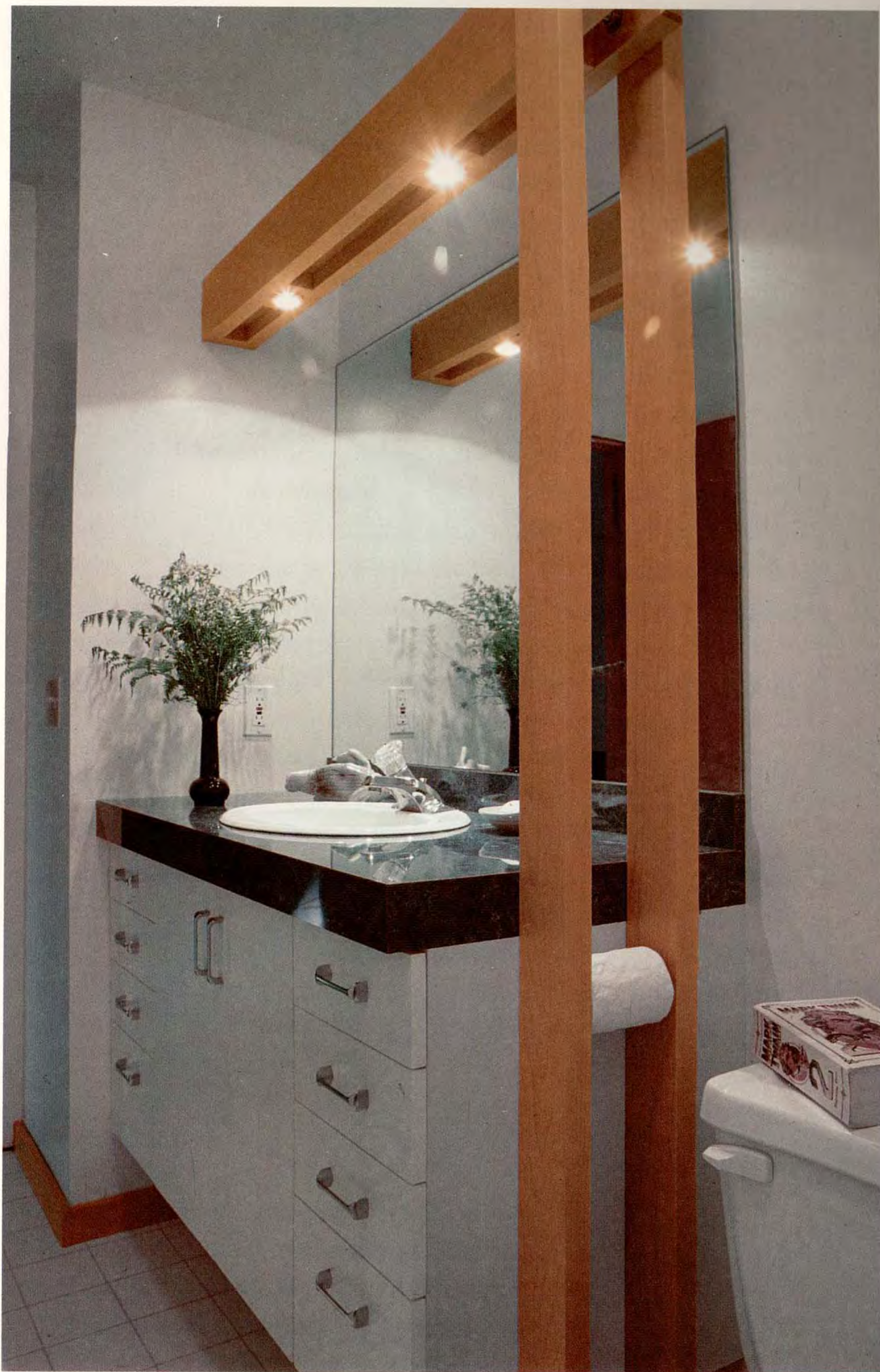
A durable, easy-to-clean surface. Melamine-laminated panels are easy to make into furniture or cabinets, such as this bathroom cabinet of melamine with a plastic-laminate counter surface. Melamine doesn't need finishing and can be machined with tools found in the standard home shop.
