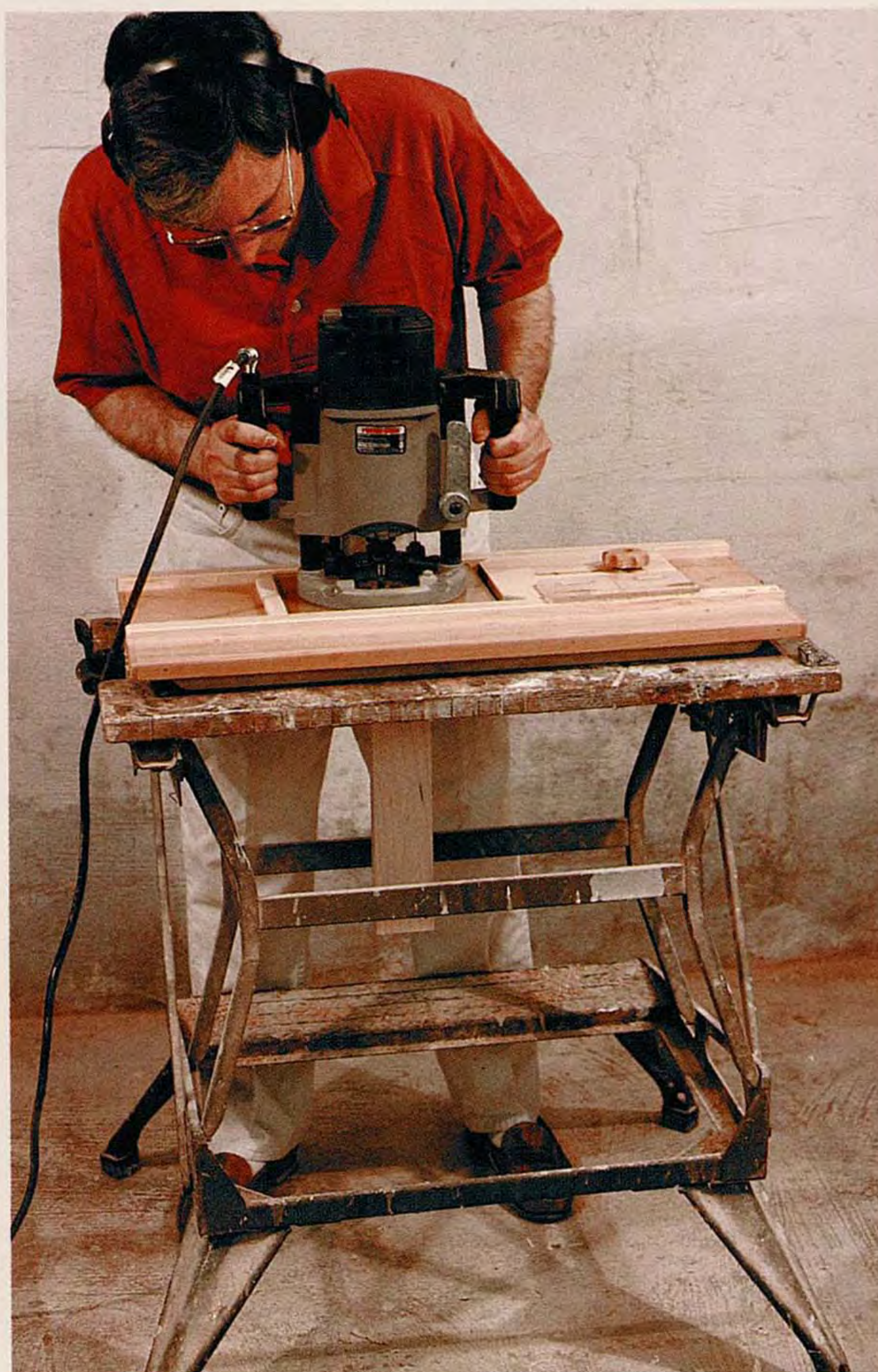
Using the fixture. A quick side-to-side pass with a ⅜-in. straight bit in a plunge router cuts a mortise whose length and width are limited by the fixture's rails and stops. The author uses a Workmate® to clamp the fixture and the workpiece simultaneously.
