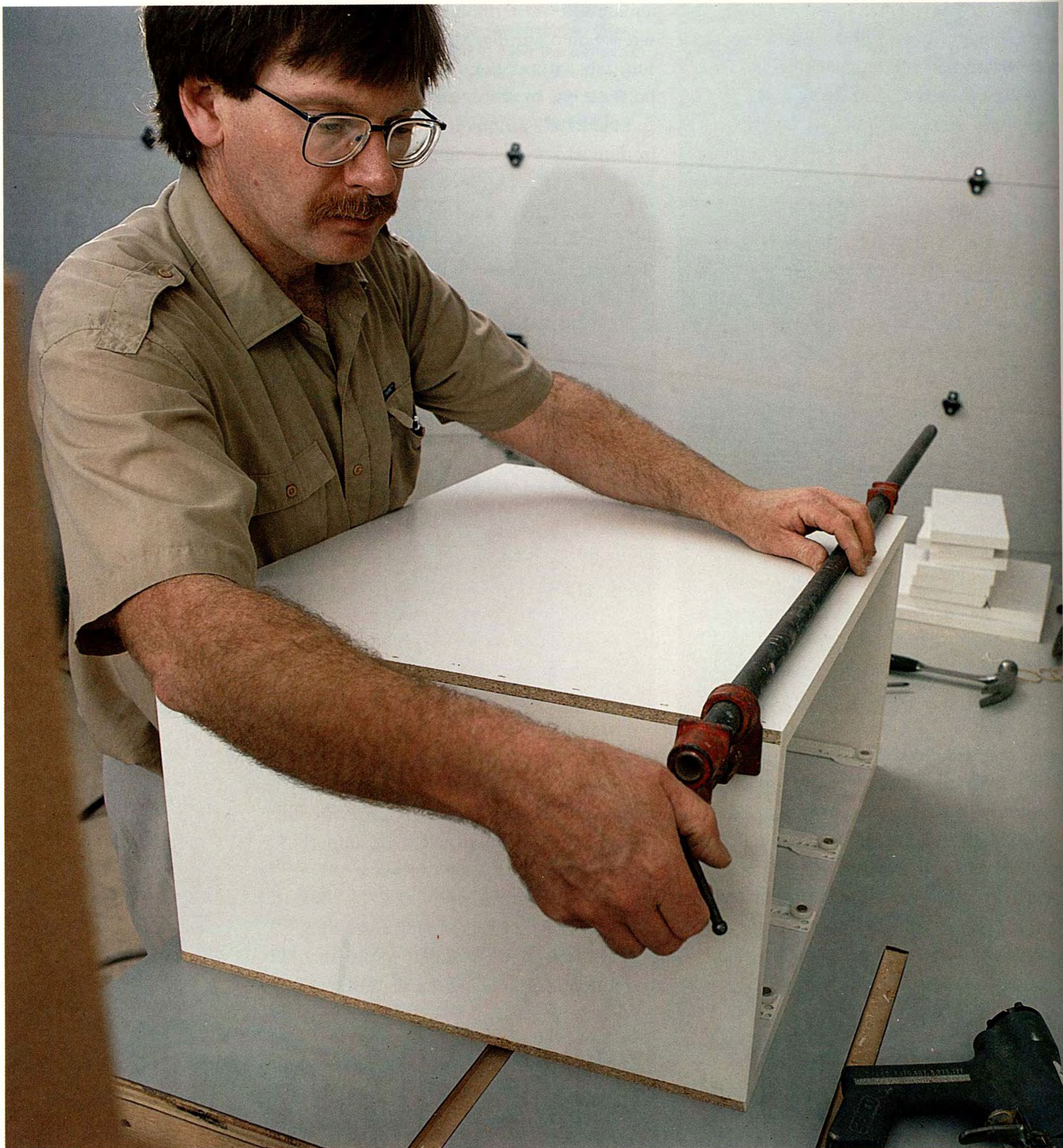
Rabbeted edges are glued and clamped. Glue doesn't stick to laminate, so the author rabbets, glues, and clamps the pieces to get a tight, durable fit.
