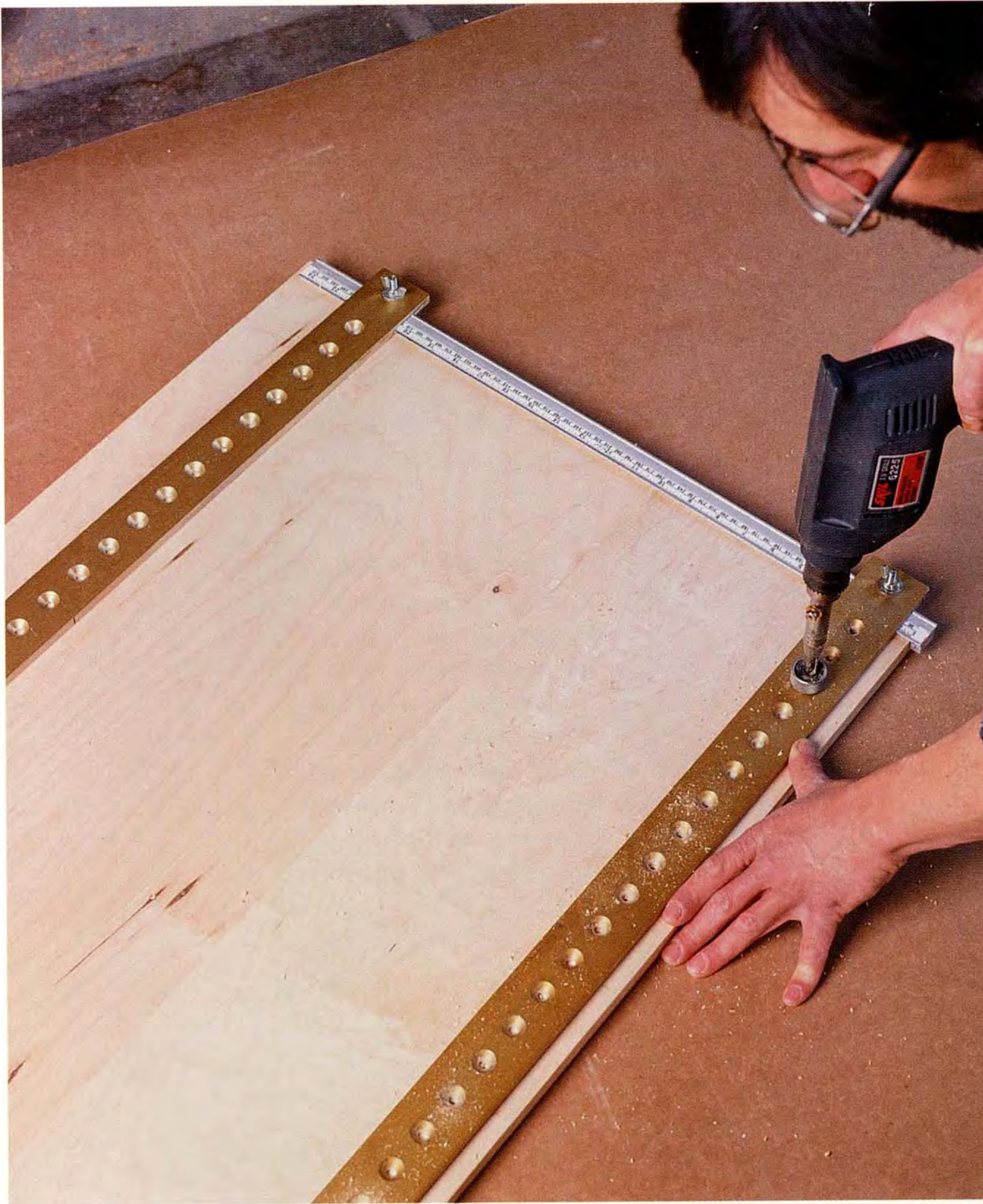
Drilling jig. Tolpin drilled 5mm holes in the carcass sides for attaching hinge plates, drawer slides, and shelf clips using his portable drill with a special drilling jig.
