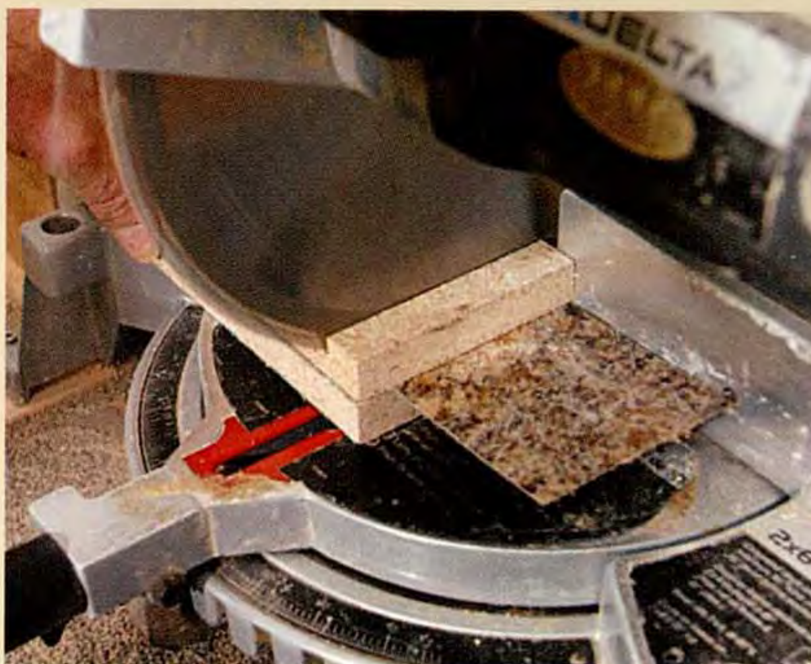
2. A laminate sandwich makes for clean cuts.
