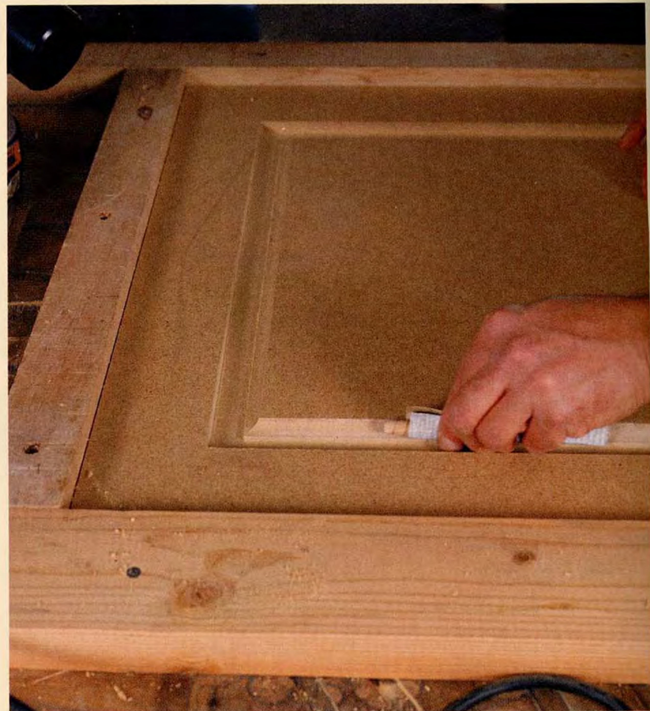
Sandpaper smooths the routed profile. The groove in the door has nearly square corners made with a \frac{1}{4} -in.-dia. flush-cutting router bit.
