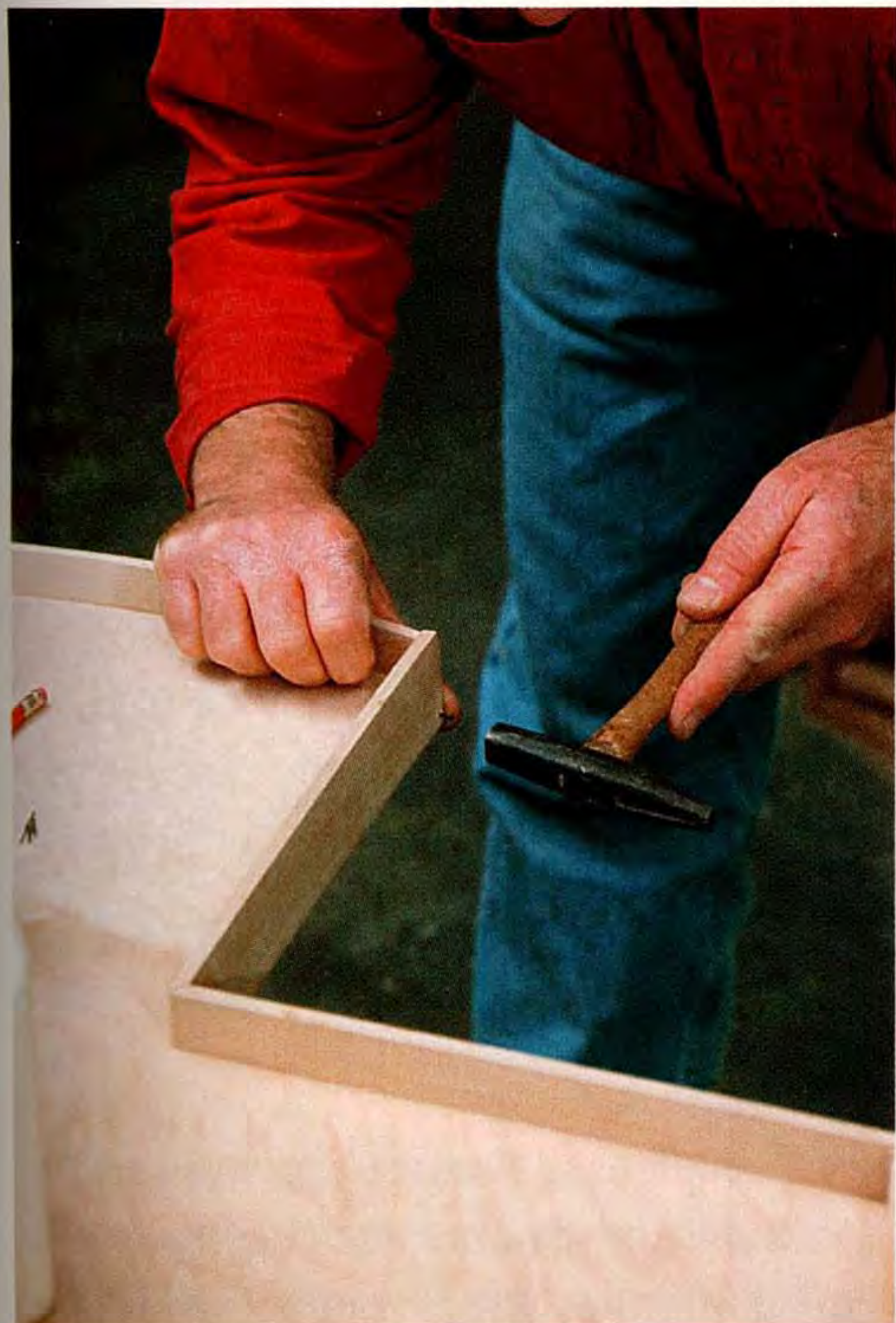
Outside corner is reinforced with brads. A potential trouble spot is the outside corner of the carousel, where edging pieces meet. Here, the author adds some \frac{3}{4} -in. brads. Drilling pilot holes will prevent splitting.
