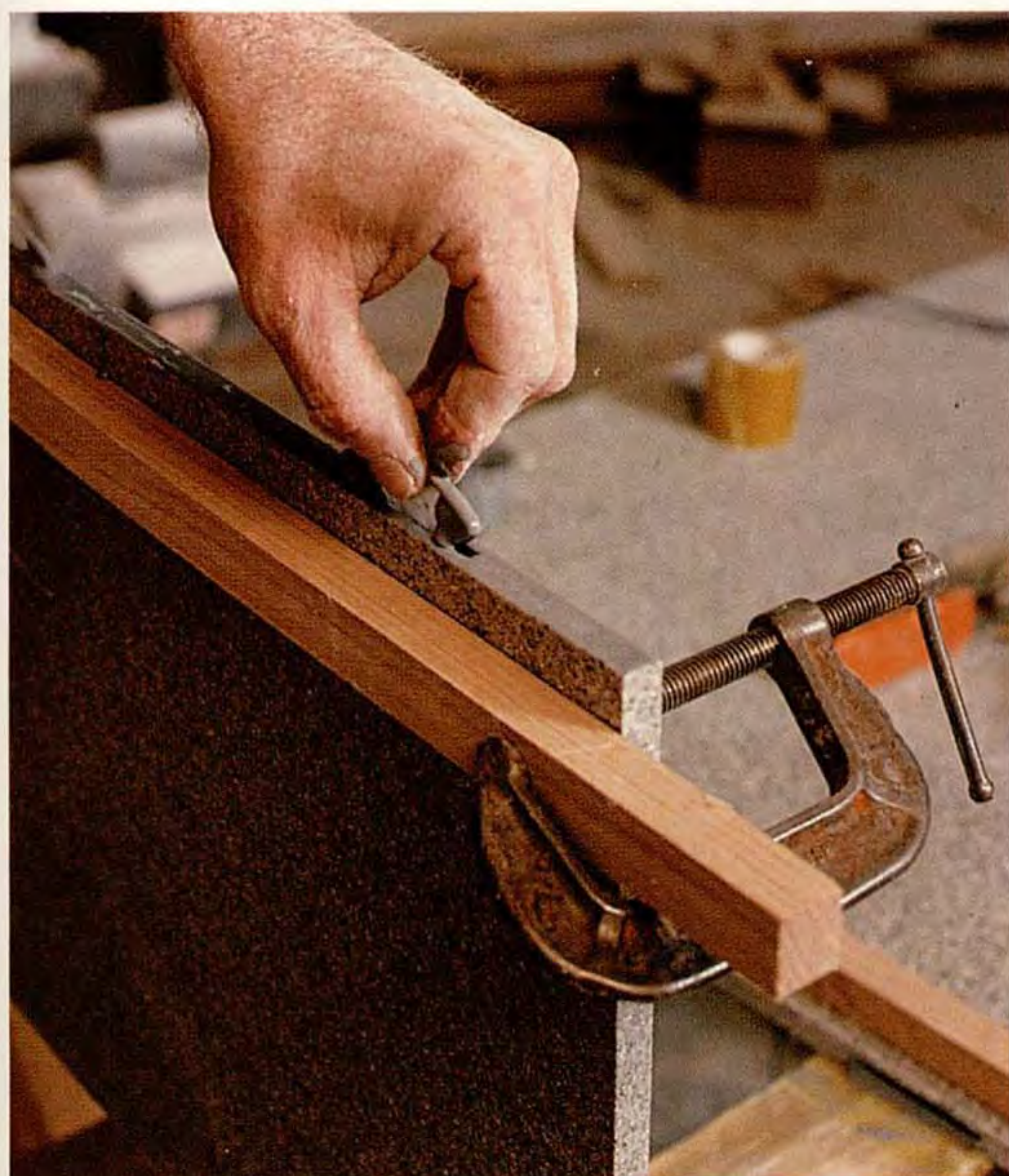
Plastic biscuits. Butt seams between mating pieces are aligned and strengthened with biscuit joints. Note the gray glue, custom mixed to match the material.
