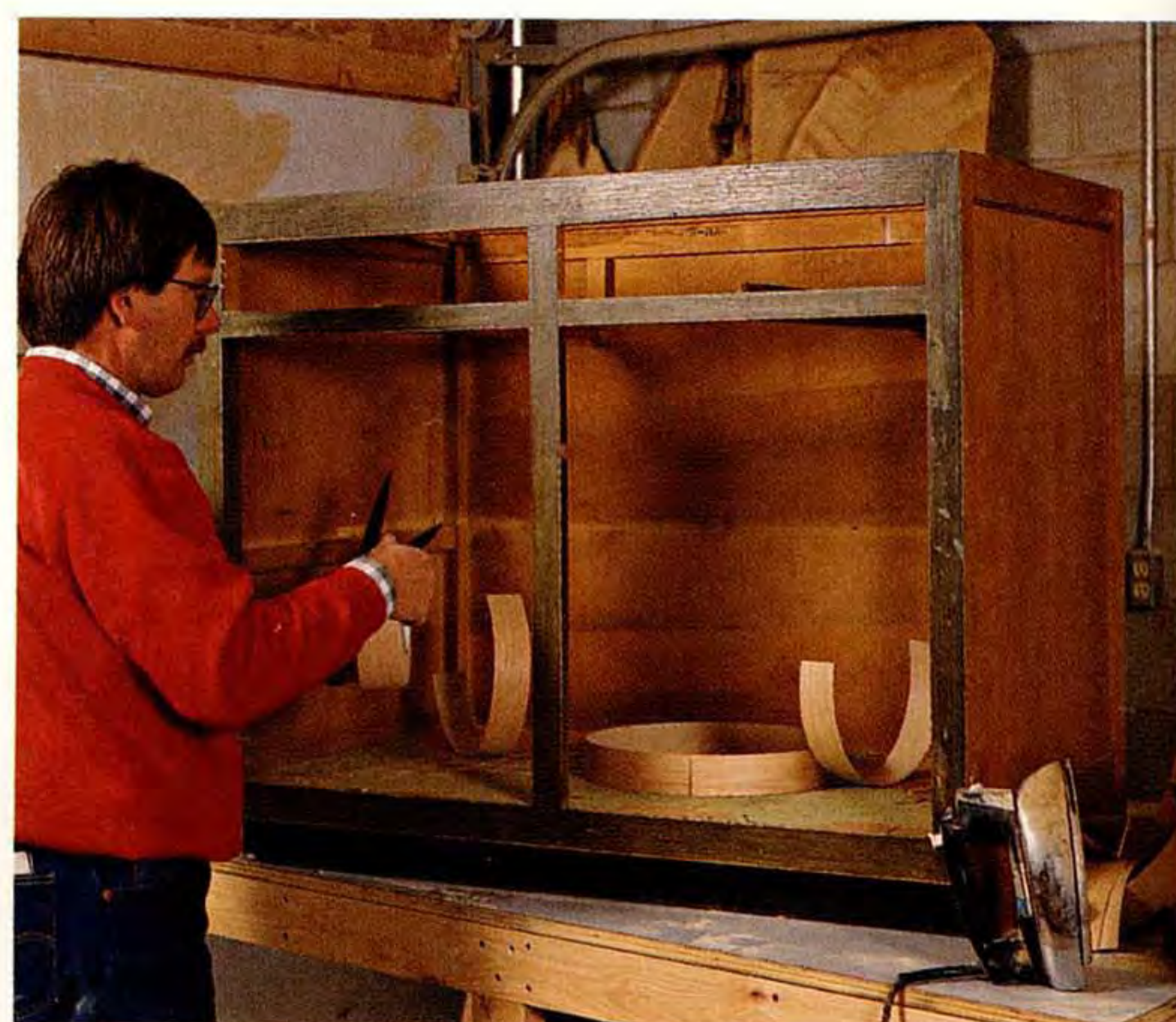
Shop demonstration. In his shop, the author cuts veneer roughly to size before demonstrating the refacing technique. The cabinet is from the kitchen shown on the facing page.
