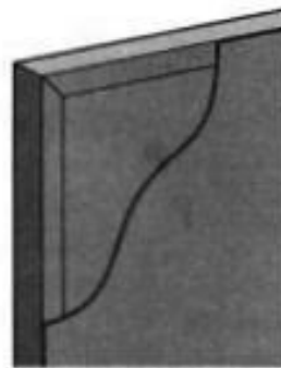
Plywood with mitered edge bands, veneer over assembly
