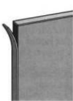
Plywood with taped edges
