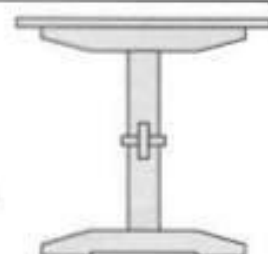
Contemporary I-Section Trestle End
