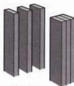
Gluing up a leg blank
