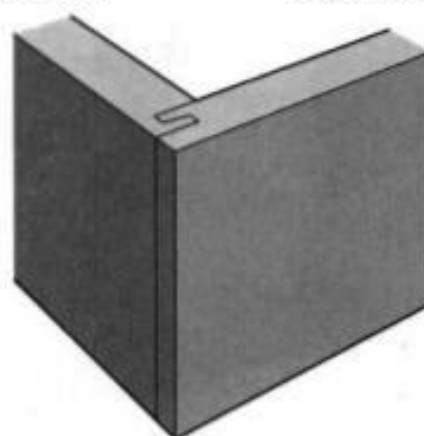
Routed Drawer Lock Joint
