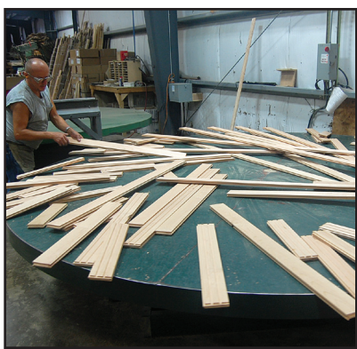
Cut flooring pieces are fed to a turntable, where they are graded. There is one common grade and a rustic grade with more knots and defects.
