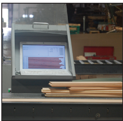
Random flooring strips are fed into one end and nested bundles are produced at the other end.
