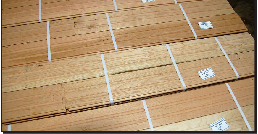
Heister House is currently producing a bundle with five layers, three pieces wide, but they can vary in width.
