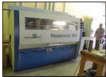
Weinig Powermat 500 moulder is one of the key machines for Luttrell's millwork operation.
