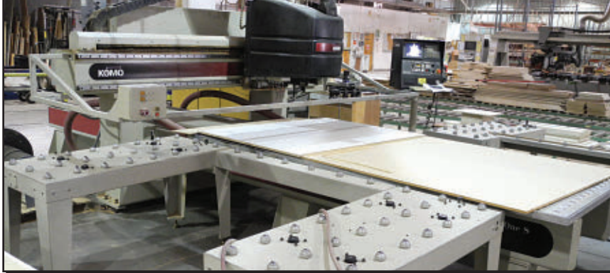
Komo router used to cut MDF pieces for foil doors benefits from Router-Cim software.
