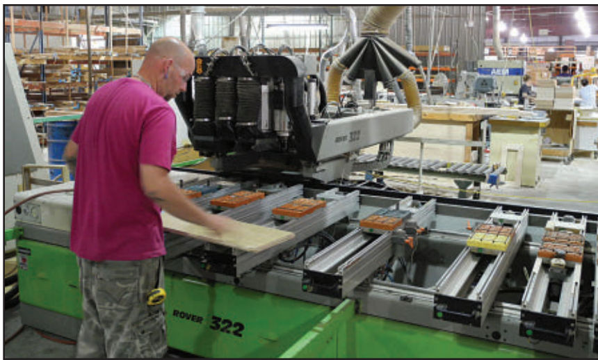
One of three Biesse Rover point-to-point machines in the Florida cabinet plant.
