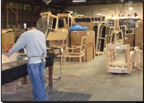
Before lean, the frame area had huge disorganized stacks of work in progress.
