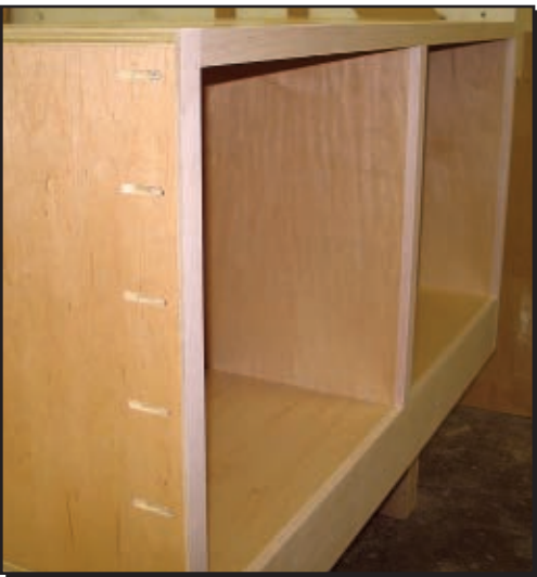
Sartini uses pocket hole construction to affix face frames to cabinets. Pocket holes are cut on a Castle machine.
