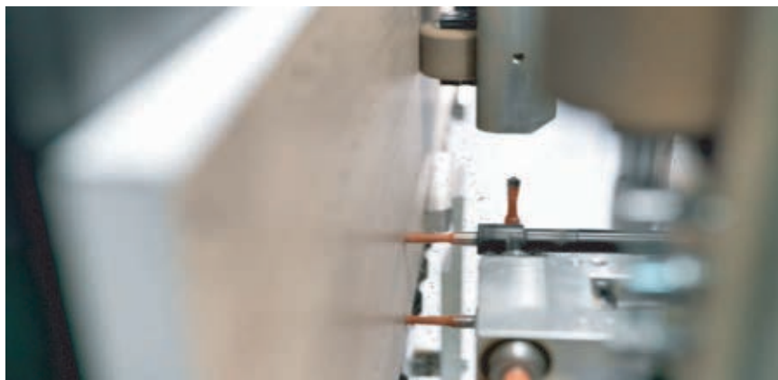
Sartini uses pocket hole construction to affix face frames to cabinets. Pocket holes are cut on a Castle machine.
