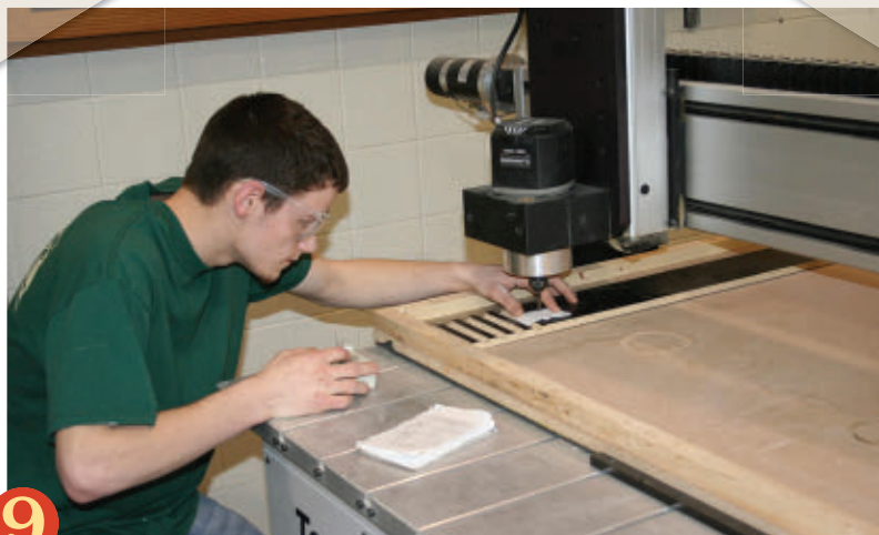
A student uses a Techno CNC router to make slots for a DVD tower holder as part of the cabinetmaking program at Mahoning County Career and Technical Center.
