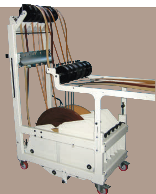
2 or 6 roller vertical magazine with automatic edge change over (optional)
