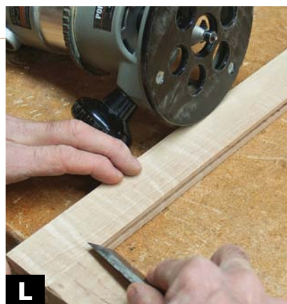
USE A STRAIGHT chisel to cut the miters in the corners of the doors.
