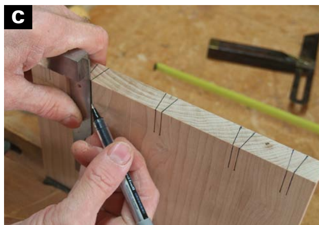
EXTEND THE MARKS down to the gauge line on the outside of the stock. Use a small square to guide the pen or sharp pencil.
