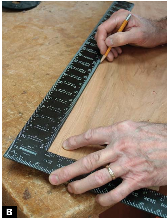
FIND THE CORRECT ANGLE to cut the front of the top and bottom. Lay a square on each side and draw from the corners to center.
