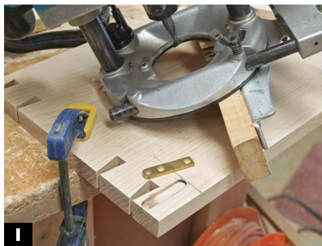
ROUT THE MORTISES FOR THE KNIFE HINGES. Use a \frac{3}{8} -in. straight router bit. The fence keeps the bit the precise distance from the edge and penciled points indicate stopping and starting locations for the router.
