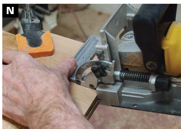
CUT #0 BISCUIT SLOTS at a 15° angle where the two roof sections meet.
