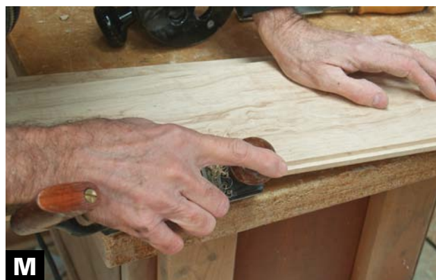
CHAMFER THE EDGES OF THE RAISED PANEL. Plane the end grain first and then the grain along the sides of each panel.
