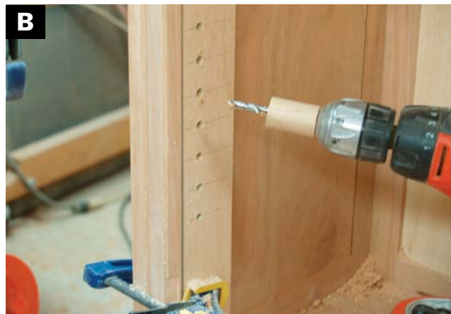
MAKE A DRILLING TEMPLATE to position the shelf pin holes. A piece of dowel serves as a stop.
