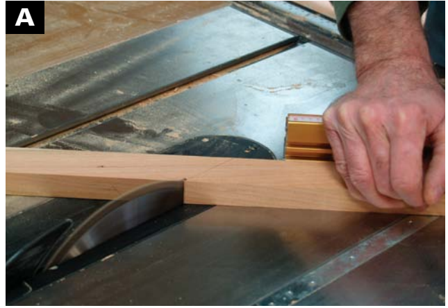
TO MAKE THE PARTS FOR THE TOP MOLDINGS, use a miter gauge set to 45° and cut on the tablesaw.
