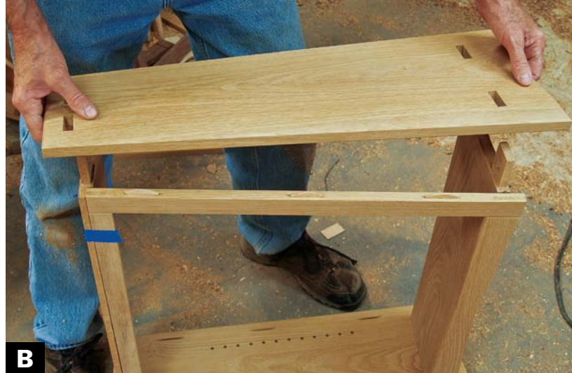
PUT THE WEDGES IN ONE SIDE to hold the parts tight while you align the other side over the tenons.
