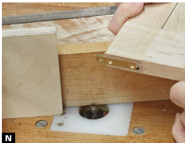
CUT THE HINGE MORTISES with a 3/8-in.-dia. router bit. The stop block is carefully placed to control the length of the cut.
