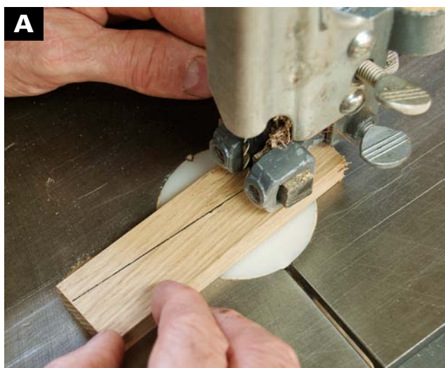
CUT WEDGES FROM 1/2-IN. STOCK. The rough size is 1 1/4 in. × 5 in. You'll trim and shape the wedges after assembly.
