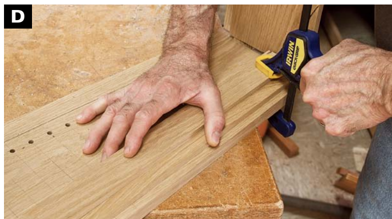
CLAMP A GUIDE PIECE TO THE SIDE to align the biscuit joiner. Place the clamps so that they will not interfere with the cut.
