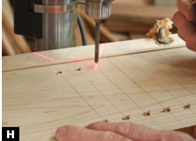
H DRILL \frac{1}{4} -IN. HOLES FOR THE SHELF SUPPORTS. Clamp a fence to the table to align the holes a uniform distance of 1\frac{1}{2} in. from the edges of the stock.
