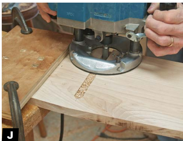
J ROUT THE FIXED SHELF with a \frac{3}{4} -in. router bit to a depth of \frac{5}{16} in. This groove will be for the drawer stop.
