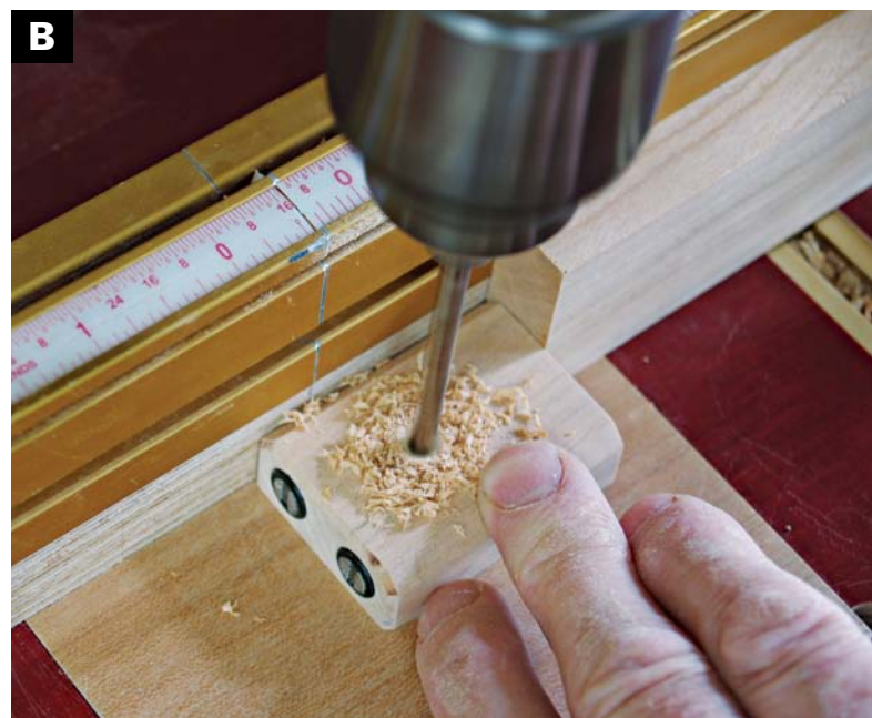
B DRILL AND COUNTERSINK a hole for the mounting screw. Install the metal catches on the doors, then drive the screw to attach the stop.
