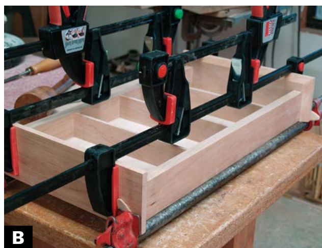
PULL THE JOINTS TOGETHER with clamps after the biscuits and glue are in place.
