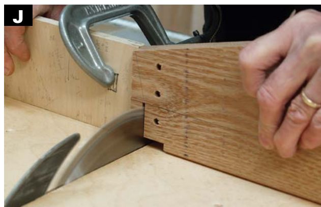
BEGIN TO SHAPE THE BACK GABLE on the table-saw using a crosscut sled and stop block.
