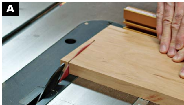
MAKE THE CUTS on each end of the top and bottom with the tablesaw miter gauge set to 5°.
