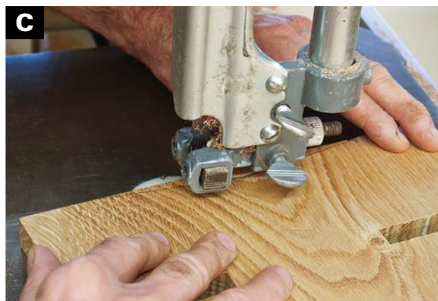
CUT THE BOTTOM PROFILE on the bandsaw, cutting from each side toward the center.
