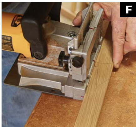
CUT MATCHING BISCUIT SLOTS in the stiles of the front panel and the hinge strips.
