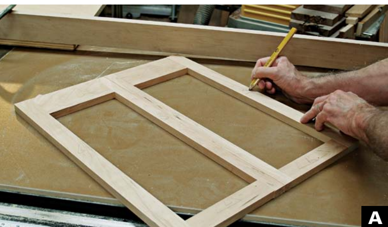
LAY OUT THE PARTS FOR THE DOORS and mark the stiles and rails in the position they will be assembled.
