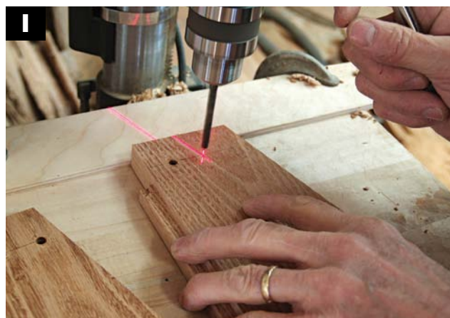
DRILL ¼-IN. HOLES FOR THE DOWELS in the front and back gables 1 in. on center from both sides. Set the drill press to drill through the stock.
