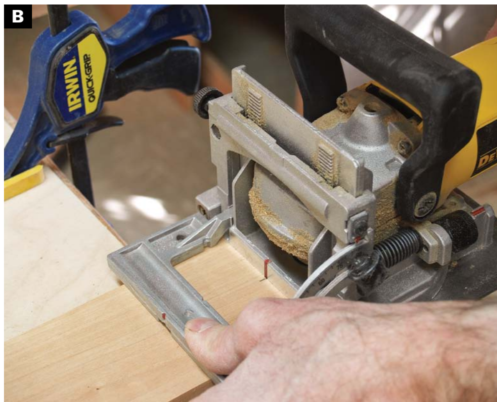
MARK THE CENTERS of each end of the rails and cut biscuit slots. Secure the wood to the workbench with a clamp.
