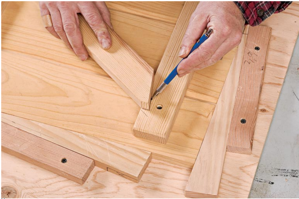
As an alternative to using the standard Z-brace, I extend the ends of the diagonal brace into the cross battens, producing a shouldered Z-brace.
