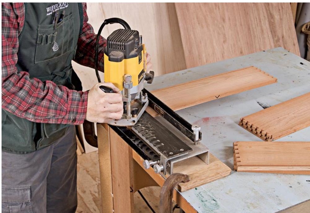
My trusty old Sears® Craftsman® router template speeds up the task of cutting dovetails for drawer boxes.
