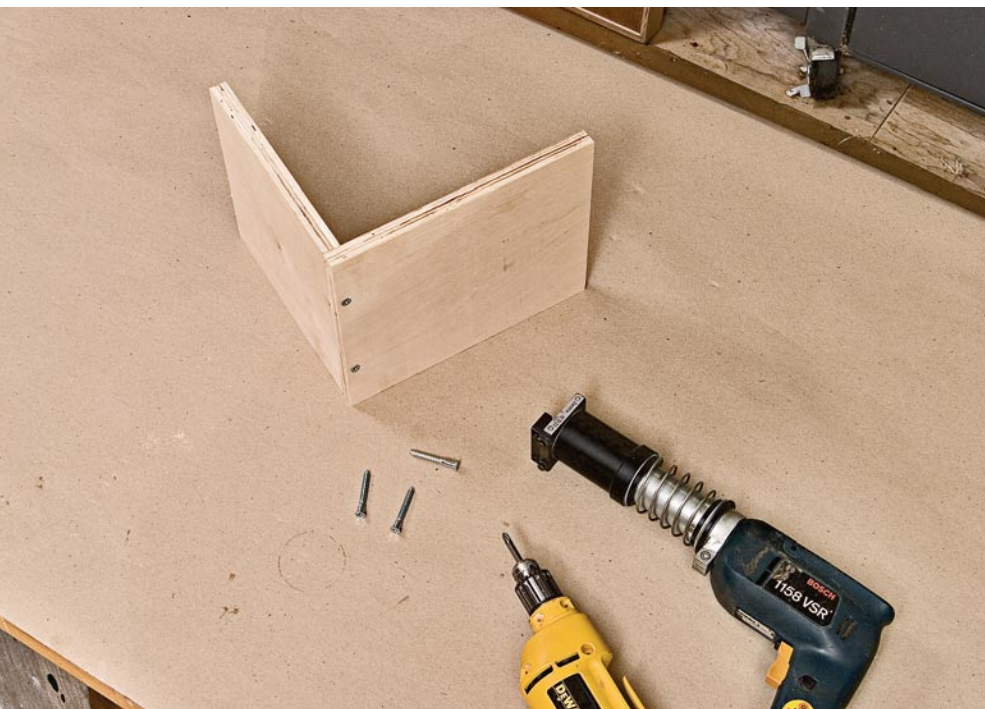
Incredibly strong case fastenings—Conformat® screws made by Hafele Co. are shown here—are quickly predrilled for use with a proprietary fixture and then installed with a powered screwdriver.
