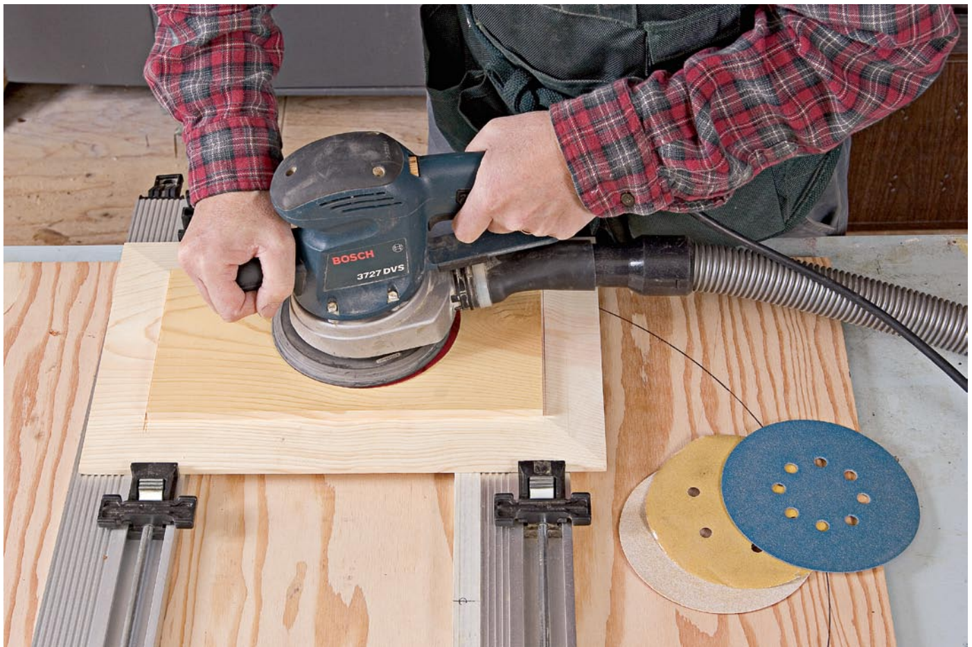
A random-orbit sander produces a better (more swirl-free) finish in less time than the older type quarter-sheet orbital.
