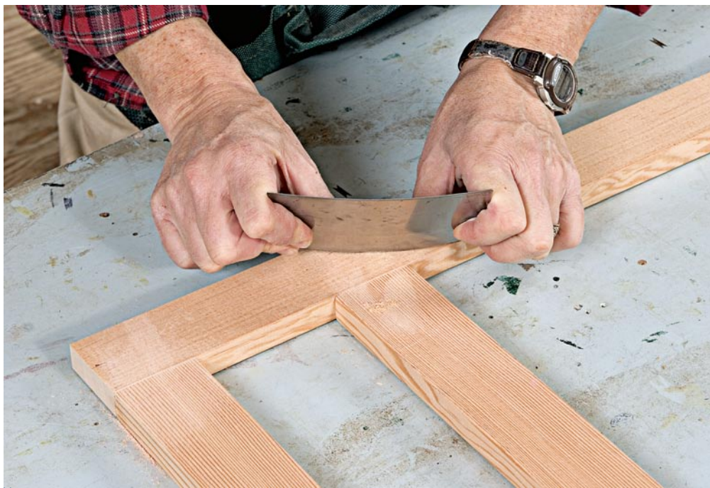
On hardwood, a cabinet scraper makes quick work of flushing the surface of each joint. I follow up with 180-grit sandpaper on a random-orbit sander.
