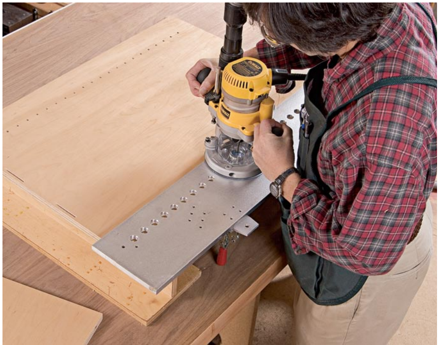
Using a commercially made jig by MEG® Products and a plunge router I can quickly create a precisely spaced line of holes for shelf clips.
