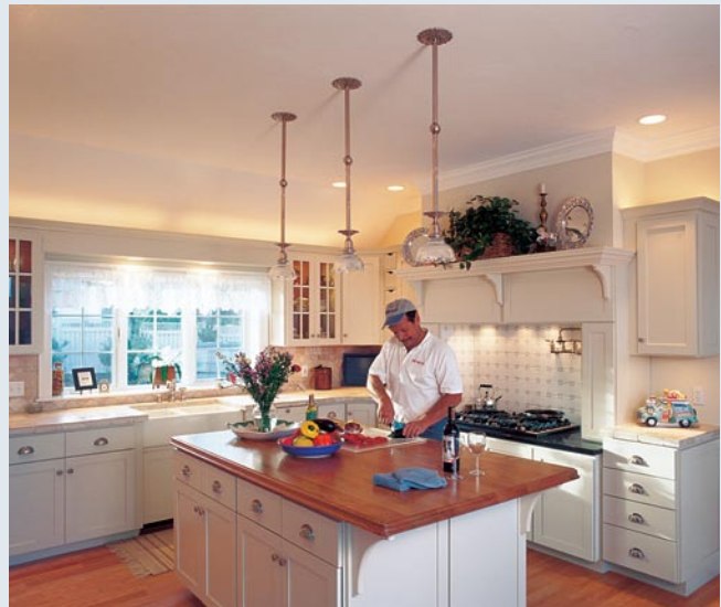
The natural light flowing through the generous windows of this kitchen—along with up-lighting installed above the upper cabinet cornice—provide all the ambient lighting needed (at least during the day).
