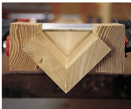
Here is one method that works well for holding the leg assembly square during gluing.
