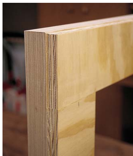
Here you can see the \frac{1}{16} " lip created by the straight moulding when attached to the inner top panel.
