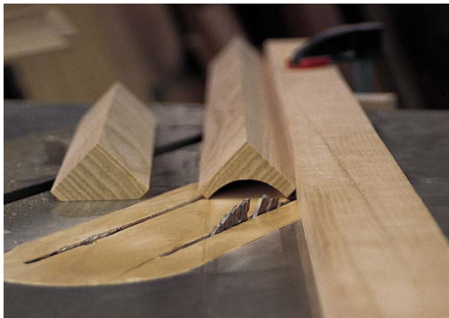
Cove moulding on the table saw is safe if done correctly. It works best if you use a sharp, carbide-tooth blade.
