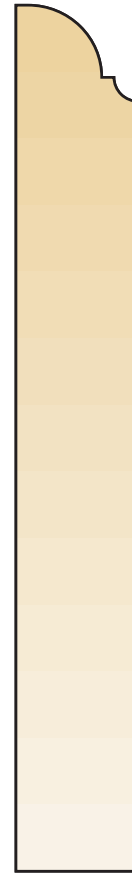
FULL-SCALE BASE MOULDING
