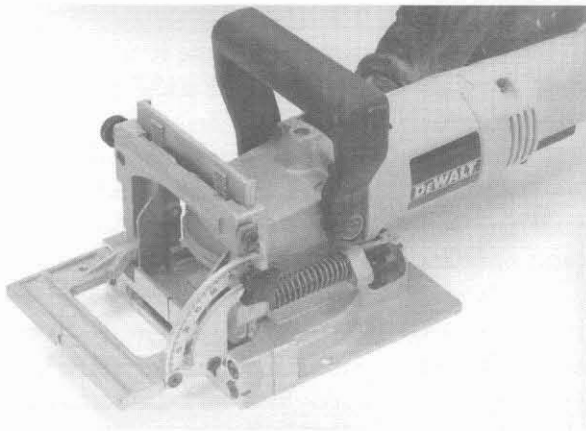
A plate joiner is a great addition to any woodworking shop.
