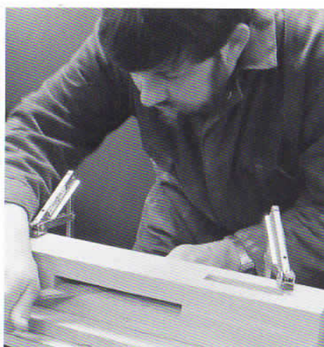
photo 2: Trimming the settle mortise with a file
