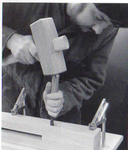
photo 1: Trimming the settle mortise with a chisel
