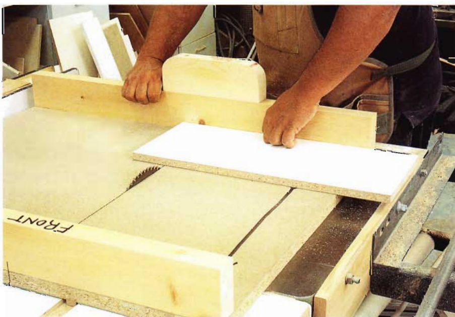
Here's the crosscutting sled you'll be building in this demonstration.
