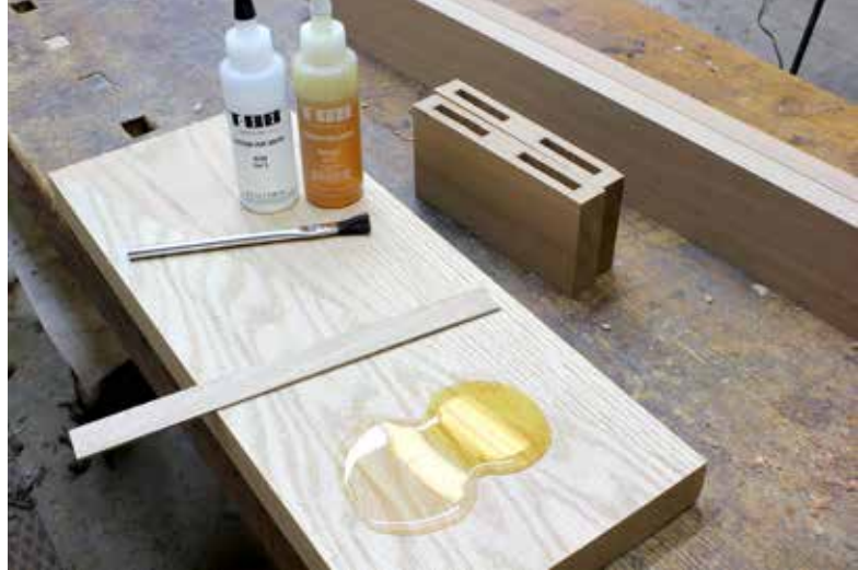
(Fig. 10) A scrap board, a brush and a stick are all that's necessary to mix and apply the epoxy to the joints.
