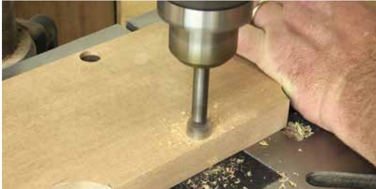
(Fig. 8) Locate and drill the holes in the base stretcher before you start assembling all the frames for the table.
