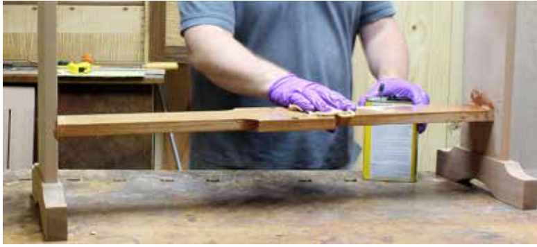
(Fig. 12) Rag on a couple of coats of Tung oil to begin the finishing process. The rest will take place over the next few months as additional coats are added while the piece gains color from exposure to the sun.
