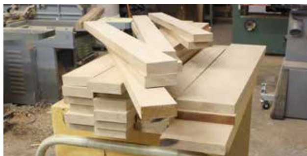
(Fig. 2) Skip-planed material is becoming more prevalent today. The thinner material often makes it difficult to mill the lumber properly and still maintain the desired thickness.
