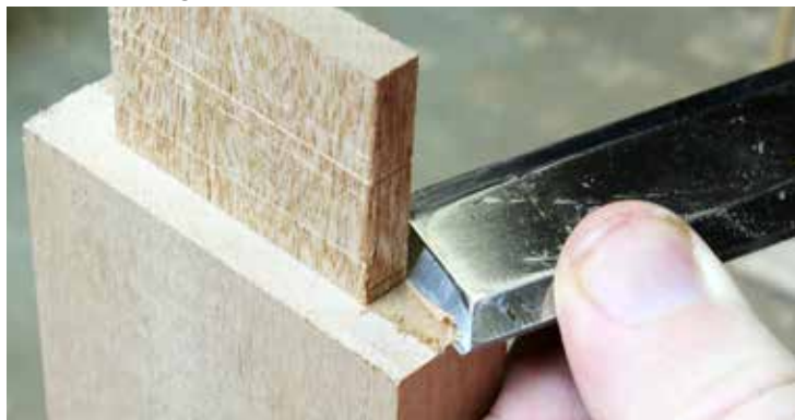
(Fig. 7) Use a wide chisel to pare the shoulders perfectly flush.
