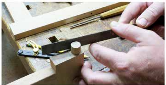
(Fig. 11) Layout the round tenons on the square tenon nubs you left on the gate frame. Use a hand saw to make relief cuts at the corners and around the perimeter of the round tenon to help ease the removal of the waste with a chisel. Fine-tune the tenon with a file, rasp or sandpaper until it slips into the hole in the base stretcher.
