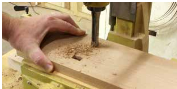
(Fig. 4) In order to cut the three through tenons on the legs, chop a little more than half way through on one surface, flip the board and finish the job from the other side.
