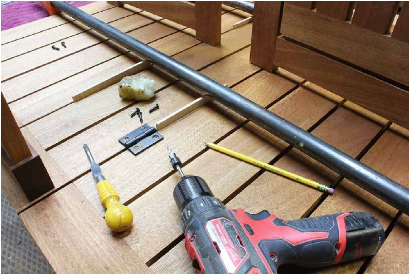
(Fig. 15) Flip the table on its top and surface mount the hinges to the leaves. You can use longer screws which will hold up better outdoors. Note the pocket hole screws that are used to attach the top to the base. Use deck screws for best weather resistance.
