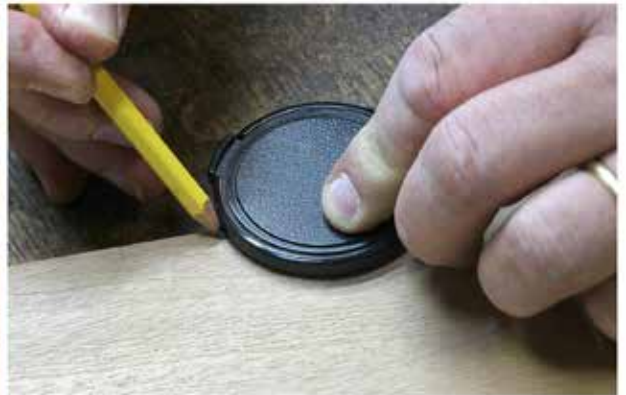
(Fig. 9) Because I'm only making one table, I draw one half of the foot and use it as a pattern for the rest once it's cutout. Drawing the curves can be an easy, no-math involved problem if you find items around the shop to help. Here I use a camera lens cap to draw the curves for the foot and base stretcher.
