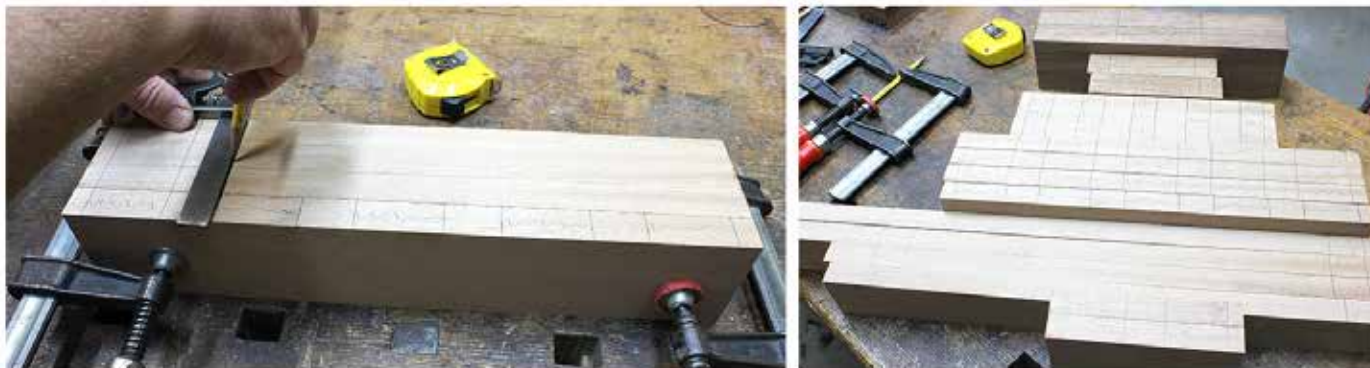
(Fig. 3) Careful layout on a single breadboard end or leg allows it to be used as a pattern to layout the other identical parts.
