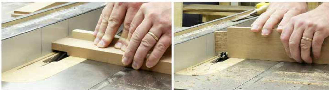
(Fig. 6) Using a rip fence as a stop for making tenons isn't a problem because material is never trapped between the fence and the blade. Raise the dado to just over 1/2" to cut the shoulders on the tenons. Be sure to bump the fence a smidgen to ensure you don't bugger up the tenon shoulders.
