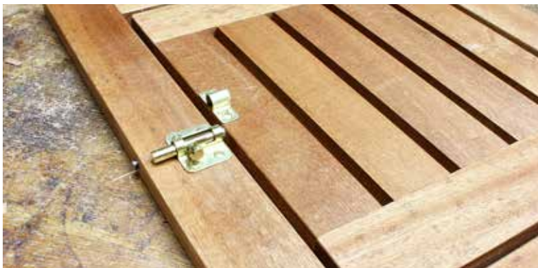
(Fig. 14) A simple barrel bolt holds the shelf in the horizontal position keeping your outdoor amenities off the ground.
