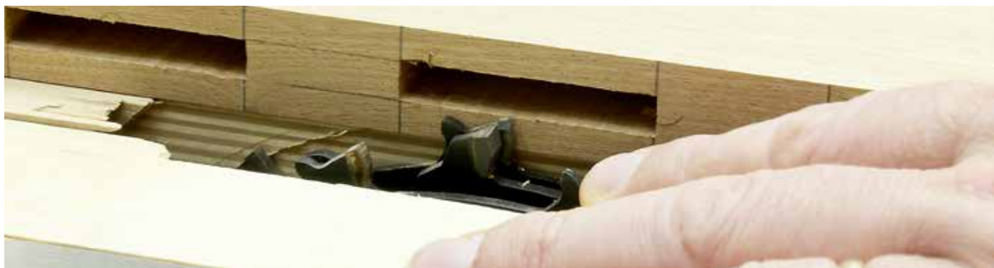
(Fig. 5) With the show face of the breadboard and toward the tabletop, raise the stack dado until the apex is at the level of the mortise wall.
