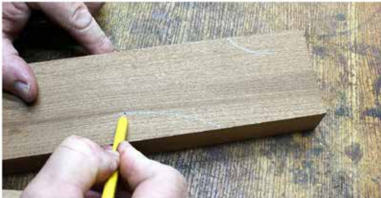
(Fig. 9) Because I'm only making one table, I draw one half of the foot and use it as a pattern for the rest once it's cutout. Drawing the curves can be an easy, no-math involved problem if you find items around the shop to help. Here I use a camera lens cap to draw the curves for the foot and base stretcher.
