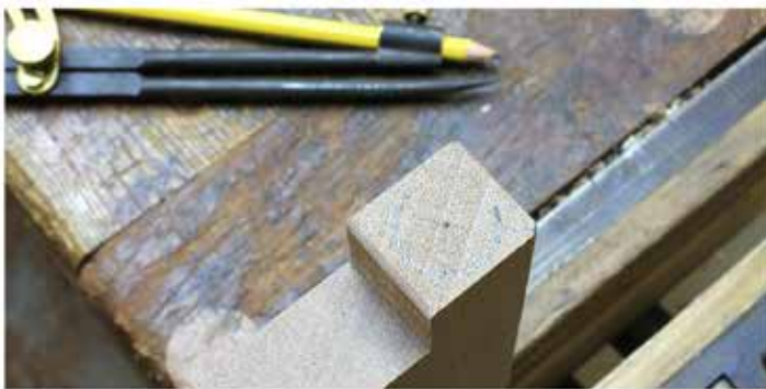
(Fig. 11) Layout the round tenons on the square tenon nubs you left on the gate frame. Use a hand saw to make relief cuts at the corners and around the perimeter of the round tenon to help ease the removal of the waste with a chisel. Fine-tune the tenon with a file, rasp or sandpaper until it slips into the hole in the base stretcher.
