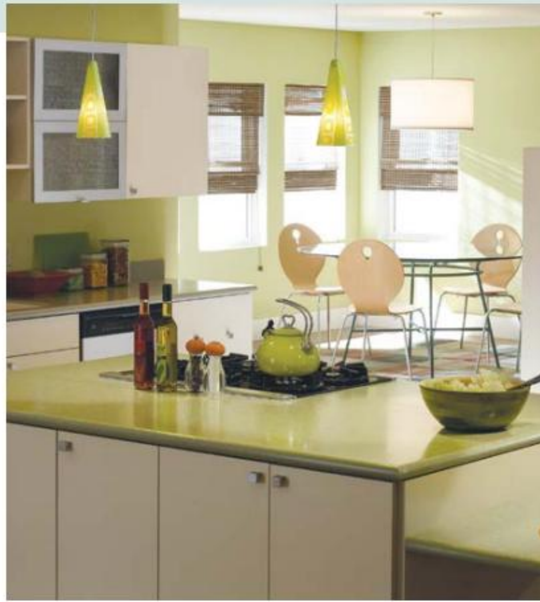
These slab doors can be quickly made with white melamine board—as long as you are able to make very straight cuts in sheet goods.
