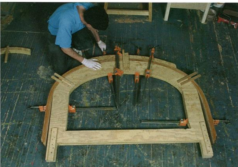
Photo D: Start clamping the laminations at the center. Before aligning the cauls on the side, pull the ends around and hold them with clamps. This makes positioning the cauls much easier. (Photo by Strother Purdy, © The Taunton Press, Inc.)
