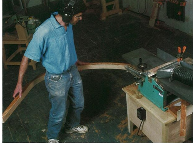
Photo G: The curve in the arch doesn't affect the operation of the planer at all, though I look like I'm doing a hula dance.
