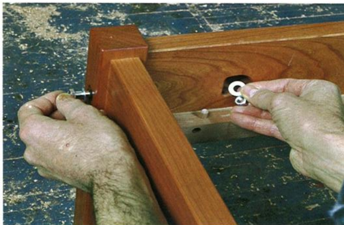
Photo H: To put the bed bolt joints together, insert a bolt with washer from the outside of the bed, until it just reaches into the nut recess. Then place the washer and nut over the end of the bolt, and start turning.
