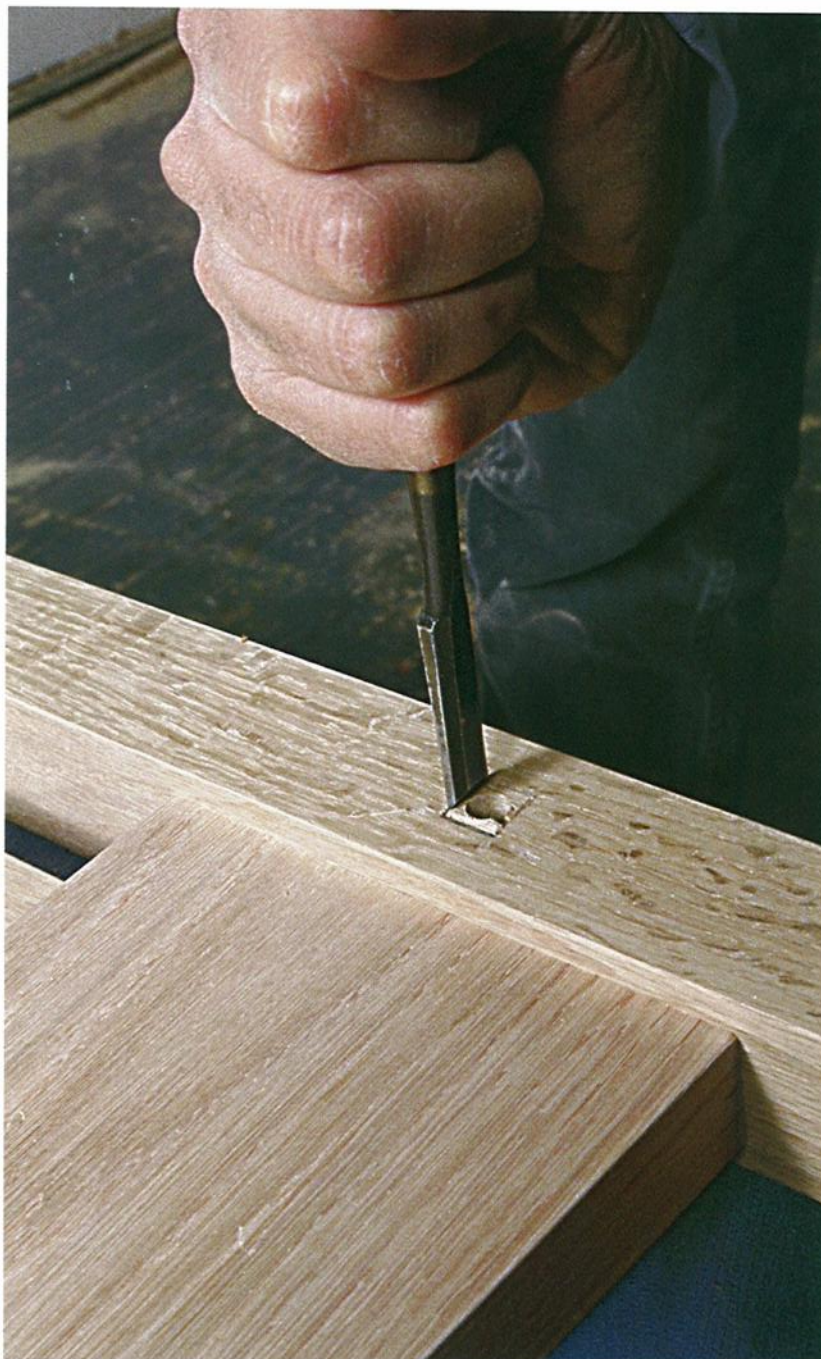
Photo K: Chisel the recess for the nut around the \frac{3}{8} -in. bolt hole on the outside of the leg. Chop across the grain first.
