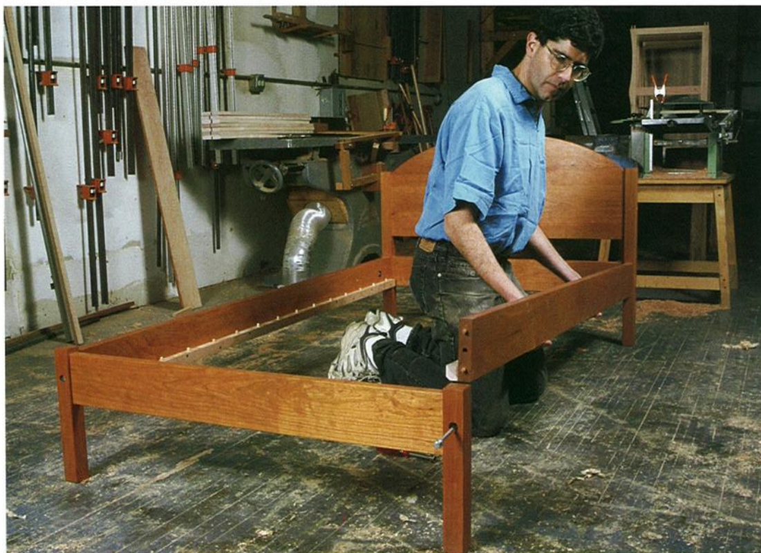
Photo I: To get the second side rail into place, it's easiest to lift the rail in the middle, then work on one end at a time.
