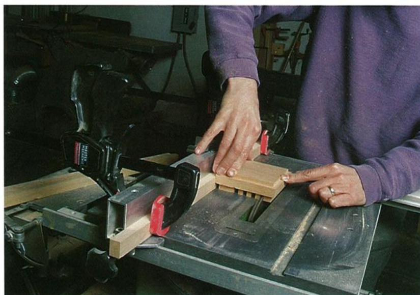
Photo F: Removing a strip lets you cut the next series of dados. I still have to remove this strip to cut the outsides of the outermost columns.
