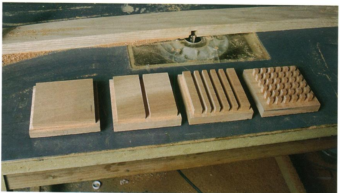
Photo C: A router table setup works well for cutting the rabbets in the base and capital parts.
