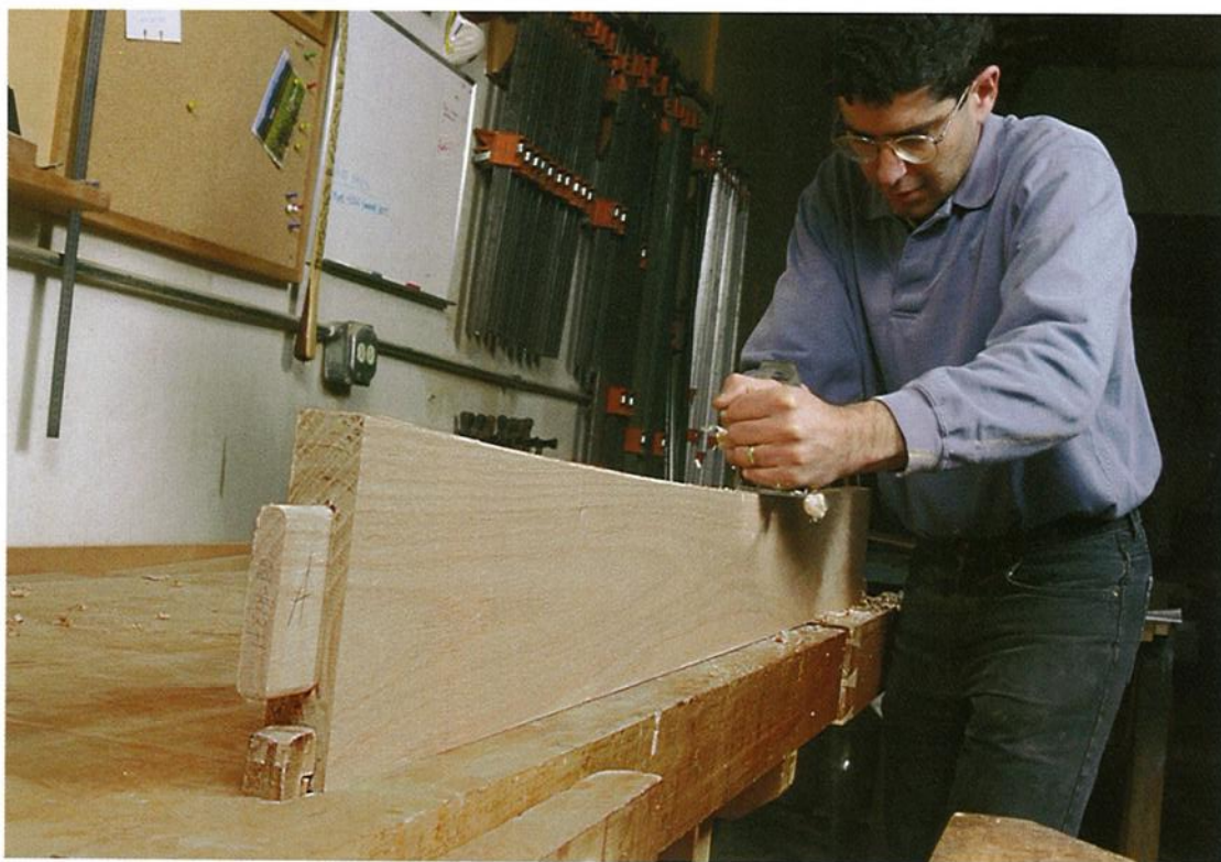
Photo E: A flat-soled plane can smooth a gentle curve if skewed in the cut.
