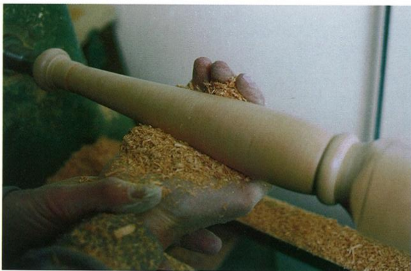
Photo G: Burnish the leg with a handful of clean shavings after all the sanding is done.
