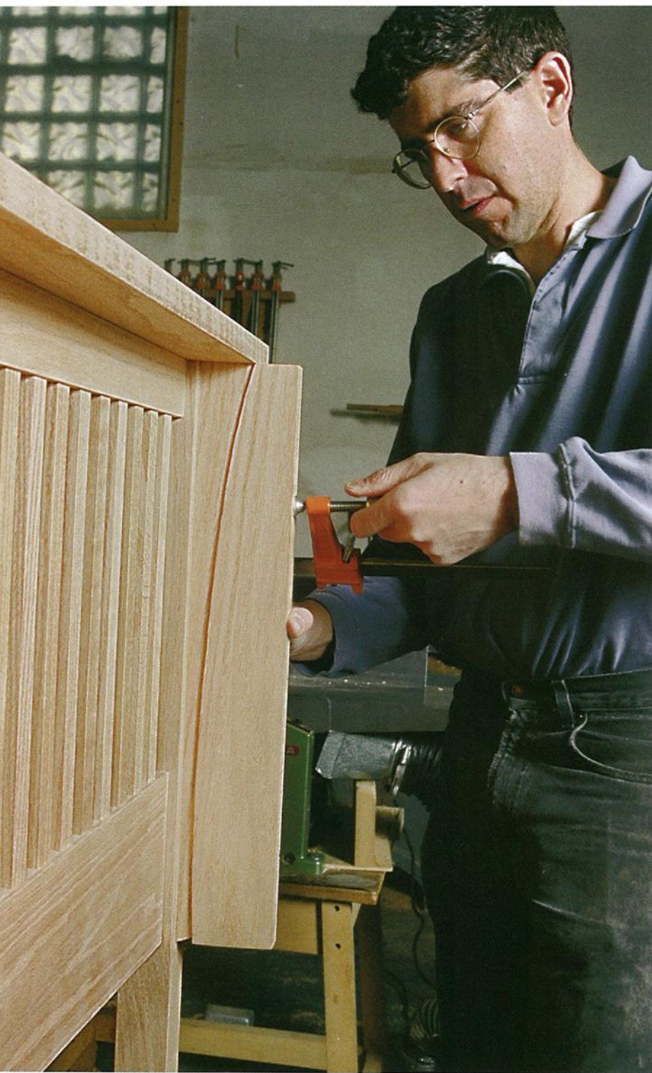
Photo M: Using the cutoff from bandsawing the wing as a caul makes it easy to clamp the wing in place and ensures even pressure.
