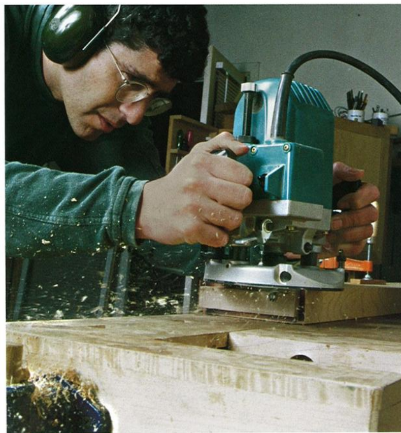
Photo F: Rout the rabbets on the sides of the rails one at a time. Be very careful not to run the bearing around the end of the tenon when starting or finishing the cut.
