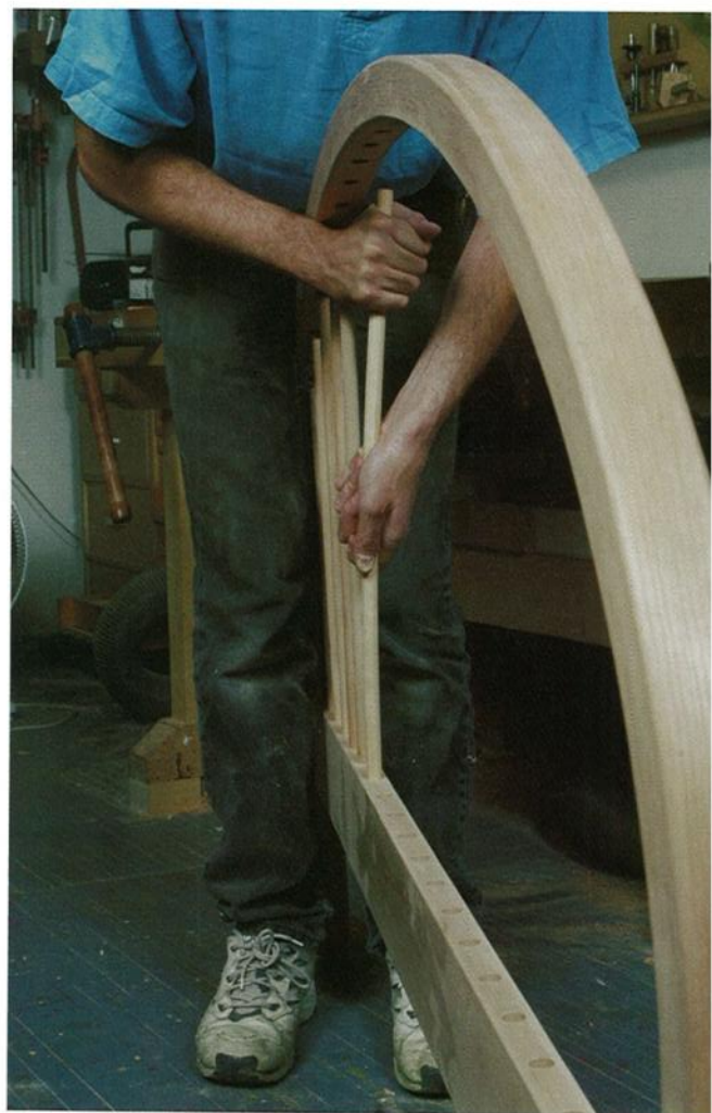
Photo L: Push with the lower hand to bow the spindle a little, so that the lower part aims straight into the hole. It's much easier to insert it into the hole this way.
