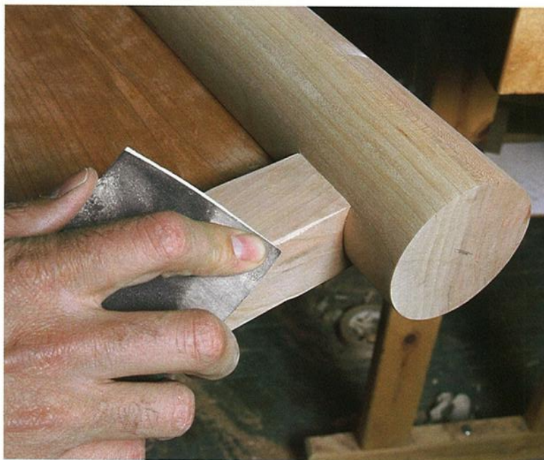
Photo L: Finish-sand the rounded edges of the legs all the way up to the crest rail. You can also ease the transition between the underside of the rail and the flat section if the leg and rail don't meet perfectly.
