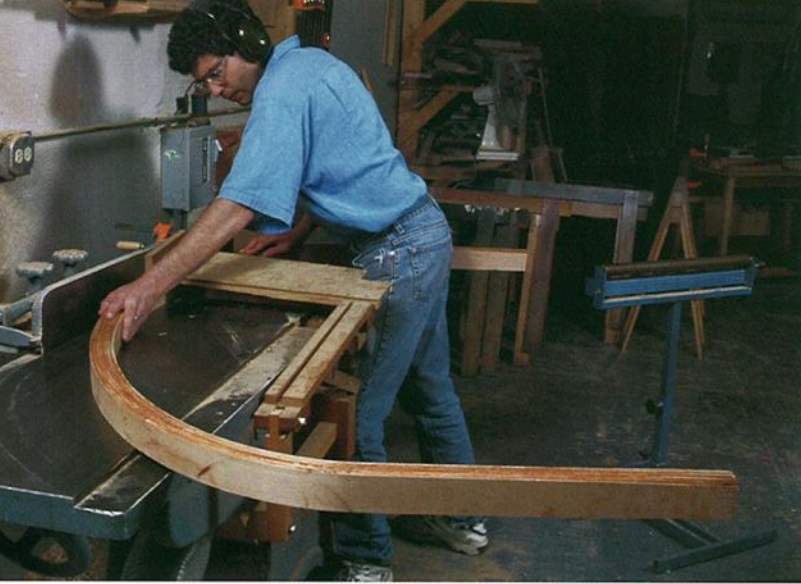
Photo F: My wide jointer helps keep the lamination stable. But roller stands or an assistant can make jointing the arch on narrower machines possible.
