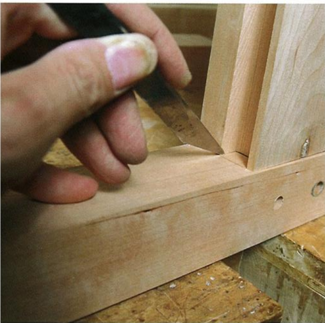
Photo H: Scribe the location for the panel groove in the leg carefully from both the lower and crest rails.
