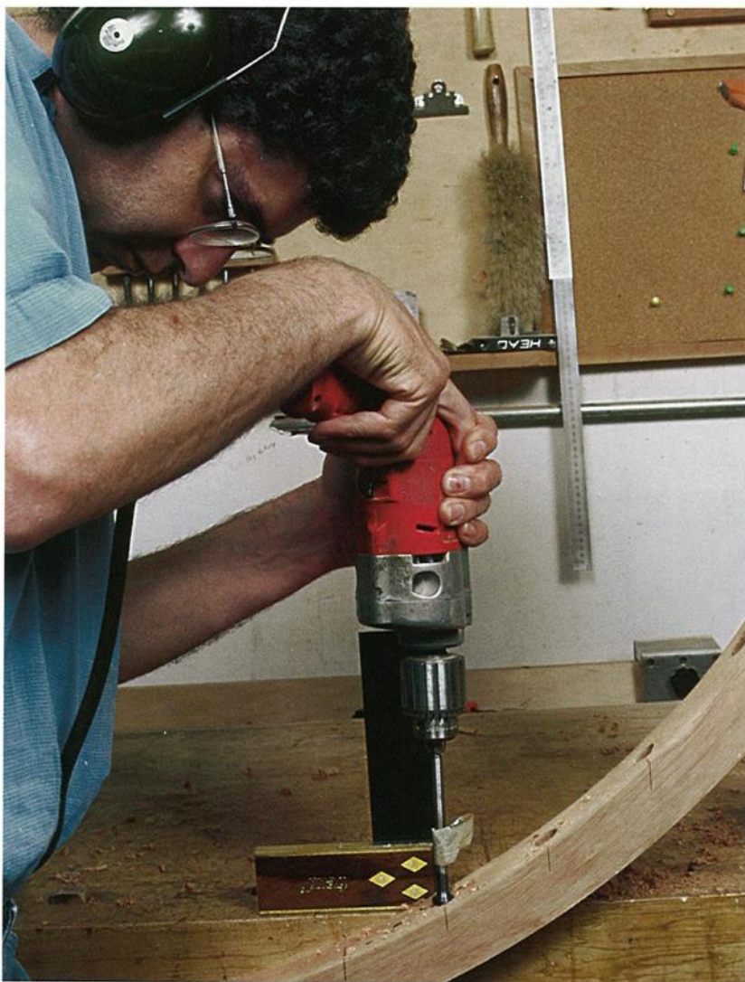
Photo J: Sighting down the square helps you drill parallel to the sides of the lamination. First square up the sides of the arch to the bench.
