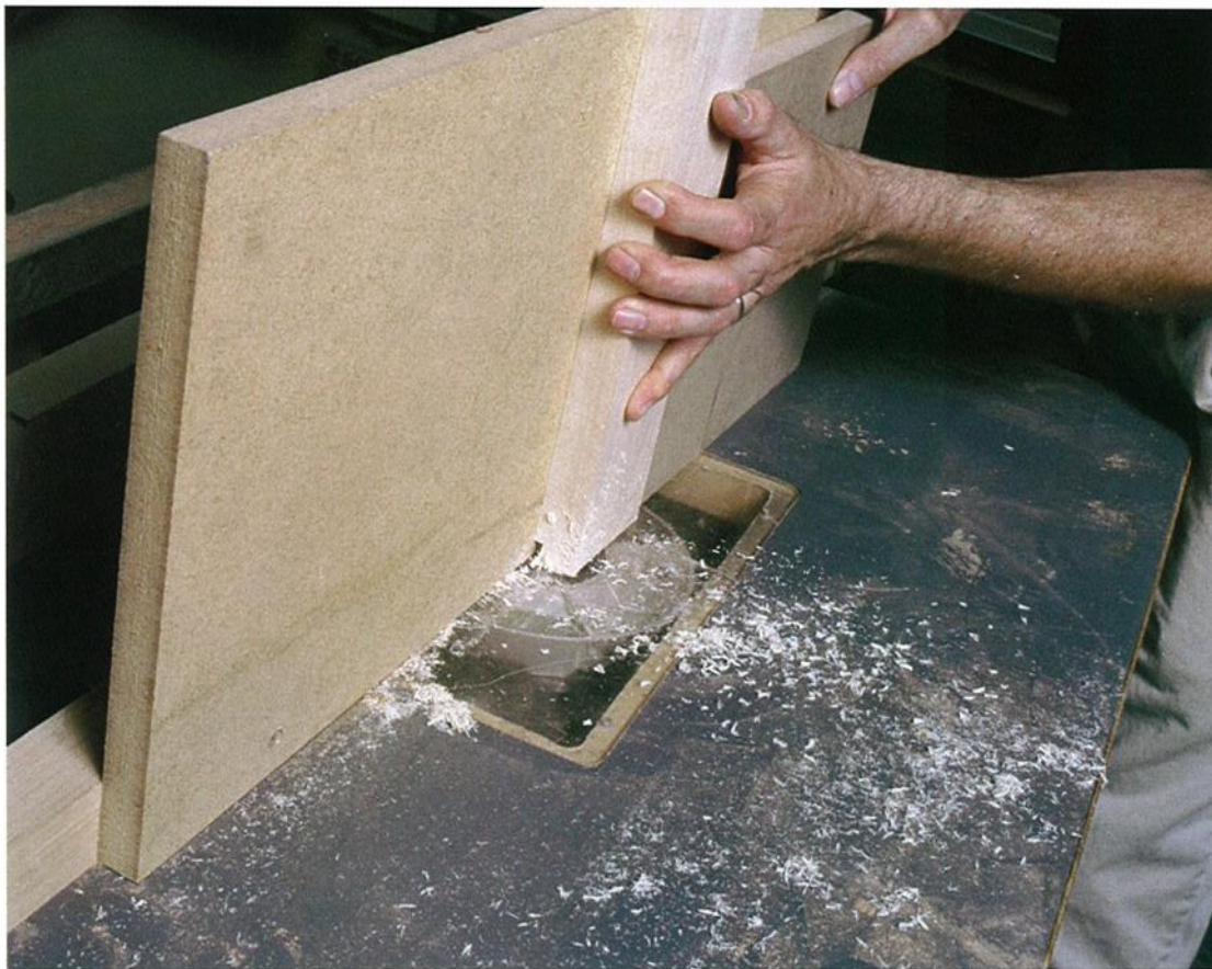
Photo D: Rout the dovetails in the ends of the rungs on the router table with a high fence. Use a large square of plywood as a guide and push stick.
