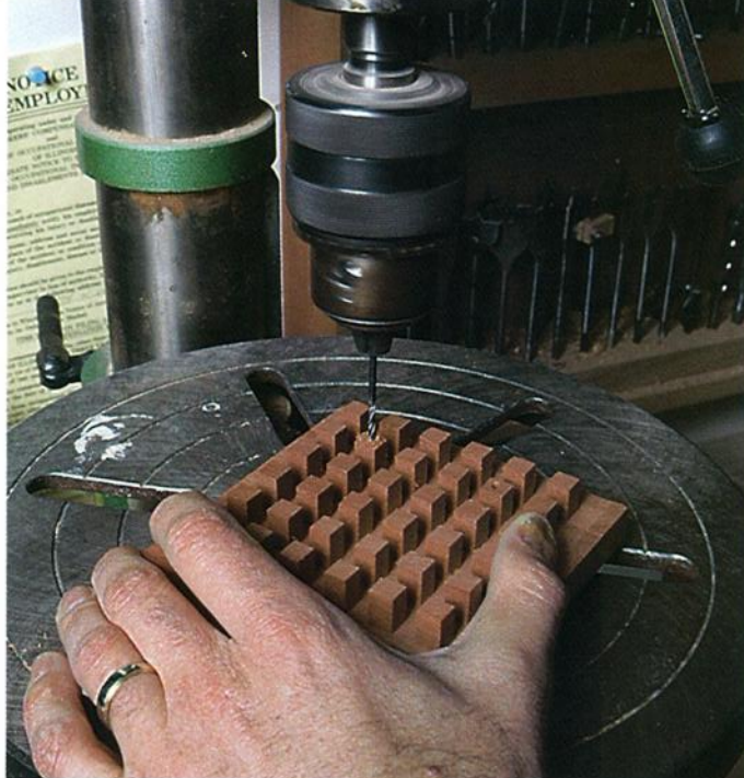
Photo G: Drill \frac{3}{32} -in. pilot holes in the second-row corner columns on a drill press slowly and carefully. I eyeball the center on each of the columns.
