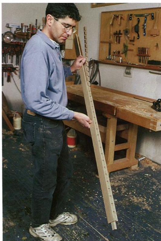
Photo D: Slowly and carefully push the fragile dentil strip into the rail groove.
