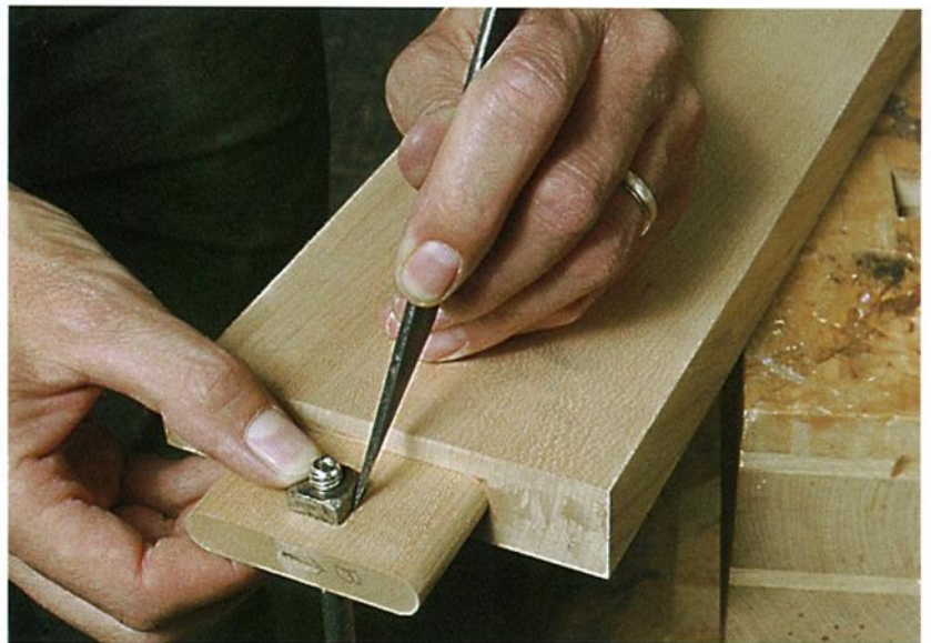
Photo F: Scribe the square nut carefully on the outside cheek of the footboard rail tenon. Wrapping a bit of tape around the bolt before slipping it into the hole in the tenon will help keep you on center.
