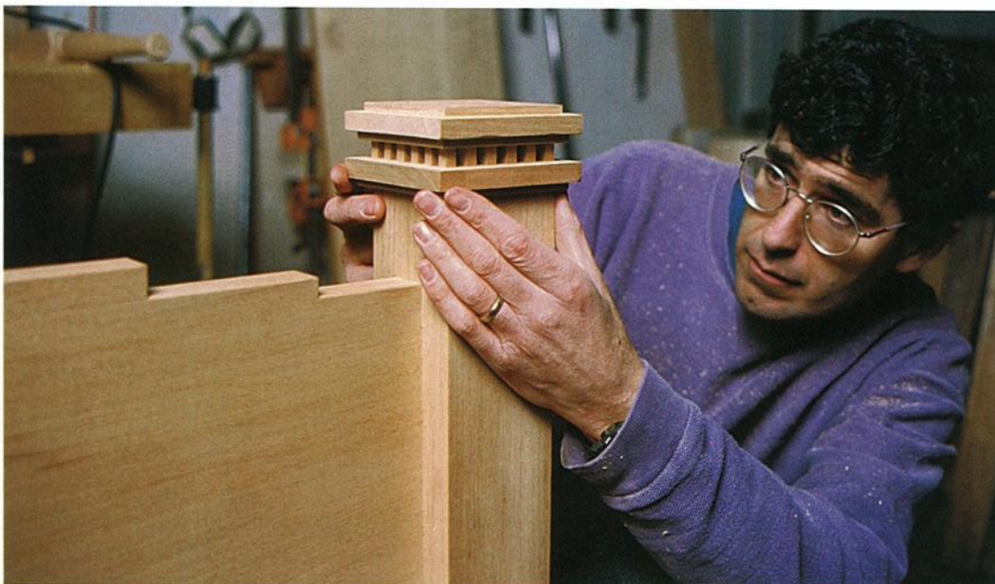
Photo I: Center the capital on the leg. You can measure or just eyeball.
