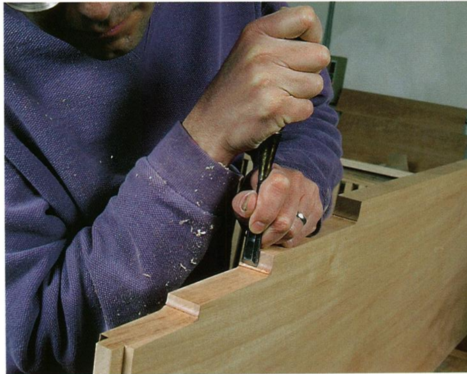
Photo B: Next, hold the chisel firmly against the vertical part of the step and pare down. Take off only a small amount of wood at a time.
