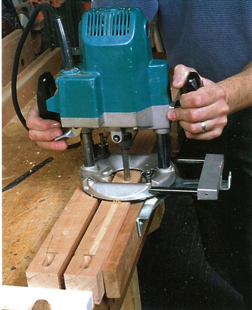
Photo I: The second leg supports the router for cutting the panel groove.
