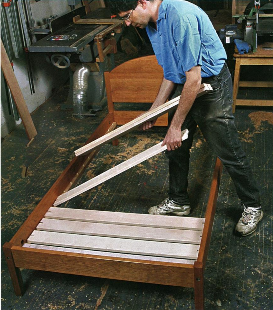
Photo J: Drop the slats into place with the notches around the locating pins in the cleats to complete the bed.
