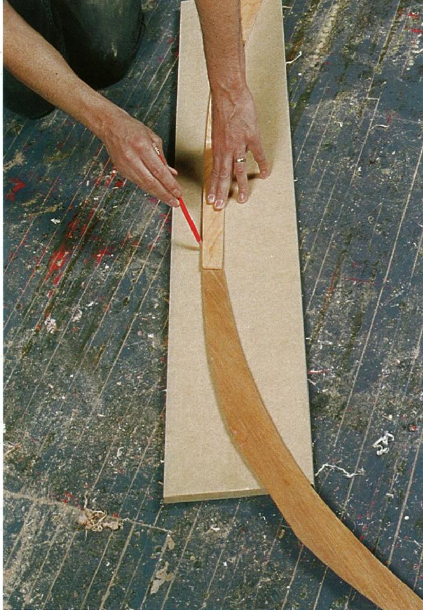
Photo A: The single curve for the curved-panel form is made up from the two leg patterns. You can overlap the patterns slightly and line them up so the curve flows from one to the other.
