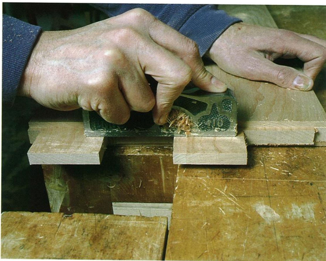
Photo H: Trimming the cheeks of the tenons to fit the mortises is easy with a shoulder plane. Note that you cut across the grain.
