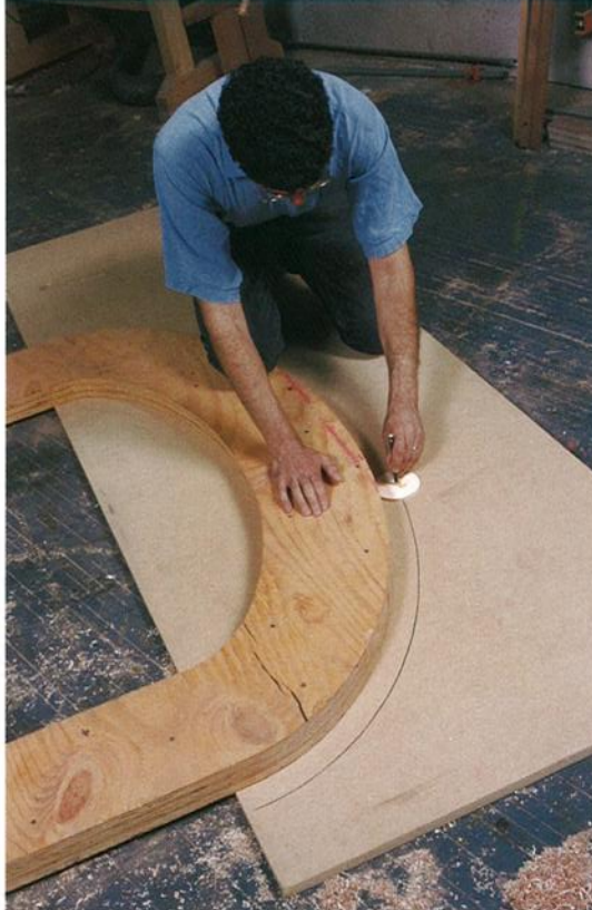
Photo B: Lay out the inside edge of the cauls 1¾ in. from the forms with a 3½-in. layout disk and pencil.
