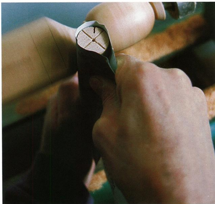
Photo F: Sand the transition from square to round using a sanding dowel so you don't blur the edges sanding by hand.
