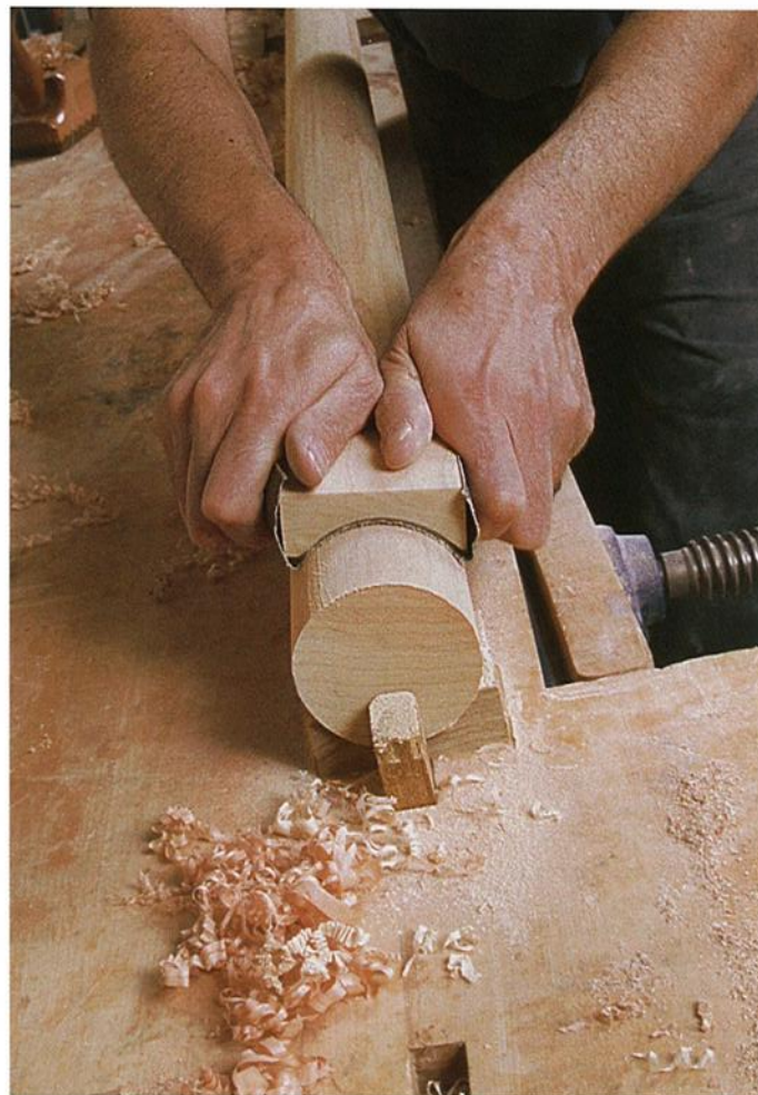
Photo I: A curved sanding block and some 80- or 100-grit sandpaper are the keys to getting the rail round. Once you're satisfied with the shape, use finer grits to smooth the rail.
