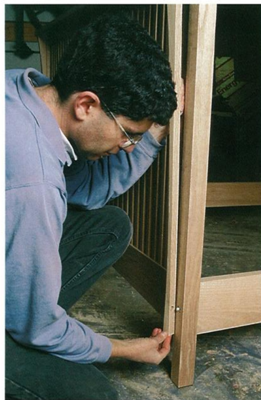
Photo L: A recess in the back of the wing allows room for the bolt to come through the leg. Without it, the bolt will break the wing right off when you tighten it during assembly.
