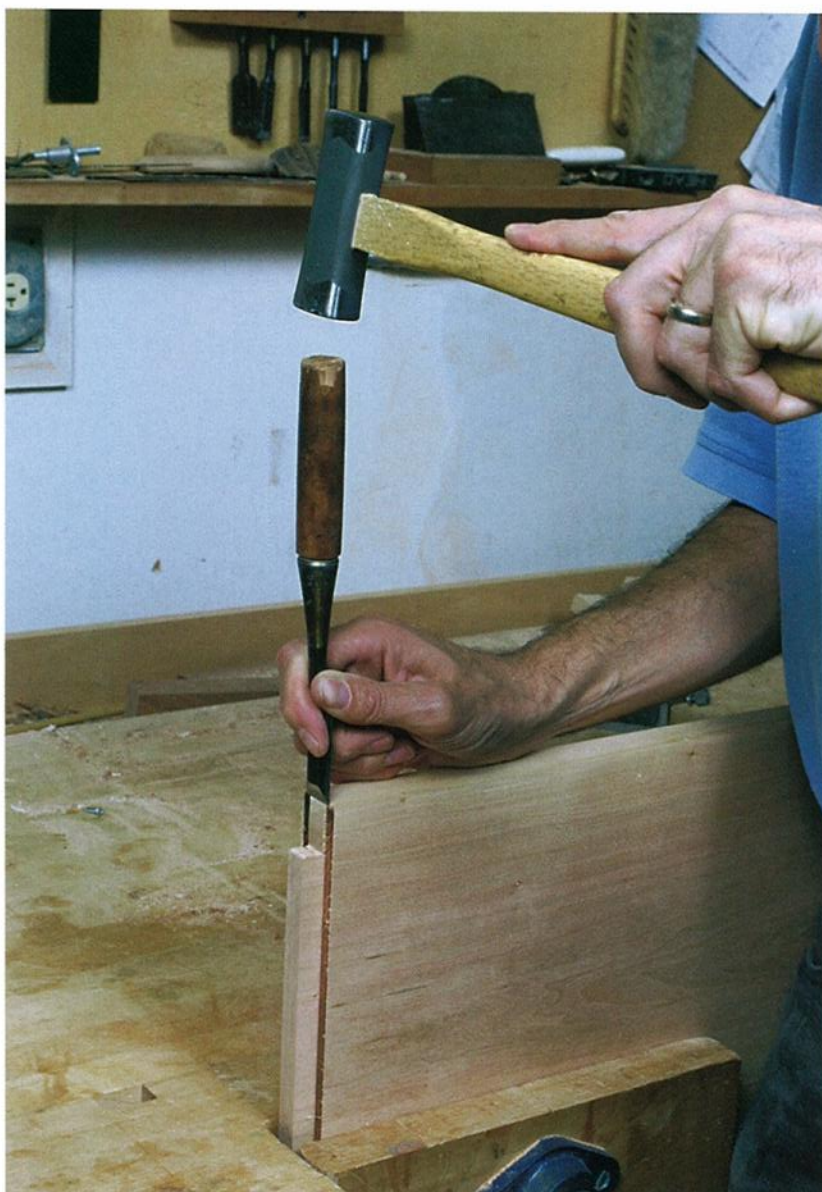
Photo D: Chisel away the thin waste left after bandsawing the tenon ends. It's easy to get a precise surface by hand because the chisel is guided by the tenon shoulders.
