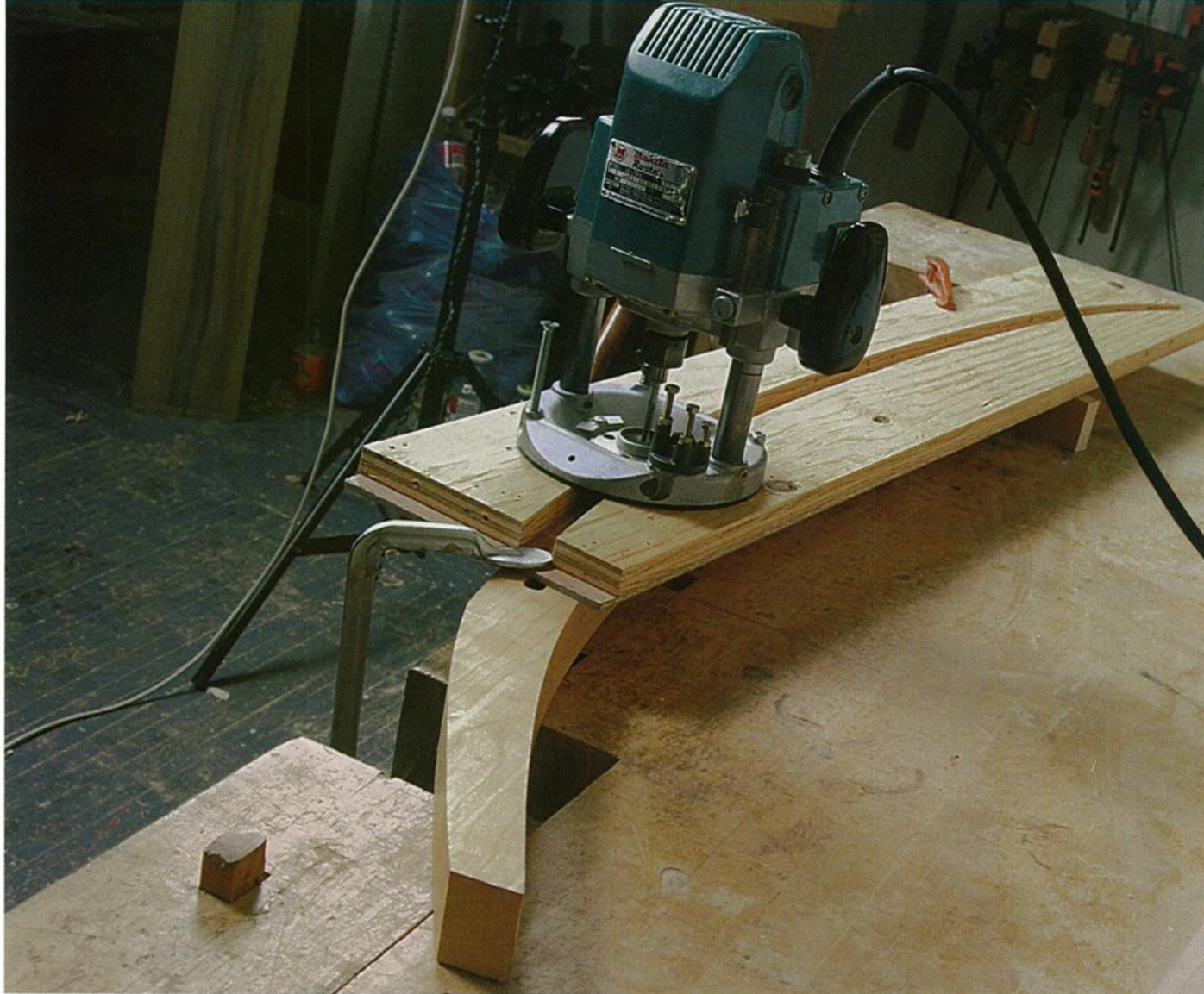
Photo J: The leg and template are set up for the curved groove to be routed.
