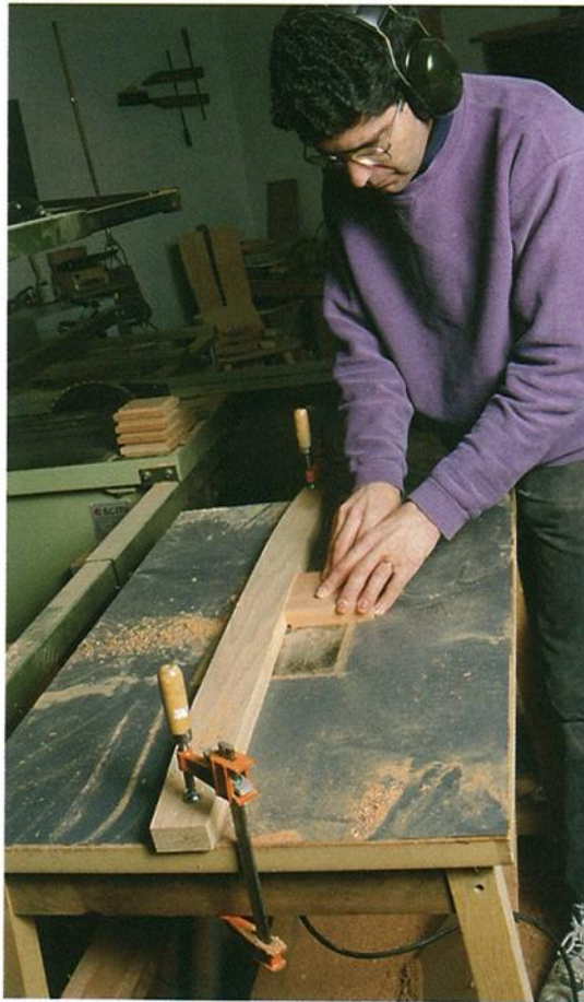
Photo C: A router table setup works well for cutting the rabbets in the base and capital parts.
