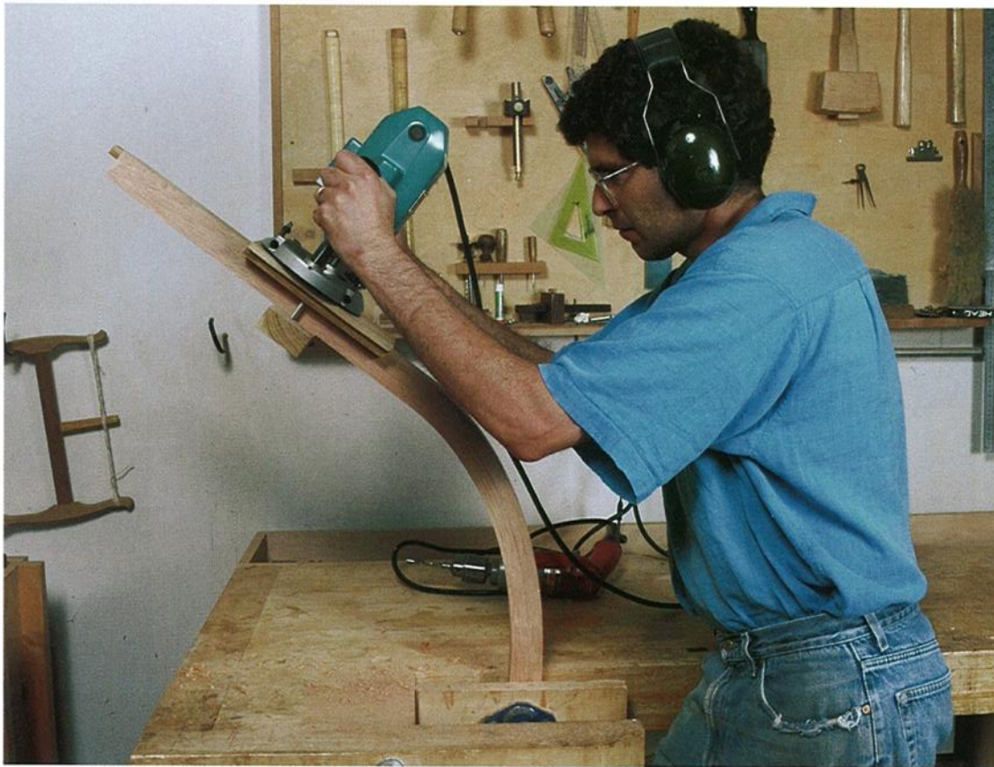
Photo H: Though still awkward, this is the most comfortable position I've found for mortising the arch.
