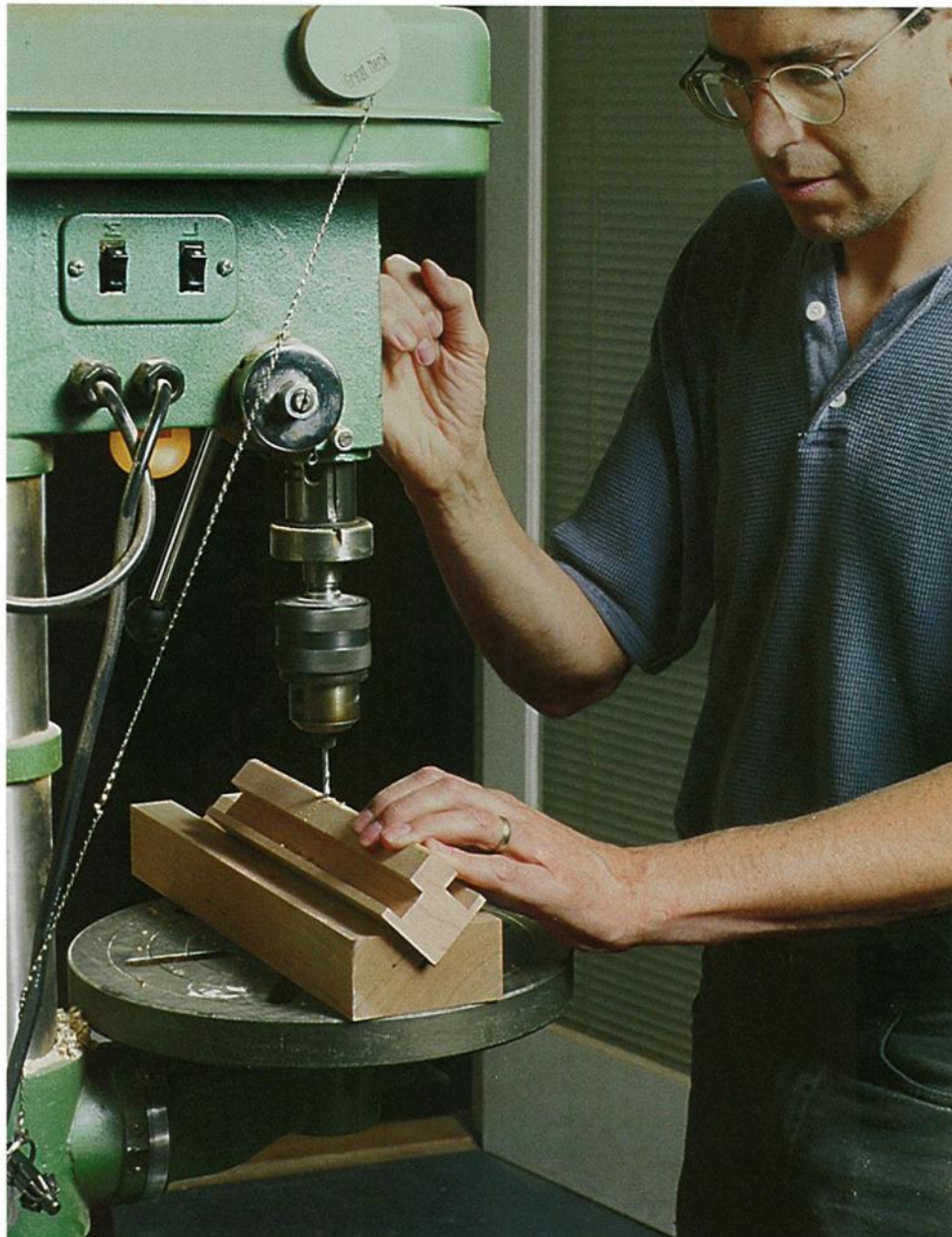
Photo C: A V-shaped groove jig helps you drill the holes for the screws in the corners of the base blocks.
