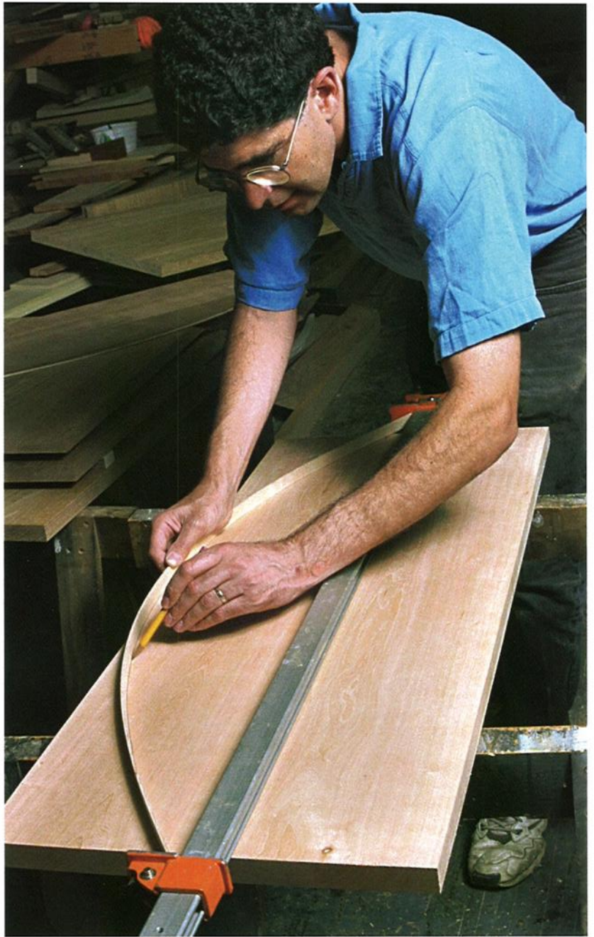
Photo C: Springing an evenly thin piece of wood into a gentle curve is an easy way to lay out the top of the headboard. You can loosen or tighten the clamp to fine-tune the shape.
