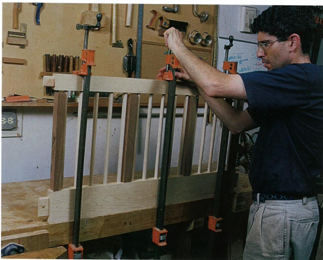
Photo A: The four walnut blocks (they don't have to be walnut) keep the rails the right distance apart when they're clamped during glue-up.
