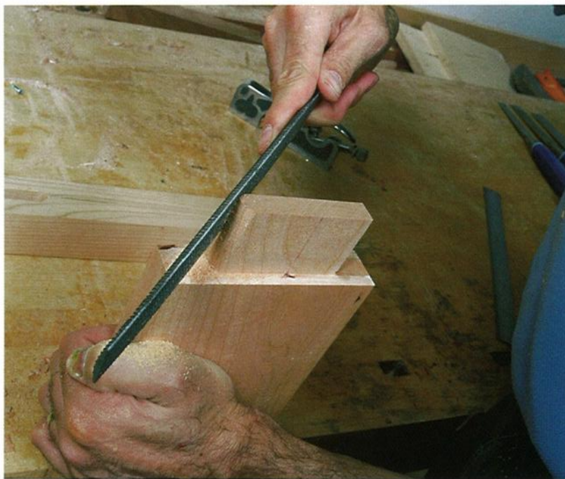
Photo B: Rasping the edges of a tenon is quick and easy. It's a lot easier to make the tenon fit a routed mortise than to square up the ends of the mortise.
