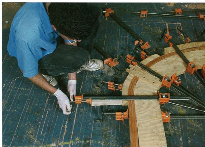
Photo E: A wooden block between the clamp and the caul makes it possible to use a long clamp where a short one is needed. (Photo by Strother Purdy, © The Taunton Press, Inc.)
