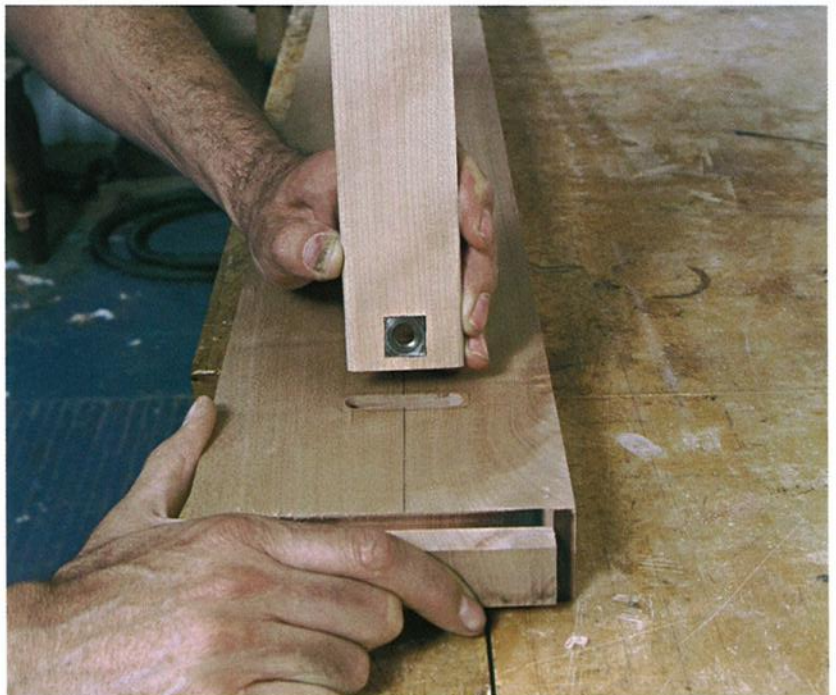
Photo H: A captured nut is ready to be inserted into the mortise in the side rail. When glued in place and cut flush against the rail, it makes an elegant joint.
