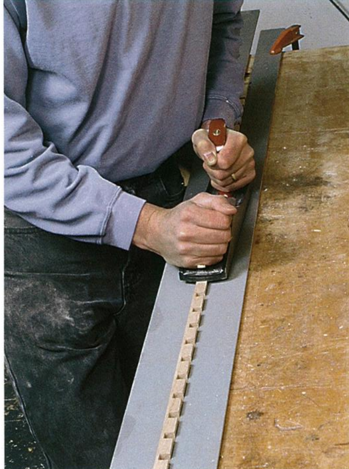
Photo C: The notched strip is too flexible to plane without support. Two plywood strips clamped to the bench keep the strip from bending or breaking.
