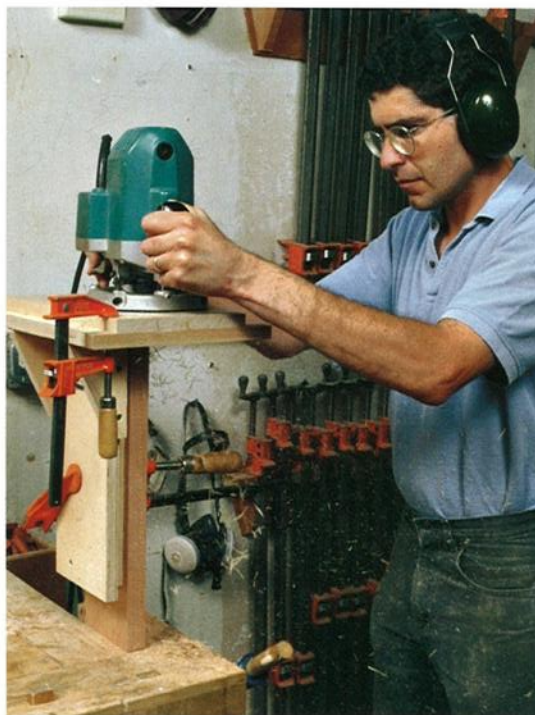
Photo A: The tenoning jig positions the workpiece upright and supports the router on the end of the rail.
