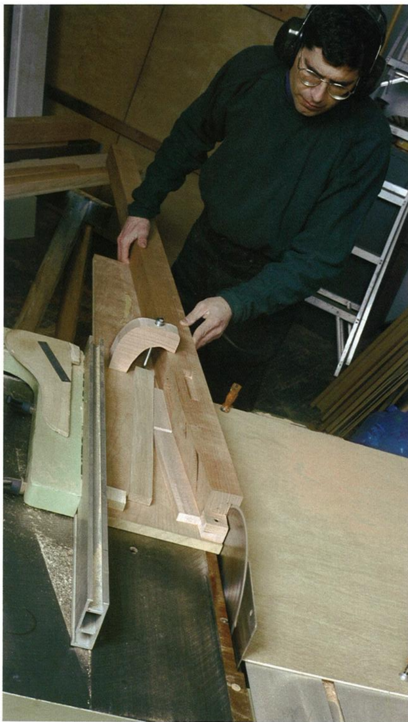
Photo B: On a table saw with a blade that can be raised to at least 3½ in., the tapering jigs work very well. Clamp a piece of plywood on the other side of the blade to prevent the wedge-shaped cutoff from dropping through the throat plate.
