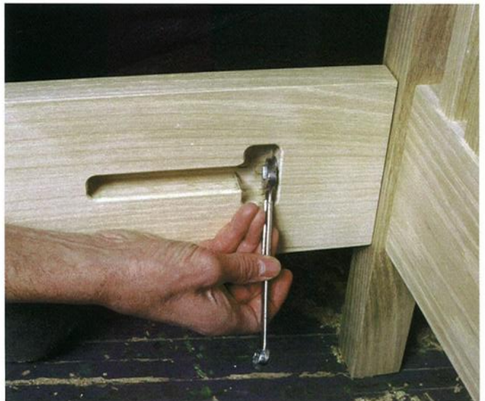
Bed bolts can be hidden by reversing their orientation so that they screw in from the rail into the leg. This requires some ingenuity and a fair bit more work.
