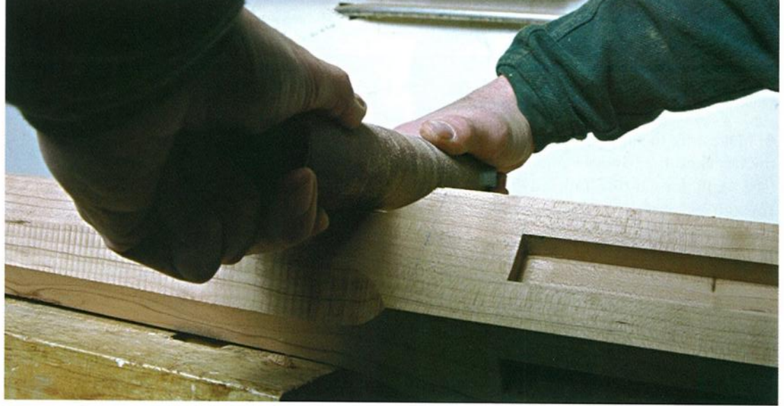
Photo C: It takes a twisting motion with the sandpaper-wrapped dowel to clean up the curved transition area between the square joinery block and the octagonal post effectively.
