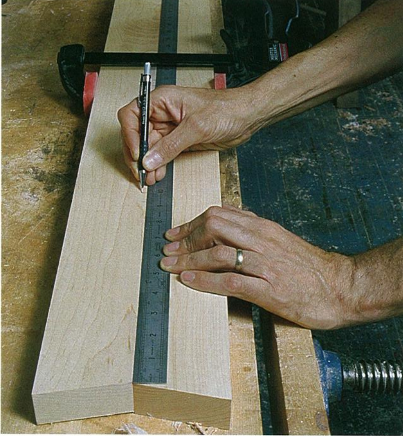
Photo B: Clamp the two sides of the ladder together to lay out the rung locations.
