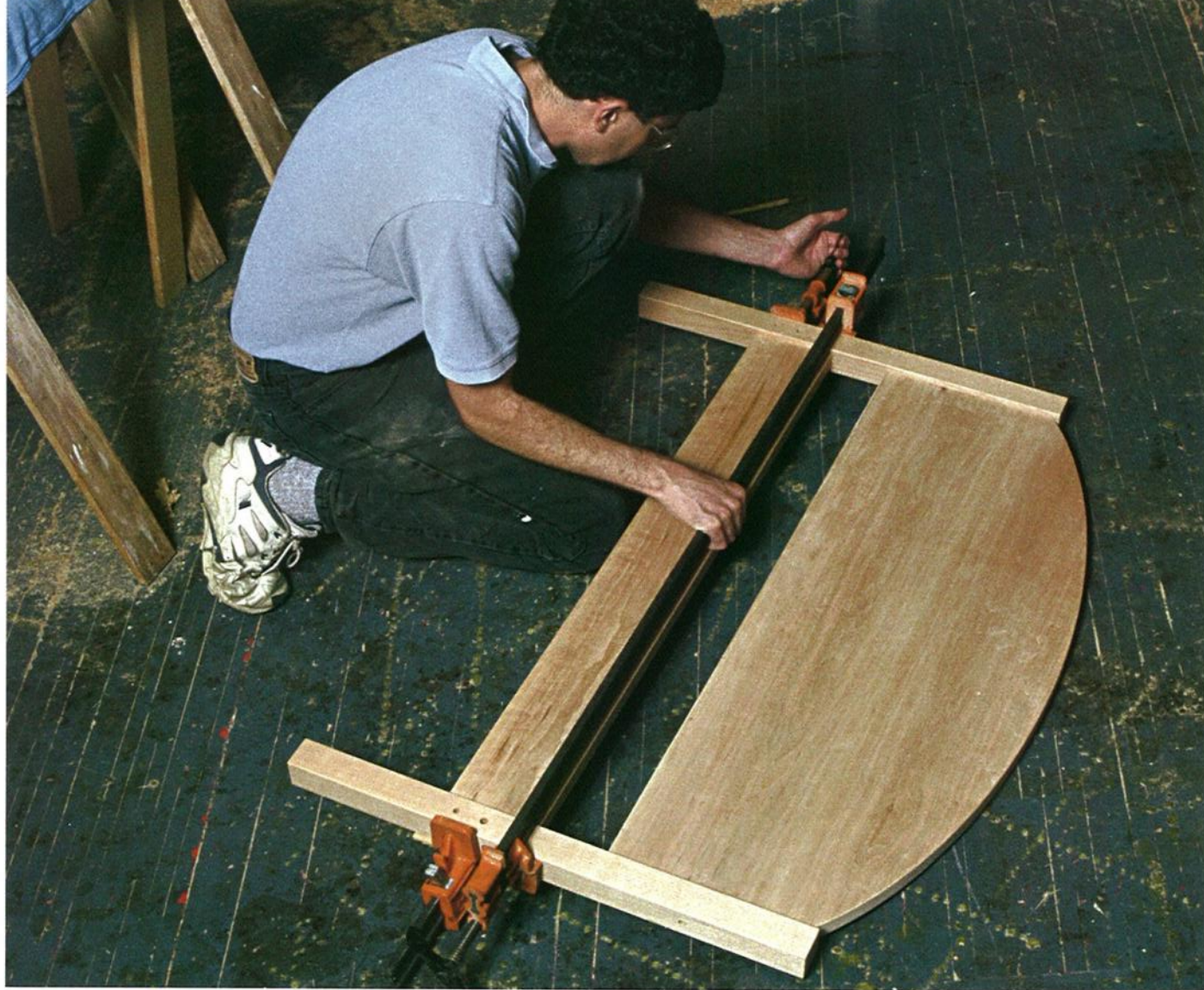
Photo E: When clamping up the headboard assembly, use two clamps on the rail—one in front of the headboard and one behind—and offset them slightly.
