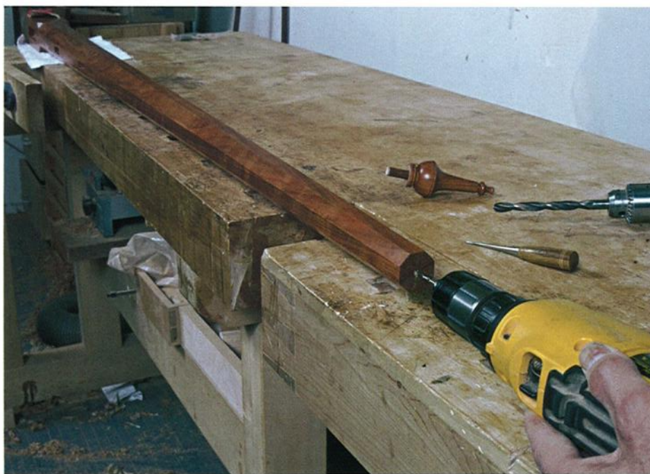
Photo K: To drill dowel holes for the finials, lay the posts down on a bench to guide your eye.
