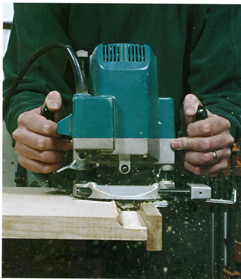
Photo I: Rout the tenon and the transition curve of the back of the headboard. Do this before you shape the headboard so the router fence can register against a long tenon edge.
