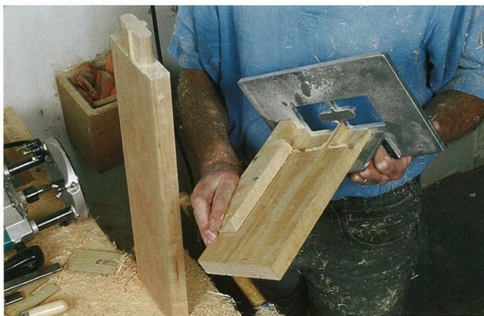
Photo I: This tenoning jig shapes the ends of the through tenons perfectly. It leaves an odd-looking strip on each cheek of the tenon, which is easy to trim off. (Don't let my aluminum jig intimidate you; it works fine if it's made of plywood.)
