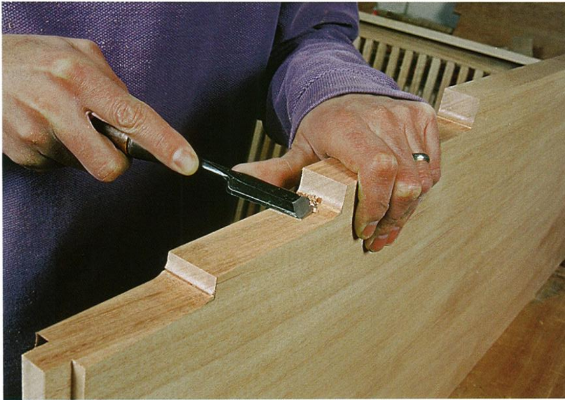
Photo A: To pare the headboard detail corners square, first work horizontally from both sides to the middle, so you don't chip off any wood by paring over the opposite edge. Watch those fingers!
