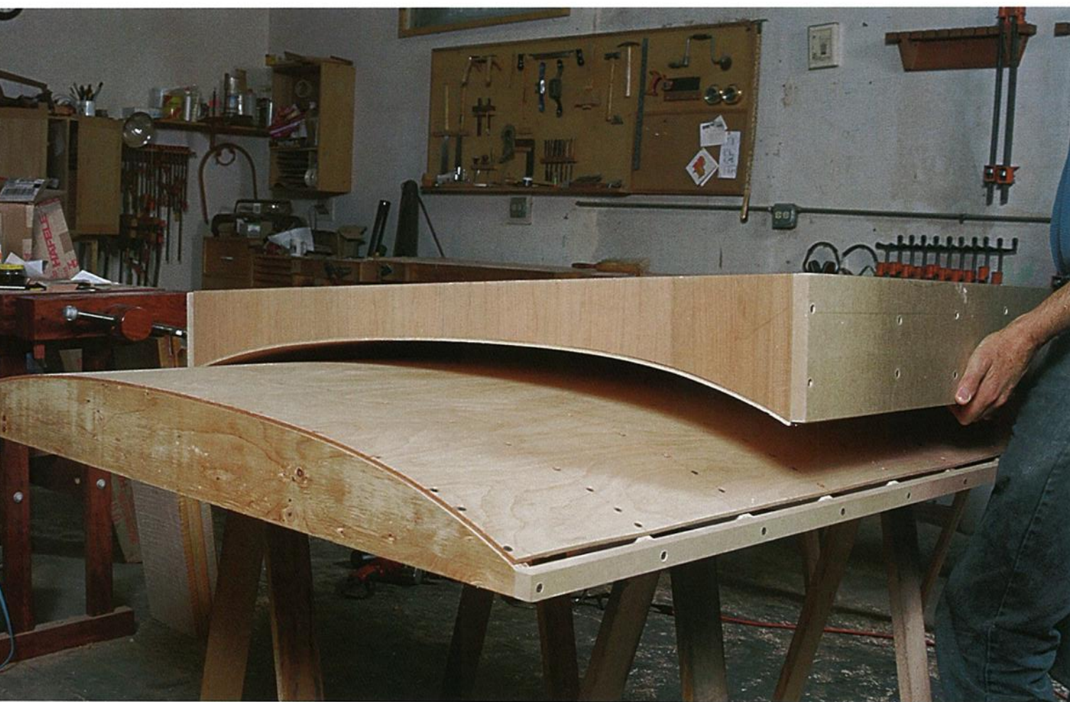
Photo C: The form is larger than either panel but will bend the footboard and headboard panels at once.
