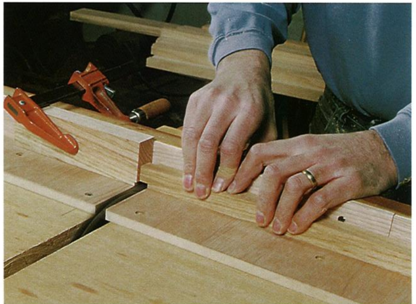
Photo F: For cutting the tenons on the slats, the crosscut sled works well, though a miter gauge will work, too. The stop clamped on the far side of the sawblade registers the slat so the shoulder on each side of every slat will be cut the same.
