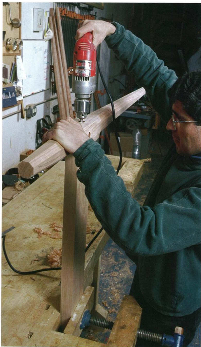
Photo G: Drilling the hole for the bed bolt in the end of the rail is best done by using the post itself as a drill guide. Hold the post securely in place while you drill.
