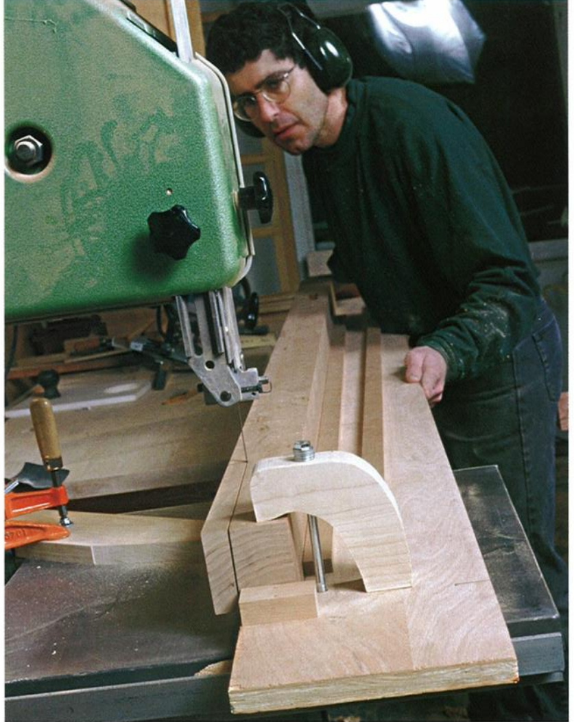
Photo A: The hold-down clamp in the foreground is a block and a bolt threaded into a recessed T-nut on the bottom of the jig.
