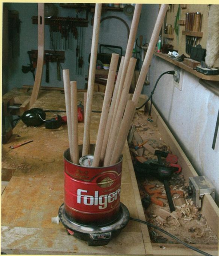
Sand in a can on a hot plate will effectively shrink dowel ends, making it easier to insert them into their mortises.
