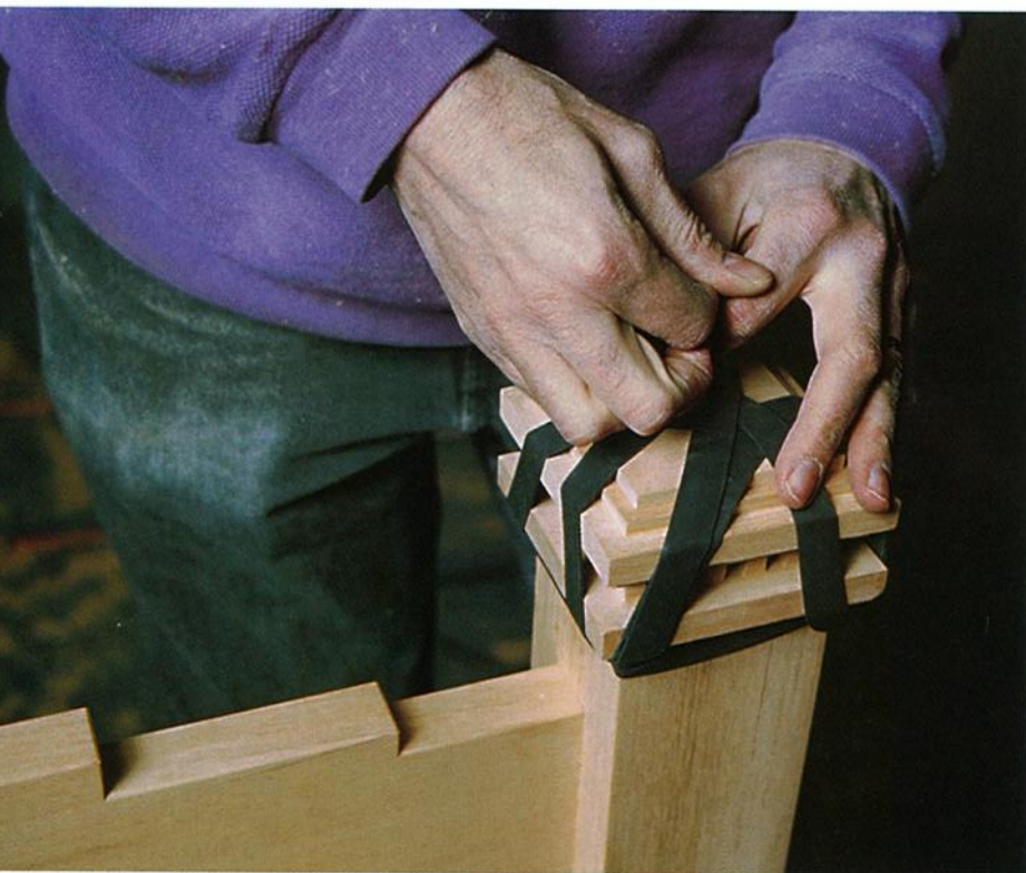
Photo M: Secure the glued pyramid to the column top with rubber strips cut from an inner tube or with strong elastic bands.
