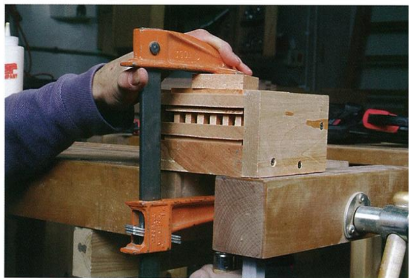
Photo H: Place a set of capital parts into the jig with a scrap on top as a pad, and clamp.
