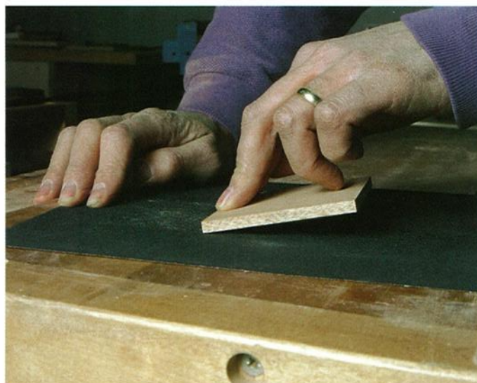
Photo L: Sanding the pyramids smooth takes a careful touch. Place the sandpaper on a flat surface and draw the pyramid slowly and carefully over it.
