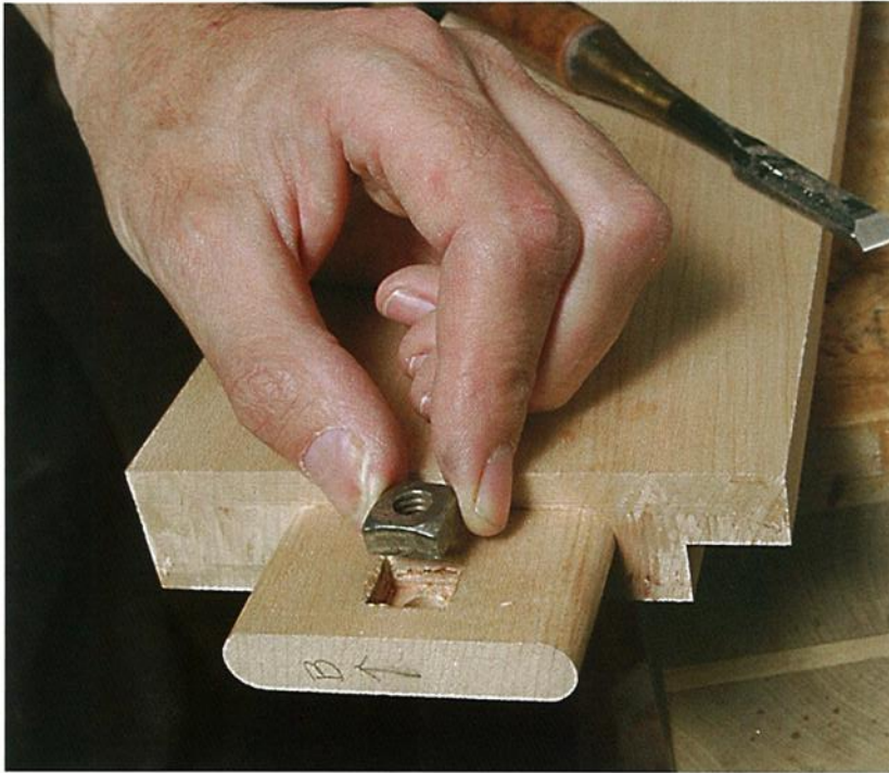
Photo G: Chisel the recess so the nut fits snugly and drops just below the surface of the tenon.
