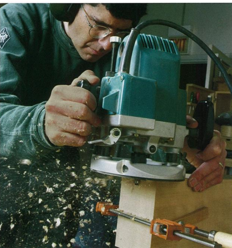
Photo E: To make the tenons on the side rails, clamp the two rails together and rout a rabbet on the top and bottom.
