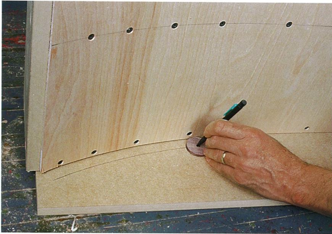
Photo B: Roll the disk along the completed concave side of the form, keeping the pencil against the near edge of the hole to draw the shape of the mating convex form.
