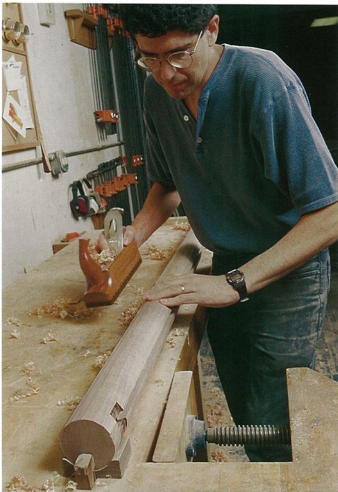
Photo H: Handplane all the edges to produce a 32-sided polygon, which is getting very close to round. The handwork is fun at this point.
