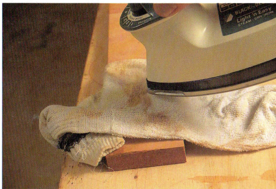
Touch the hot iron on the damp cloth to remove dents.
