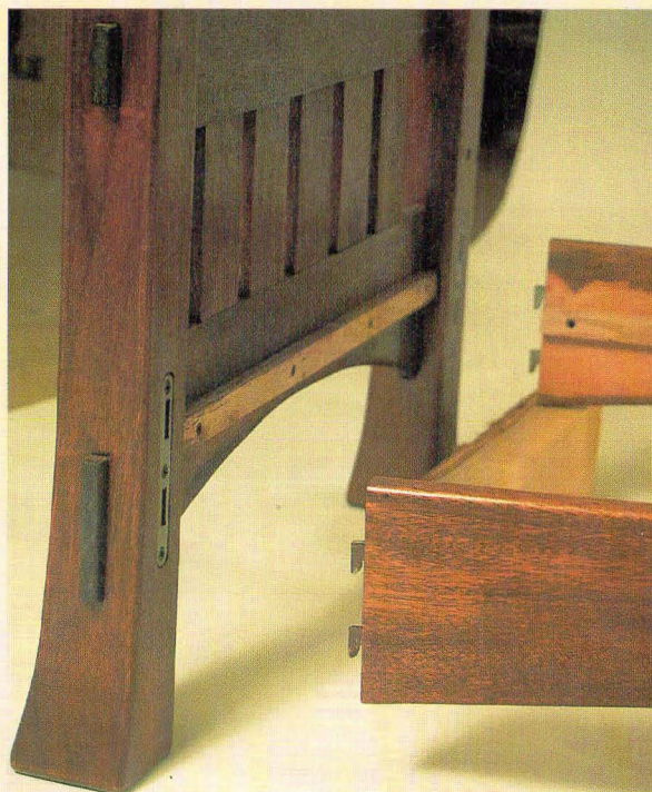
Bed-rail fasteners allow the settle to be knocked down in construction without losing the smooth lines of the design.
