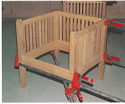
10 Clamp diagonally across the chair frame, to adjust square to perfect.
