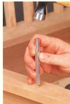
Now square the hole. I bought inexpensive steel bar stock from my local home center (7/16" square and 5/16" square). Then I tapered one end on my grinder. Tap the bar stock into your round hole and it will become a square hole.
