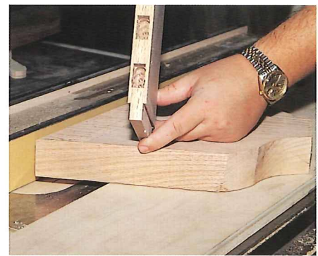
3 A featherboard provides stability and safety while cutting the tenons.
