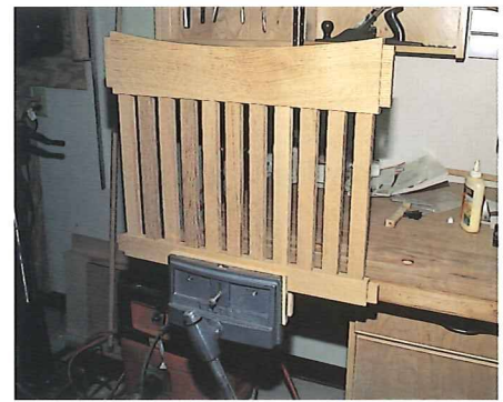
6 The side assemblies should fit snugly, but if you force them, you'll split wood!
