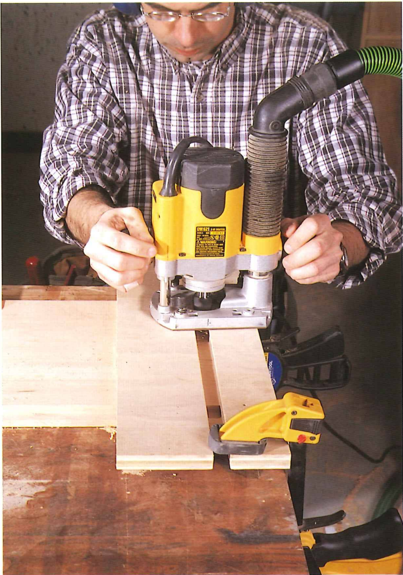
1 This plywood jig cuts the dados in the sides that hold the top and bottom pieces. Here I'm cutting the dado for the bottom. Note how the edge of the jig is flush to the bottom of the case.
