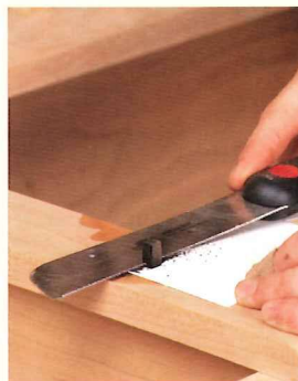
Use a piece of cardboard as a spacer between your work and a flush-cutting saw. Cut the plug and sand it slightly so there's still a raised bump.
