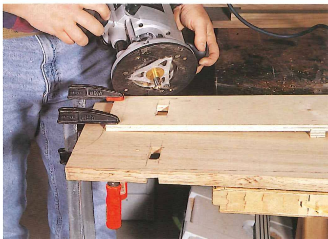
This simple scrap-wood jig made angled mortises a fairly simple task.
