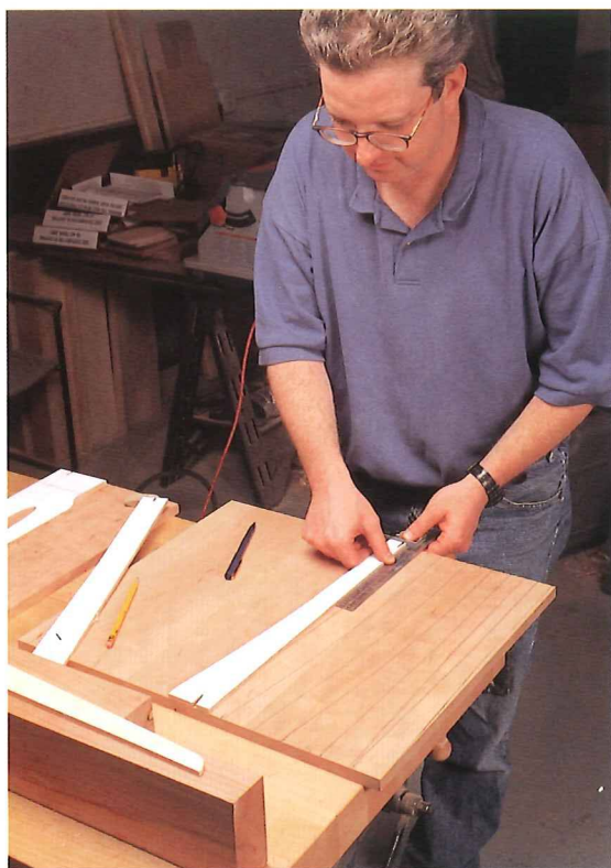
The templates for the slats are provided on the scaled-down grids. After enlarging them, lay out the templates on your wood, cut the tenons on the end of the board and band saw the slats to shape.
