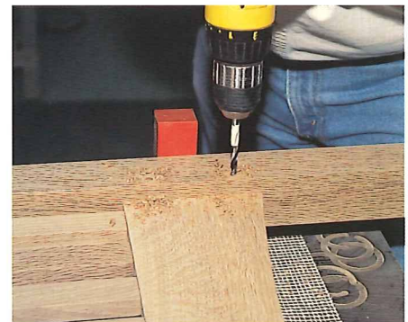
8 When drilling the peg holes, a piece of tape on the bit inexpensively controls depth.
