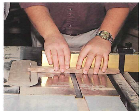
5 Use a stop block on the miter gauge to set the tenon shoulder depth.
