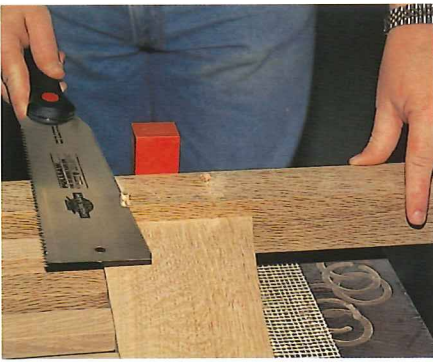
9 Keep the saw blade parallel to the leg surface while cutting the peg flush.
