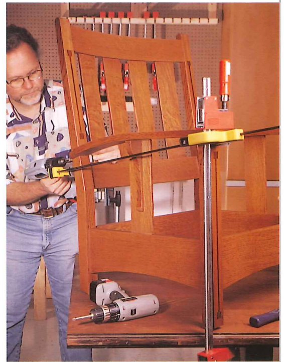
9 A screw in the tenon of the arm will add extra strength to the back of the chair. The hole can be plugged with the same wood used in the inlays.
