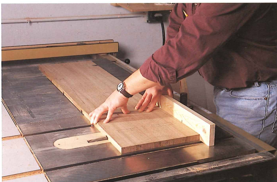
After carefully laying out the shelf locations, the sides are run over a dado stack (set at a 5-degree angle) using the saw's miter gauge to support the side on the final cuts.
