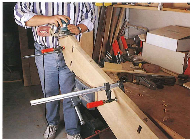
With the sides clamped together and mounted in my vice, shaping the sides took some sanding and planing.
