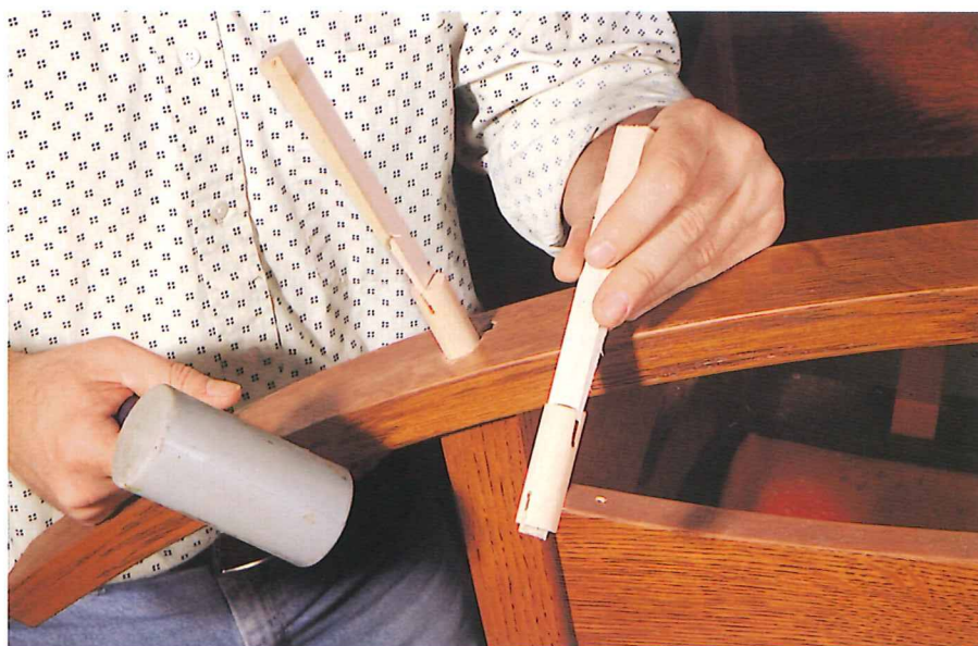
8 A \frac{3}{4} " dowel with slots and wedges will hold the rockers in place for many years to come.
