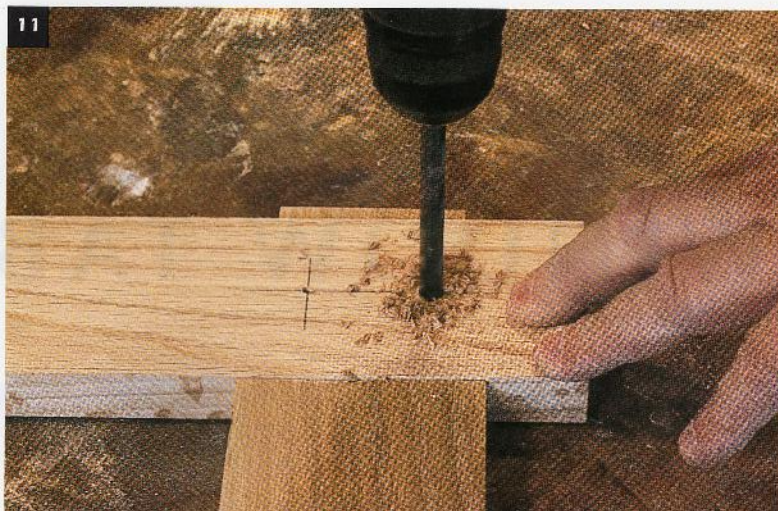
11. Mark the positions of the through dowels at each of the four corners, then drill the holes and insert the dowels using a little glue. This makes for a very strong frame.
