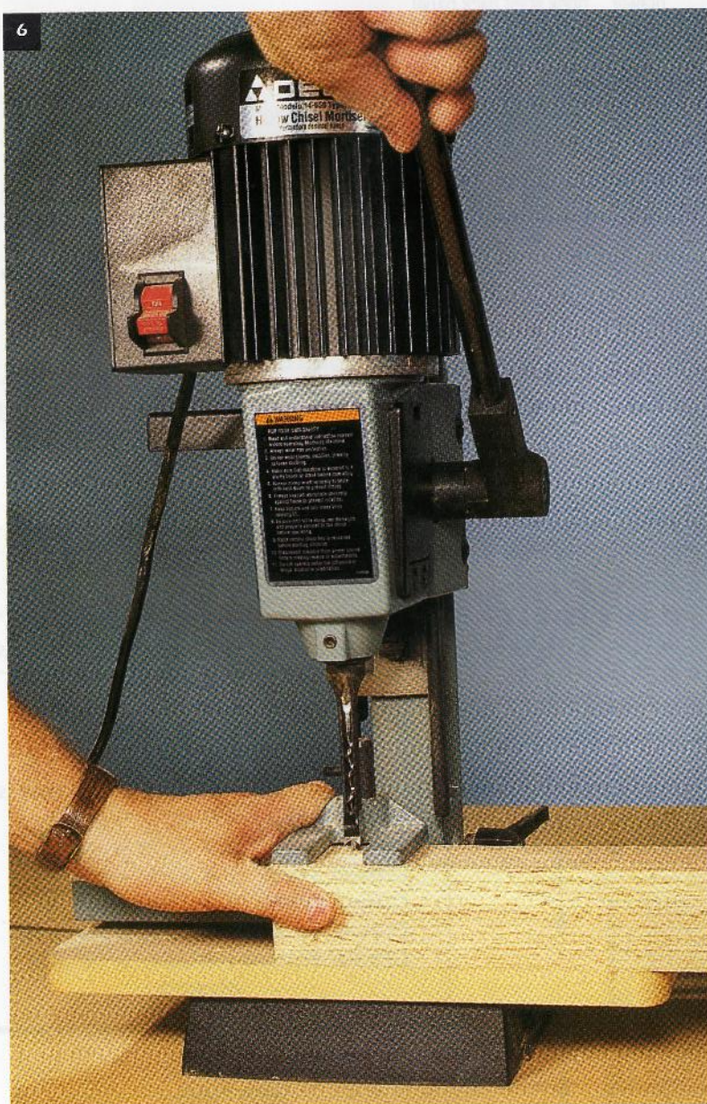
6. The quickest and most accurate way to mill a mortise is to use a dedicated machine.
