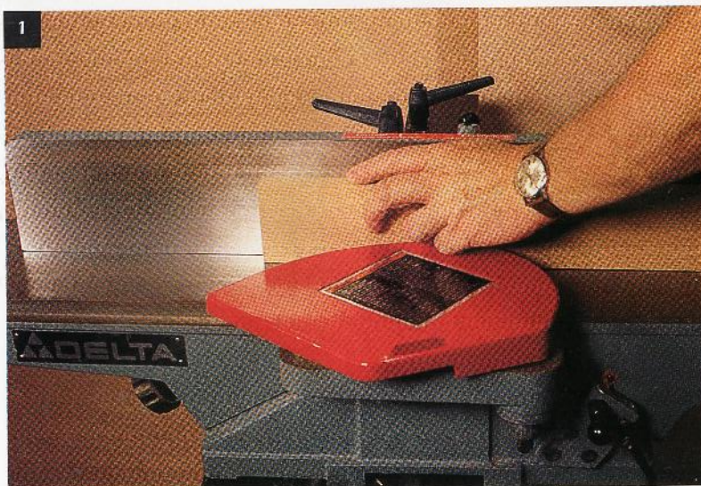
1. True the edges of all pieces of stock on your jointer.
