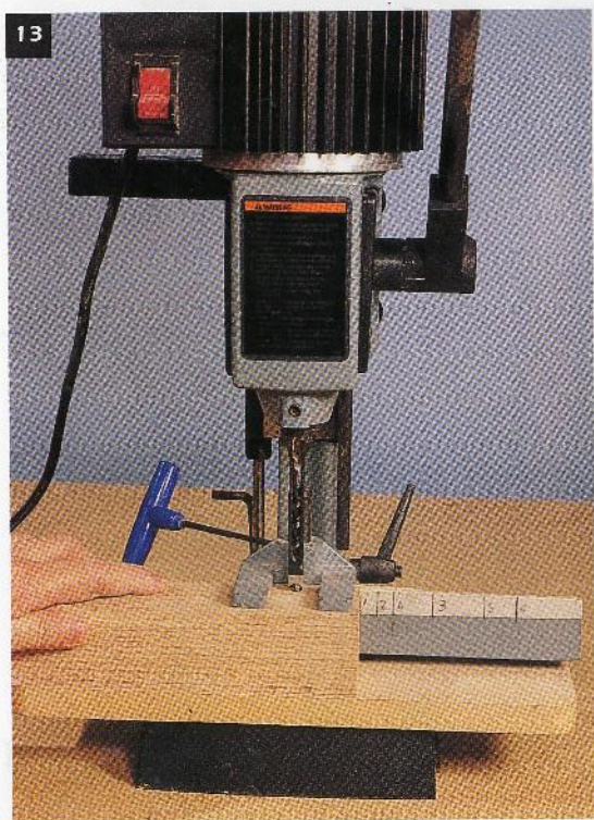
13. Use witness marks on the back fence of your mortising setup to ensure accurately cut mortises.
