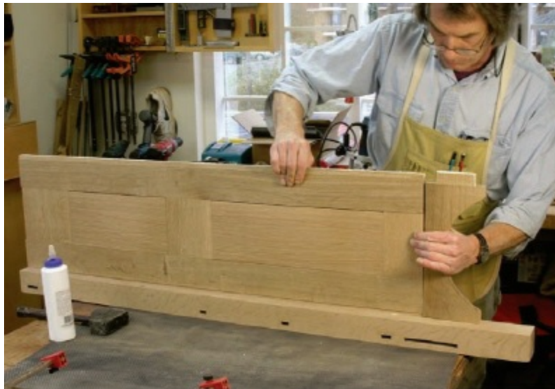
The side panels are assembled as a unit, then fit in a groove in the leg, and butted at the bottom to the thicker arched rail.
