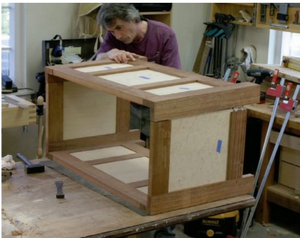
Assembling the front and back panels first simplifies the final assembly — putting the sides together results in a completed case.
