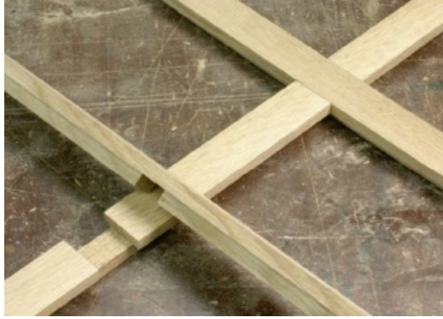
Half-lap joints hold the intermediate stiles and rails of the doors together.
