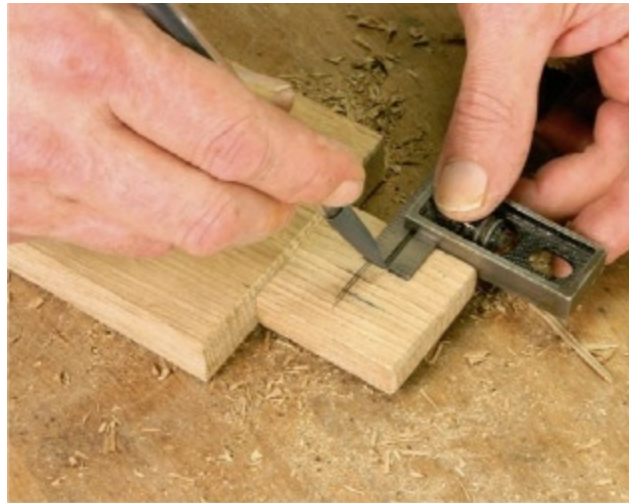
After fitting the through tenon, the location of the second mortise is laid out, keeping the back of the hole just behind the face of the rail.
