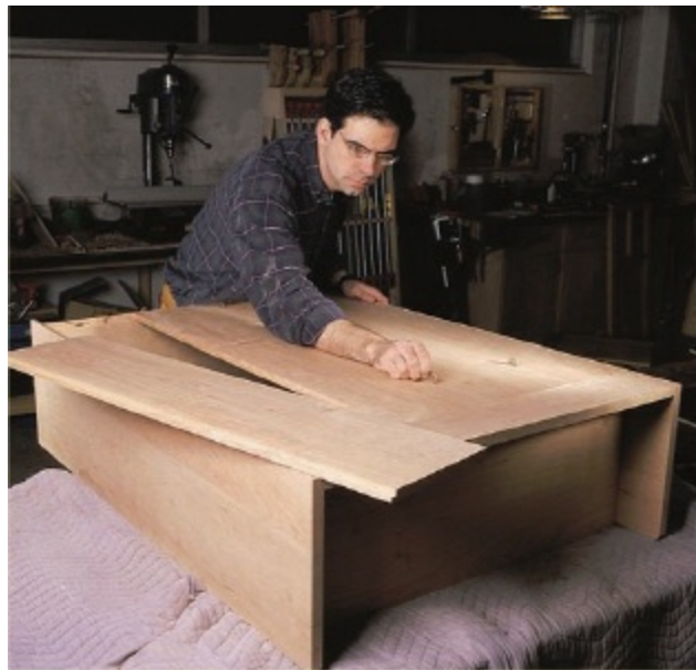
Shiplapped backs allow for solid wood movement.
