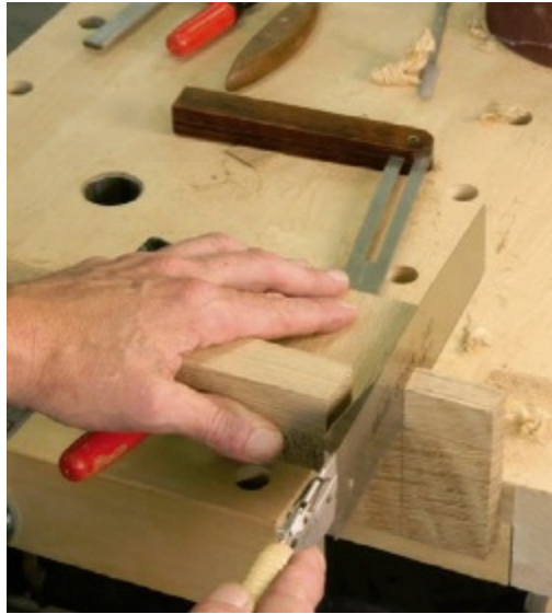
The quick and easy way to make the angled cuts for the through tenons is with a handsaw, guided by an angled block of wood.
