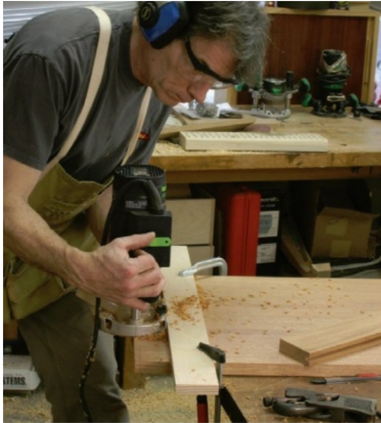
A piece of plywood clamped across the top guides the router to cut the tongue for the breadboard ends.
