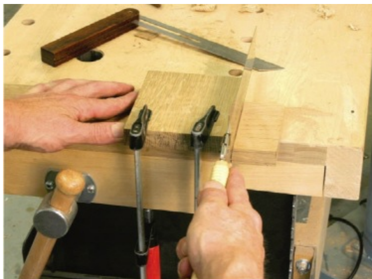
These angled shoulder cuts would be tricky to make with power tools.
