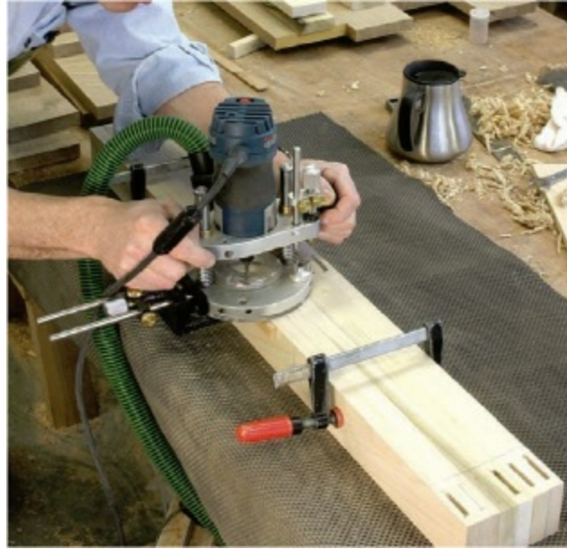
A group of stiles for the web frame is clamped together to lay out the joints. Leaving the stack clamped together provides a stable base for the router used to cut the mortises.
