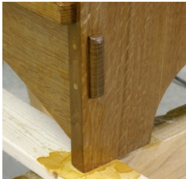
Garnet shellac adds some color, and highlights the distinctive grain. Dark wax will complete the finish.
