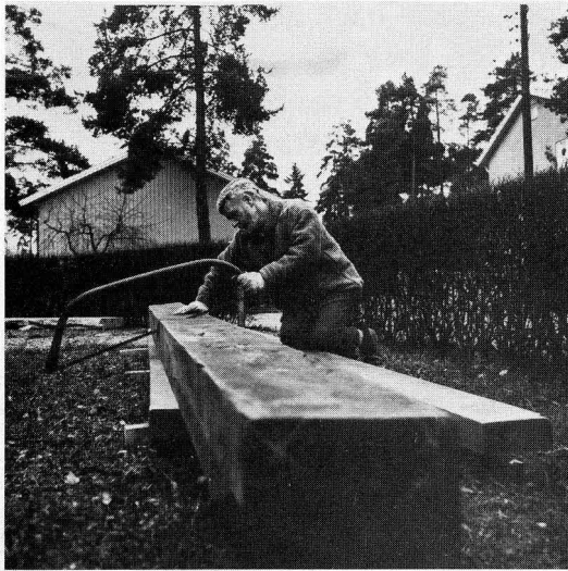
Above: Much of the blackwood being sawed has cracked through the years; only part of it will finally be usable. But that part is hard, fine to work—beautiful. (See cabinet, page 121.)
