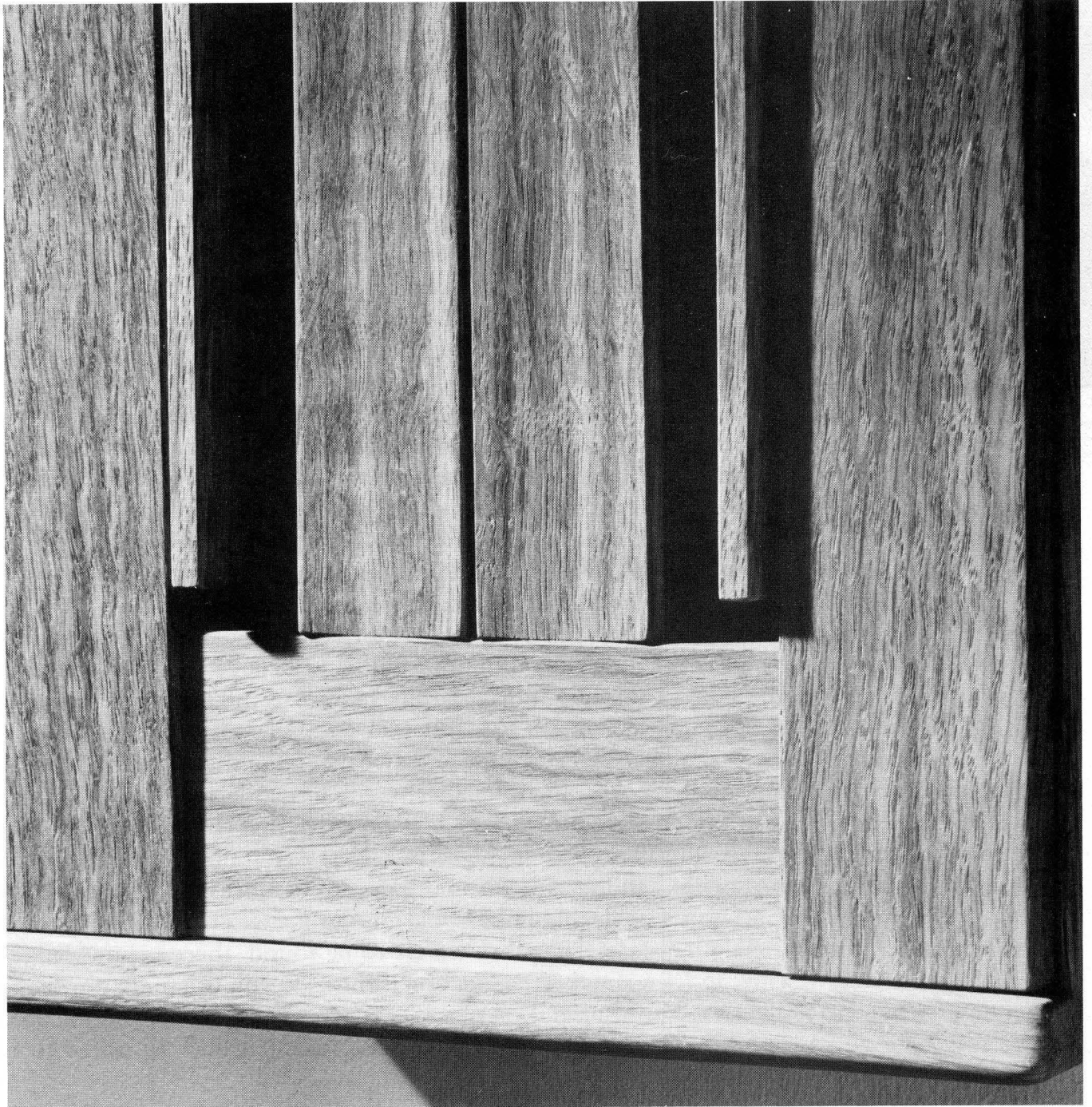
Details of pipe cabinet: grip at right-hand edge of door (left) and closeup of the door. The middle pieces of the door are hand-planed into a slight hollow.
