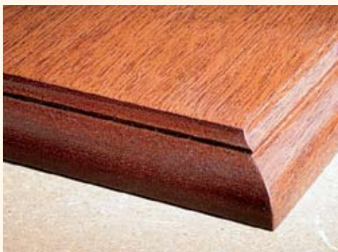
▲ When staining end grain, a regular stain will soak deep into the pores of the wood, darkening the ends much more than the face.
