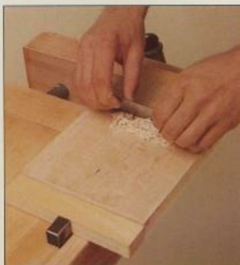
Properly sharpened, a scraper will produce finer and shorter shavings than a plane.
