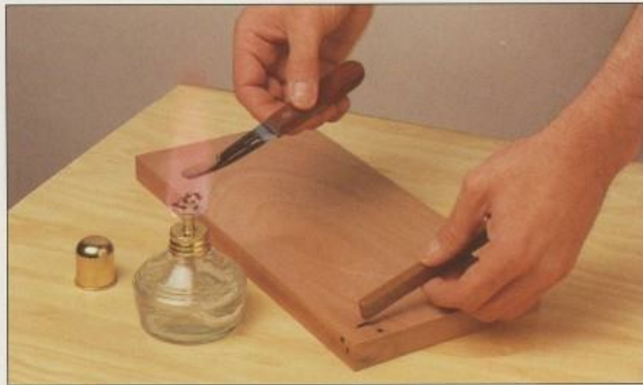
A traditional shellac stick remains one of the best methods of repairing minor damage in wood. Heated by the flame from an alcohol lamp, a burn-in knife melts a small bit of the shellac stick, which fills the hole level with the surface.
