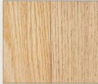
Applying a filler to an open-grained species like oak does more than simply fill the wood pores. In contrast with the natural surface on the right, the filler added to the sample on the left has accentuated the wood's grain pattern.
