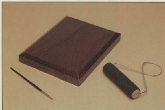
A deftly wielded artist's brush and a grain-rolling roller combined to etch a vivid pattern of heart grain on a piece of particleboard.
