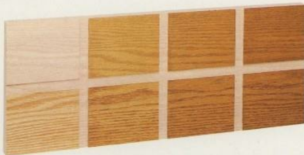
A test strip takes the guesswork out of staining. This sample illustrates the effects on unstained oak of one, two and three coats of stain (moving from left to right). The bottom half of the strip is topcoated to show how the stain looks under a clear finish.
