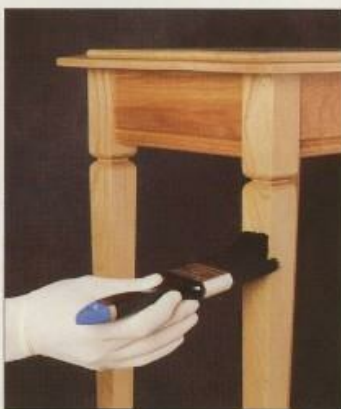
A varnish topcoat brings out the luster of an oak table. Finishing a piece by hand demands care. Loading the brush with too much finish, particularly when coating vertical surfaces, can result in drips and runs.
