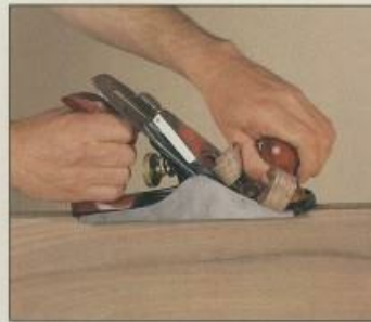
Planing the edges of a workpiece with a smoothing plane—also known as edge jointing—is usually done before planing the faces. This allows you to remove any blemishes from the faces left by the jaws of a clamp or a vise.
