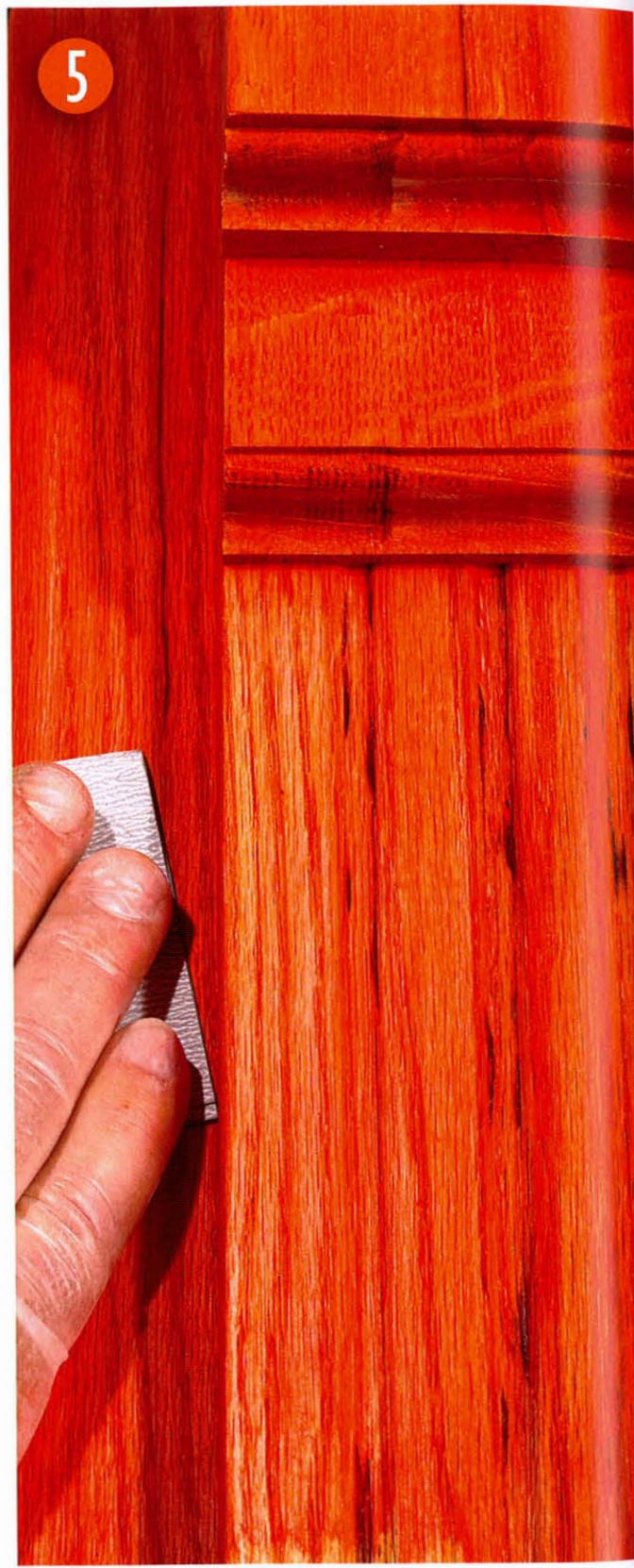
Once the foundation color had dried, I brushed on a sealer coat of orange shellac (photo 4). All the flat sections of the wood were then lightly sanded using 320-grit silicon carbide sandpaper (photo 5).
