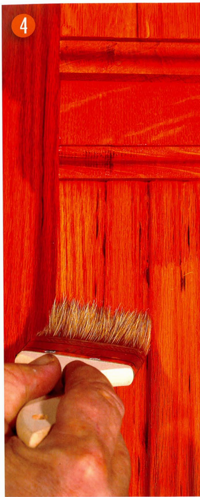
Once the foundation color had dried, I brushed on a sealer coat of orange shellac (photo 4). All the flat sections of the wood were then lightly sanded using 320-grit silicon carbide sandpaper (photo 5).
