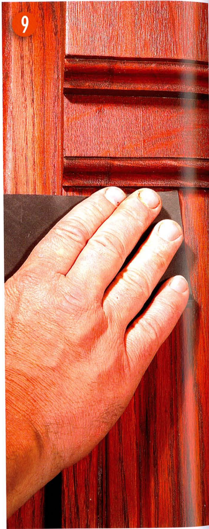
When the shellac had dried, I sanded lightly with 320-grit sandpaper.
