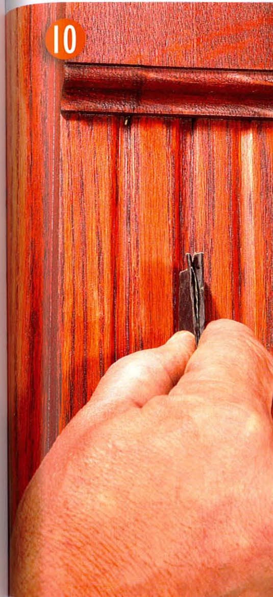
Notice how I have folded the paper to lightly sand the flutes of the pilaster. After dusting and tack-ragging, you can top coat with lacquer or varnish. Do not use polyurethane because it will not adhere to the shellac.
