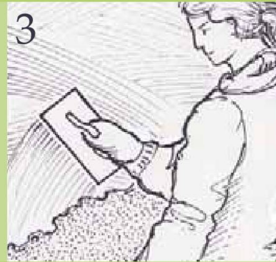
3 Spread mortar upwards in a wide arc.
