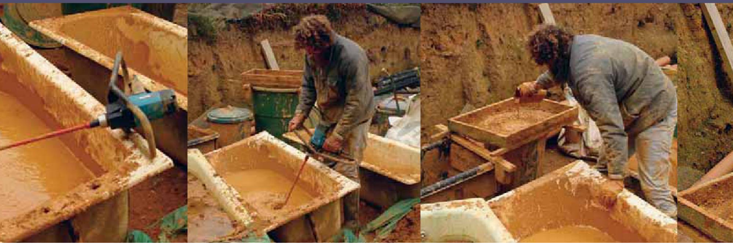
Left to right: Clay soaking in an old bathtub. Blending the soaked clay to break down large clods. Sieving the soaked and blended clay.
