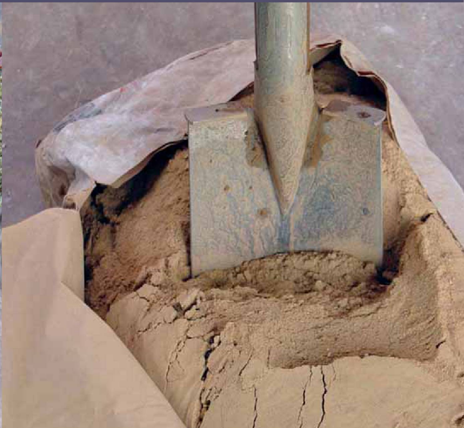
Above left: Dry clay and aggregate mix for an earth plaster. Above right: Sieving dry clay through a sieve set up at a 45 degree angle. Middle left: Straw can be used in earth plasters to provide tensile strength. It must be chopped into short lengths for ease of application. Bottom left: Kaolin clay can be used to make earth plasters. Below: A pre-manufactured earth plaster. It simply needs the addition of water.
