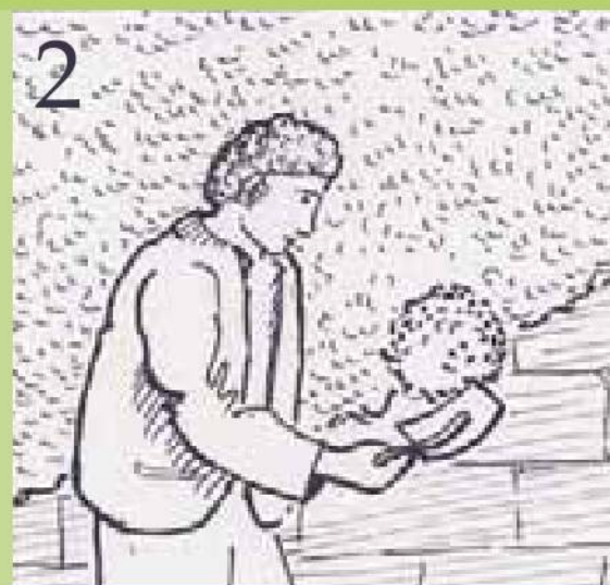
Stand at right angle and forcefully flick the mortar onto the wall evenly.
