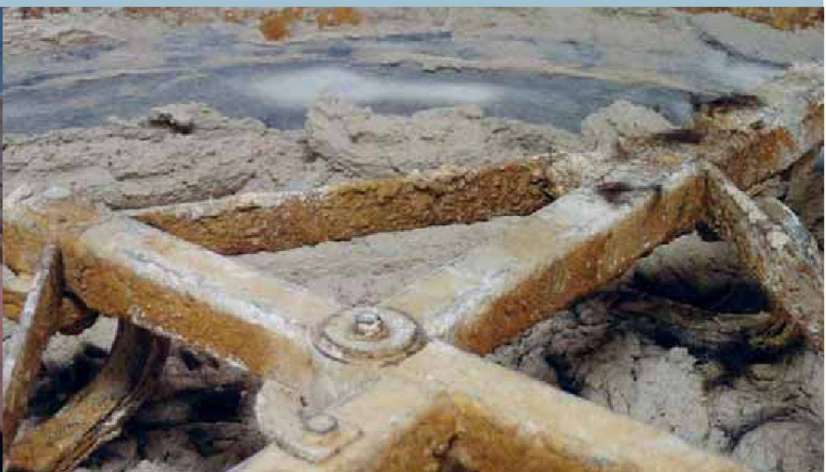
Left: Teasing in animal hair to a mortar mill. Right: Hair being blended into a lime-aggregate mix in an industrial-sized pan mixer.
