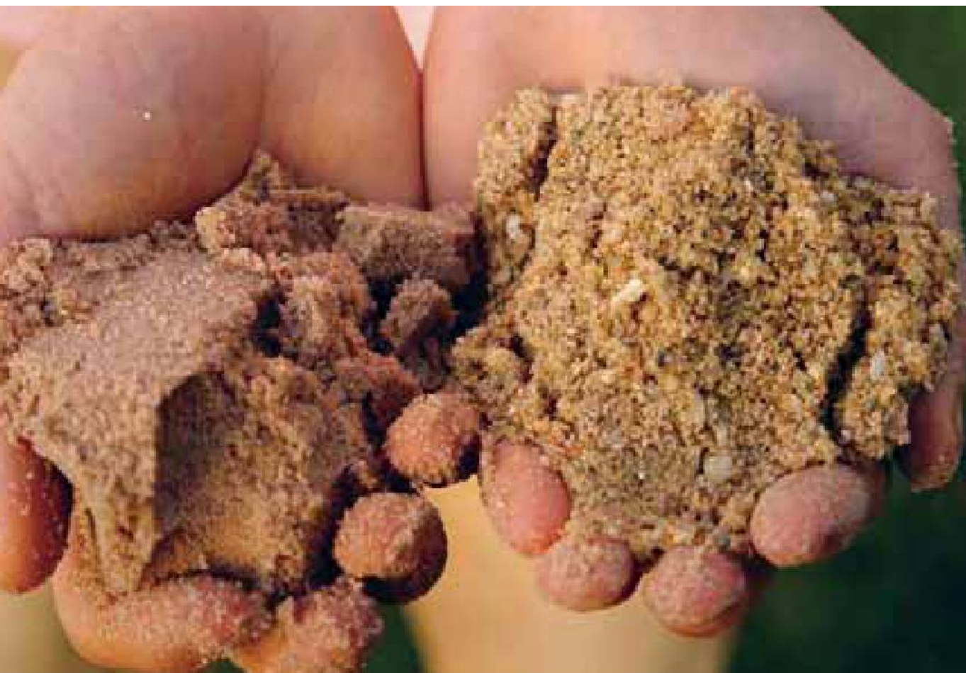
Left: Well-graded fine aggregate for internal finishing coats (left hand), and well-graded coarse aggregate for base coats and external finishing coats (right hand). Right: Home-sieving aggregate to create a well-graded mix.
