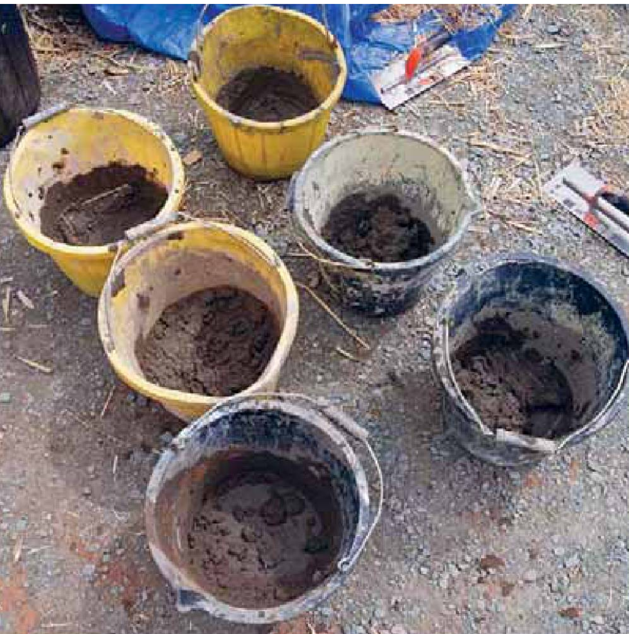
Left: A variety of sample earth plaster mixes with differing proportions of clay and aggregate. Right: The samples are applied to the wall to be plastered, allowed to dry, and then monitored for cracking, durability, adhesion and dusting.
