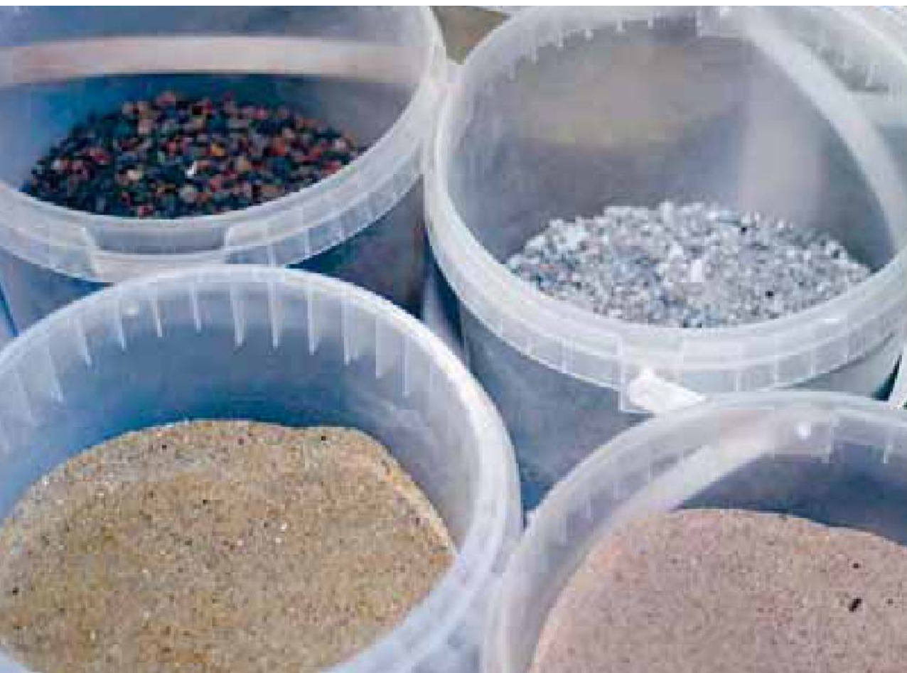
Left: Different aggregates used for making lime plasters and renders. Right: A range of synthetic and natural animal fibres used to give tensile strength in lime renders and plasters (yak, goat and horse hair, and polypropylene fibres).
