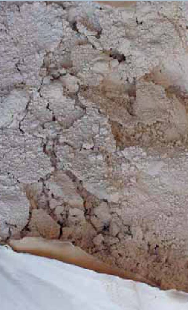
Natural hydraulic lime powder after it has been fired in a kiln and slaked with small amounts of water or steam.
