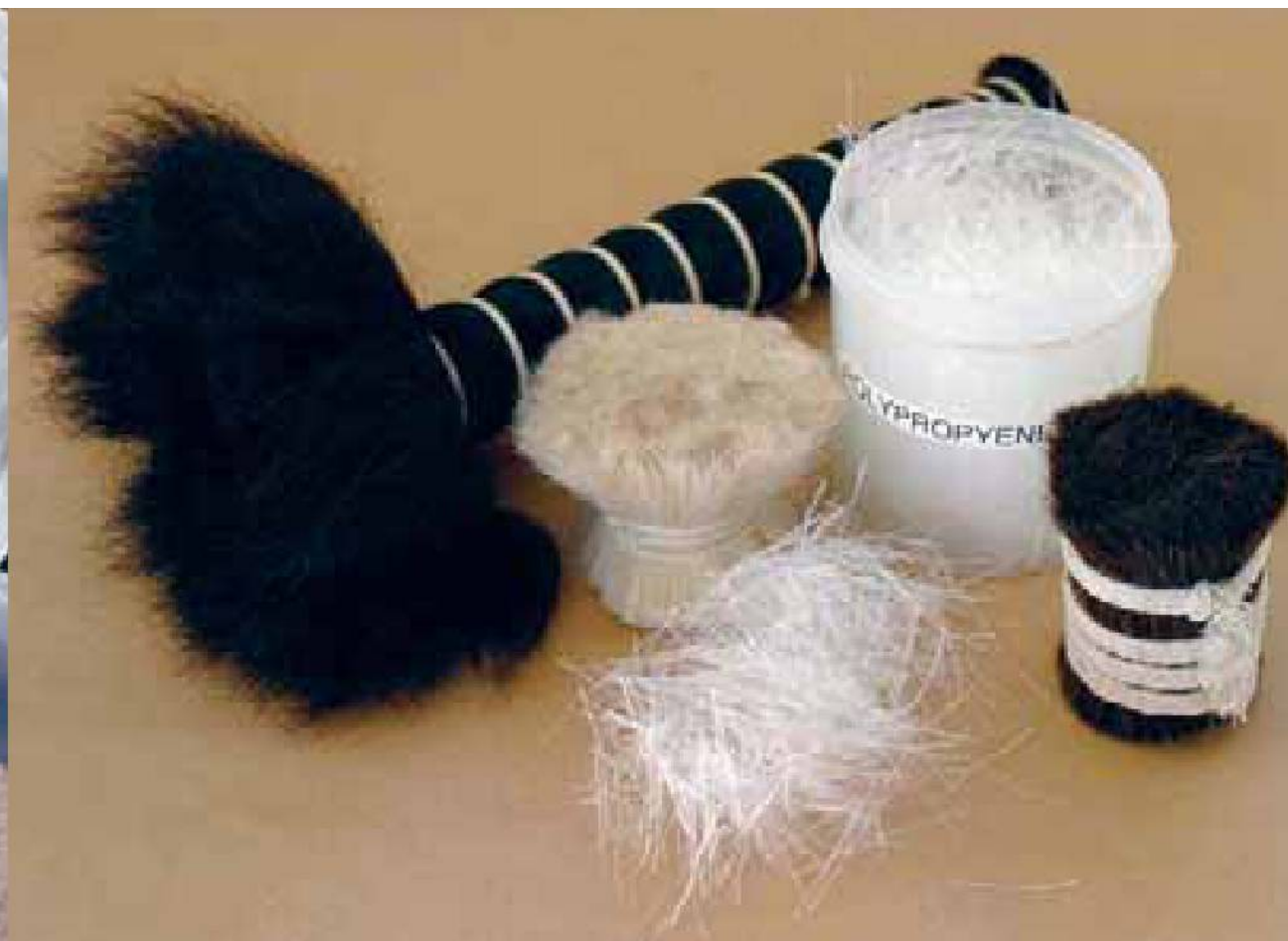
Left: Different aggregates used for making lime plasters and renders. Right: A range of synthetic and natural animal fibres used to give tensile strength in lime renders and plasters (yak, goat and horse hair, and polypropylene fibres).
