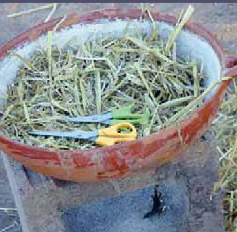
Above left: Dry clay and aggregate mix for an earth plaster. Above right: Sieving dry clay through a sieve set up at a 45 degree angle. Middle left: Straw can be used in earth plasters to provide tensile strength. It must be chopped into short lengths for ease of application. Bottom left: Kaolin clay can be used to make earth plasters. Below: A pre-manufactured earth plaster. It simply needs the addition of water.
