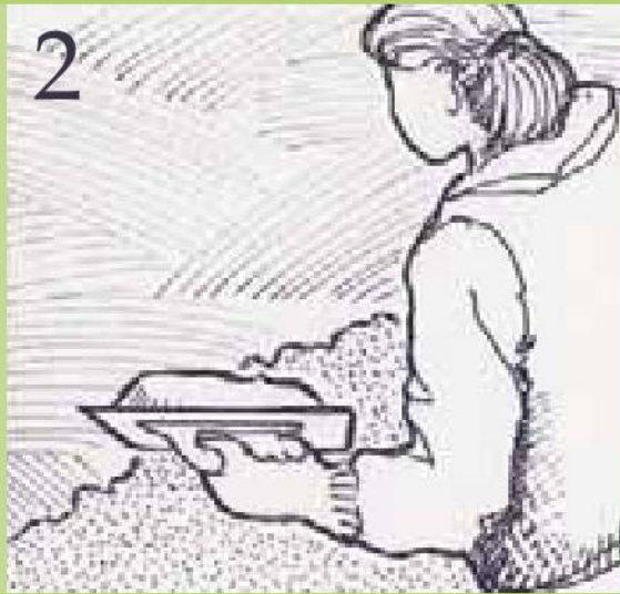
2 Position trowel up against wall with the leading edge open.
