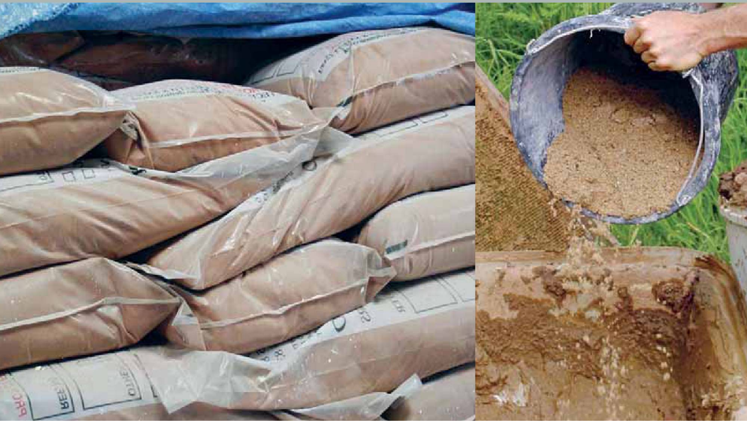
Left: Sacks of brick dust, used as a pozzolan. Right: Adding a well-graded coarse aggregate into a base coat earth plaster.
