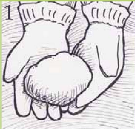
Scoop up a handful of mortar and mould into a flat pancake.
