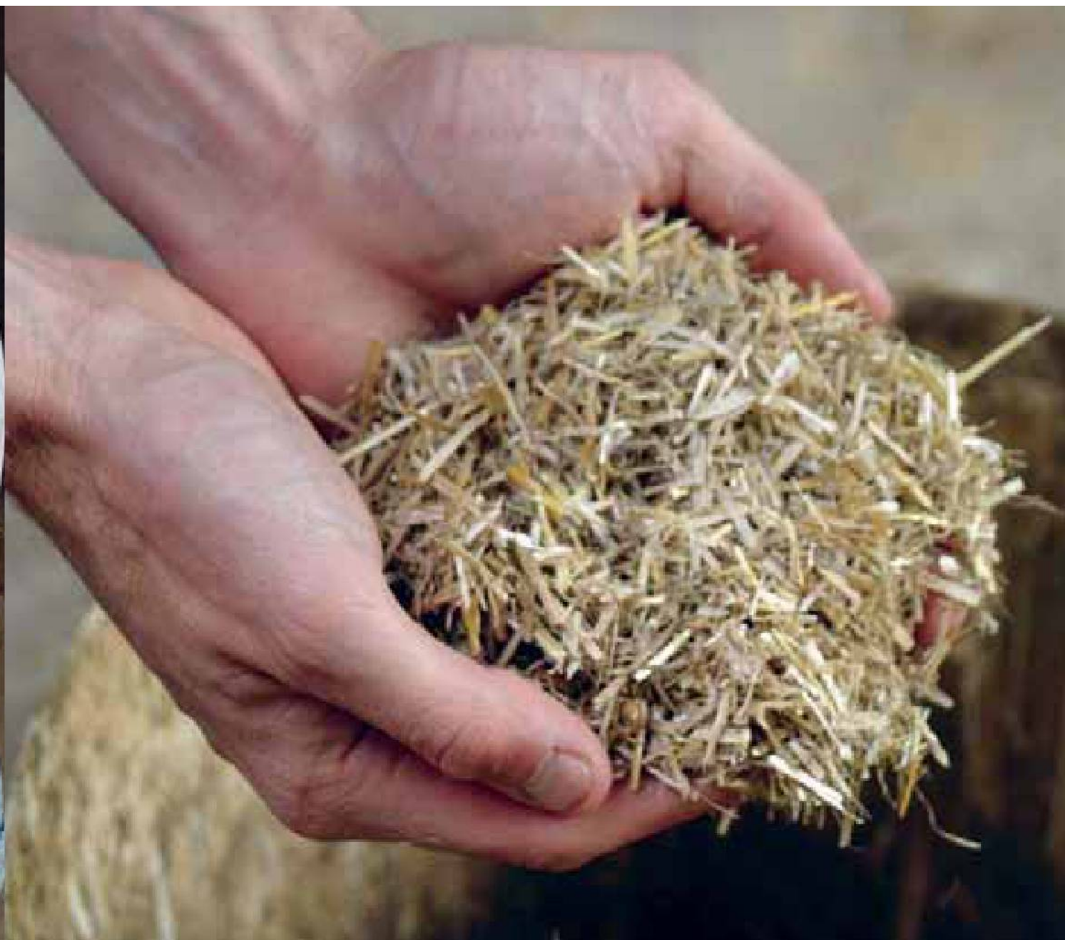
Above left: Sieving straw for the finishing coat. Above right: The fine, sieved straw ready to be mixed into an internal finishing coat earth plaster. Below left: Processing long fibres of straw through a leaf mulcher to chop it to the desired length. Below right: Adding the processed straw to the earth plaster mix.
