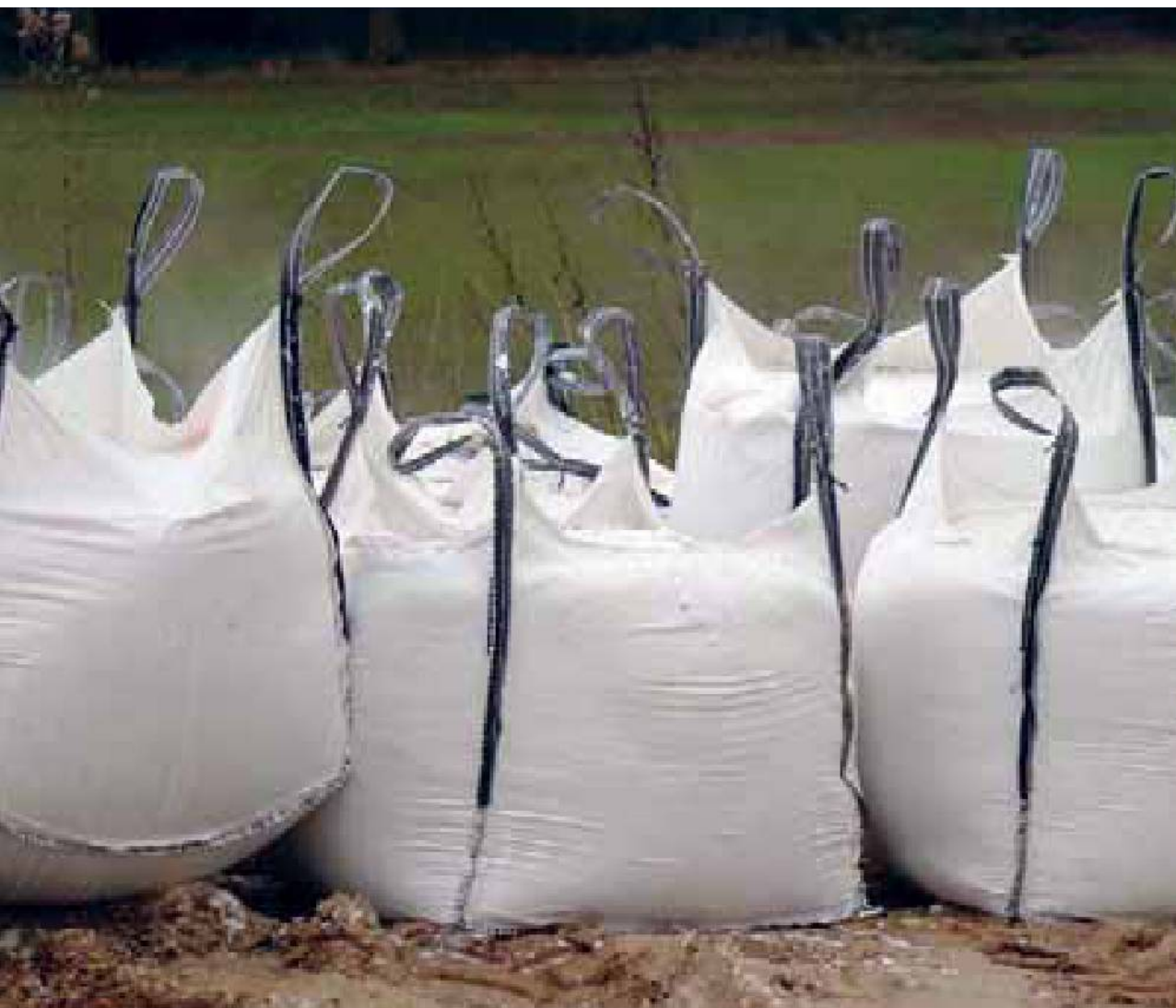
Left: Steaming non-hydraulic lime putty stored in 1-tonne sacks after it has been slaked. Right: 1-tonne ready-mixes being delivered to site.
