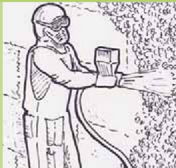
Spray the wall with clay or lime slip standing back approximately 300mm (12") from the wall.
