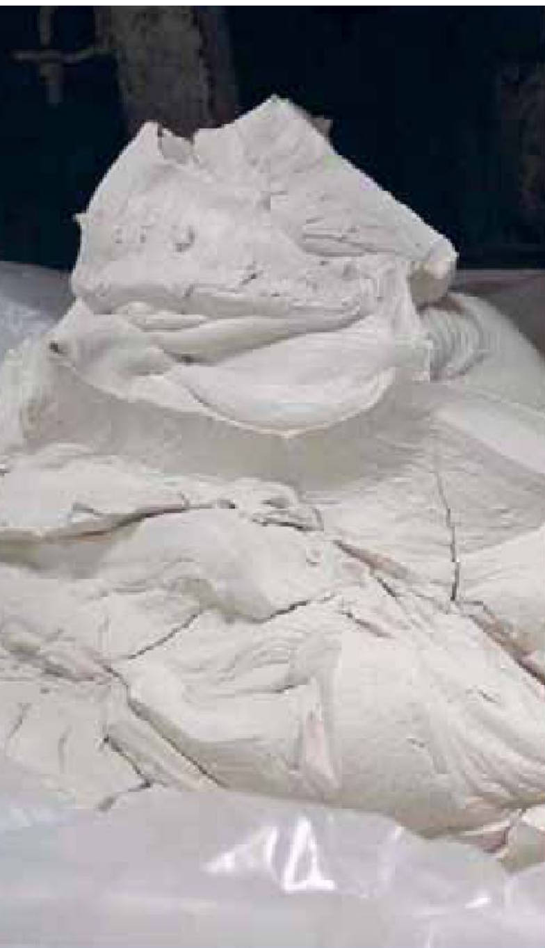
Non-hydraulic lime putty maturing after it has been fired in a kiln and slaked with water.
