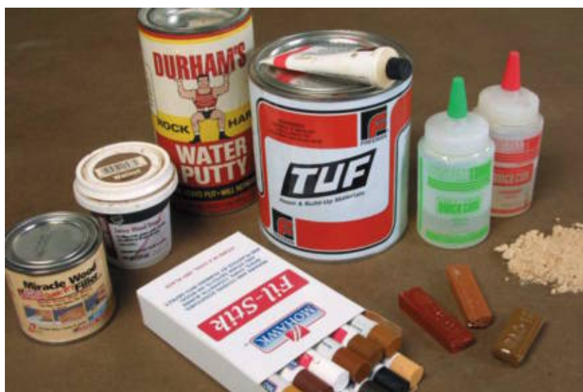
Wood fillers (clockwise from left): solvent-based and latex premixed putties; powdered putty; polyester resin, epoxy, and sanding dust; resin sticks; and wax crayons.
