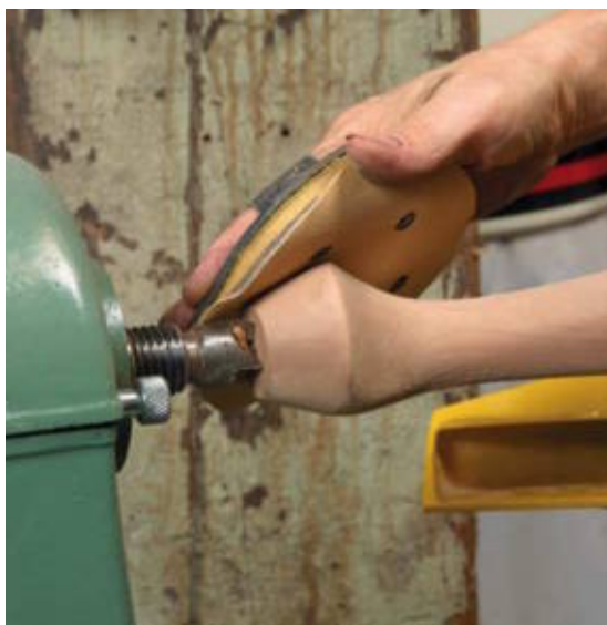
A grip-backed hand-sanding pad outfitted with a ½-in.-thick cushioned interface pad is perfect for sanding curved or complex parts, like this cabriole leg.
