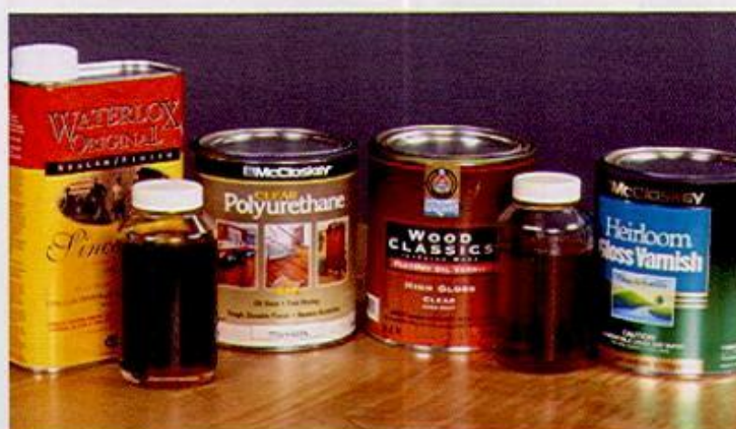
Particular varnishes vary in their characteristics. Tung oil/phenolic resin varnishes (far left) tend to be the darkest, while soya alkyds are the lightest (far right). The Fast-Dry varnish, second from right, is a vinyl-modified alkyd.
