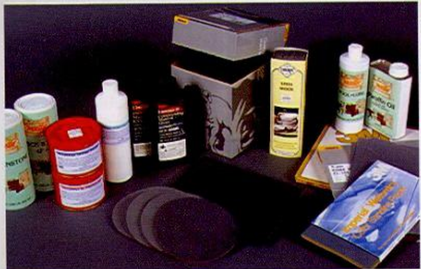
Various abrasives are used for rubbing out finishes. From left, dry pumice and rottenstone powders; compounding pastes and liquid polishes; synthetic and regular steel wool; foam-backed abrasive pads and wet/dry sandpaper; and rubbing lubricants.
