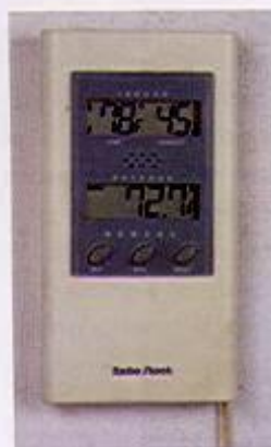
This digital thermometer/hygrometer will tell you when conditions are right for finishing. The temperature and humidity shown here (top row) are about as good as it gets.
