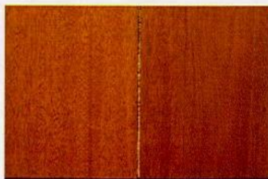
Applying filler over sealed wood creates a better aesthetic, because the filler colors the pores darker than the intermediate areas, providing contrast, as seen at left.
