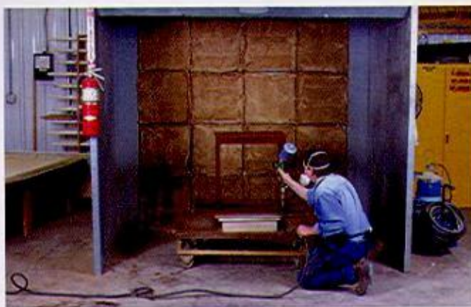
This open-faced commercial metal booth satisfies all local codes with its explosion-proof fan, motor, lights, and metal walls. Note the fire extinguisher at hand.
