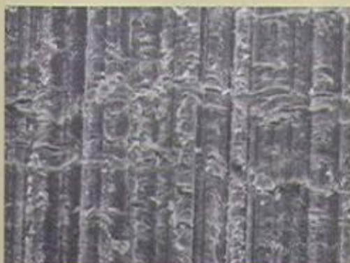
Taken at 100x magnification, the north/south 180-grit scratches shown here are clearly visible as deep furrows running across the grain.
