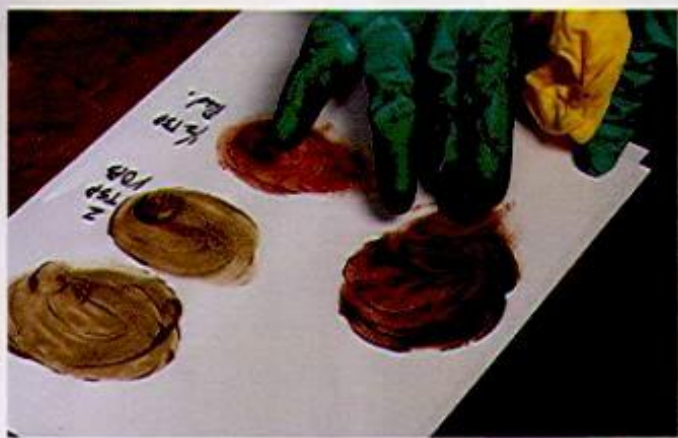
It's easy to gauge the color and intensity of a custom-made glaze mix by smearing some of the test mix on a sheet of white paper.
