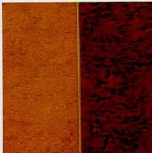
The pigment gel stain applied to the left side of this panel masks the bird's-eye figure, while the water-based dye on the right enhances it.
