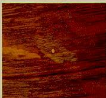
The lighter smudges around this nail hole are a result of the stain not taking to the residual smeared filler.
