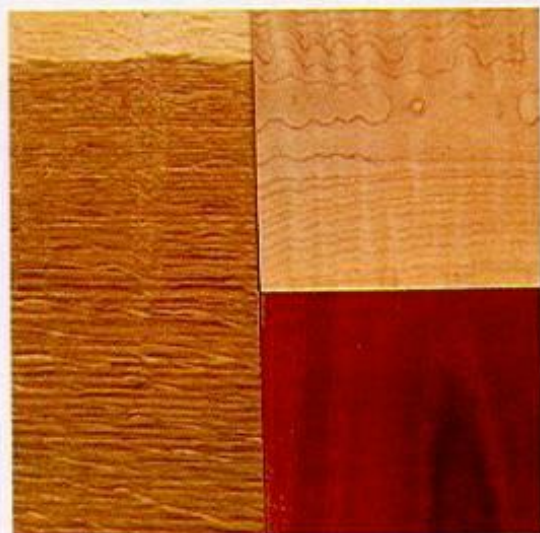
Alkali stains react to tannins in the wood. Clockwise from top right, sodium carbonate on maple, lye on cherry, and ammonia on white oak. Note the unaffected sapwood on the edge of the oak.
