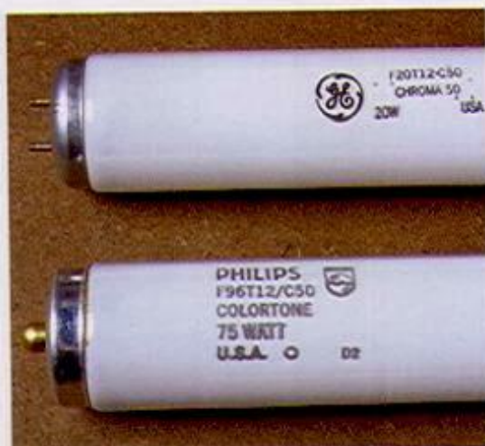
Full-spectrum fluorescent tubes often aren't labeled with their color temperature or CRI rating, but the product name usually includes the number "50," such as "Chroma 50," "Colortone 50," "SPX 50," etc.
