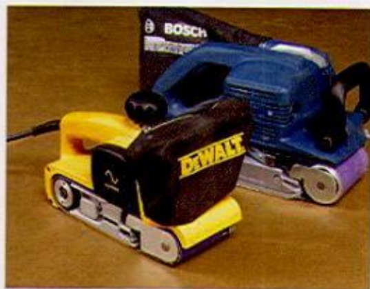
Belt sanders are the most aggressive portable sanding tools. Large, heavy, 4-in. x 24-in. sanders (right) excel at leveling, while a lightweight 3-in. x 21-in. model (left) is better for tasks that require greater maneuverability.
