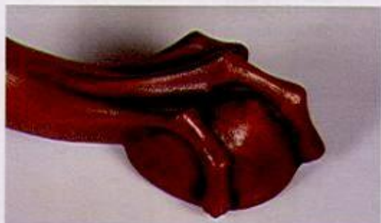
To retain the crispness of carvings, such as on this ball-and-claw mahogany foot, the author applied two light coats of shellac with an artist's brush, followed by a gentle rubbing with 0000 steel wool.
