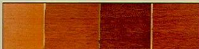
Oil-based filler on mahogany: from left, natural filler, burnt sienna added, black added which cools the color, red added to warm the color.
