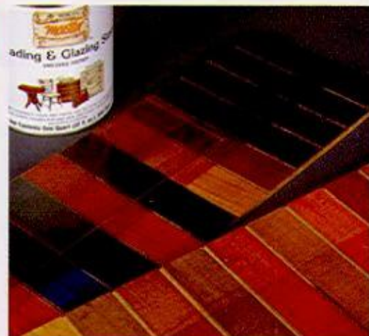
The author's stain boards—one colored with pigment stains and one with dyes—provide a great reference for color matching. A piece of acrylic wiped with glaze allows you to preview the effect that glaze will have over a stain.
