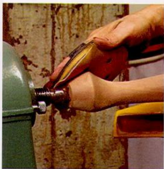
A grip-backed hand-sanding pad outfitted with a 1/8-in.-thick cushioned interface pad is perfect for sanding curved or complex parts, like this cabriole leg.
