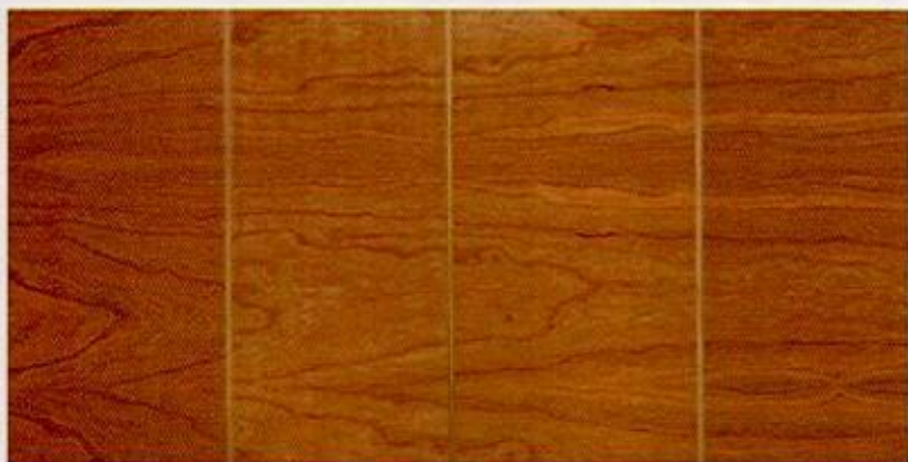
Water-based finishes do not share the same general properties with regard to clarity, warmth, color, grain raising, and flow-out. From left, an exterior-grade water-based spar varnish; an acrylic urethane blend; an acrylic co-polymer; and an oil-modified urethane.
