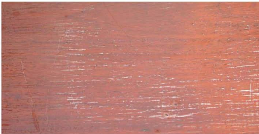
You will be able to see your progress leveling a finish better if you use gloss finish. When you remove the rubbing sludge, glossy spots show the places you haven't sanded enough.
