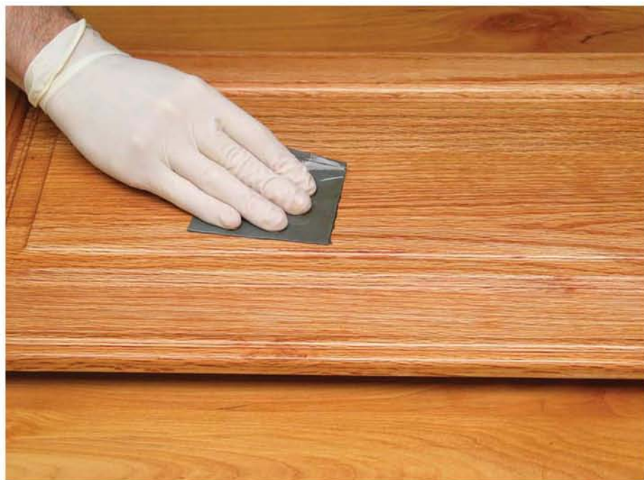
To create the smoothest oil finish possible, sand the second and each subsequent coat while it is still wet with finish (before wiping off) using #600-grit (P1200-grit) sandpaper.
