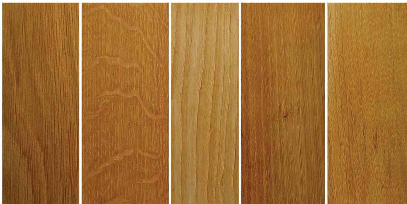
Common coarse-grained woods include from the left: plainsawn oak, quartersawn oak, ash, chestnut and elm. All stains and finishes look good on these woods.
