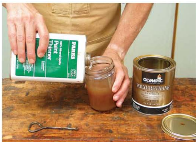
Any petroleum distillate or turpentine can be used to thin wax, oil or varnish, but mineral spirits (paint thinner) is best. It gives the finish time to level and is less expensive and has less unpleasant odor than turpentine.
