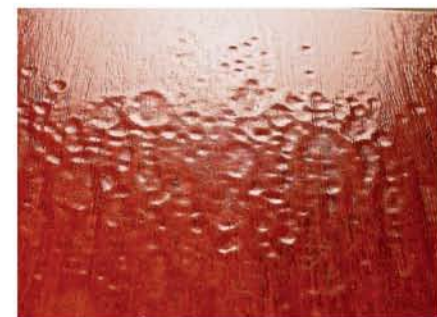
Myth 8: Silicone in furniture polish does not damage your finish. The only problem silicone can cause are craters or "fish eyes" when the wood is refinished. This will take more effort to overcome.
