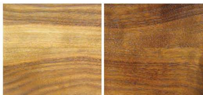
The dye stain applied to the right side of this walnut board is fairly effective at blending the sharp contrast between sapwood and heartwood.
