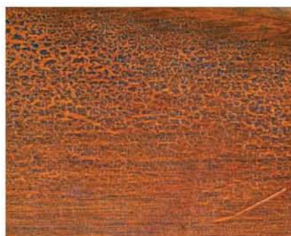
Finishes that have softened and become wrinkled (and also dirty) because of extended contact with acids contained in body oils and sweat (as shown at left) usually have to be stripped and replaced with a new finish.
