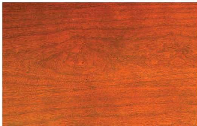
Furniture factories disguise blotching by using glazes and toners to put most or all of the color in the finish rather than in the wood. This creates a different appearance than naturally aged cherry.
