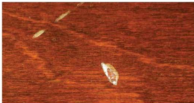
A weakness of sanding sealer is that it can crumble under finish topcoats when struck by a blunt object if the sanding sealer is applied thick. Sanding sealer weakens the strength of the finish film, so it's better to not use it except in production situations with many objects.
