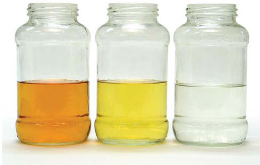
When poured into glass jars, it's easy to see the different colors of lacquers. On the left is nitrocellulose, which is made with fairly orange modifying resins. In the middle is water-white lacquer, which is made with fairly colorless modifying resins. The color that exists is supplied mostly by the nitrocellulose. On the right is CAB-acrylic lacquer, which is totally colorless.
