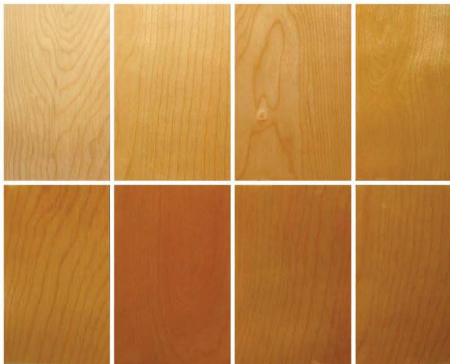
Seven finishes on maple. Top row from left: unfinished, clear paste wax, water-based finish, nitrocellulose lacquer. Bottom row from left: clear/blonde shellac, amber/orange shellac, polyurethane varnish, boiled linseed oil.
