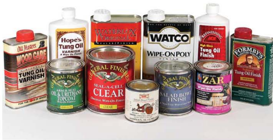
Wiping varnish is any full-strength varnish thinned about half with mineral spirits so it's easy to wipe on wood. All of these products are wiping varnish – though, as you can see, many are labeled to make you think they are something else.
