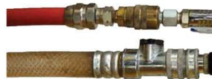
Air hoses also differ for compressor- and turbine-supplied guns. The red air hose is for compressed air. The amber one with a larger diameter accommodates the high volume air produced by a turbine.
