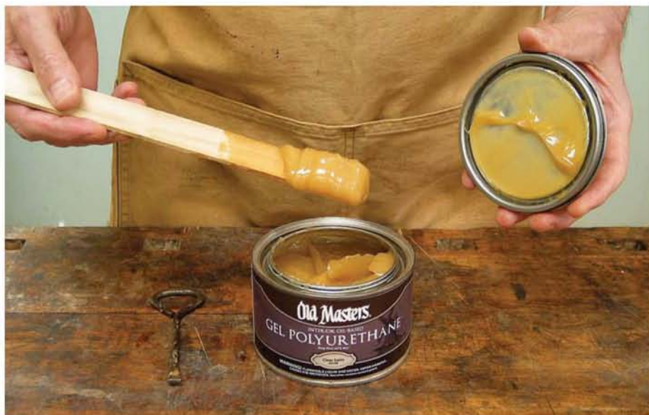
Gel varnish is thick in the can, but it spreads easily because of its thixotropic quality.
