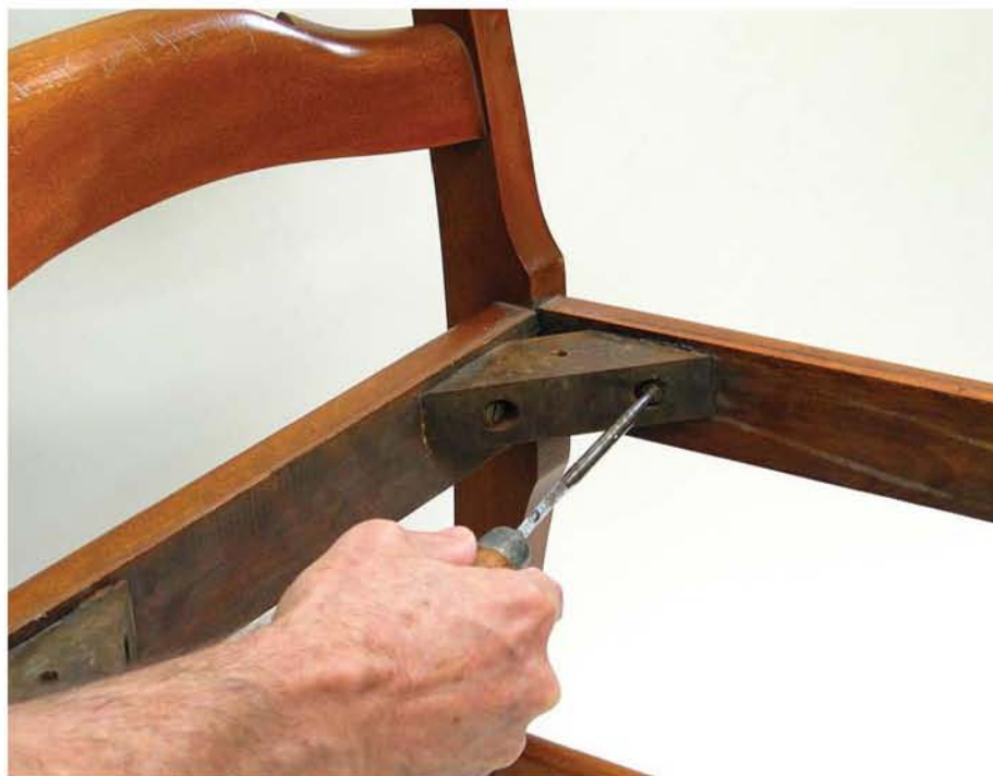
The first step in regluing a chair is to remove corner blocks inserted to support the seat. Remove the screws and then the blocks using a deadblow hammer. If the blocks resist, try wicking denatured alcohol into the bond using a syringe. If these blocks were attached with animal hide glue, the alcohol will crystallize the glue, making it easy to knock them loose.
