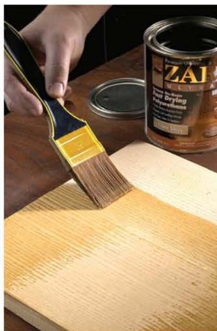
You can brush any of the varnishes I've discussed, including the polyurethane shown here. But brushing and leaving a gel varnish can cause severe ridging.
