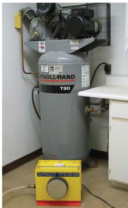
Compressors big enough to supply spray guns sometimes come with wheels but are otherwise not easily portable. Turbines are small and fairly light so they are very portable. This compressor is 5 hp, produces 15 CFM and has a 60-gallon tank. The turbine is three stage—the smallest that atomizes adequately.
