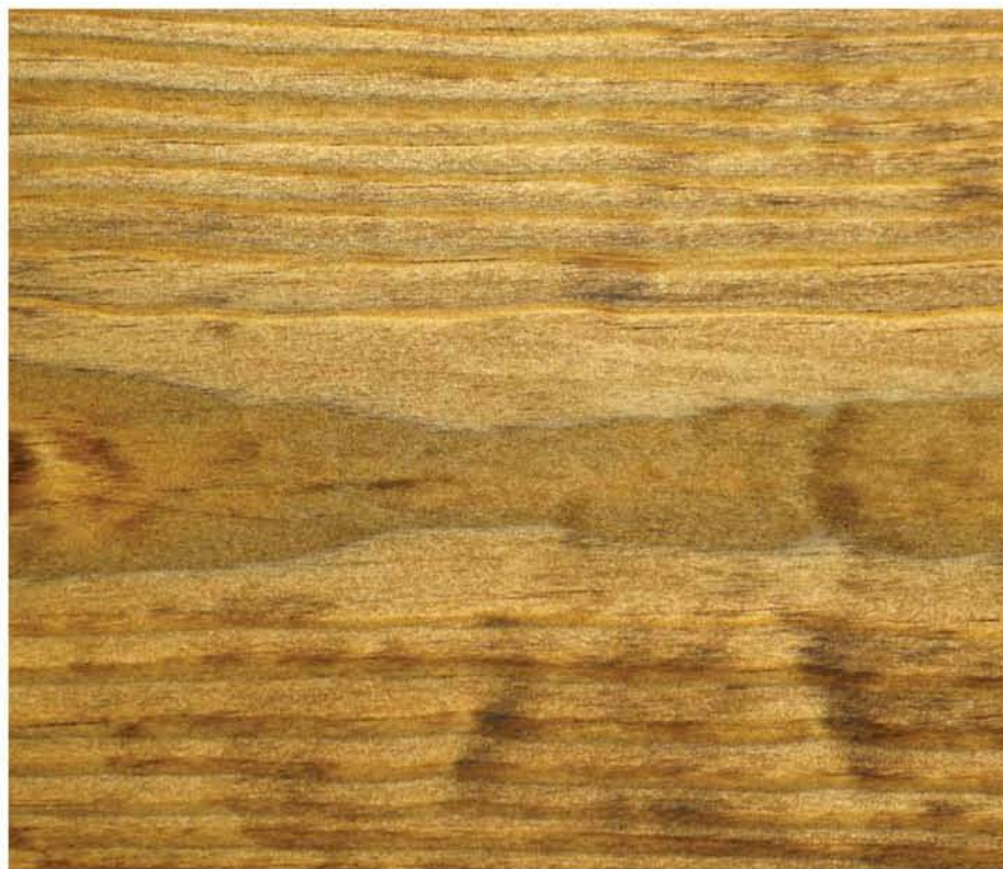
Pine is notorious for the uneven way it takes stain. This Southern yellow pine board was handplaned to perfect shimmering flatness and a liquid walnut stain was applied. The board experienced both grain reversal and significant blotching. In other words, the problems occur with even the most careful preparation.
