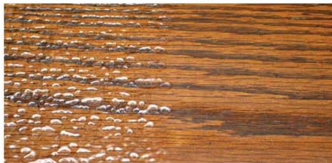
Shellac is extremely useful as a barrier against problems in wood that are commonly encountered when refinishing. This oak has a very bad case of silicone contamination, which causes fish eye (left). A sealer coat of shellac (right) "seals off" the silicone so a lacquer finish can be sprayed on top without problems.
