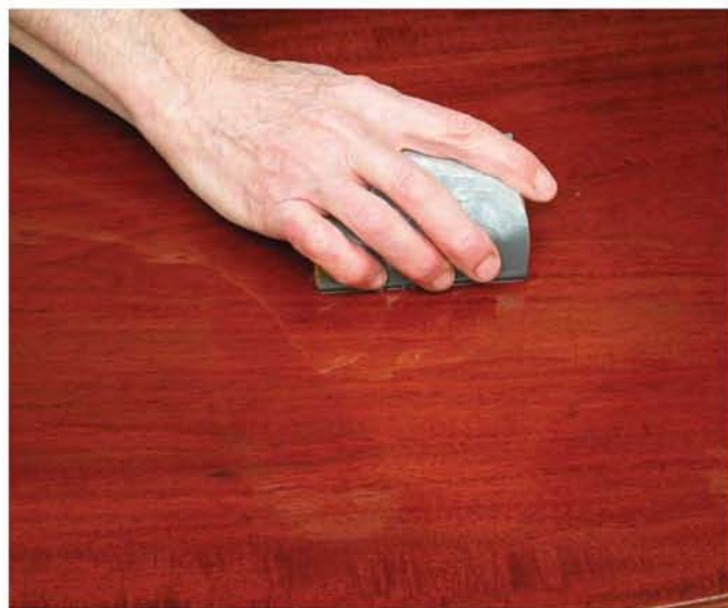
If you want to create the most perfect results when using a film building finish, you have to level it using fine wet/dry sandpaper, a backing block and a lubricant.
