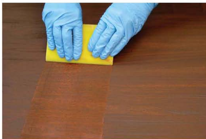
An efficient method of removing the excess grain filler is to scrape it off with a plastic spreader. Then follow with a cotton cloth or burlap. Whichever method you use, finish by wiping lightly with the grain to remove streaks.
