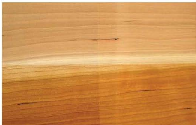
Because the darkening of cherry is accelerated by light, you can place your sanded parts in sunlight for a couple days (as I did with the left half of this panel) and achieve some degree of darkening to begin the process. The bottom half has a clear finish applied. The middle stripe is where some of the UV passed through the masking tape.
