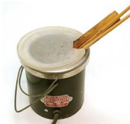
A commercial glue pot maintains the temperature of the glue at an ideal 150 F. To retard evaporation and keep the glue from thickening, I keep the pot covered with a plastic lid. The lid has a cut out for brushes and a stirring stick.
