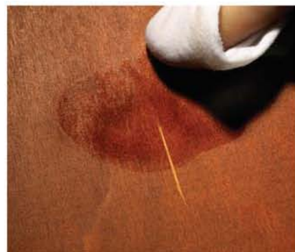
The simple test to determine the procedure to repair a scratch that shows white is to dab some liquid onto it.
