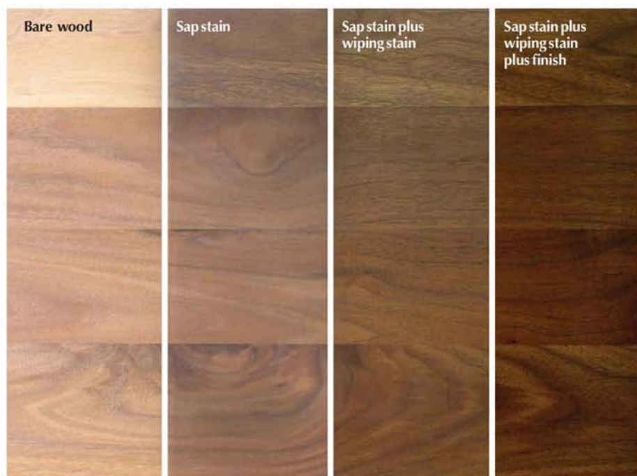
A more effective method of blending sapwood with heartwood is to apply a sap stain (first colored column from the left), then apply a walnut wiping stain and finally apply a finish.
