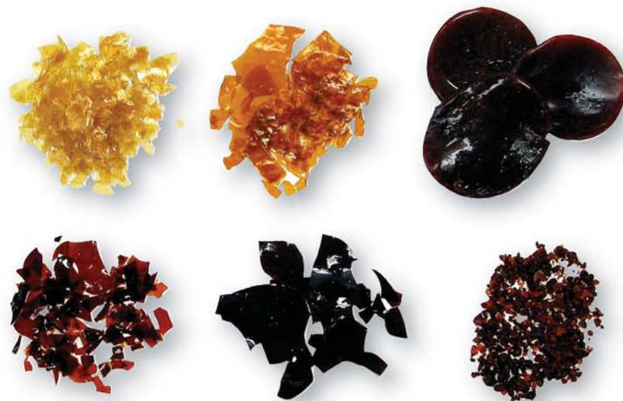
Shellac in flake form is available in various colors and grades. Across the top from left is dewaxed blonde shellac, orange shellac with the wax unremoved and crudely refined button shellac. Across the bottom is dewaxed garnet shellac, dewaxed extra-dark (ruby-red) shellac and totally unrefined seed lac.
