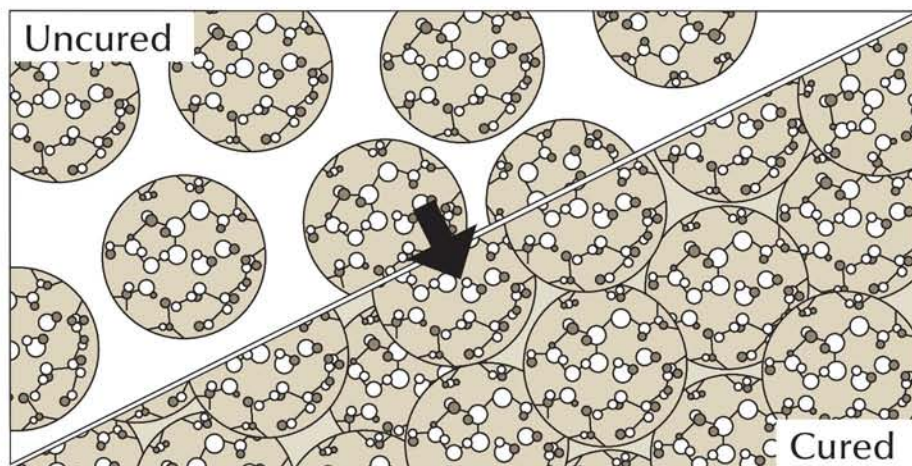
Coalescing finishes (water base) cure as droplets of reactive finish come together and stick to each other when the water, then the solvent, in the finish evaporate. The droplets resemble microscopic soccer balls containing Tinker-Toy-like networks of reactive finish inside each.
