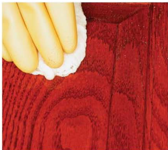
Toluene and xylene are very useful for removing latex paint spatter from all surfaces except water-based finishes. The commercial products Oops! and Goof Off are based on xylene and sold for this purpose.
