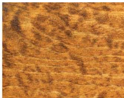
Some woods, such as the pine shown here, blotch when stained. Blotching is the only situation in finishing that can't be fixed fairly easily, with stripping and starting over being the worst-case scenario.
