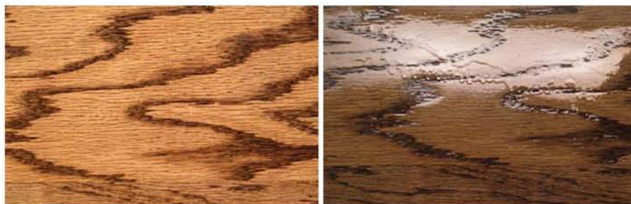
When there's no light reflected in the surface (left), you can't see problems as they develop. Move your head to pick up a reflection from some light source so you can see what's happening – for example, the runs and sags in this finish (right). Once you see a problem, it's usually easy to fix, most often by brushing back over the surface.
