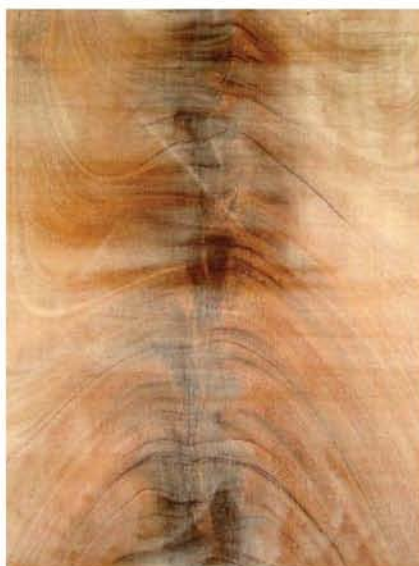
It's nearly impossible to get all water-based grain filler wiped off of wood (such as this crotch mahogany) when no washcoat is applied. You'll have to sand it off, trying to avoid sanding so deep you open up some of the pores.
