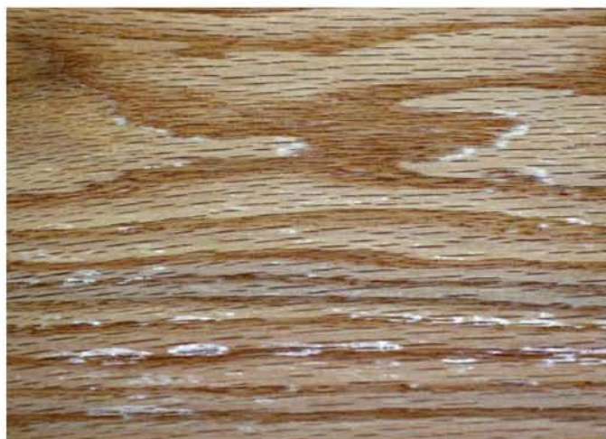
The shiny spots on this oak panel show where an oil/varnish blend has oozed out of the pores and dried on the surface. To keep this from happening, check your project every half hour or so after you apply the finish and wipe off any bleeding before it dries.
