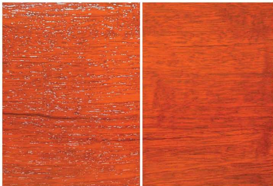
The difference on a wood such as this mahogany between an unfilled surface (left side) and a filled surface (right side) is striking. The pores on the unfilled side break up the light creating a raw look. The filled side looks richer, deeper and more elegant.
