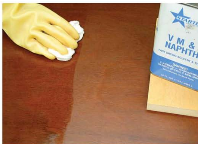
Naphtha is usually better than mineral spirits for cleaning oily or waxy surfaces (including crayon marks) because it evaporates much faster. Naphtha also has more solvent strength than mineral spirits, which is sometimes helpful on old waxed surfaces such as this one.
