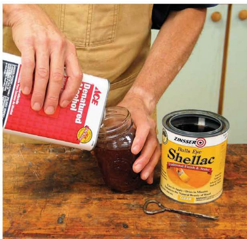
Denatured alcohol is the best solvent for thinning shellac. It is much less toxic than methanol.
