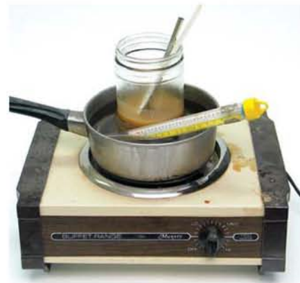
You don't need to invest in a glue pot. Any situation you can arrange that will keep the glue at about 140-150 F will work well—in this case a jar of glue in a pan of water on an electric hot plate. Keep an eye on the temperature.
