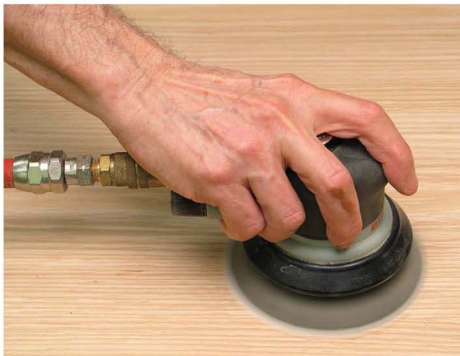
Random-orbit sanders are easy to use and efficient for smoothing wood. To reduce the likelihood of the squiggles these sanders produce, use a light touch. Don't press down on the sander; let its weight do the work.
