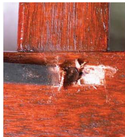
Nails are often inserted into stretchers in factory-made chairs. To remove the nails, first dig out some of the wood on two sides of each using a 1/8" chisel.
