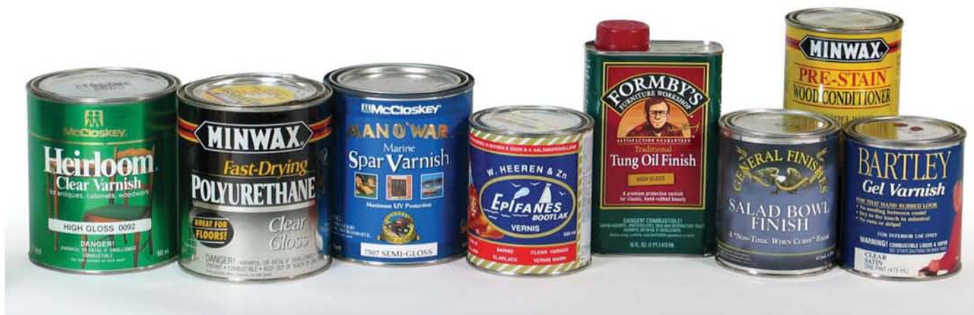
Varnish is the only finish that both thins with mineral spirits and cures hard. All of these products are varnish. From the left: alkyd varnish, polyurethane, spar varnish, marine varnish, wiping varnish, salad bowl finish, wood conditioner and gel varnish.
