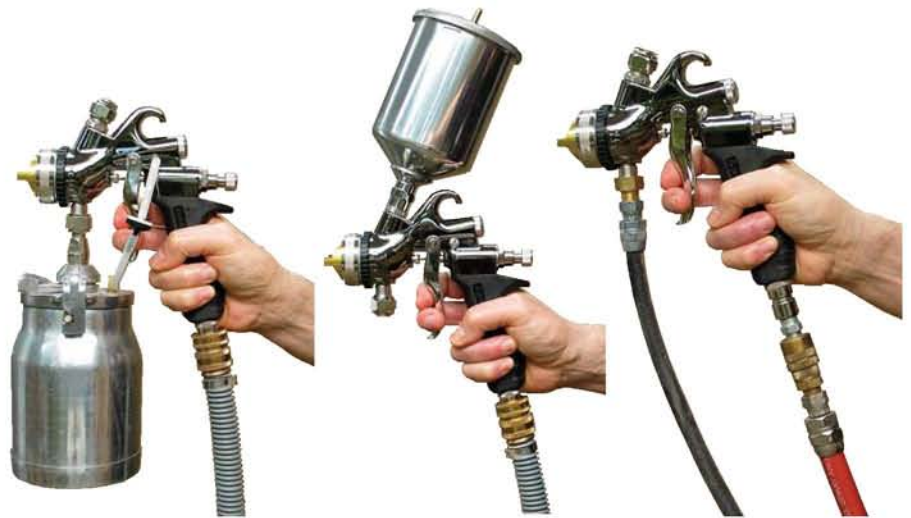
Spray guns are available in three configurations: siphon-feed with the cup under the gun, gravity-feed with the cup on top of the gun, and pressure-feed where the finish is fed to the gun through a hose connected to a separate pressurized pot. To illustrate the three configurations, I'm using the Apollo Atomizer spray gun, which is unique in that it can be set up in all three configurations and it can run off either a turbine or a compressor.
