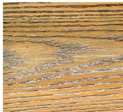
Myth 7: The main reason to sand polyurethane between coats is to level dust nibs and other flaws, not to create a better bond. This is demonstrated here by the gloss remaining in the pores after sanding the surface. The next coat of finish still bonds in the pores even though the finish there is rarely scuffed.
