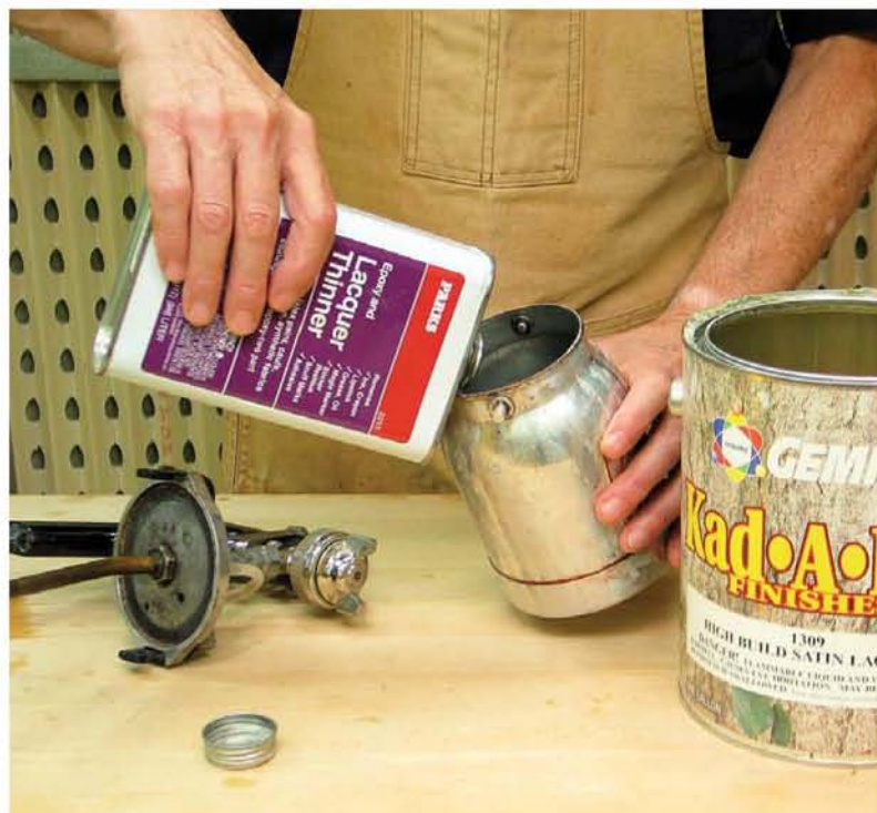
Lacquer thinner is a blend of half-a-dozen or so solvents specially formulated for thinning lacquer. The blend allows for differing evaporation rates and for evaporation in steps to reduce runs on vertical surfaces.
