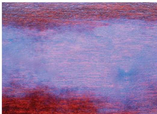
The milky white area in the center of this panel is called "blushing" and occurs often during the application of shellac or lacquer on humid days. To keep it from happening, slow the drying of the finish by adding a little lacquer retarder to it.
