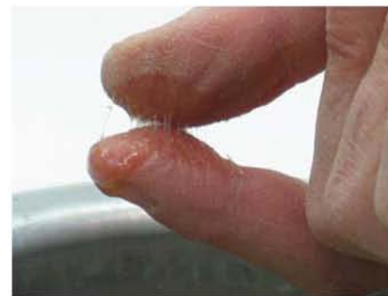
Rub joints work well with hot hide glue because of the strong tack created when the glue cools to about 95 F. Use your fingers to check the strength of the glue as it ages and loses tack. The glue cleans off quickly in hot water.
