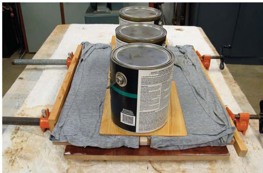
When straightening a board, place it in clamps so the cupped side is face down. Place a wet cloth on the bowed side. Weights encourage compression shrinkage.
