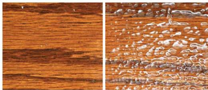
Fish eye (cratering) is one of the most serious problems in refinishing. It's caused by silicone from furniture polishes getting into the wood and causing the new finish to wrinkle when applied. One easy way to avoid fish eye is to block it with a first coat of shellac, applied here to the left side of the board. The only new-wood use for shellac as a first coat is over resinous knots in softwoods such as pine.
