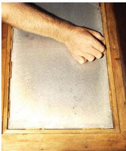
Using small blocks of wood and the rub-joint technique with hot hide glue to install mirrors in frames is far safer than using a hammer to pound in nails or other metal fasteners. In this case, I'm reinstalling a mirror in an old frame after refinishing.
