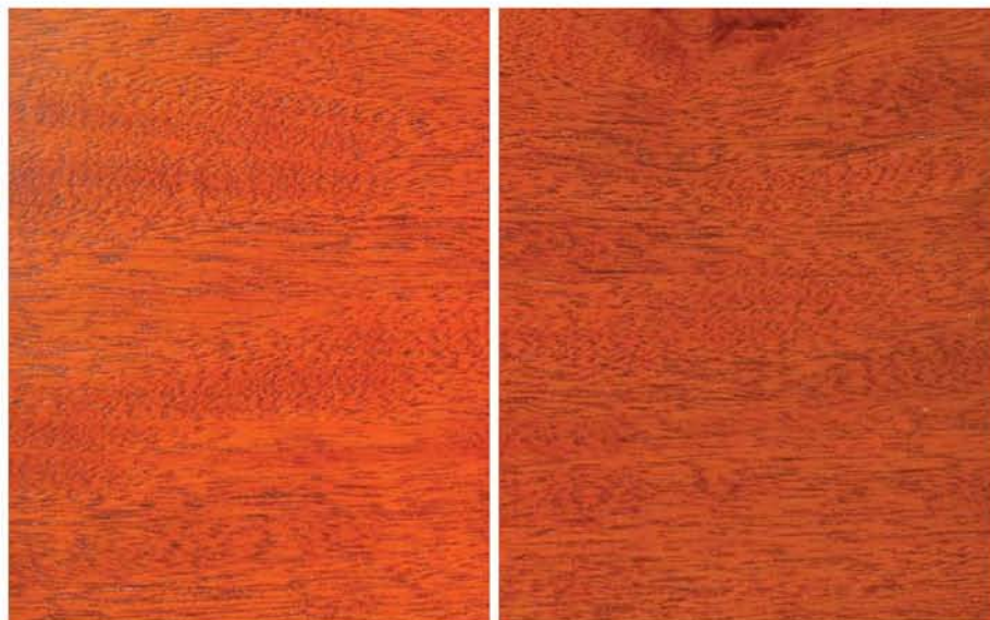
This photo shows how I used a green toner on the right side to “kill” some of the red in the red-dyed mahogany. The added green makes the color more brown.
