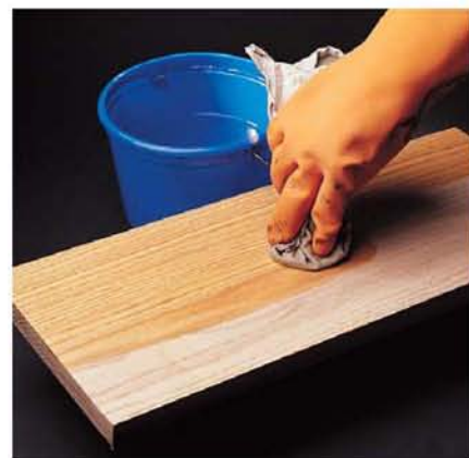
When the wood dries, the crystals will reappear. Wash them off with a hose or wet rag or sponge. Never brush the crystals off the surface because they are toxic to breathe.
