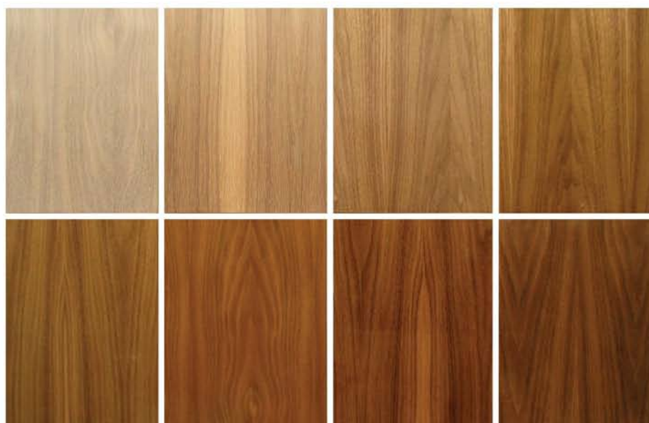
Seven finishes on walnut. Top row from left: unfinished, clear paste wax, water-based finish, nitrocellulose lacquer. Bottom row from left: clear/blonde shellac, amber/orange shellac, polyurethane varnish, boiled linseed oil.
