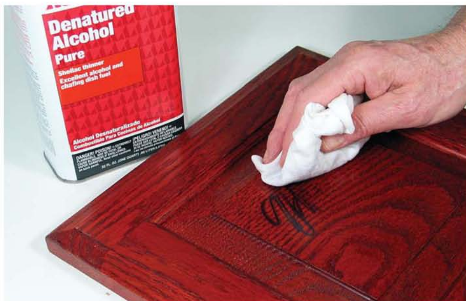
Felt-tip pen marks can be removed without damaging any coating (except shellac) by wiping lightly with denatured alcohol.
