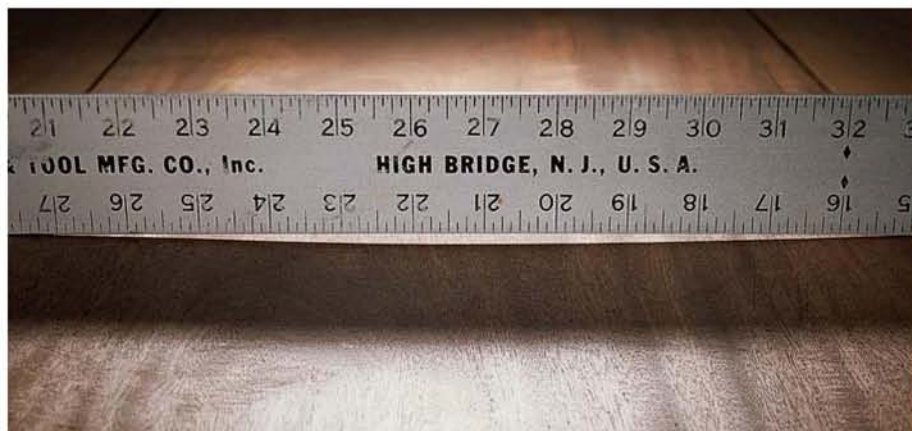
Old tabletops commonly cup on their tops even though the direction of the boards' rings and the fact that the bottom sides are often left unfinished would indicate that the opposite should have happened. The cause is compression shrinkage. The gap of light between the ruler and the wood indicates a warp.
