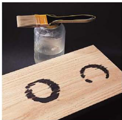
To remove dark water stains, you'll usually have to remove the finish first. Then dissolve some oxalic acid crystals to a saturated solution in hot water.
