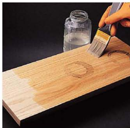
Brush on the oxalic acid solution over the entire surface. The dark marks will begin to fade immediately, though it will take a little longer for them to disappear entirely.
