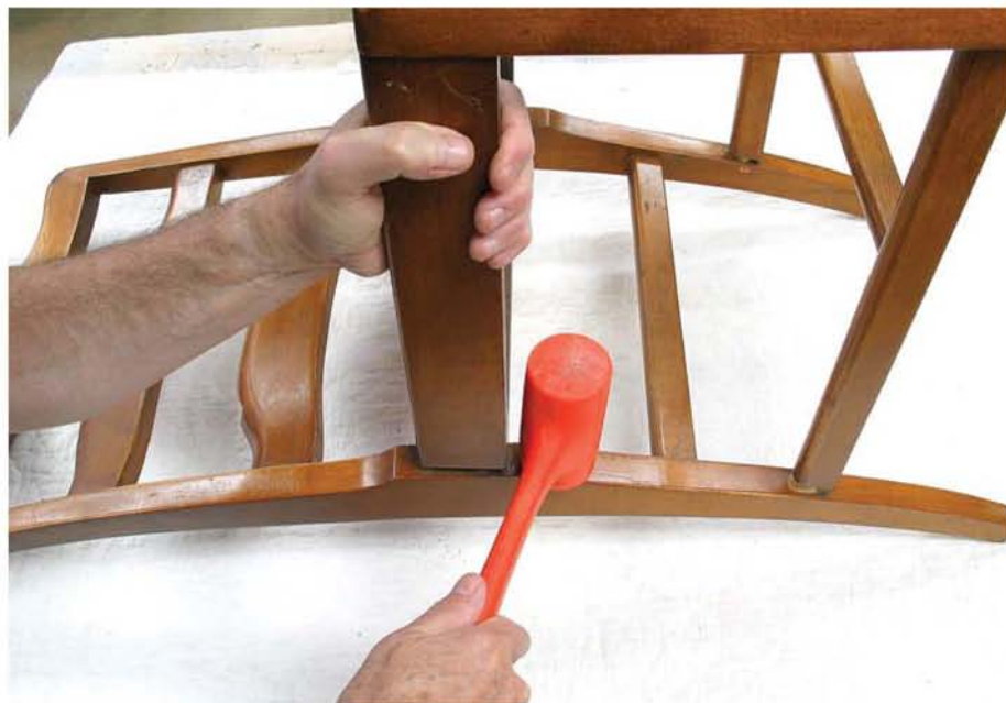
With all restraining devices removed, knock the chair apart. The most efficient tool to use is a deadblow hammer. Hold the parts a fraction of an inch above a soft surface and strike them as close to the joint as possible to avoid breaking or splitting something.
