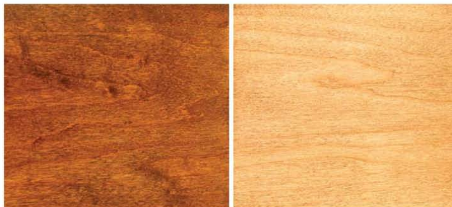
A dye stain is dye dissolved in a liquid. When applied to wood, the dye penetrates along with the liquid (left). An oil, varnish or water-based stain is dye and/or pigment in a solvent and binder. The binder limits the versatility of the stain, keeping most of the colorant on the surface of the wood. So the wood doesn't get as dark when you wipe off the excess stain (right).
