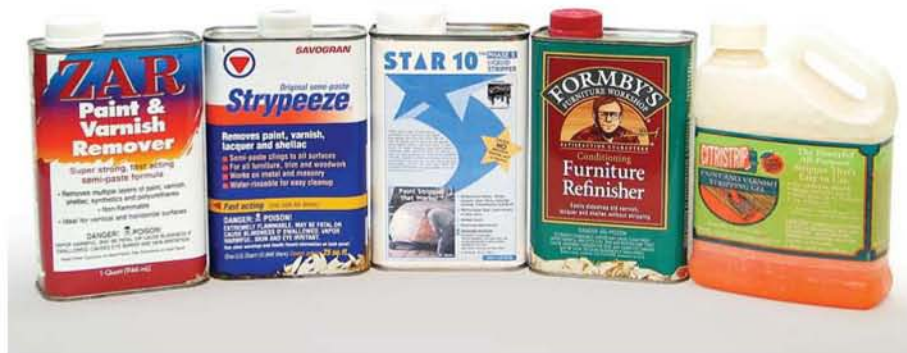
From the left, the four types of solvent strippers plus refinisher are methylene chloride (MC); a combination of methylene chloride and acetone, toluene and methanol (MC/ATM); acetone, toluene and methanol (ATM) with wax added to make it a stripper and ATM "refinisher" without wax; and n-methyl pyrrolidone (NMP).
