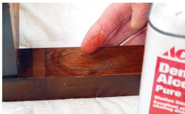
Here is the stripped tabletop after the residue solvent had dried out of the wood.
