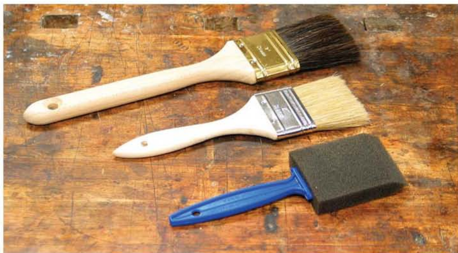
Brushes differ in their ability to keep their bristles from falling out, in the amount of finish they can carry and in their comfort to use. More expensive brushes, such as the oxhair brush (top) don't reduce brush marks noticeably over the very cheap chip brush (middle), or the foam brush (bottom). The finishes themselves differ in how well they flatten out.
