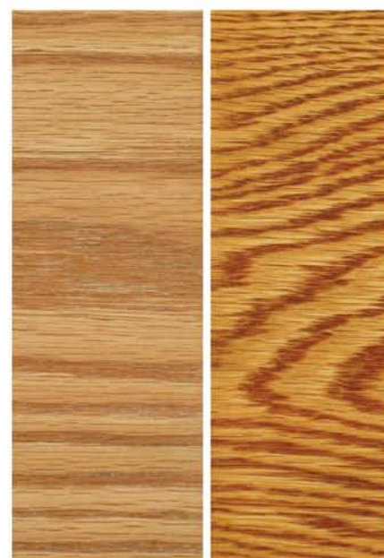
Boiled linseed oil (shown here on oak) and to a lesser extent varnish darken considerably as they age. On the left is freshly applied boiled linseed oil. On the right is boiled linseed oil that has aged about 10 years.
