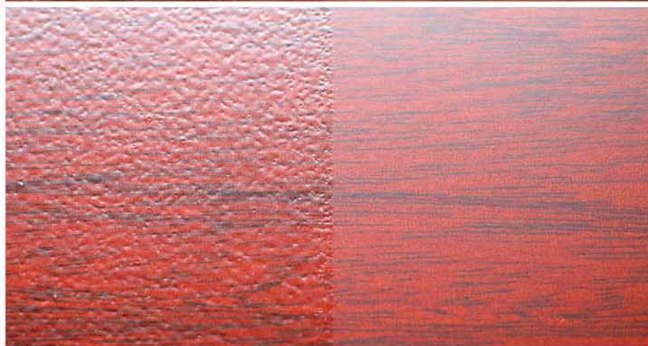
The thicker a finish during application, the less it flattens out and the more brush marks and orange peel show. On the left side of each of these panels, I applied the finish right out of the can – brushing varnish on the top panel and spraying lacquer on the bottom panel. On the right side of the panels I brushed and sprayed the same finishes thinned significantly with the appropriate thinner.
