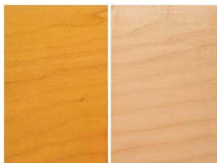
Water-based finish (right) maintains the natural color of maple while oil-based varnish "yellows" the maple considerably.
