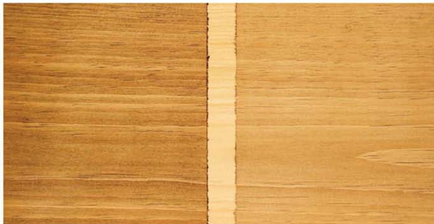
The color intensity of a stain is determined by the ratio of colorant to liquid. A full-strength commercial oil stain darkens wood more (left) than the same stain thinned 50 percent with mineral spirits (right).
