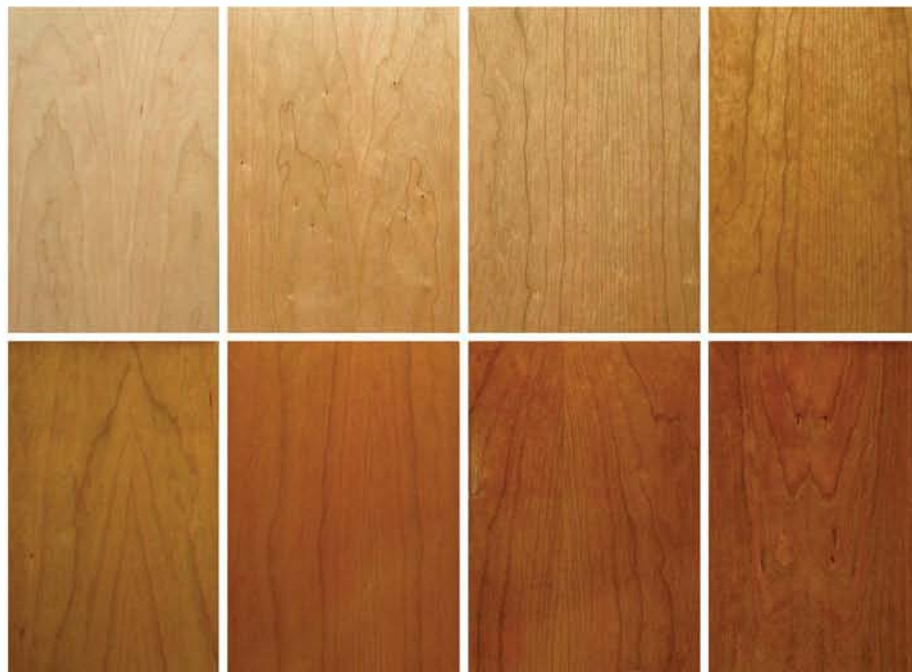
Seven finishes on cherry. Top row from left: unfinished, clear paste wax, water-based finish, nitrocellulose lacquer. Bottom row from left: clear/blonde shellac, amber/orange shellac, polyurethane varnish, boiled linseed oil.
