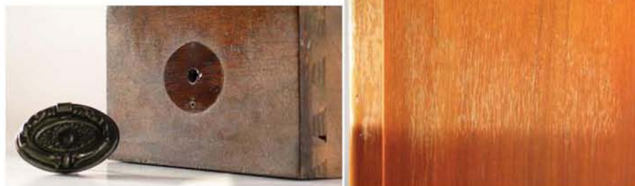
Light destroys finishes. Direct sunlight and fluorescent light are the most damaging. The 100-year-old drawer front on the left is badly crazed except where the finish was protected from light by the hardware. There, the finish is in near-perfect condition. The backside of the walnut cabinet on the right sat next to a west-facing window for 10 years. The finish is peeling and the color is faded where the sunlight hit.
