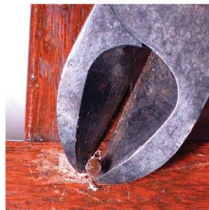
With enough wood removed so you can grab each nail with a pair of electrician's side-cutting pliers, pry them out of the wood. Fill the damage with wood putty if you are refinishing, or with a matching colored wax crayon after the chair has been reassembled if you aren't.
