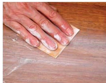
Sanding sealers contain a soap-like lubricant that causes the finish to powder so it doesn't clog the sandpaper. But sanding sealers don't seal the wood any better than the finish itself and, in fact, weaken water resistance and the bond of the finish.
