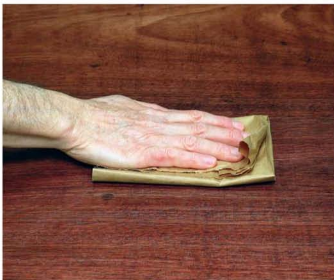
A folded brown-paper bag from the supermarket is fairly effective at leveling dust nibs so the finish feels smoother. As long as the finish is fully cured, the paper won't scratch it.
