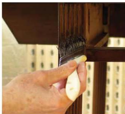
If you don't get your cloth wet enough with stain, you'll have trouble getting the stain into recesses. You can always use a brush to help do this.
