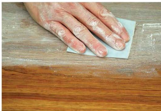
A varnish or lacquer sanding sealer has soap-like lubricants included, which make the finish powder when sanded. Sanding sealer reduces protection for the wood, however.
