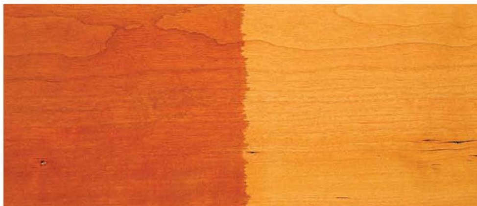
If you are using relatively non-blotchy wood or are willing to live with the blotching, you can achieve a color very close to aged cherry immediately by using a cherry dye stain (left). Lockwood "Natural Antique Cherry" water-soluble dye (also sold as Moser "Natural Antique Cherry") provides the most accurate coloring in my experience. These dyes are available by mail order from many suppliers. But keep in mind that the color of the wood under the dye will still darken and result in a much darker coloring than you may want after a number of years.
