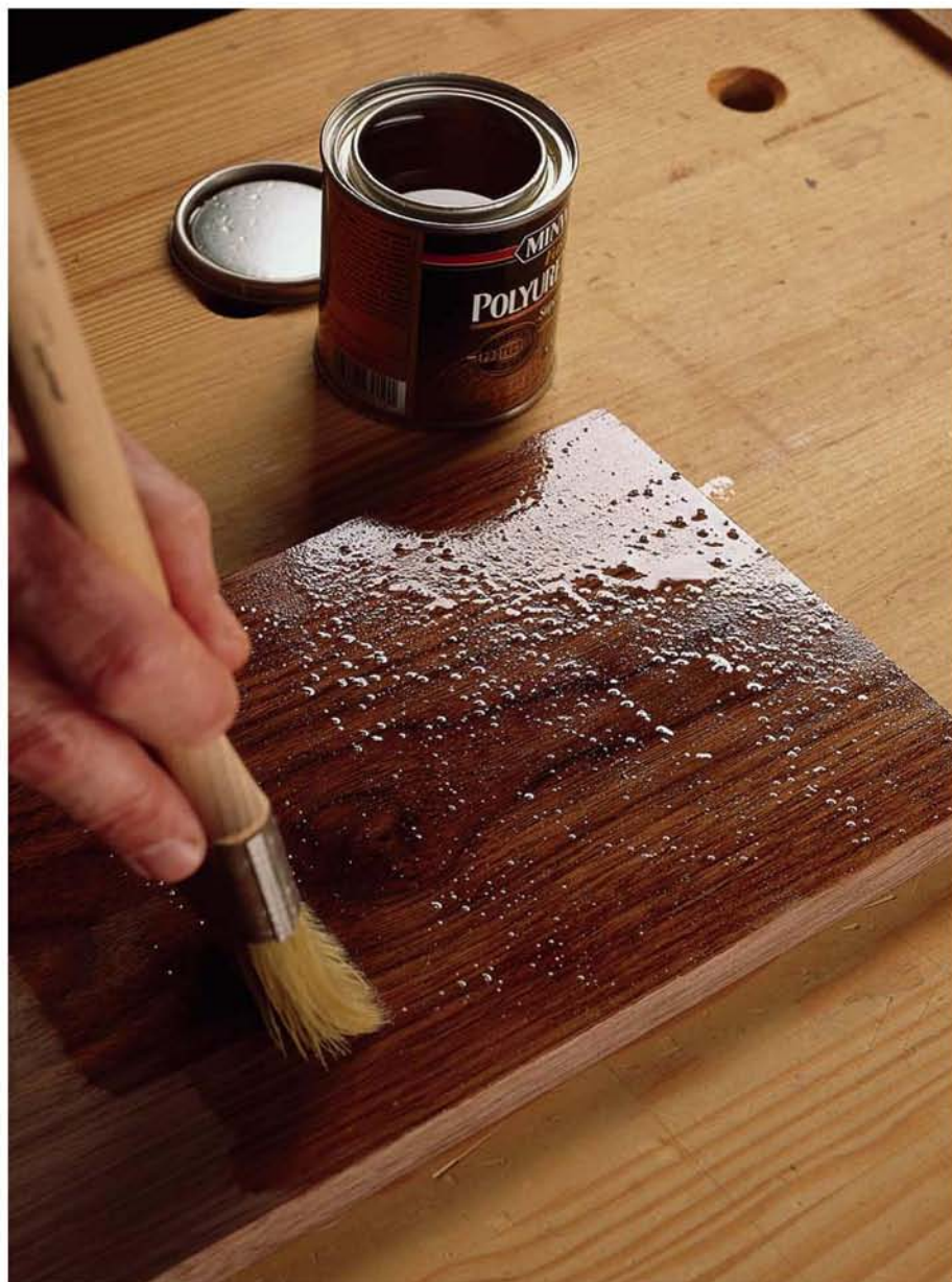
Myth 7: Bubbles in your finish aren't caused by shaking the can. They're the result of turbulence created as you move your brush. You can usually fix the problem by brushing back over the finish.
