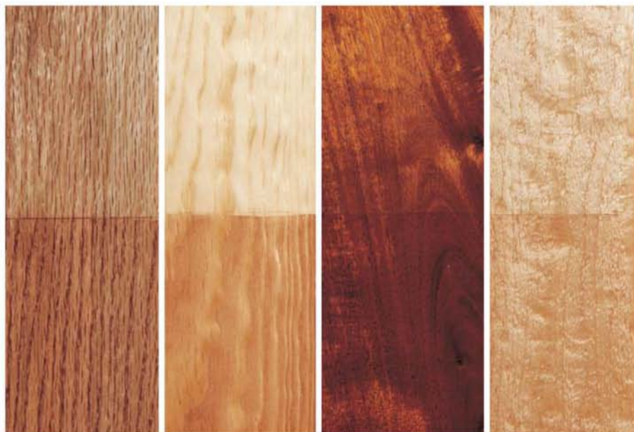
The same stain was applied to the lower side of each of these woods – from left to right: oak, pine, mahogany, maple. Yet each still looks like the wood it is. There are limitations in what you can accomplish in trying to make one wood look like another.
