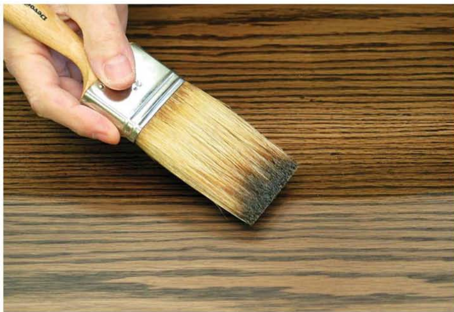
If your varnish brush is picking up some of the stain color as shown here, the most likely cause is cool temperatures in your shop. I let this oil stain dry 24 hours in a shop at about 55 F, clearly not long enough at this temperature.
