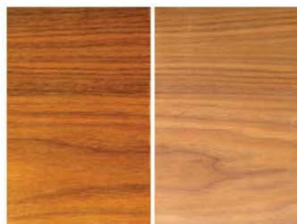
Water-based finish "washes out" the color of dark woods such as walnut (right) while oil-based varnish gives them a warm glow.
