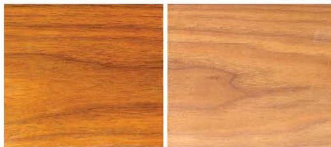
Varnish applied to the left side of this walnut board adds a warmer coloring than does water-based finish applied to the right side.
