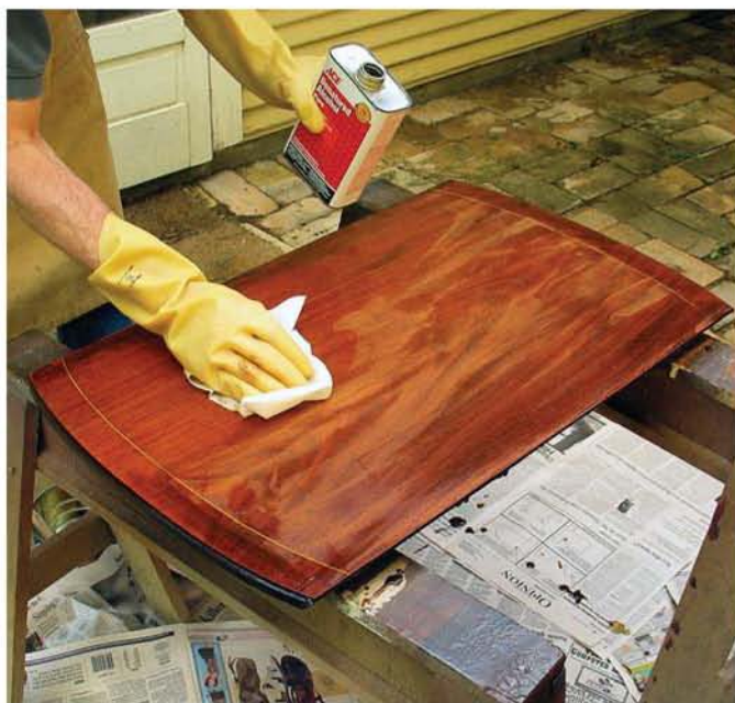
With all strippers except lye and NMP, wash the surface with a solvent to remove the wax residue. In this case the stripped finish was shellac, so I'm using denatured alcohol to aid in removing any remaining shellac.
