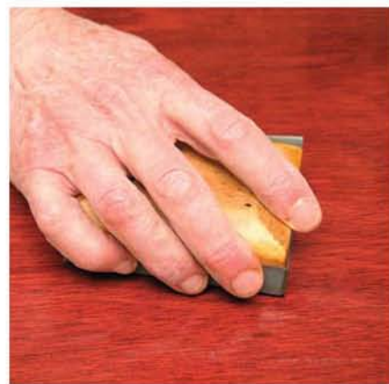
Myth 6b: The way to apply a brush-mark free finish using polyurethane is to first sand out the brush marks on the next-to-last coat using a flat backing block and a mineral oil, mineral-spirits or water lubricant. Then thin the last coat about 25 percent with mineral spirits so it levels well.
