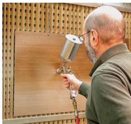
Because lacquer thinner is made up of individual solvents that evaporate at different rates, it's possible to spray relatively heavy coats of any finish thinned with lacquer thinner onto a vertical surface with no runs or sags. This is one reason finishers love spraying lacquer.
