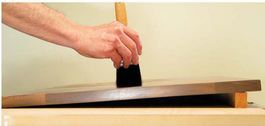
Myth 6a: Slanting a panel 5° or 10° is not the way to reduce brush marking, but this has actually been suggested recently. You would have thought furniture finishers working during the last several hundred years would have figured this out if it were true.
