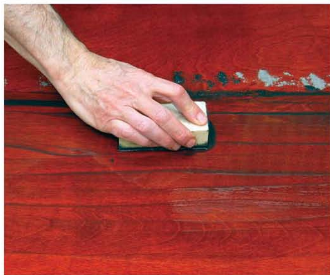
To achieve a soft-appearing gloss on a leveled surface, first sand up to about #2,000 grit, then rub with rottenstone and a mineral-oil or mineral-spirits lubricant. Use a felt or sponge pad.
