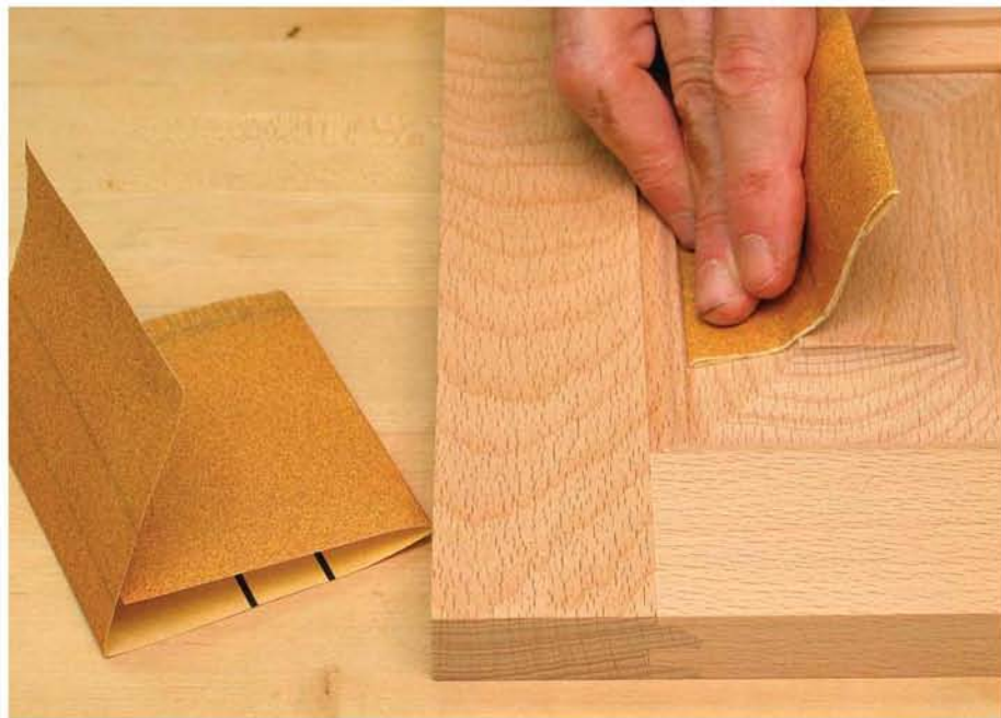
The most efficient use of sandpaper when backing it with just your hand is to tear the sheet into thirds crossways and then fold one of the thirds into thirds lengthways. Flip the thirds to use 100 percent of the paper.
