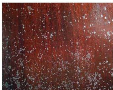
Mildew spores can be killed (to stop further growth) by washing the surface with half-and-half household bleach and water. Dry the surface quickly so the water doesn't damage the finish.
