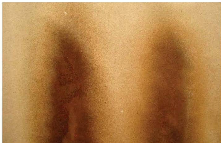
The biggest difference between inexpensive and expensive spray guns is the quality of atomization they produce. The finer the atomization of the liquid material, the more level the surface produced—that is, the more reduced the orange peel. The spray pattern on the left (made by an inexpensive spray gun) has a much poorer atomization than the spray pattern on the right, which was made by an expensive spray gun. This is evident from the much larger dots around the edges of the pattern on the left.
