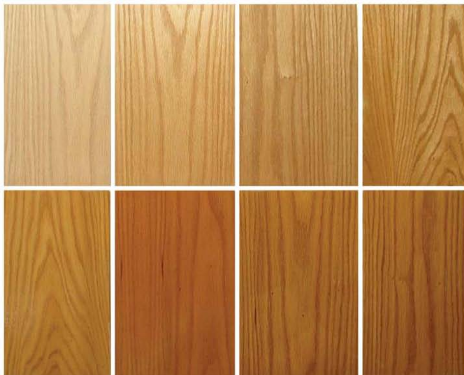
Seven finishes on oak. Top row from left: unfinished, clear paste wax, water-based finish, nitrocellulose lacquer. Bottom row from left: clear/blonde shellac, amber/orange shellac, polyurethane varnish, boiled linseed oil.
