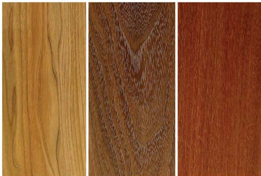
Three common examples of medium-grained woods used in woodworking are from the left: butternut, walnut and mahogany. These woods are widely considered the most elegant when their pores are filled. All stains and finishes can be used successfully.
