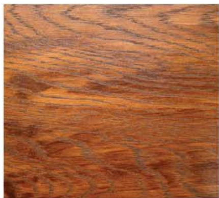
Lacquer, water-based stains and dye stains dry rapidly. So they could lead to this type of blotching if some of the stain dries before you have time to get it all wiped off.
