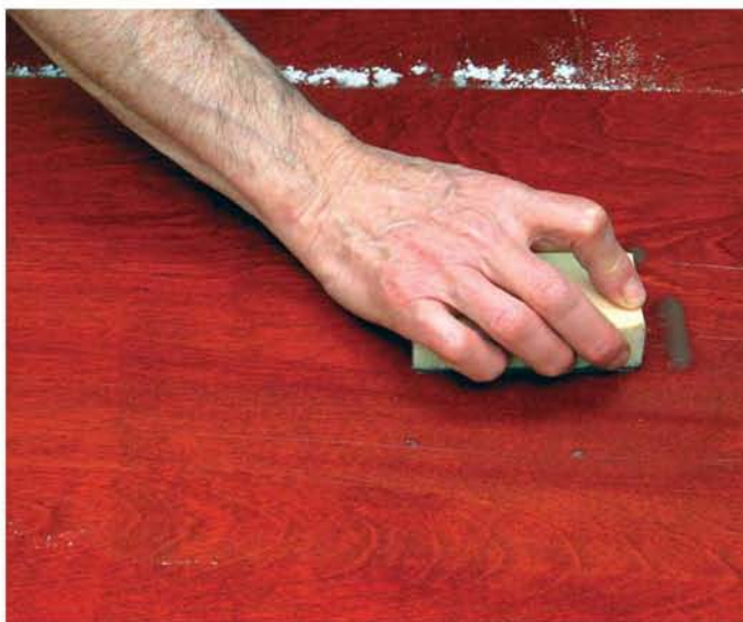
You can create an even satin sheen on a leveled surface by rubbing it with pumice and a mineral-oil or mineral-spirits lubricant. Use a felt or sponge pad.
