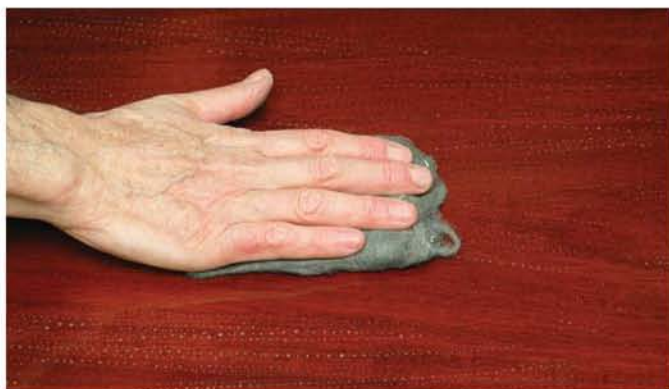
Instead of using steel wool dry, wet the surface with soap and water or mineral oil and then rub. Rubbing wet produces better results, but you run the risk of rubbing through and not seeing it happen. You will make the rub-through much worse.
