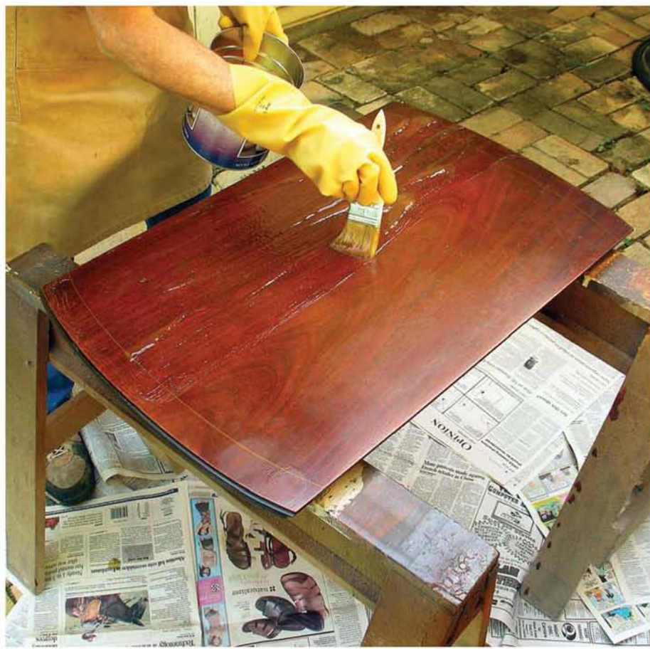
Working outside in the shade or inside with cross-ventilation, spread the stripper thickly onto the surface using an old or inexpensive brush.
