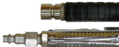
Quick-connect air inlets differ for compressor- and turbine-supplied spray guns. The air inlet on top is for turbine air; the one on the bottom is for compressed air.
