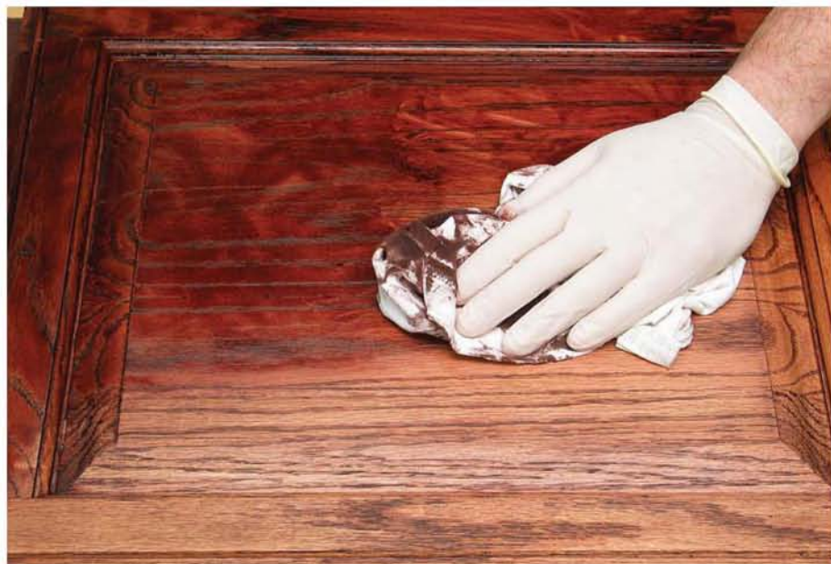
As long as you wipe off excess stain, the coloring will always be even unless the wood is naturally blotchy or, as with this oak, the grain is highlighted.
