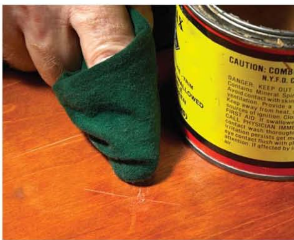
If a liquid makes the scratch too dark, apply some clear paste wax.
