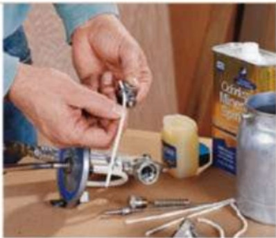
Break down your gun by removing the air cap, fluid tip and needle. Soak them in solvent until they are clean.
