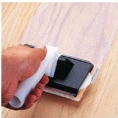
Over-applying is one of the top problems with water-based finishes. To prevent this, use a foam paint pad, as shown above.
