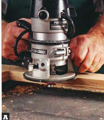
A Rout the rabbeted panel and glass openings in the doors in three passes for accurate, chip-free results.
