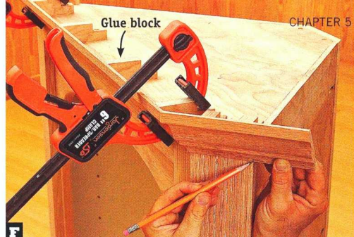
F With the front molding dry-clamped, hold your side moldings in place and mark flush with the cabinet back.
