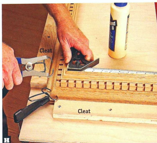
H Assemble the moldings with PVA glue, holding the miters tight and square with spring clamps at the outside corners.
