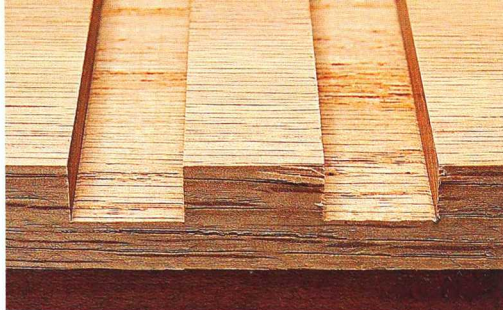
These \frac{3}{4} " dados were cut in red oak with a scrap board to back up the cut (left) and then without (right). The backer board eliminates tear-out.
