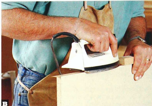
B All you need to apply veneer is an inexpensive household iron. If you plan to do a lot of cabinetwork, you can buy veneer tape in 250' rolls.
