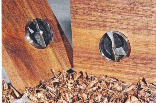
A multispur bit (left, with the toothed rim) or a Forstner bit (right, with the smooth rim) bores a large hole easily.
