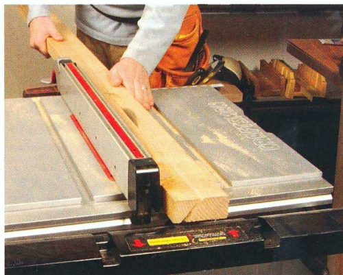
Rip a bevel on the backer. Set the blade to cut a 38-degree bevel—the angle of the back of the molding when in place.
