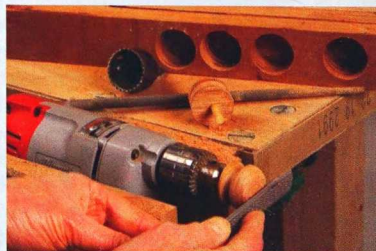
To make a wooden knob, cut a plug with a hole saw and glue a dowel into a hole in the back. Chuck it in your drill and shape it with wood files.
