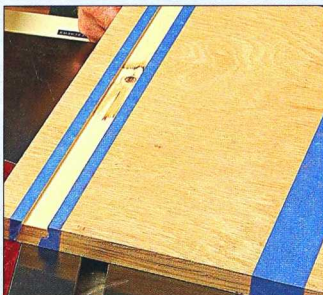
Score \frac{1}{16} " deep to cleanly shear the veneer, then cut the channel to depth.
