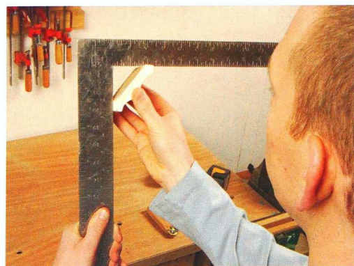
Use a scrap and a framing square to measure the height and width of the space behind the molding.
