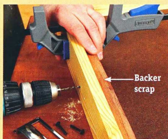
Scrap clamped to the inside of this drawer front prevents tear-out on the back surface.
