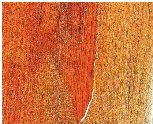
Polyurethane's slow drying time can cause sags. An angled light source reveals excess finish you'll need to brush off.
