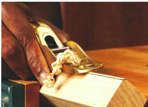
Draw layout lines to define the limits of the chamfer on a table leg. As you plane adjust the angle of the tool on the table leg as needed to meet the lines.
