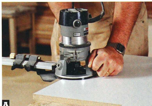
A Equip your router with a good edge guide before you start making grooves for cabinet backs. Set the guide and then do all the backs at once.
