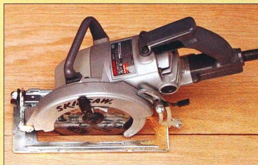
The long, narrow worm-drive saw runs about 20 percent slower than other circular saws but has more power.
