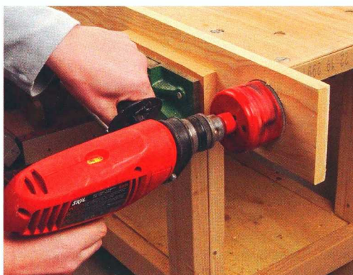
A hole saw is a great way to cut a large, neat round hole, but it can bind unexpectedly. Grip tightly or, better yet, attach an extra handle to your drill as shown.
