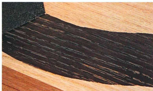
Ebony dye lays the groundwork for a dark finish, but it doesn't fill oak's deep pores. For that you need a stain with pigment particles.
