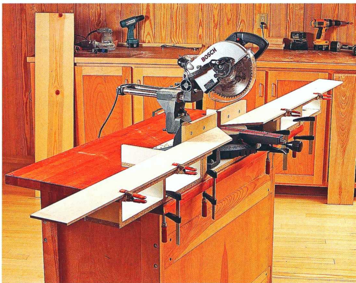
Supporting your molding using an auxiliary fence and extension table, made from plywood or MDF, eliminates tipping of long moldings and enables you to produce accurate cuts.
