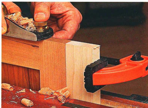
When planing end grain attach a piece of scrap wood to prevent blowing out the grain as the blade exits the workpiece. The scrap tears out instead of your project.
