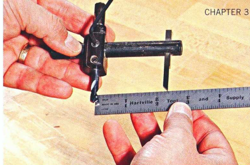
You can set the circle cutter to make any size hole. Measure the radius of the hole (half the diameter) from the center of the pilot bit to the outside of the blade.
