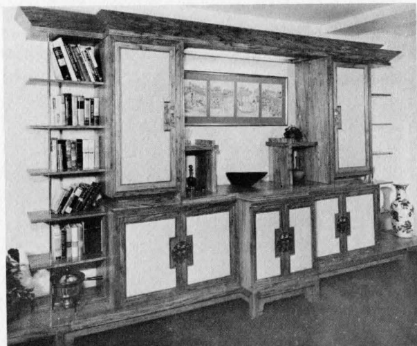
The wood of this breakfront is wormy chestnut. Frank and his men applied a coat of clear lacquer to the wood, then painted it with thinned-down asphaltum paint to darken the pores. The wood was then cleaned off, and a second coat of lacquer applied.
