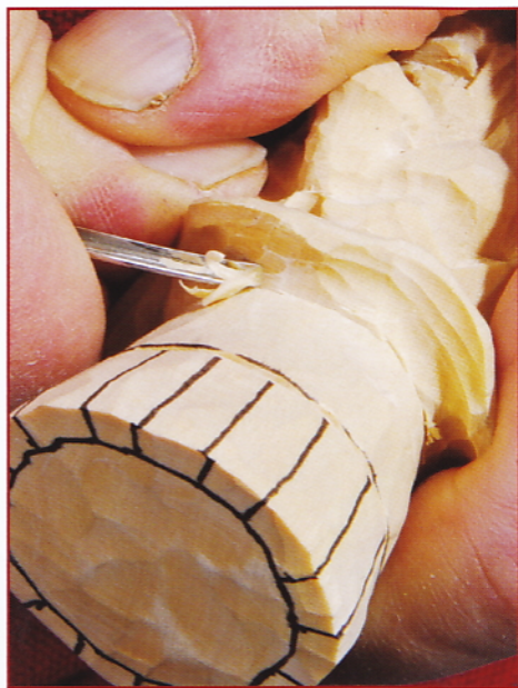
Go around the bottom of the hat band with the same tool, following the natural line of the brim.
