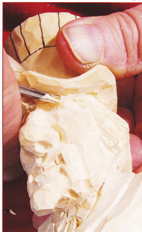
Undercut the eyebrow with a small gouge.
