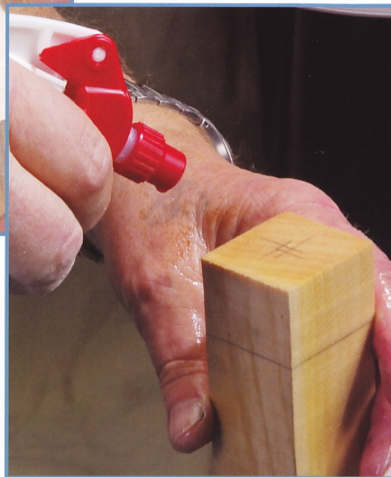
Spraying the block with a 50-50 mixture of rubbing alcohol and water makes it easier to carve.
