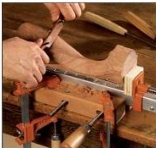
The contours of a cabriole leg are shaped with a spokeshave. The leg is held in a bar clamp, which is secured to the work surface by a hand screw and two quick-action clamps. This setup exposes the entire front surface of the leg for shaping.
