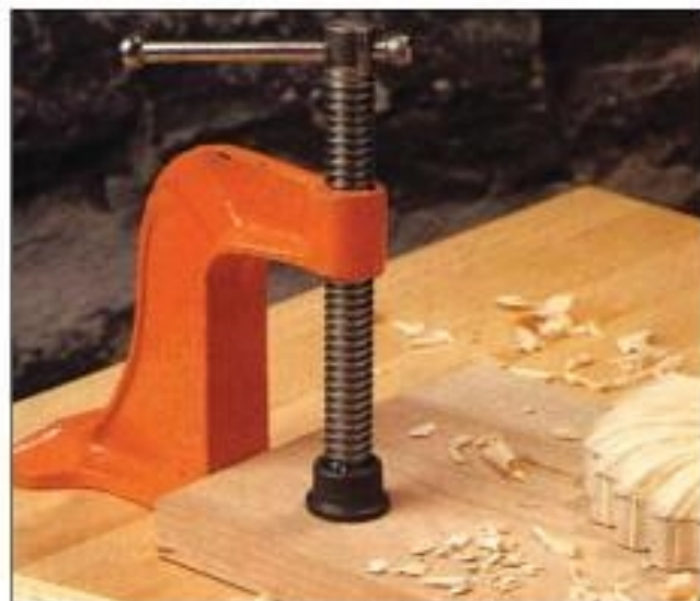
This hold-down clamp fits into a workbench recess originally intended for a bench dog.
