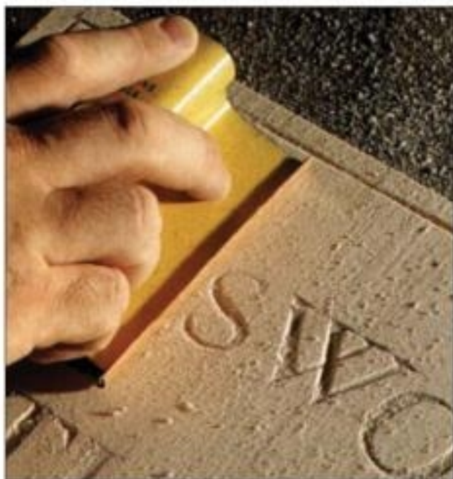
A sanding block is used to remove any splinters and pencil or carbon paper marks around the letters in a sign. Using a block will keep the letter edges crisp. Holding the sandpaper in your hand will tend to round over the edges.
