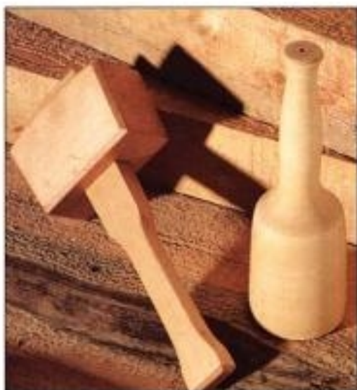
Wooden mallets are classic elements of the carver's tool box. The flat-faced carpenter's mallet (above, left) has its face angled relative to the handle, making it easier to control. The cylindrical carver's mallet (above, right) will not slip, since it strikes on one narrow spot only, due to its oval face.
