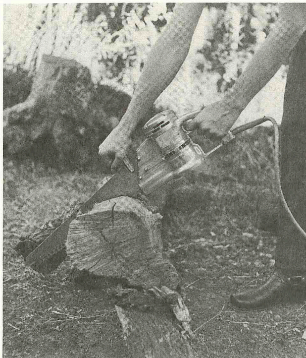
RECIPROCATING HANDSAW does fast, efficient rough cutting of green logs into shapes for seasoning, carving.
