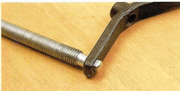
Fig 4.39 A square hole in the fly engages a spigot on the end of the screw in order to tighten it into the workpiece
