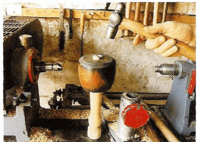
Fig 1.26 Driving the wedge home. It may be an idea to leave the mallet for a while in case the handle shrinks; then tap the wedge finally home, trimming it off so the mallet sits upright on the bench
