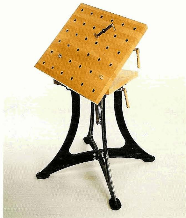
Fig 4.14 The adjustable woodcarver's bench by Veritas. Work is held by a combination of 'Pup' screw clamps (available separately) and metal bench dogs, which can be positioned in any of the drilled holes as required
