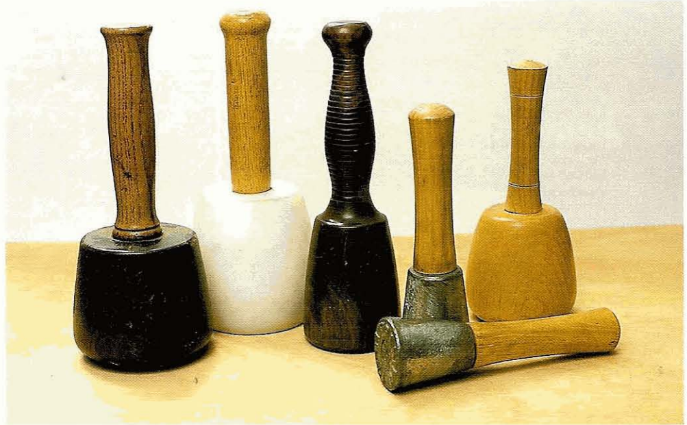
Fig 1.5 A collection of carving mallets. Left to right: lignum vitae , nylon, lignum vitae , annealed iron (two examples), beech
