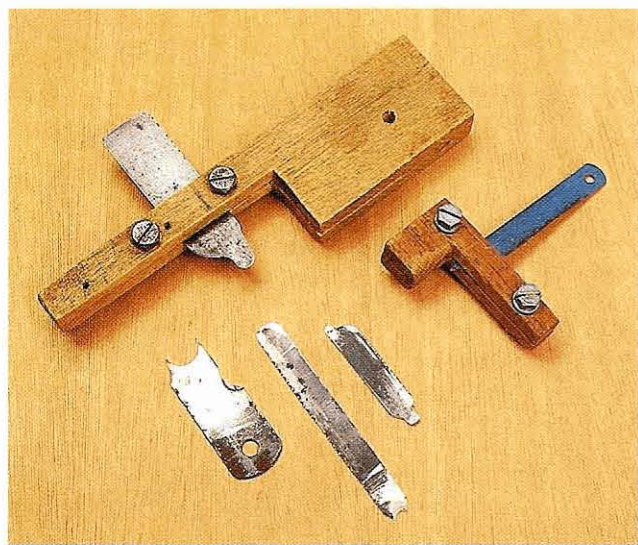
Fig 1.71 Scratch stocks are quickly made and can produce a wide range of moulded edges; any number of interchangeable blades can be made for them
