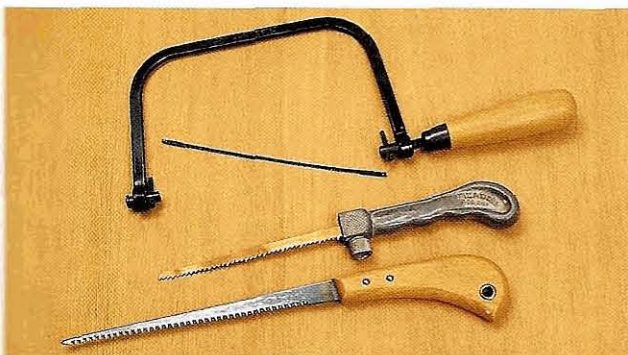
Fig 1.49 Two versions of the keyhole saw; the bottom one is Japanese and cuts on the pull stroke. Above is the coping saw with blade detached
