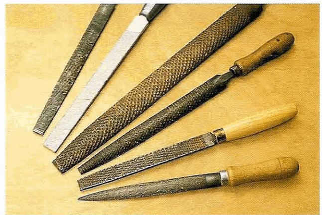
Fig 1.31 A selection of rasps: the largest is 2in (50mm) wide. The two on the left are intended for use on plastics, but are also effective on wood
