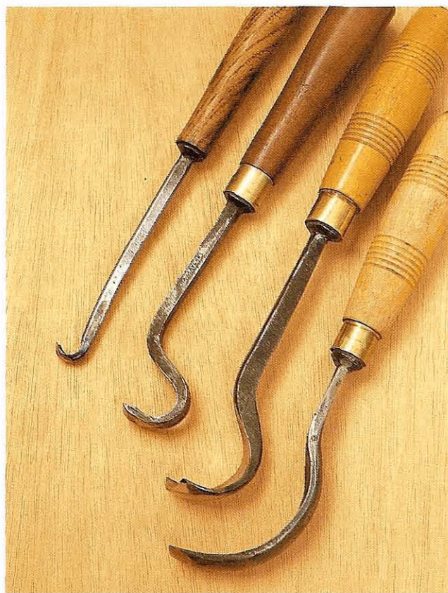
Fig 3.6 All these tools were bent from the original shape for a particular purpose, using the basic techniques discussed in this chapter; in each case the original sweep is retained
