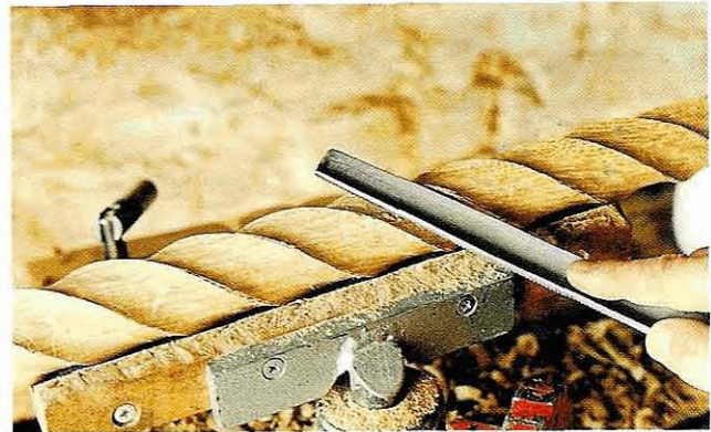
Fig 1.43 Winding the rasp through its cut is essential to achieve the smooth, unspoilt lines appropriate to this type of work. This rasp is one sold for car bodywork, and gives a very clean cut on wood
