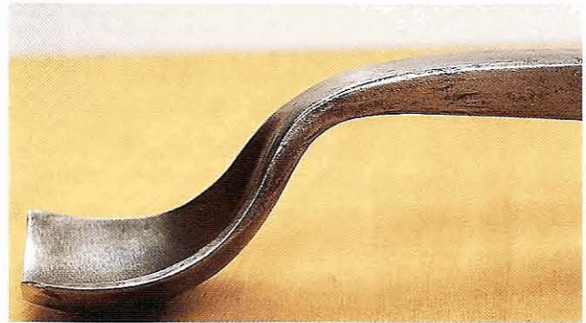
Fig 3.24 Detail of the crank in the home-made shortbent gouge shown in Fig 3.2
