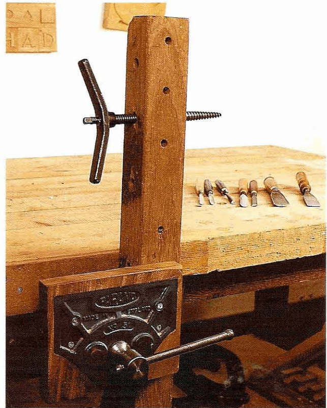
Fig 4.43 A screw post, or board, held in a vice allows work to be held vertically
