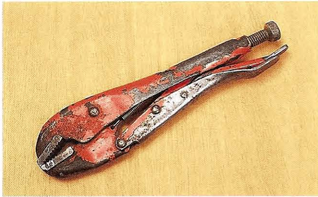
Fig 3.23 Mole (locking) grips lock securely on to the tool on which you are working
