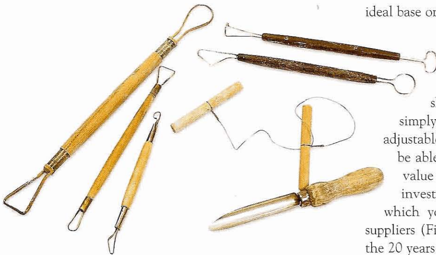
Fig 8.14 Tools for cutting and removing clay include a fine wire with handles each end, stout wire loops in wooden handles, and a half-round tool for making holes
