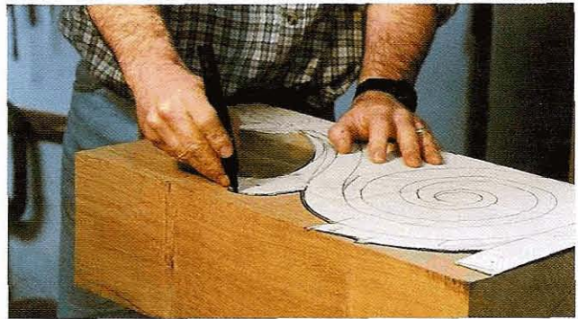
Fig 2.2 Using a template to draw an outline on the initial block of wood
