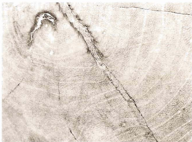
Fig 6.36 Larger cracks filled with wedges. Even though the wood was carefully matched some 10 years previously, colour changes have made them more obvious; nevertheless they help the feel of the work when it is touched
