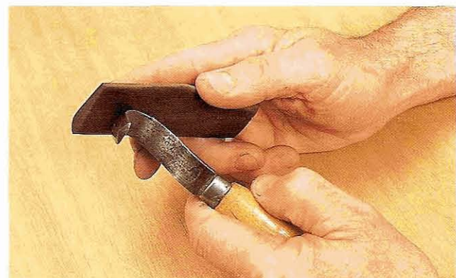
Fig 1.63 A hook knife can be similarly sharpened with round and flat slipstones
