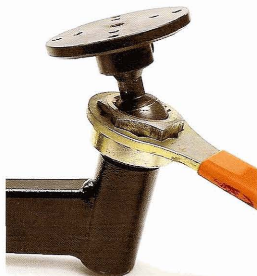
Fig 4.46 The Stretton Carver's Clamp, with its integral spanner for adjustment
