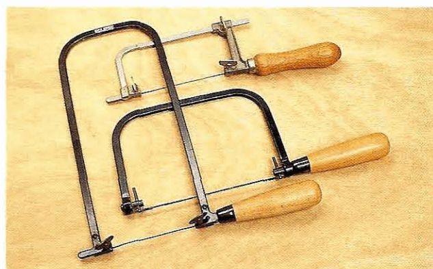
Fig 1.48 Saws for curved work, all with detachable blades that will insert through holes pierced in a carving. The one with the deepest frame is the fretsaw; the smallest (the piercing saw) takes a thin fretsaw blade; the coping saw in the middle is the most useful one to have handy
