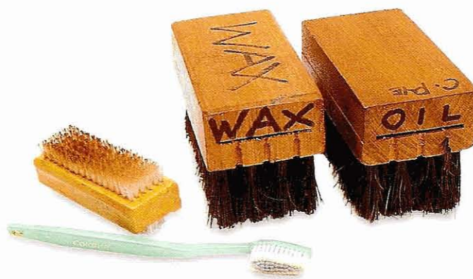
Fig 7.13 It is a good idea to keep separate brushes for polishing oil or wax finishes. Keep another brush entirely for brushing bare wood
