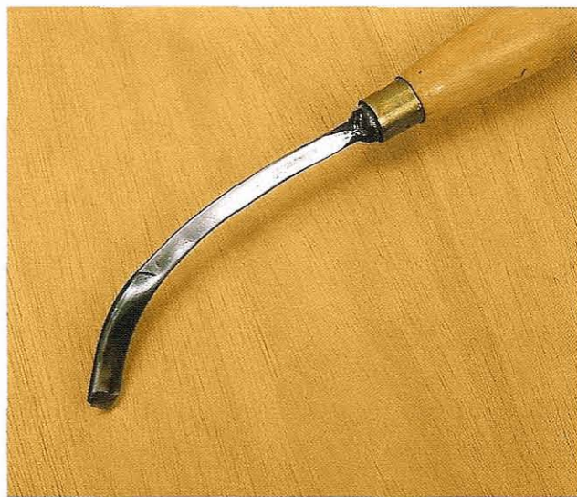
Fig 3.37 A backbent V-tool made for a particular purpose
