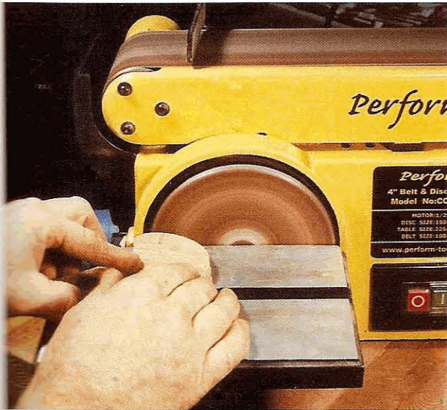
Fig 2.9 A typical small disc and belt sander. Only the left side of the disc is available for use, so that the direction of rotation keeps the workpiece on the table
