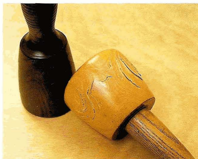
Fig 1.16 A mallet made from lignum heartwood (left) is far more durable than one made from a branch, which is mainly sapwood. Almost all commercial lignum mallets are of the second type
