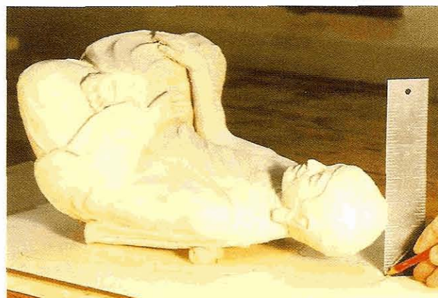
Fig 8.24 Using a try square to take a profile of the clay model for the carving in Fig 8.10. The time taken up in making the model is justified by the ease with which the wood dimensions and the placing of the joints can be calculated, which allows accurate bandsawing
