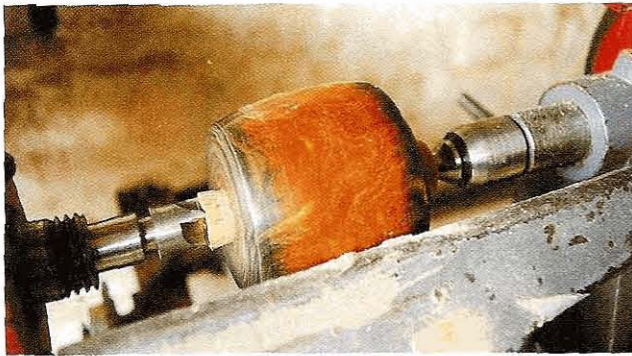
Fig 1.23 The final shape of the mallet head: bellied and slightly tapering
