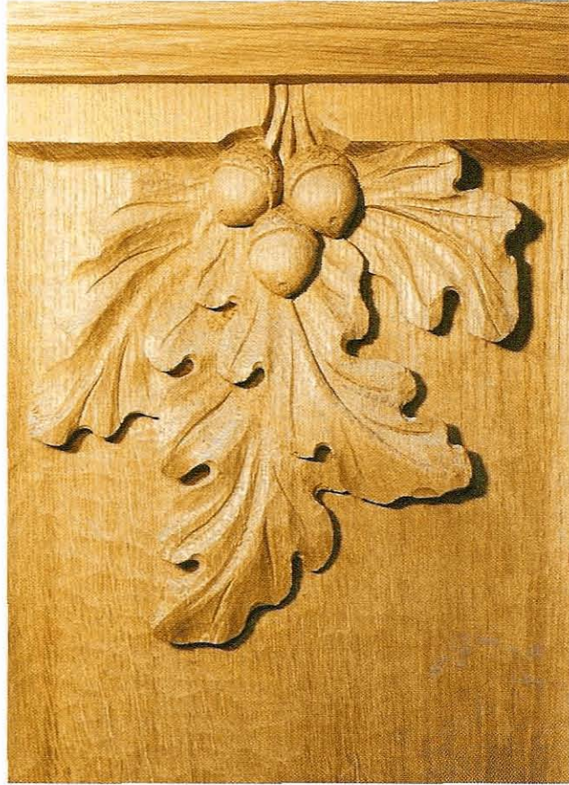
Fig 2.13 This carving was initially routed like the previous one, then the background was given a hand-tooled finish. The work of the router is completely subsumed
