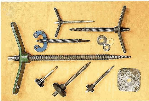
Fig 4.38 A collection of carvers' screws. Top: small and large Stubai screws; Marples screw; washers (not supplied with these models). Centre: custom-made long carver's screw. Below: Veritas screw; large and small Axminster screws; large square washer
