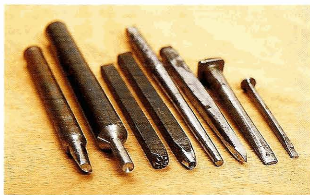
Fig 1.66 A close-up of the working ends of a variety of punches, including an oval eye punch, circular punches, two acanthus-eye punches (far right) and a floret
