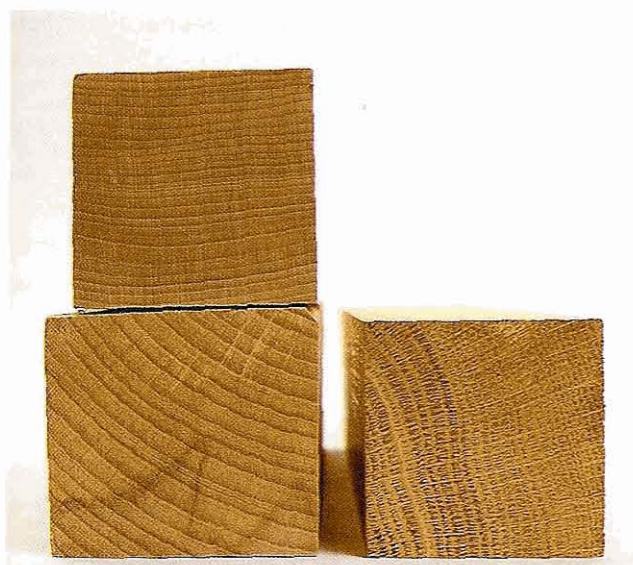
Fig 6.15 Cross sections of beech (left) and oak. Wider annual rings in the same species indicate faster growth and softer timber
