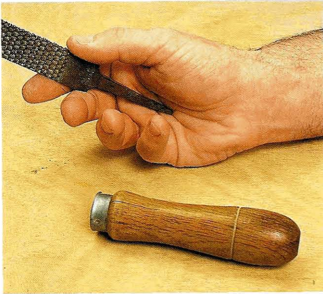
Fig 1.40 The tang of a rasp or file can be uncomfortably sharp to the palm; fit a simple handle for protection
