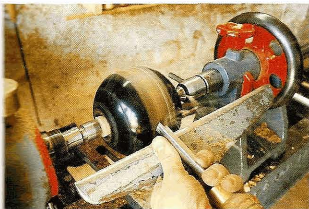
Fig 1.19 With the central hole plugged, the preliminary shaping of the mallet can be started
