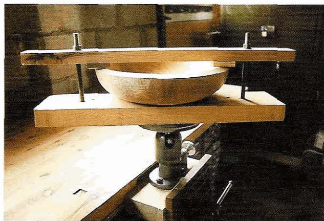
Fig 4.48 A simple way of holding a bowl in order to carve lettering on the rim
