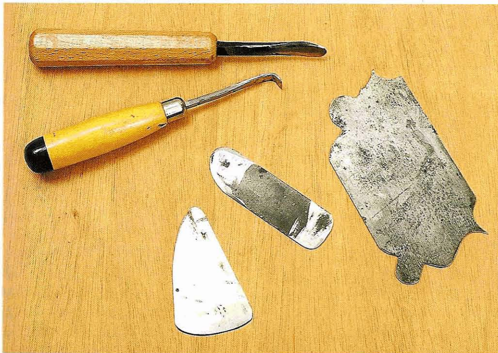
Fig 1.73 Sharpening a scraper involves burring over the edge (ticketing) – you can use the side of a chisel for this. This edge, if sharpened correctly, will remove a proper shaving and so must cut, rather than scrape
