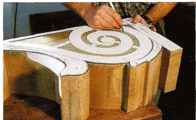
Fig 2.4 Back to the template to mark in the volutes. Provided the bandsaw was set up accurately, you can be sure the outline will fit on both sides exactly
