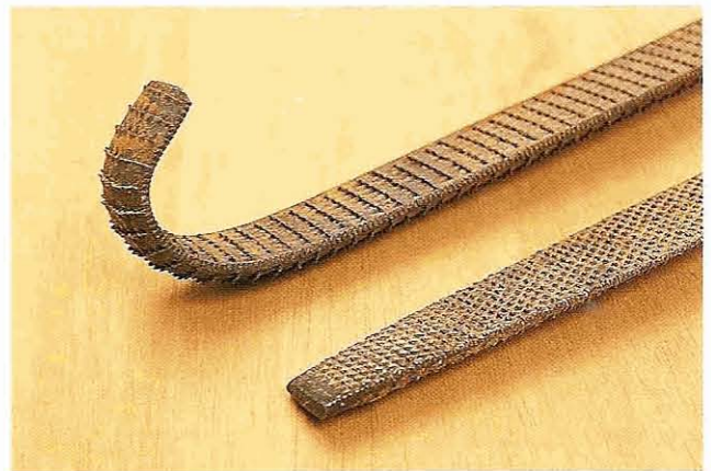
Fig 3.11 Even rasps and files can be reshaped successfully, though their tempering makes them harder, more brittle, than carving tools
