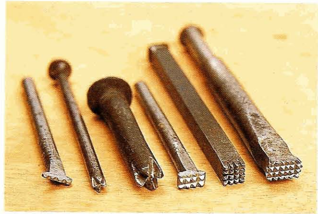
Fig 1.68 Different sizes of frosters are needed to work in different corners or shapes of the background
