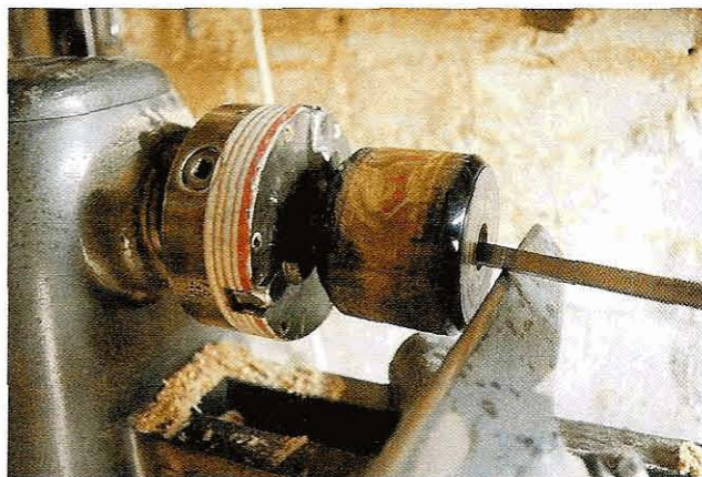
Fig 1.21 Reaming the hole to accommodate the wedge-splayed end of the handle
