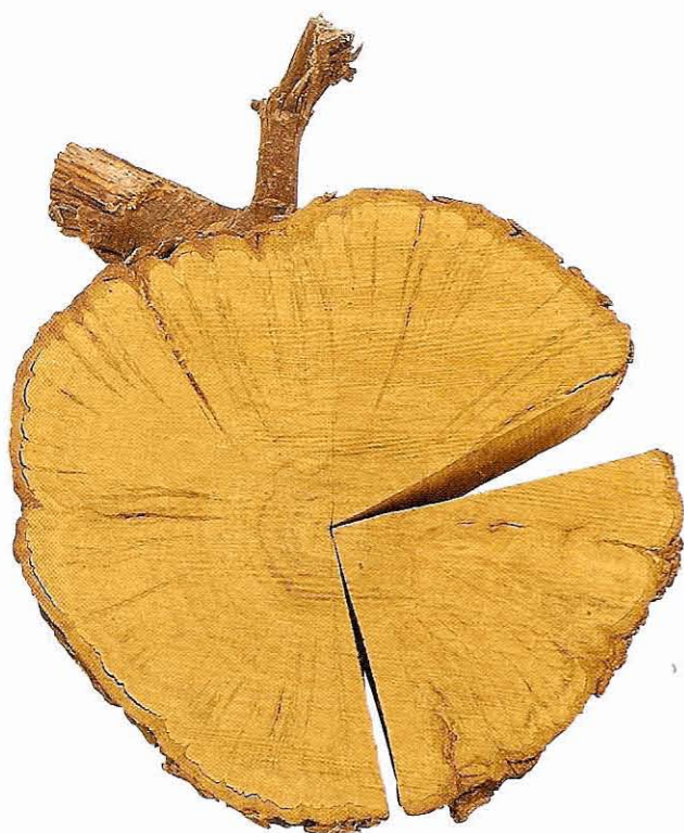
Fig 6.22 The wide gap shows how much the log has shrunk around its circumference since the segment was cut out of it. If it had not been cut, it would have split
