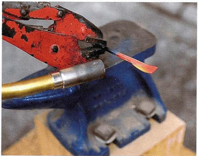
Fig 3.35 Heat to an adequate temperature the part of the blade which is to be bent
