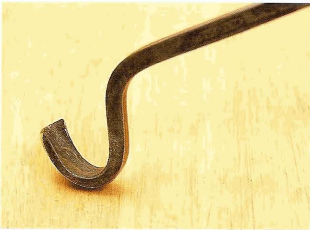
Fig 3.34 A knuckle gouge like this may enter a recess and remove wood by cutting with the grain for a clean finish, where other gouges would be cutting against it
