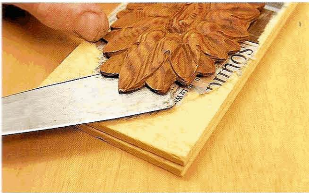
Fig 4.31 A spatula releases a finished patera by slitting the newspaper to which it is glued
