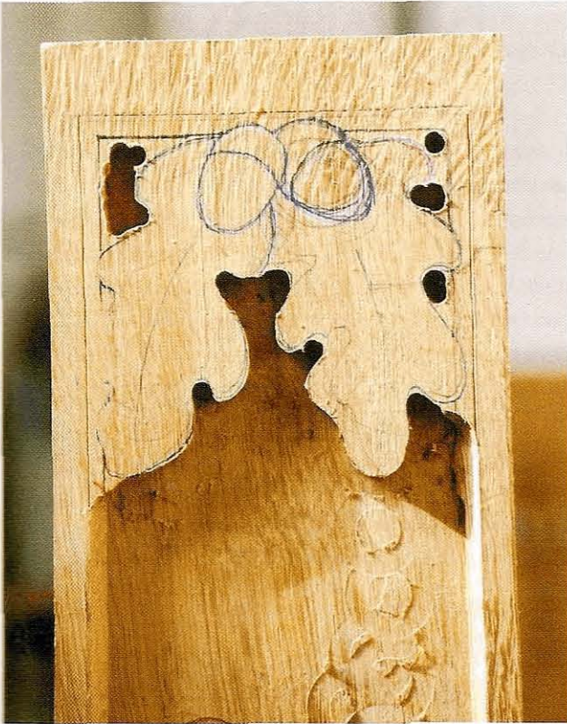
Fig 2.12 This oak-leaf panel has been routed by a mixture of plunging and wasting, which saves a lot of time in the initial stages
