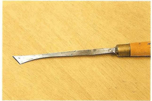
Fig 3.29 The skewed fishtail chisel: another tool useful for getting into tight corners
