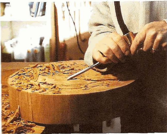
Fig 2.25 The Bordet power chisel can be held in much the same way as a normal gouge. The cuts it takes are light but smooth and easy, so, although it removes less at each stroke than a large gouge and mallet, you could carry on for much longer
