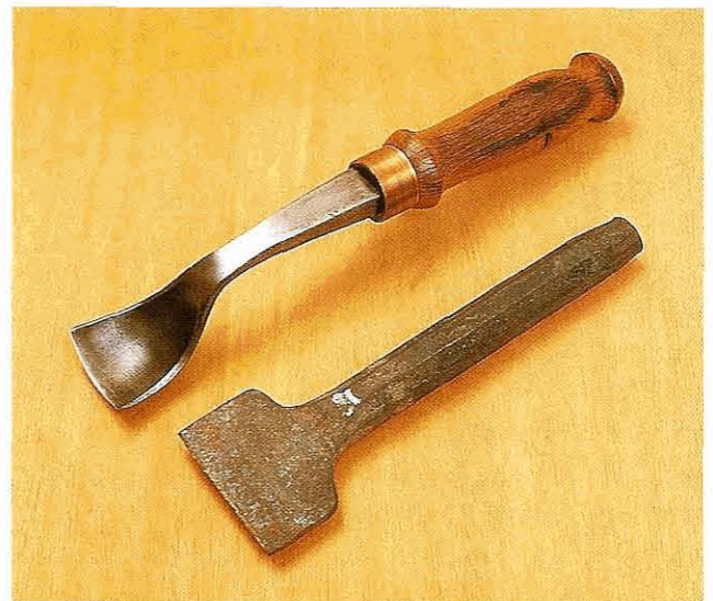
Fig 3.2 This large frontbent gouge was made from a boatbuilder's caulking chisel (similar to the bolster in the foreground) using a blacksmith's forge. Smaller shaping work is possible with a much leaner set-up
