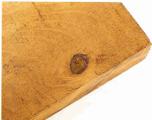
Fig 6.38 A typical dead knot
