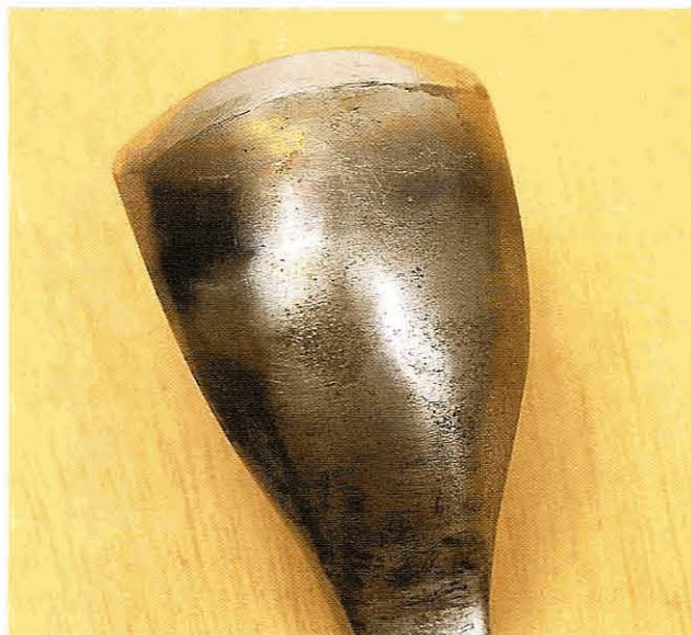
Fig 3.14 Polishing the surface of the tool before heating means that the tempering colours can easily be seen; they will remain visible unless removed by subsequent polishing
