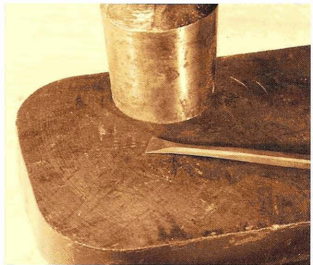
Fig 3.25 In the absence of swage blocks, a simple fishtail shape can be forged by hammering the hot end on an anvil. The shape can then be further refined over a round bar, filed and shaped
