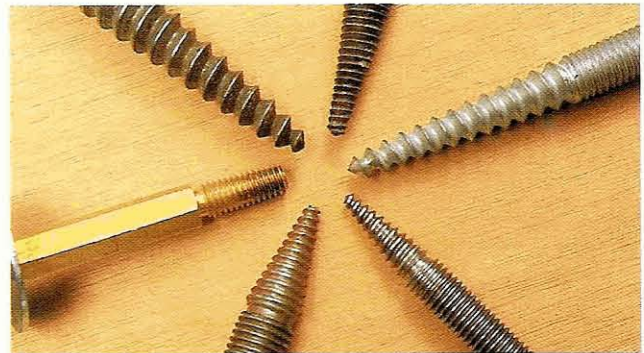
Fig 4.40 The working ends of carvers' screws differ in taper and thread according to what the manufacturer thinks will give the best grip
