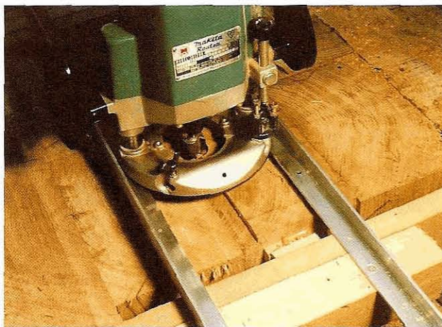
Fig 2.11 Router planing is easy: use parallel side tracks on either side of the block you wish to dress, and a simple carriage to take the router. The router sweeps across the wood, and the carriage is advanced a little for each cut
