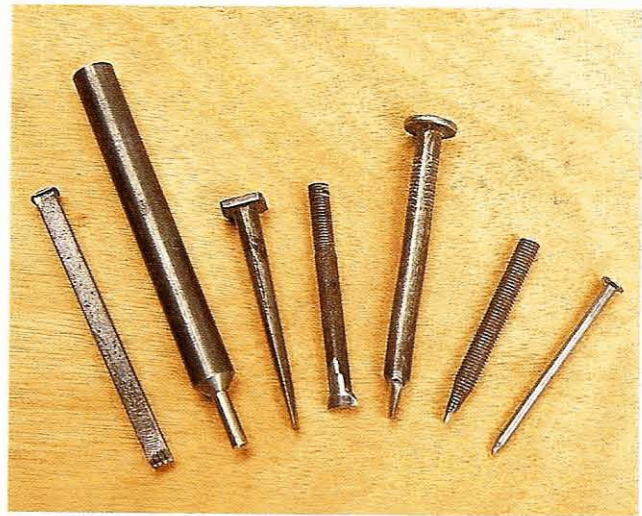
Fig 1.69 Frosting tools and many other punches can be home-made from nails or bolts
