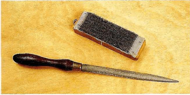
Fig 1.44 Regular use of a wire brush, and the smaller file card, will unclog the teeth of abrasive tools
