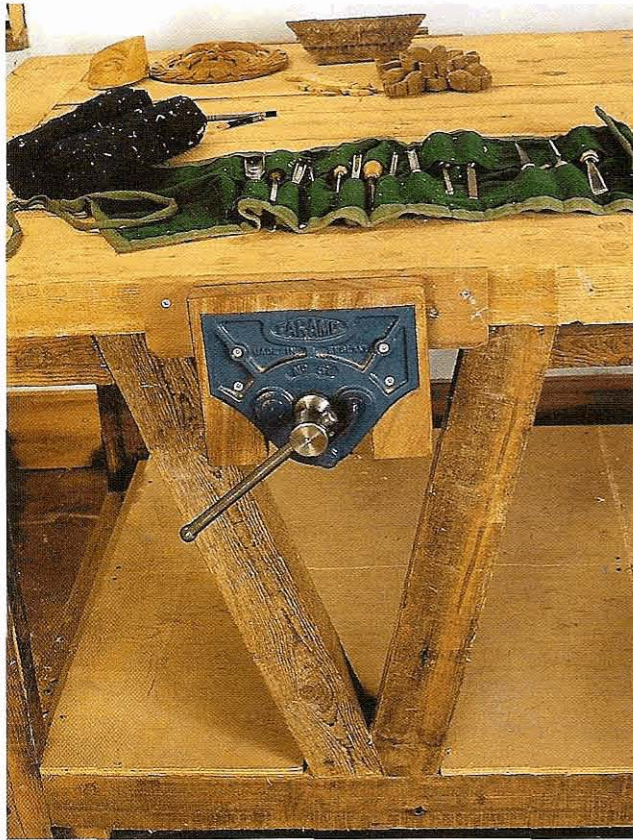
Fig 4.7 An ordinary woodworking vice has its uses for the carver; note the strong diagonal bracing beneath to ensure rigidity
