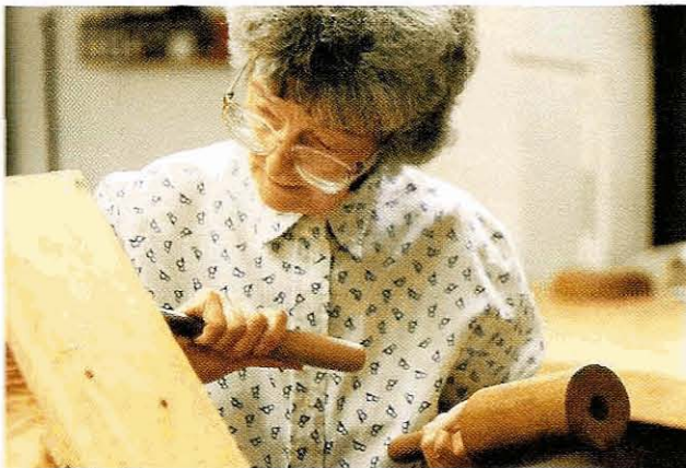
Fig 1.27 A good posture for using the mallet: the body to one side and the shoulder being used, rather than just the forearm and wrist
