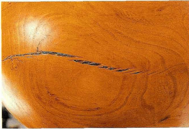
Fig 6.28 A particular pattern of shakes might be considered an interesting feature of some sculptures, rather than a 'fault' to be avoided.
