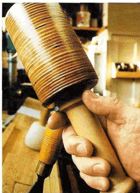
Fig 1.15 A Lignostone mallet, made from compressed beech veneers. This one has a ridge on the handle which might well cause soreness if used for an extensive period; rounding it over would be a major improvement
