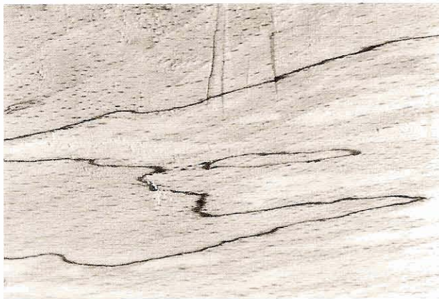
Fig 6.43 Spalted beech. Spalting usually reaches irregularly through the whole length of the piece of wood
