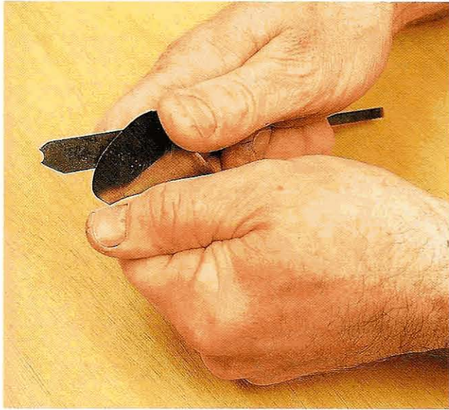
Fig 1.73 Sharpening a scraper involves burring over the edge (ticketing) – you can use the side of a chisel for this. This edge, if sharpened correctly, will remove a proper shaving and so must cut, rather than scrape
