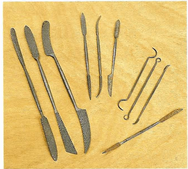
Fig 1.37 Rifflers come in a great variety of shapes and sizes. The right-hand one has a coating of tungsten carbide particles
