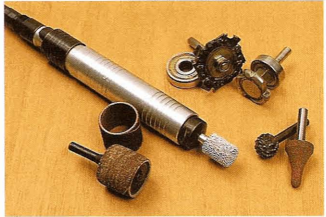
Fig 2.23 The 'business end' of a high-speed flexible shaft. Tooling comes in a whole range of sizes and shapes: shown here are two sanding drums, chainsaw-type and tungsten carbide cutting discs (with their bearing guides) and various rotary burrs
