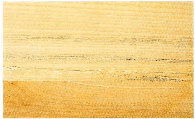
Fig 6.44 A piece of limewood, showing the characteristic blue-grey stain or foxing caused by fungal infection
