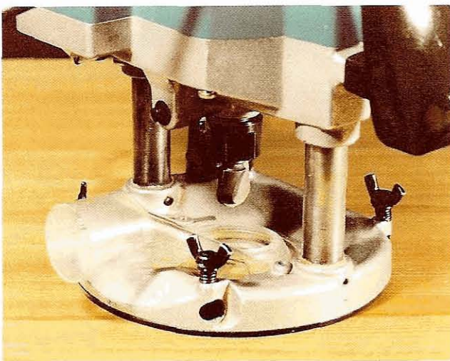
Fig 2.14 The clear plastic fitting is a dust and particle extraction unit which can be connected to a vacuum cleaner. Make it a habit to use dust extraction facilities whenever you can
