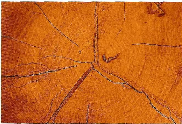
Fig 6.35 Surface checks in a whole-log elm sculpture. The smaller ones are filled with wax, which squeezes out or fails to fill, as the wood expands and contracts with the changing humidity of the seasons
