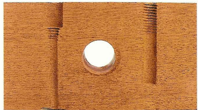
Fig 4.41 The Veritas screw (right) fits the workpiece with a taper of about 5^\circ ; the older Marples model about 35^\circ . The difference in the amount of grip they can get on the wood is obvious
