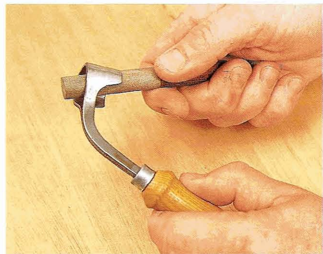
Fig 1.62 Sharpen the scorp with a round slipstone, working from the inside
