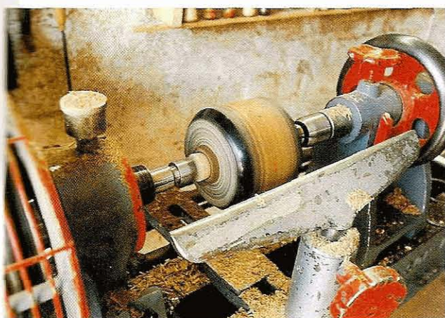
Fig 1.20 Starting to flatten the ends. The problem is how to finish up to the plug
