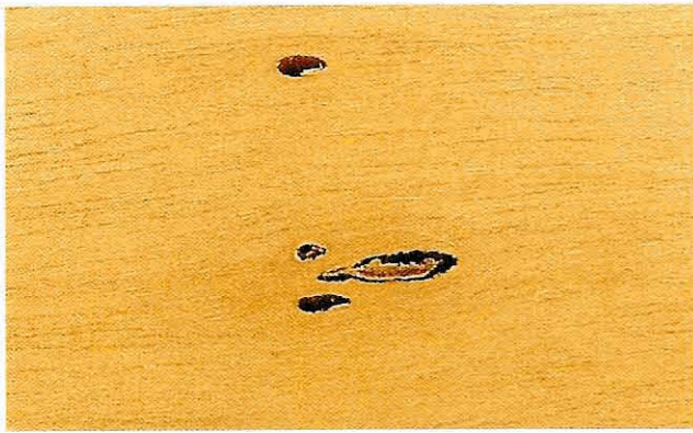
Fig 6.42 Not knots, but hollow resin channels in a piece of jelutong. Many tropical hardwoods have such channels running deeply through them, and they are not necessarily apparent on the surface
