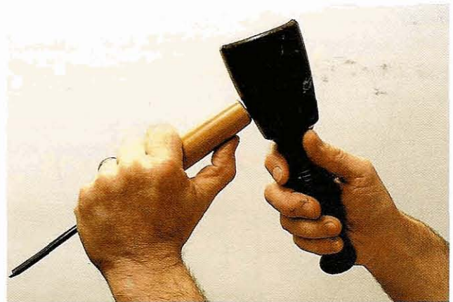
Fig 1.28 The usual way to strike with a mallet: the extended thumb helps to guide the carving tool
