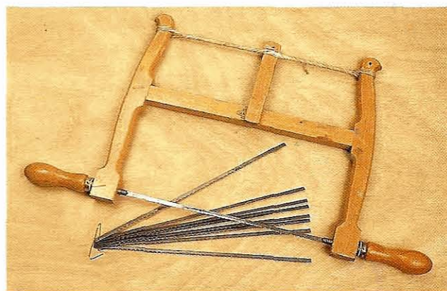
Fig 1.47 The bowsaw looks like something out of the ark – and may well be as old. The blade is held in position by removable pins so the saw can be used for pierced work
