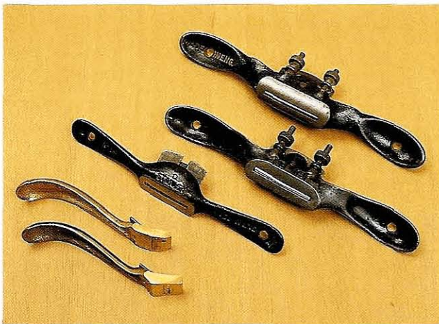
Fig 1.52 A round-faced spokeshave (top) and two flat-faced ones. The small brass carving planes in the foreground have similar uses
