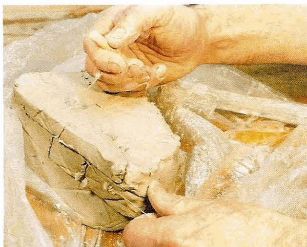
Fig 8.17 Cutting lumps from a block of clay with thin wire is the easiest way to remove what you need
