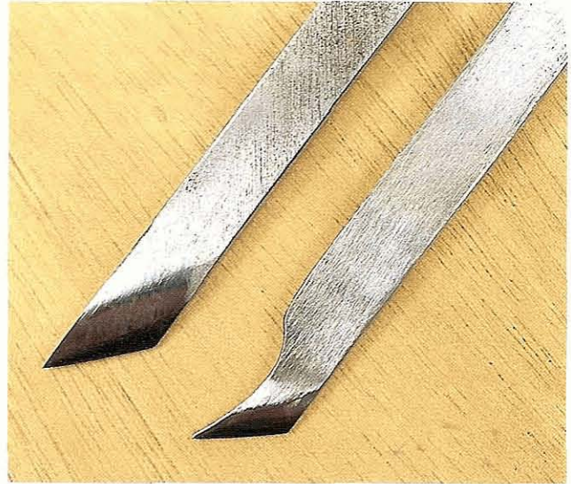
Fig 3.26 A cold procedure: grinding the back edge of a skew chisel to emphasize the point and so gain access to tight corners
