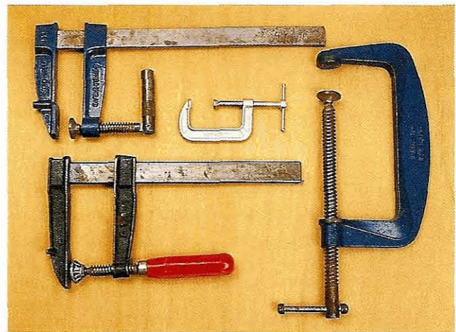
Fig 4.21 Quick-action (left) and conventional (right) screw G-clamps. The one at top left with the swivel handle is particularly good
