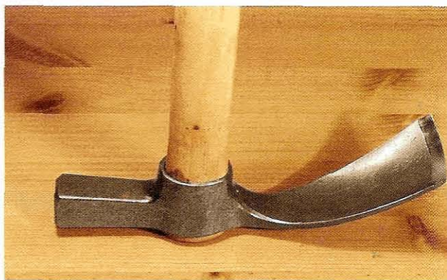
Fig 1.58 This adze by Auriou has a substantial handle passing through the head; the anvil edge may be struck to ease an embedded adze out of the wood
