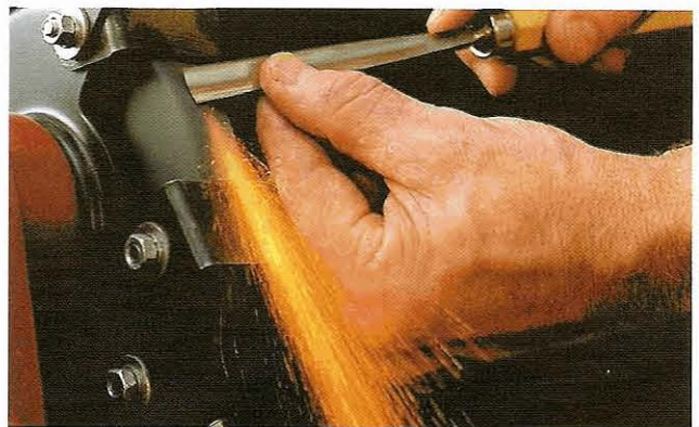
Fig 3.5 Plentiful sparks from a piece of steel indicate that it is made of high-carbon steel and is suitable for making into a woodcarving tool
