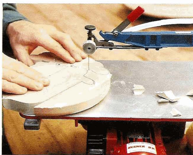
Fig 2.7 A good-quality scrollsaw gives a truly vertical cut, ideal for small, accurate profiling. For delicate work, holding the wood down with the fingers is often quite adequate
