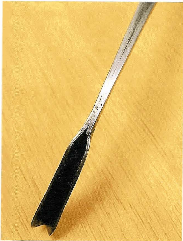
Fig 3.39 The weld in this tool is a fusion of the two sides into one shank of metal
