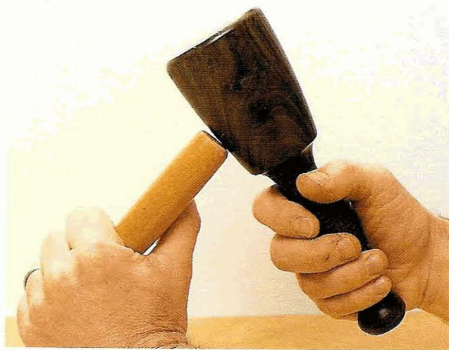
Fig 1.11 A round carving mallet should also be tapered so as to reflect the swing from the elbow and strike the tool handle squarely
