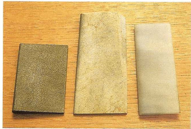
Fig 11.15 (Left to right:) Washita, hard white Arkansas, translucent Arkansas
