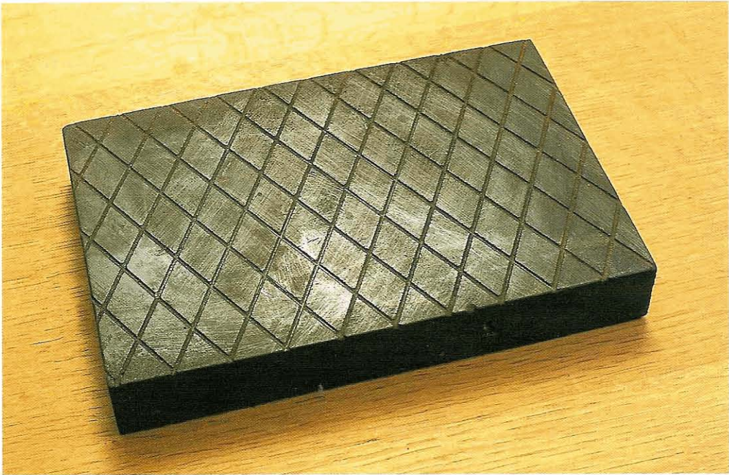
Fig 11.9 An extremely hard cast alloy block meant for dressing stones
