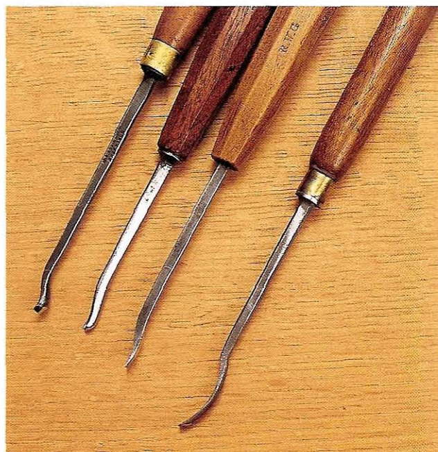
Fig 5.26 The three frontbent gouges on the left have been worn back considerably compared with the somewhat newer tool on the right
