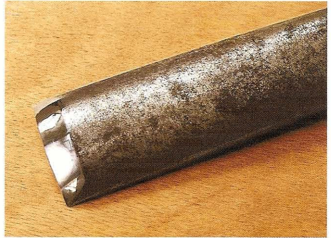
Fig 5.28 A badly rusted surface on a gouge blade, but not pitted enough to affect the cutting edge, which lies more towards the centre of the steel
