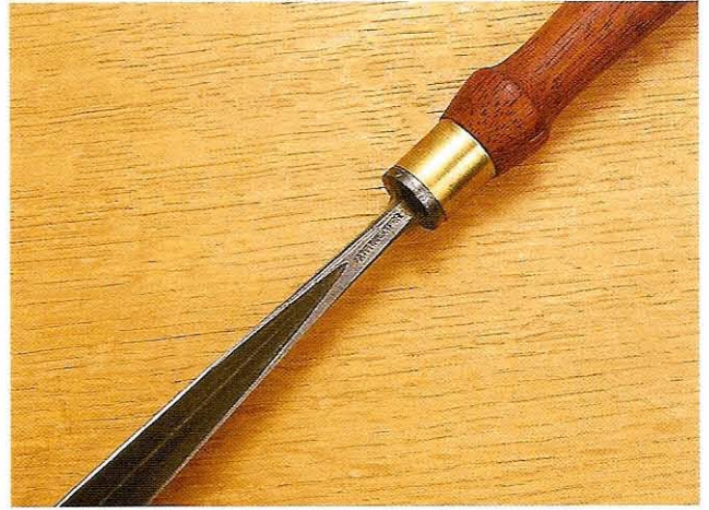
Fig 9.39 Uneven wall thickness in a V-tool may sooner or later cause difficulty in sharpening
