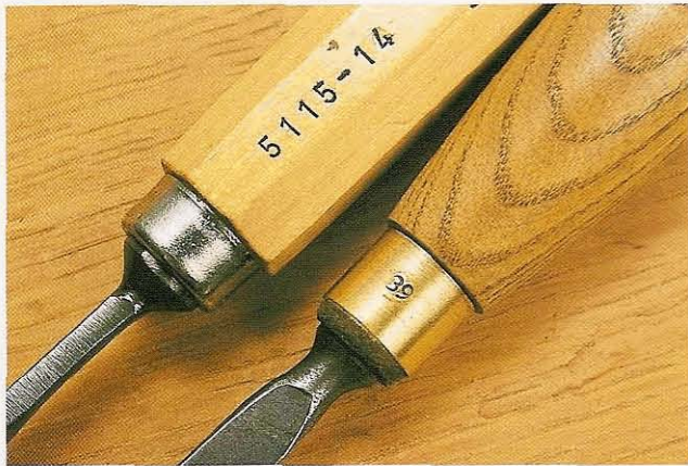
Fig 1.9 If important details are marked on the ferrule or handle instead, this information may get lost if the handle ever needs replacing
