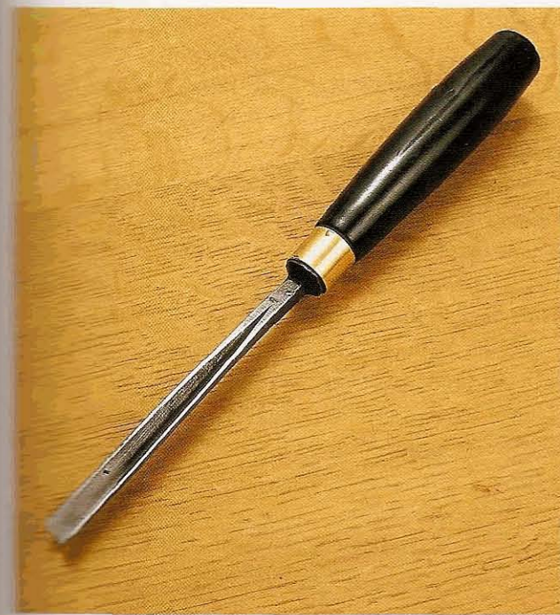
Fig 2.30 The basic V-tool or parting tool
