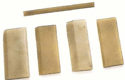
Fig 11.26 A very useful set of four small Arkansas slips with different profiles and (above) a triangular slipstone
