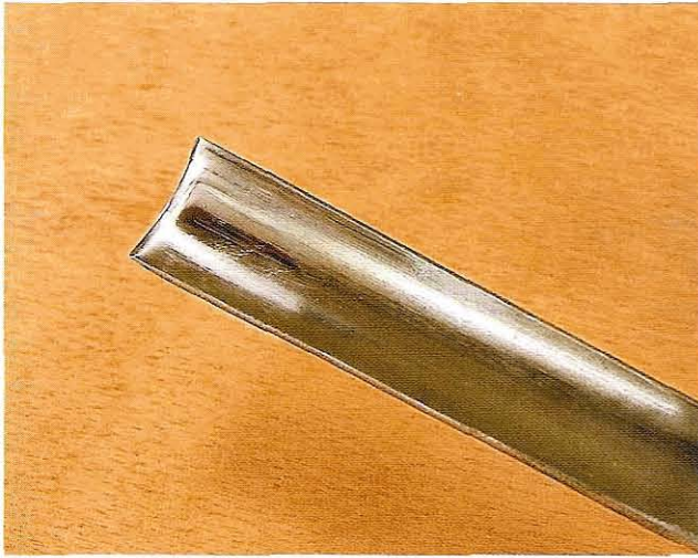
Fig 9.20 The well-stropped inner bevel, seen from above
