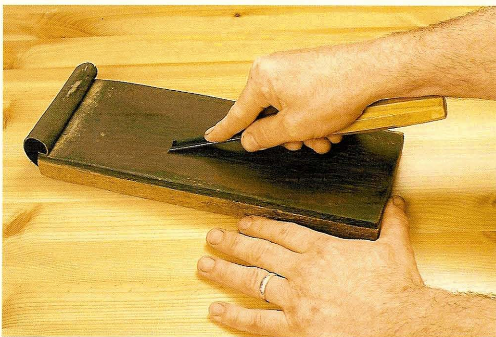
A habit of regular stropping will maintain the keenness of the cutting edge, and help to make sharpening a pleasant routine rather than a major event
