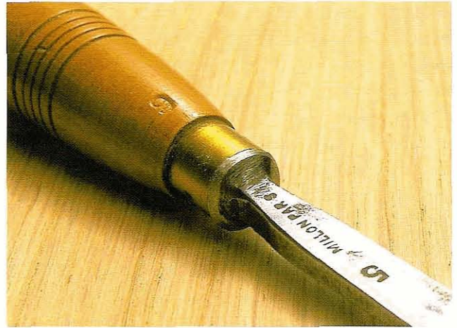
Fig 3.35 Problems in removing the handle may arise when the shoulder is very tight to the ferrule
