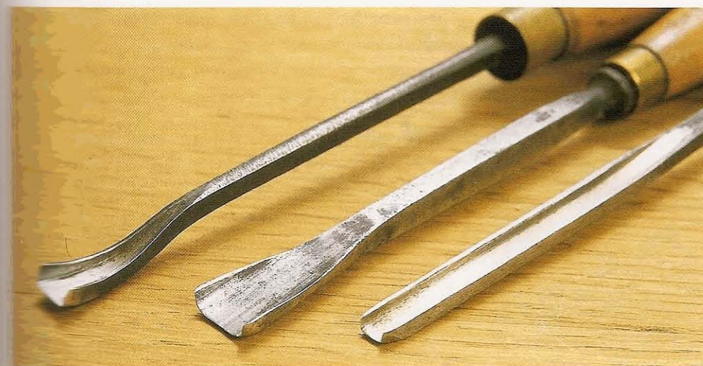
Fig 2.35 Shortbent, fishtail and straight macaroni tools
