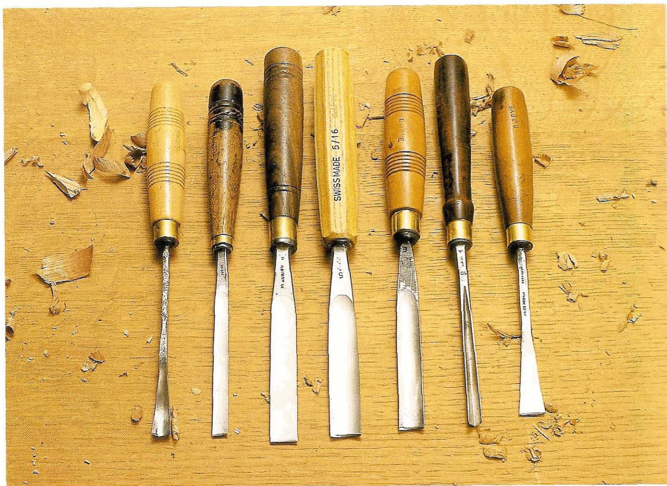
Fig 7.8 Lining up the tools in use keeps their edges from knocking against each other and makes them easier to recognize
