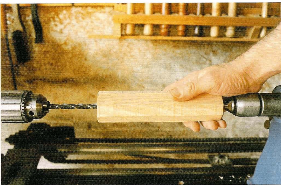
Fig 3.28 On the lathe, a hole can be drilled easily and accurately between centres
