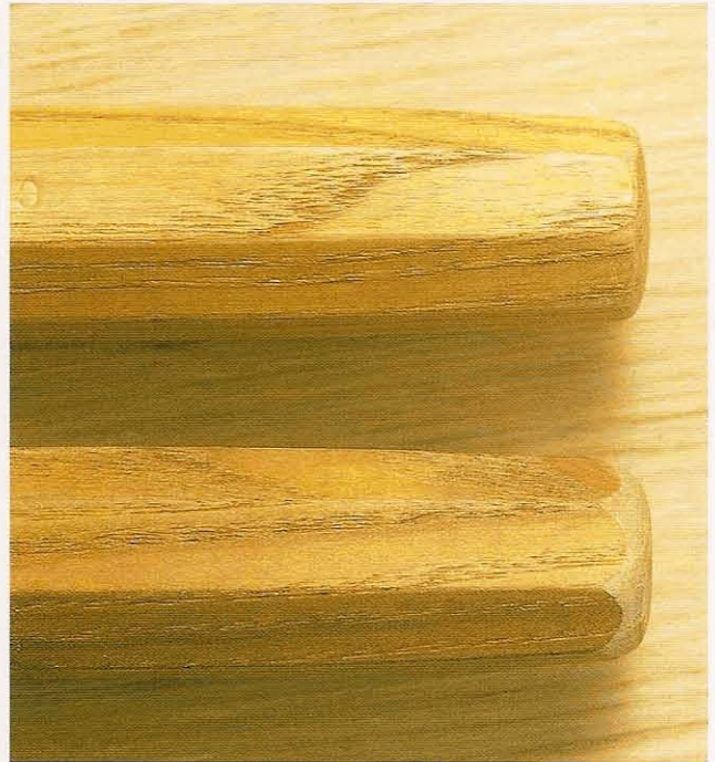
Fig 3.10 Octagonal handles can have quite sharp corners (top); round them over to make them more comfortable
