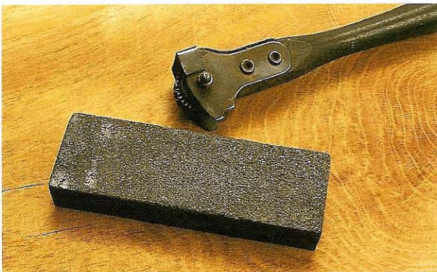
Fig 10.6 Dressing stone (left) and dressing wheel
