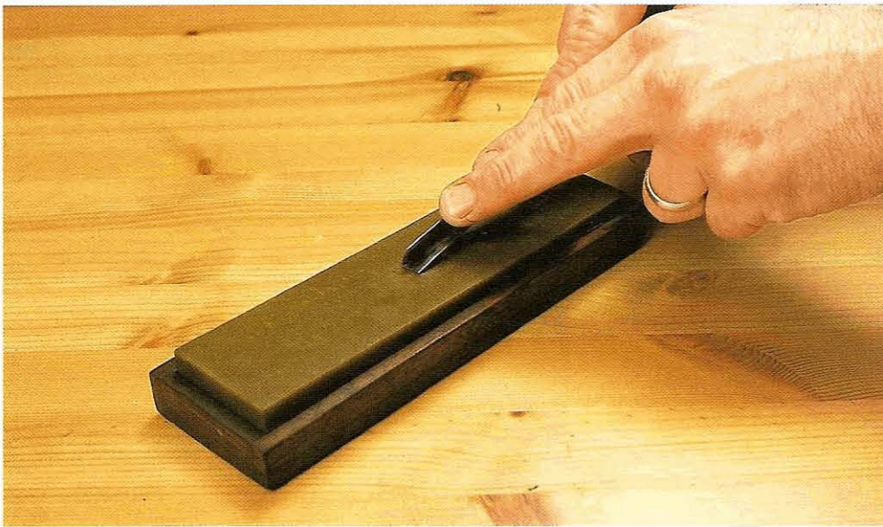
Fig 12.35 Treat one side of the V-tool like a chisel . . .
