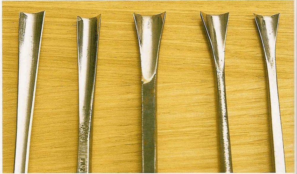
Fig 2.41 A range of tapered gouges, from spade to fishtail; nomenclature varies between manufacturers. You need to decide what you want to achieve, and ask which shape of tool will do it for you
