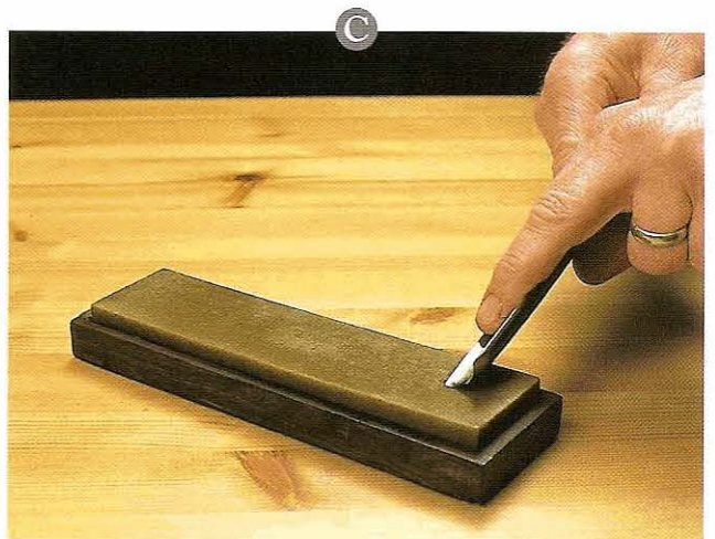
Fig 12.45 Rotating the gouge from one end of the benchstone to the other. The motion is then repeated in the opposite direction, without lifting the blade from the stone
