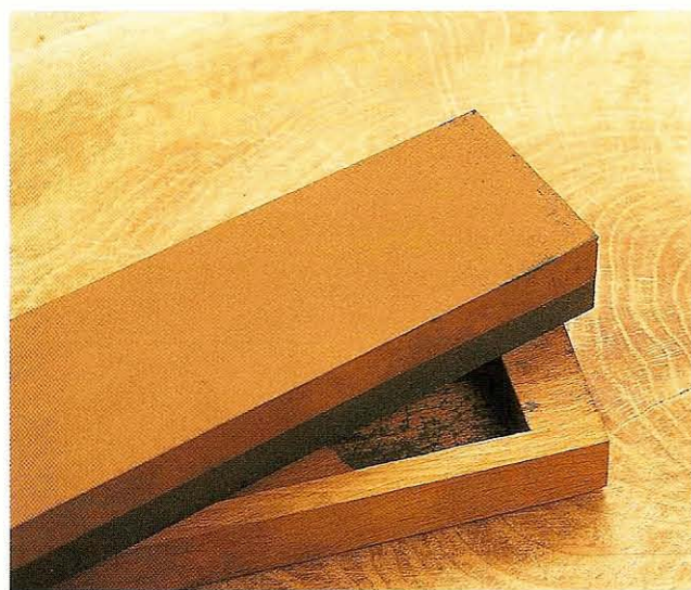
Fig 11.1 Combination stones are a laminate of coarse and fine Carborundum grits
