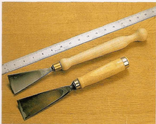
Fig 3.6 The extra-long handle on one of these shallow gouges facilitates the flattening of backgrounds
