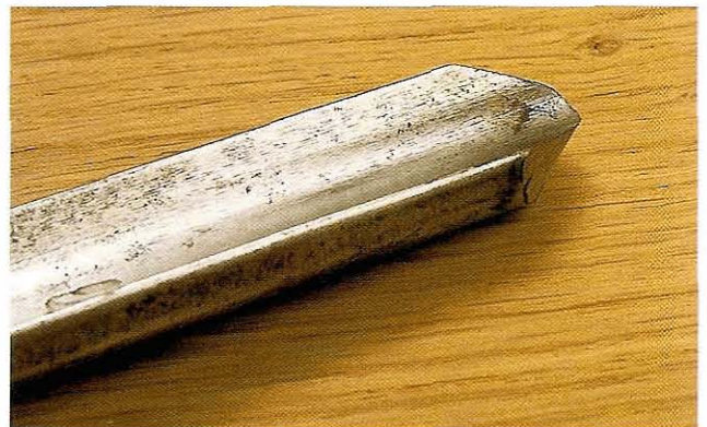
Fig 8.1 The nose of a woodturner's spindle gouge: both the steep bevel and the rounded end make this an unsuitable shape for a carving tool
