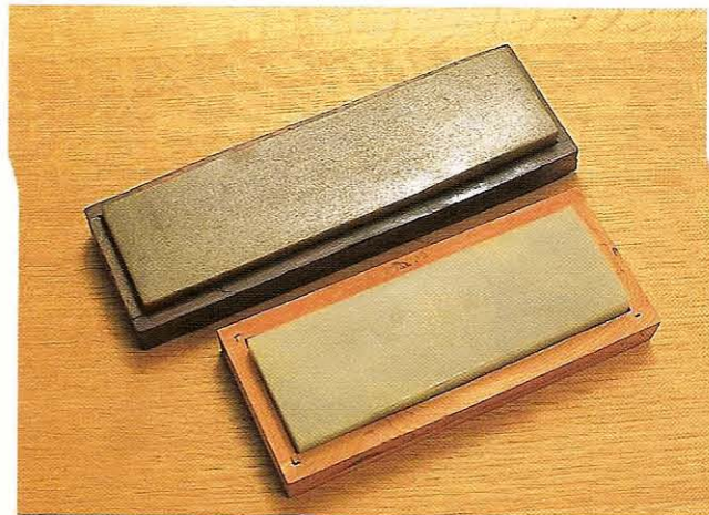
Fig 11.16 The white Arkansas benchstone appears white when new, going grey with oiling. The one with white mottling on grey has been newly dressed
