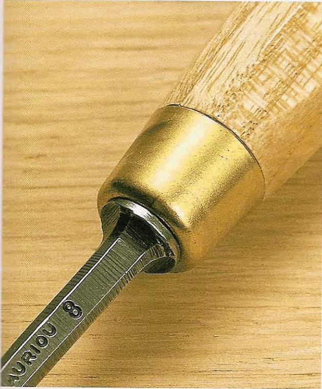
Fig 2.69 A beautifully forged shoulder with a good size and shape, seated well on the handle
