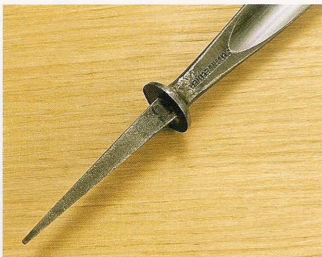
Fig 2.72 A strong, straight, well-made and purposeful tang
