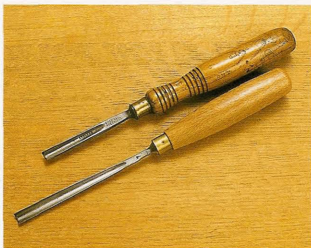
Fig 2.5 The old gouge at the top would originally have been as long as the modern one beneath. The reduction in length represents many years of carving and sharpening
