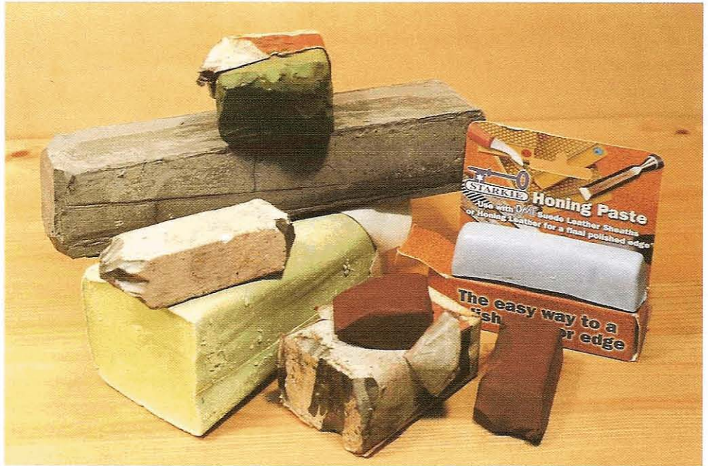
Fig 14.5 A collection of proprietary and other sharpening 'soaps'; there are many different kinds to be had
