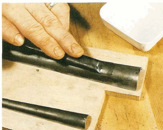
Fig 13.8 Go no further than the width of the edge, or you will lose the corners
