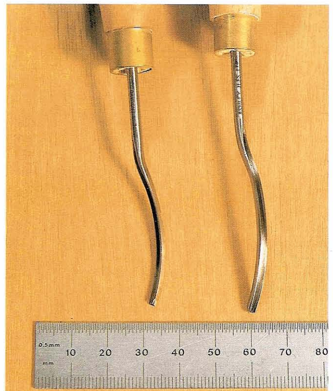
Fig 6.11 Ashley Iles back and front longbent V-tools
