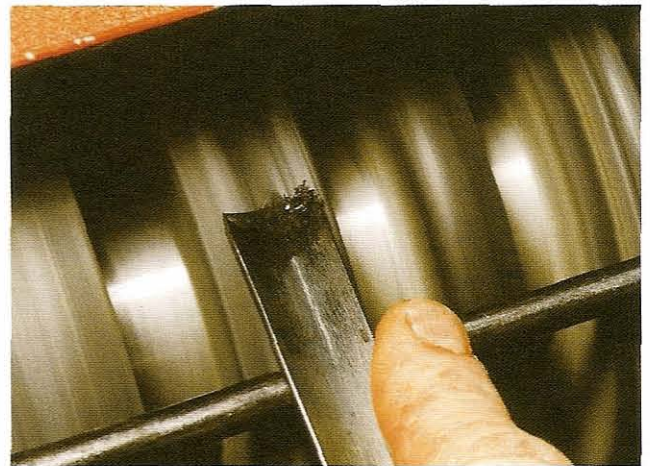
Fig 14.8 Present the heel first, then lift the handle far enough to arrive at the edge, and no further
