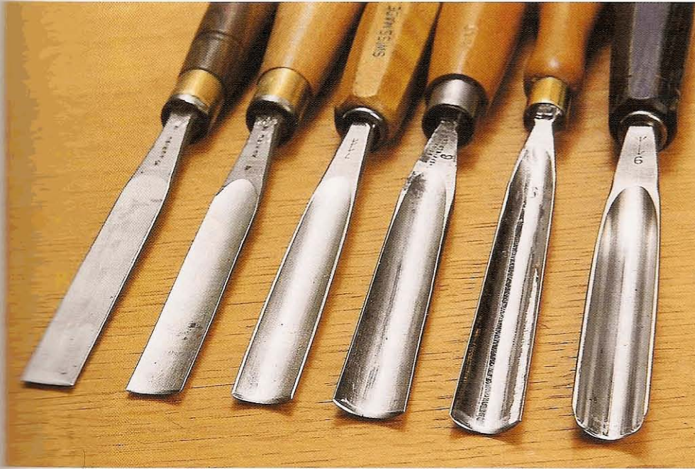
Fig 2.20 A selection of sweeps ranging from the flat to the semicircular
