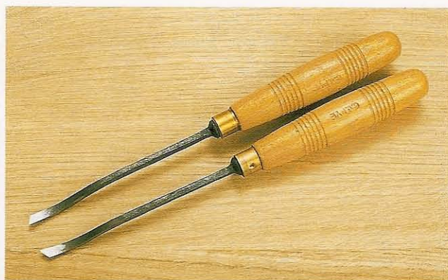
Fig 2.49 Shortbent skew chisels come in pairs, left- and right-handed, to suit different grain conditions
