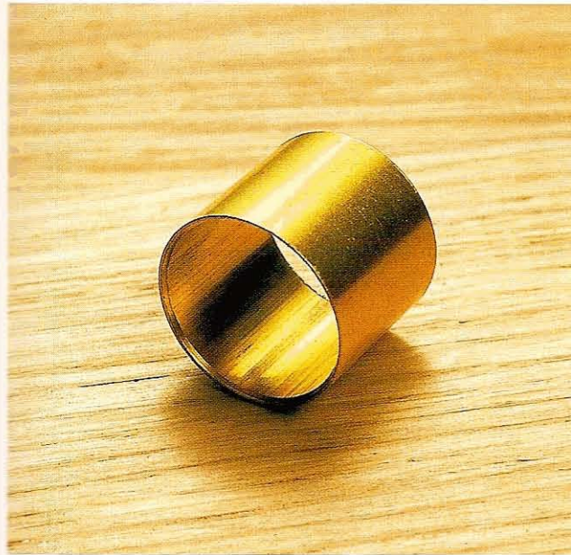
Fig 3.19 Close-up of a brass tang ferrule, showing the inside bevel. The bevel is offered to the handle first, and jams the ferrule in place by compressing the wood
