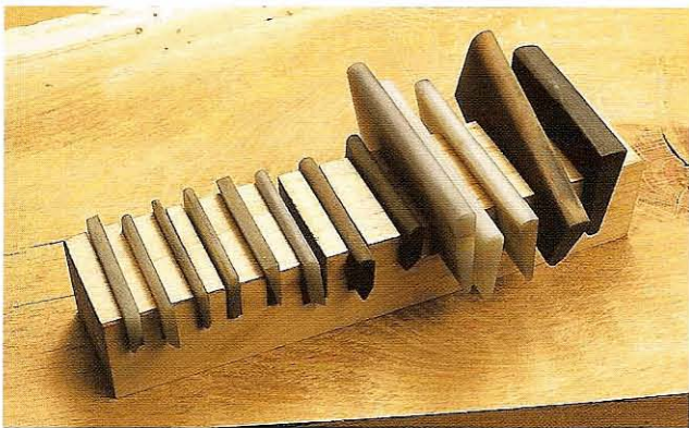
Fig 11.28 Small slipstones are quite brittle and easily chipped or broken. A rack like this will stop them damaging one another
