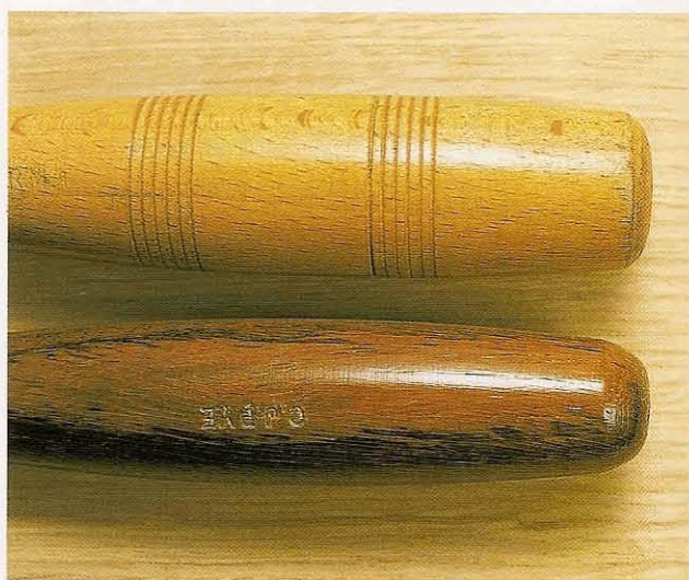
Fig 3.16 The wider end of the upper handle is a better target for the mallet than the other, which reduces towards a point
