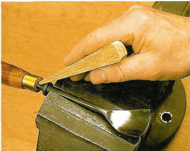
Fig 3.34 Using a wedge of hardwood to knock off the handle. Keep your hand clear of the cutting edge!
