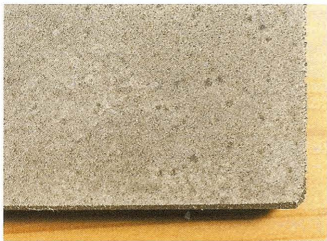
Fig 13.5 Close-up of a polycrystalline diamond surface showing the tiny cutting crystals
