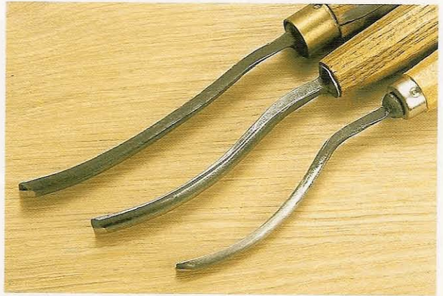
Fig 2.45 The amount of lengthwise curvature in longbent gouges varies between manufacturers. Some have so little curve as to be little improvement on the straight gouge
