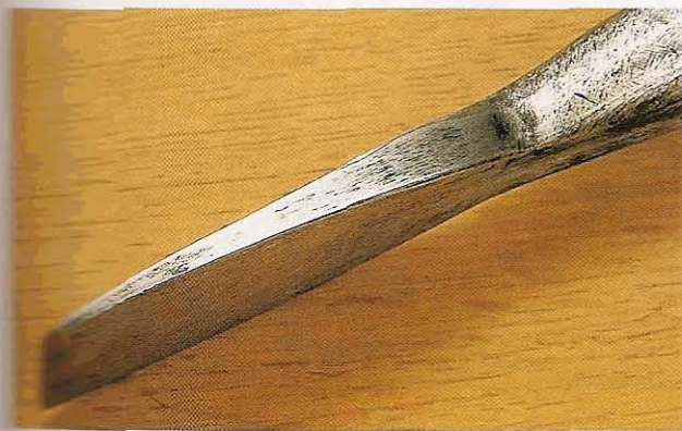
Fig 2.13 An old firmer chisel with a socketed rather than tapered blade, tapering straight to the edge
