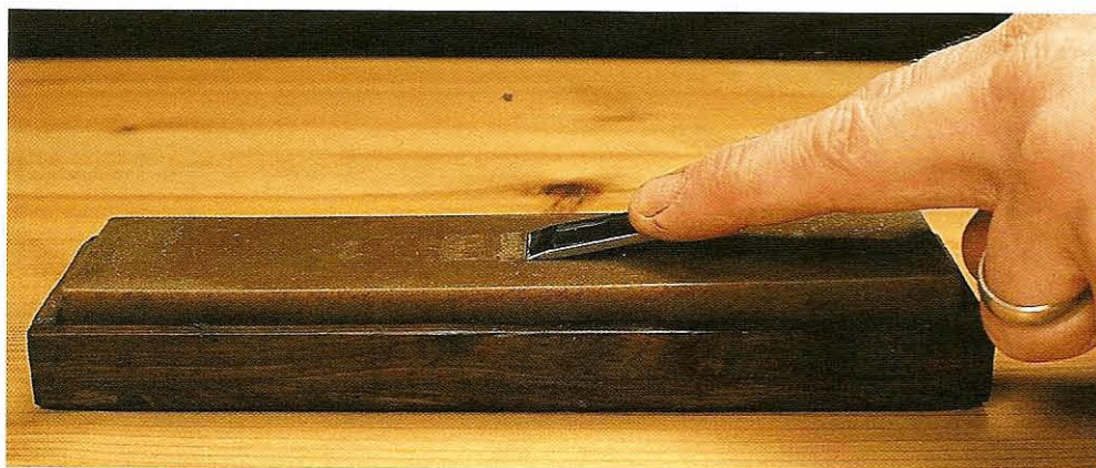
Fig 12.8 Flatten the bevel by offering it square-on to the rotation. Do this lightly and make sure your hand is supported by the toolrest. If preferred, this method can be used for all the bevel shaping
