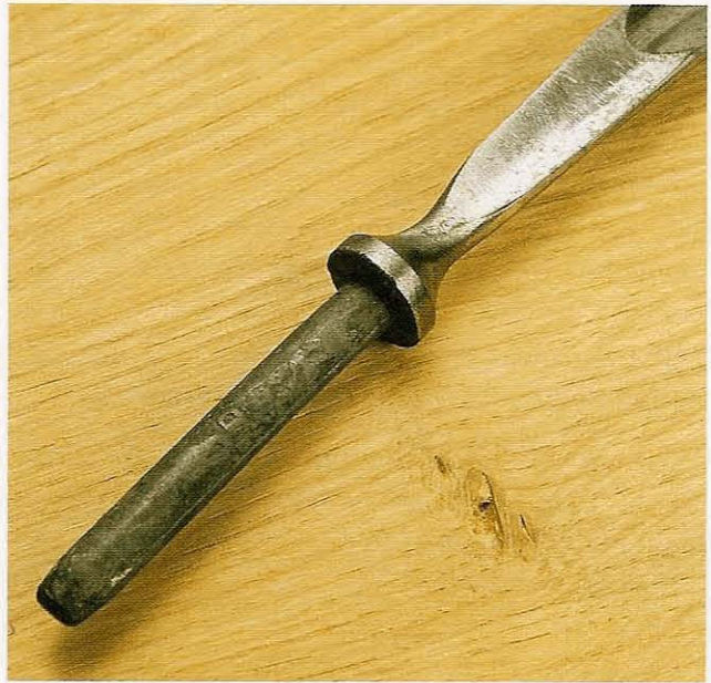
Fig 2.75 The parallel, round tang is unusual and does not 'bite' the wood like square-sectioned tangs. In this case the tang, and shoulder, are strong and well made, so there should be no problem providing the tang grips the hole in the handle tightly enough
