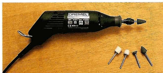
Fig 10.4 This sort of inexpensive unit is now widely available. Besides small abrasive wheels, it can be fitted with burs and cutters for working directly on wood
