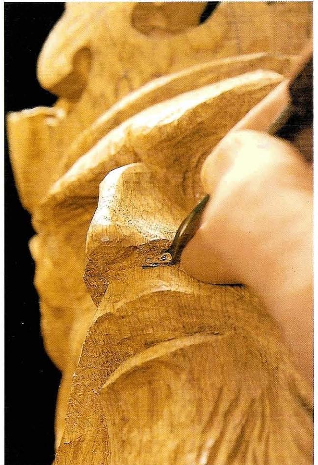
Fig 5.21 A deep hollow worked by a small frontbent gouge
