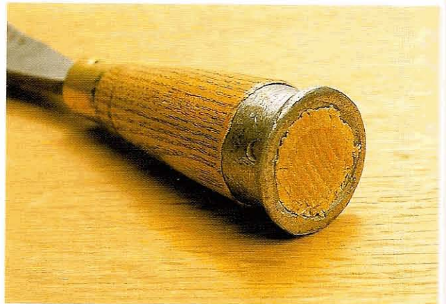
Fig 3.25 Even an iron ferrule can itself burr over after weeks of hard mallet work
