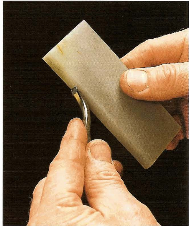
Fig 12.56 Slipstones are used with the benchstone to sharpen a backbent gouge
