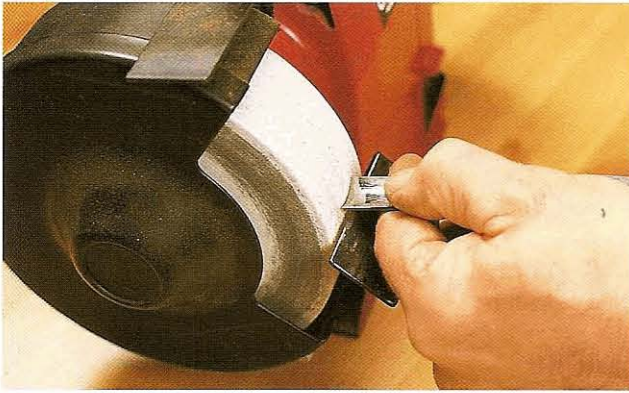
Fig 12.3 Perpendicular presentation (for clarity the grinder's perspex guards are swung up)
