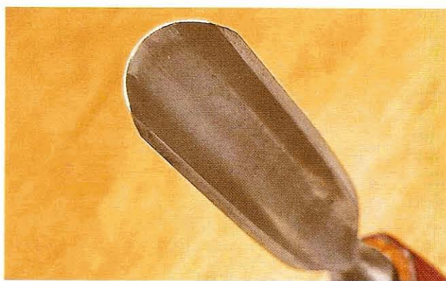
Fig 9.46 The white line of light is getting thinner and more uniform, but is still clearly visible all along the edge
