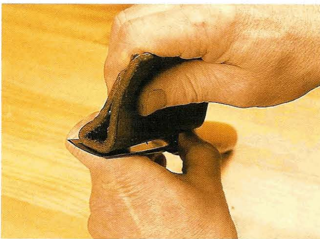
Fig 12.25 A leather slipstop will deform to fit the sweep of the gouge as it is pushed forward
