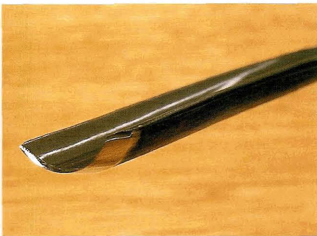
Fig 9.43 A tool with a straight edge, corners present, and flat, polished bevels inside and out
