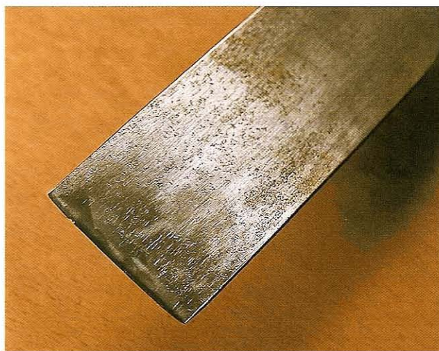
Fig 12.61 The notch in the edge of this gouge should be dealt with before putting it away
