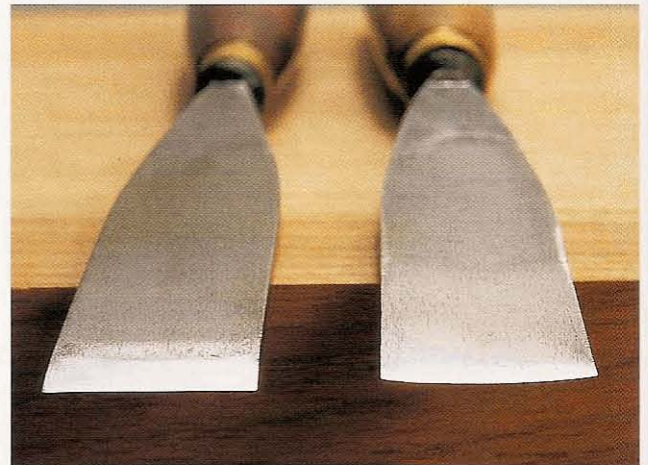
Fig 2.19 The flattest gouge (right) and a chisel (left), seen end-on. From this angle it is clear that the so-called 'flat gouge' is actually significantly curved
