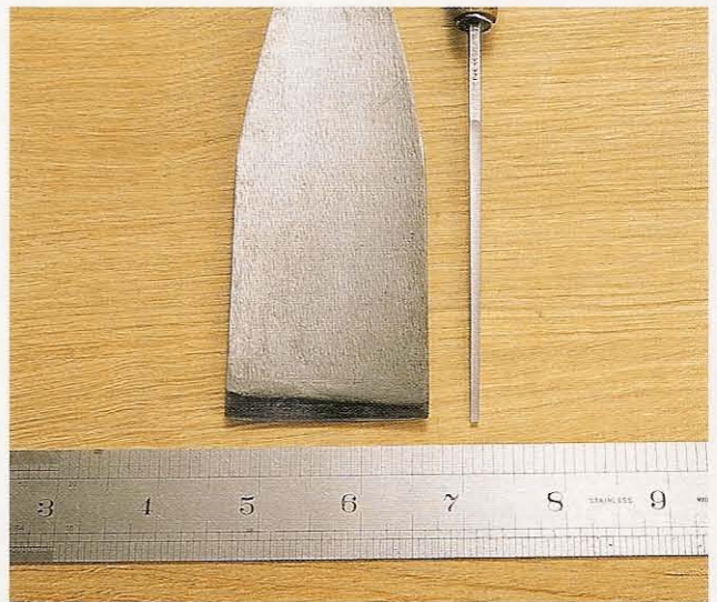
Fig 2.61 Width increments, between the smallest and largest for each type of carving tool, help to account for the enormous numbers that are available
