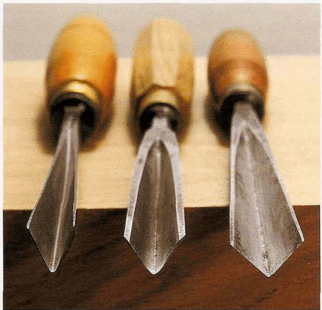
Fig 2.32 The same size of V-tool is available in three different angles: approximately 45^\circ , 60^\circ and 90^\circ (left to right)
