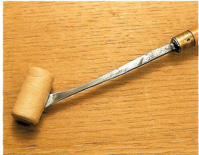
Fig 7.5 A cork, preferably plastic, will protect delicate corners, either on the bench or when the tool is stored
