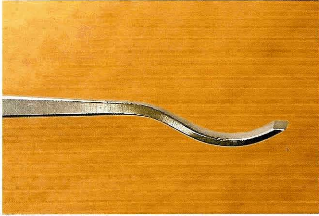
Fig 9.5 The bevel offered by the maker of this tool is about 45^\circ . It may never occur to a newcomer to carving that this can be, and needs to be, changed
