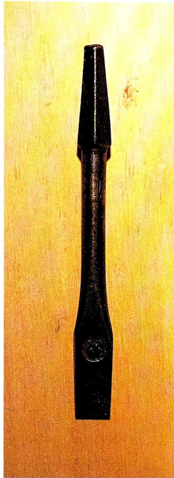
B-14 This screwdriver bit for a brace is an excellent tool for inserting or removing screws where extra purchase is required.
