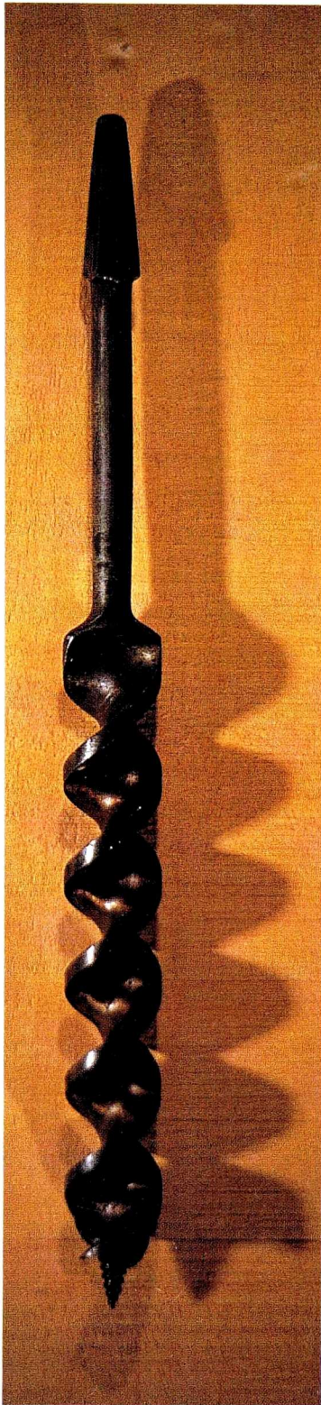
B-13 This is the kind of hole-boring "bit" for a brace. There is often considerable tearing as the bit exits the timber, and it is not a particularly satisfactory hole-boring method for carving.
