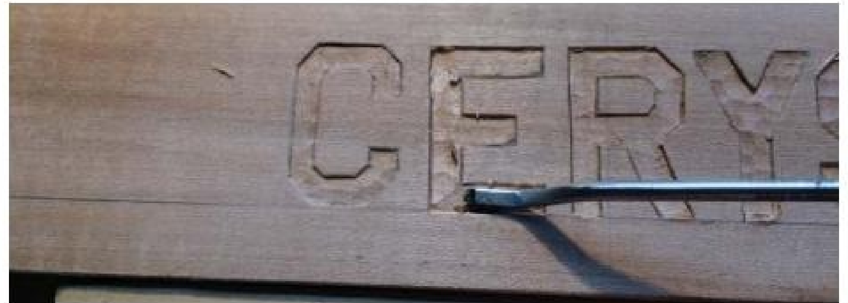
Using a dog-leg chisel to finish the letter
