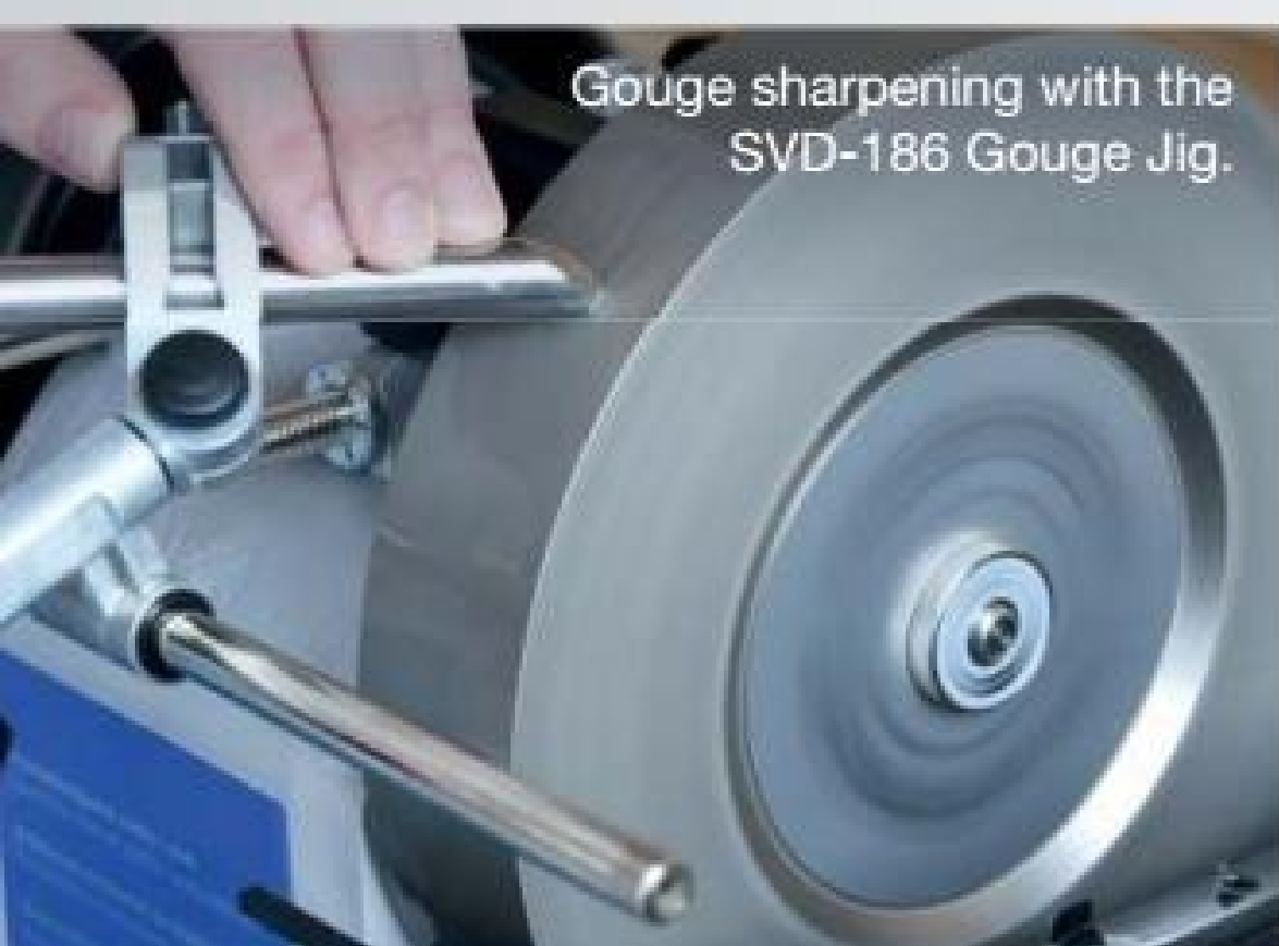
You can sharpen on the the periphery...
