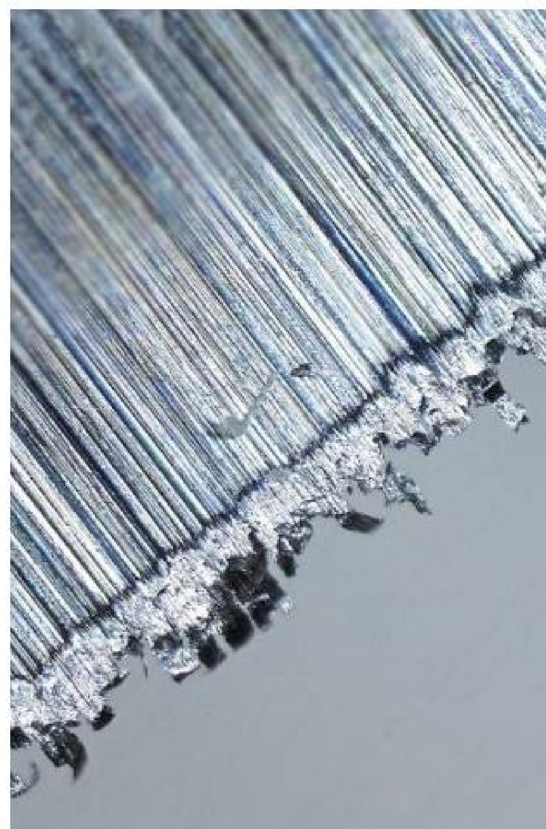
Close-up, wavy line behind the burr shows the toothy edge that needs refining
