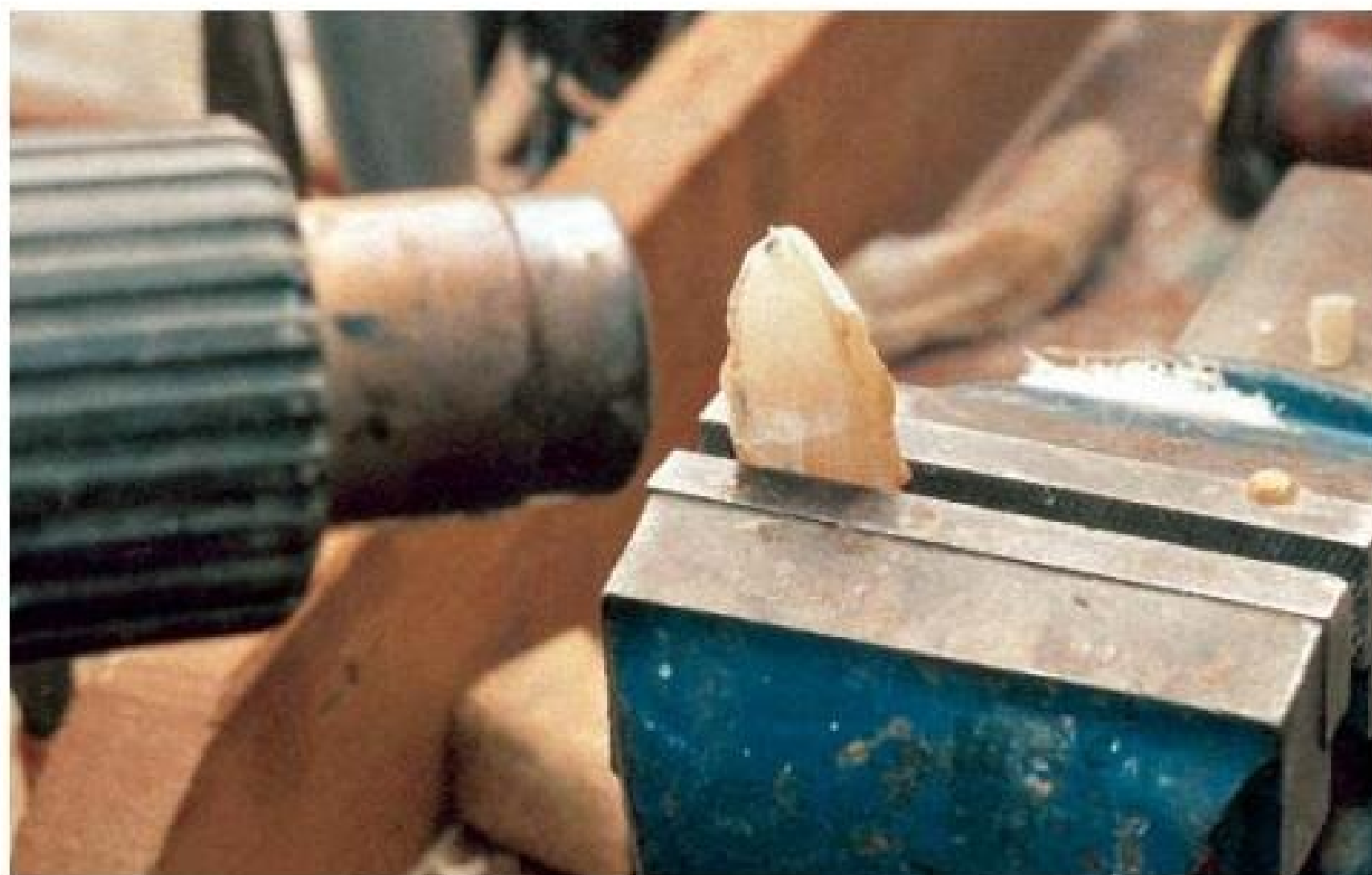
Heat the horn with a hot-air gun ...
