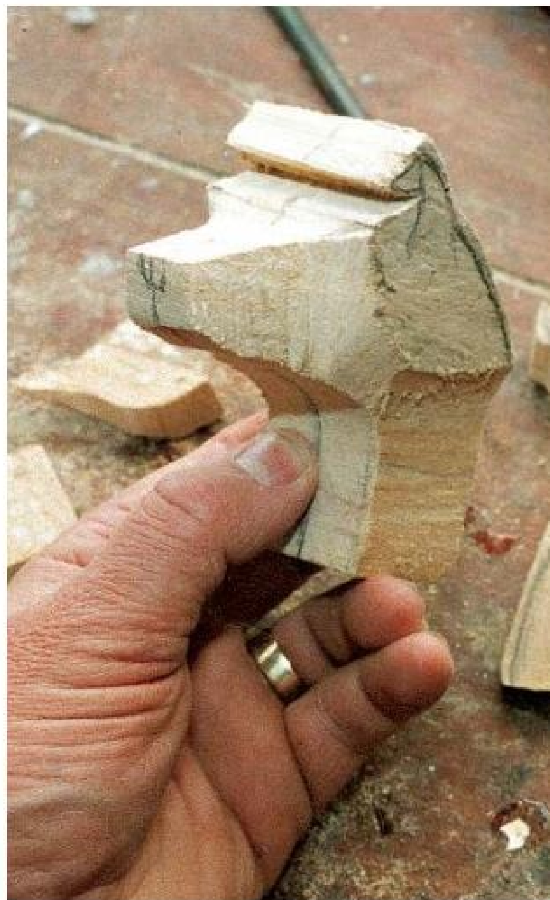
The blank with waste removed from the sides of the neck and head
