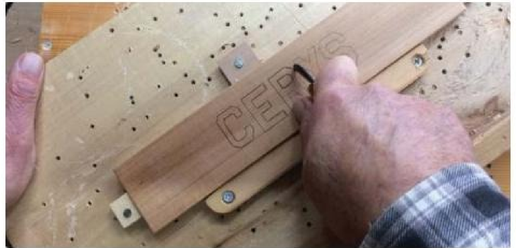
Cutting down to the baseline with a knife
