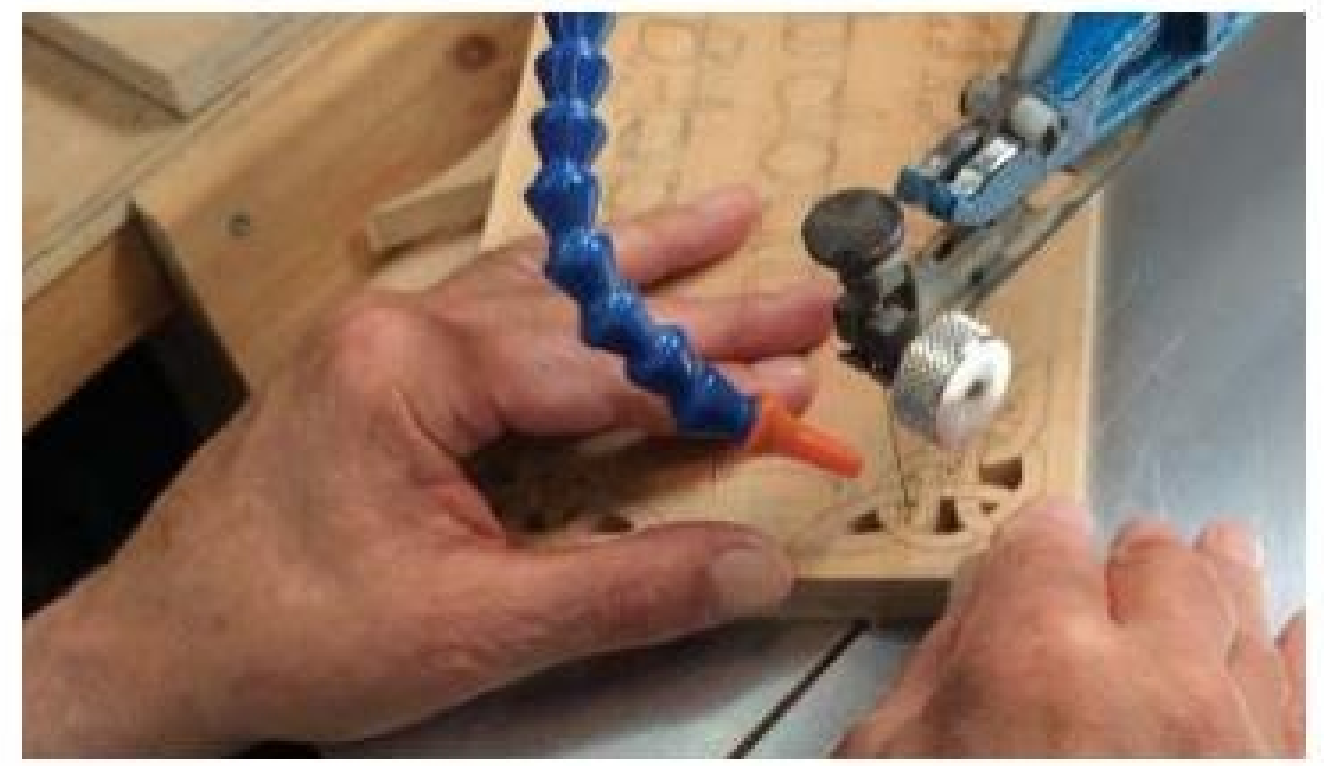
Piercing the corner motifs using a scrollsaw
