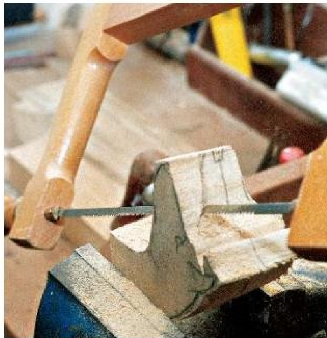
Removing the waste from the sides of the head
