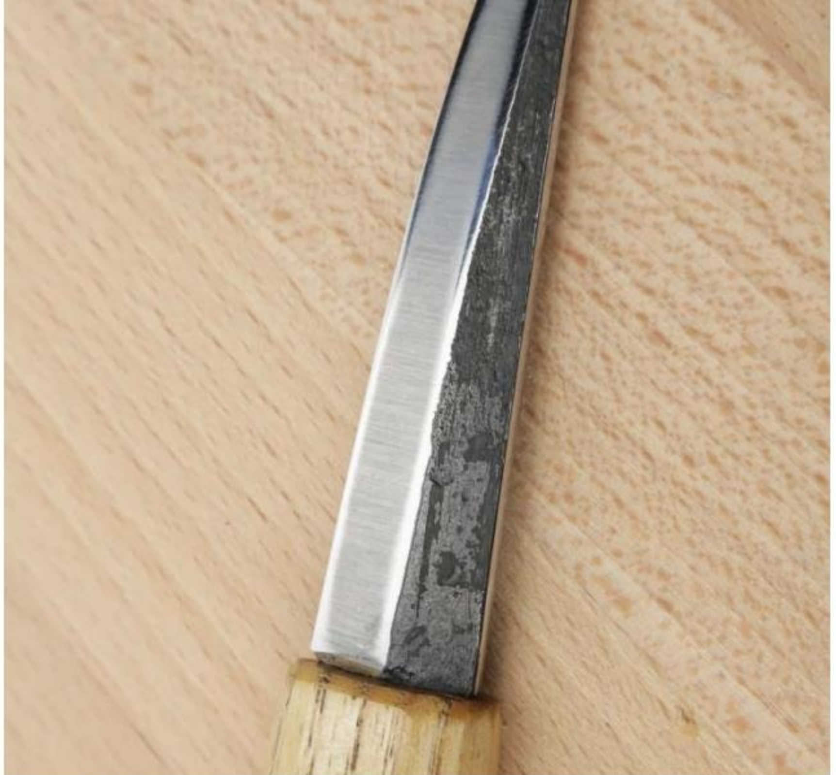
A hollow ground knife with flats
