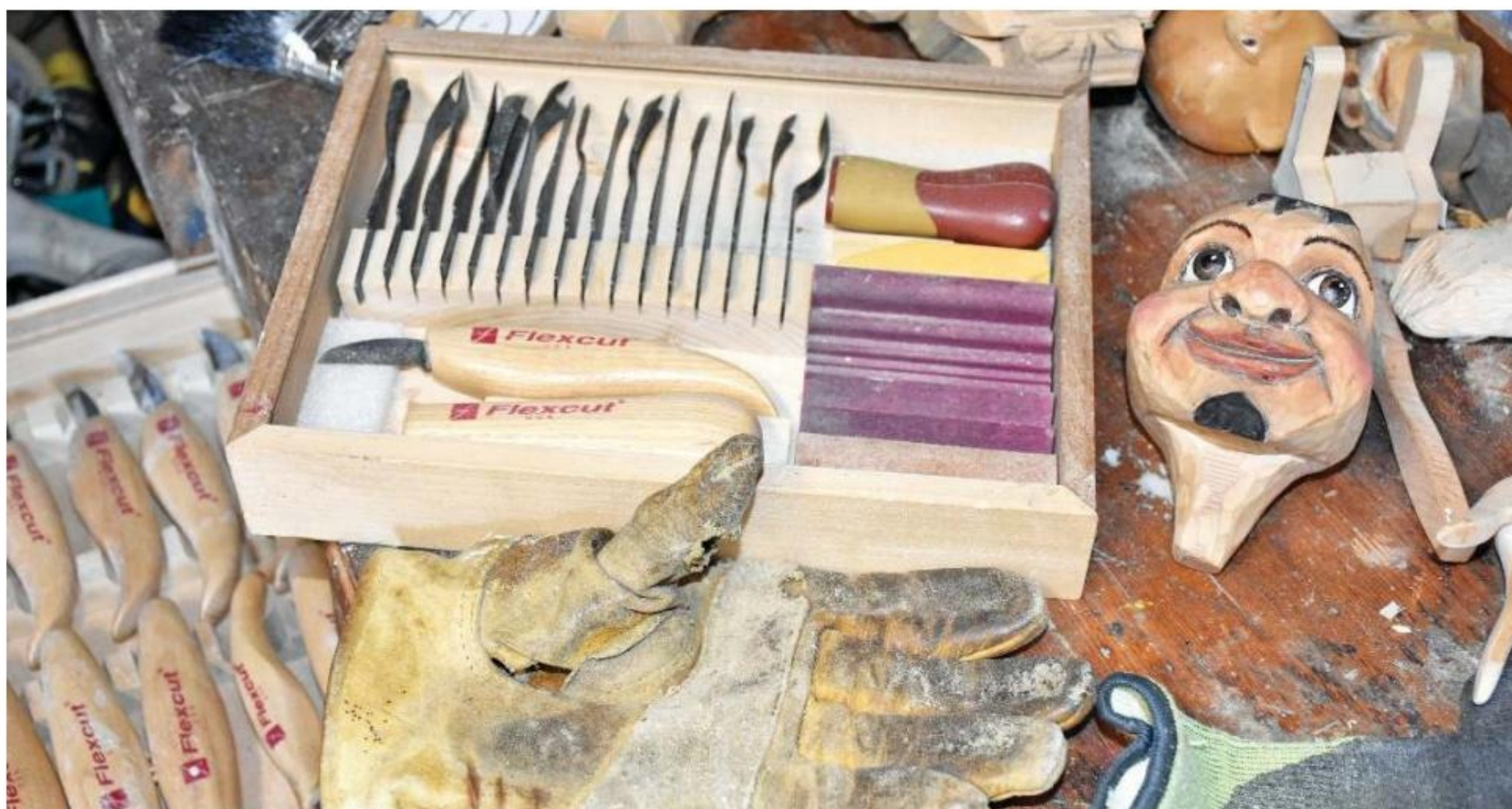
Although Tony has a lot of larger tools, he finds the smaller Flexcut gouges and knives suit his style of carving more where small parts have to often be held in the hand and worked on
