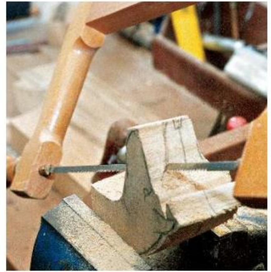
Removing the waste from the sides of the head
