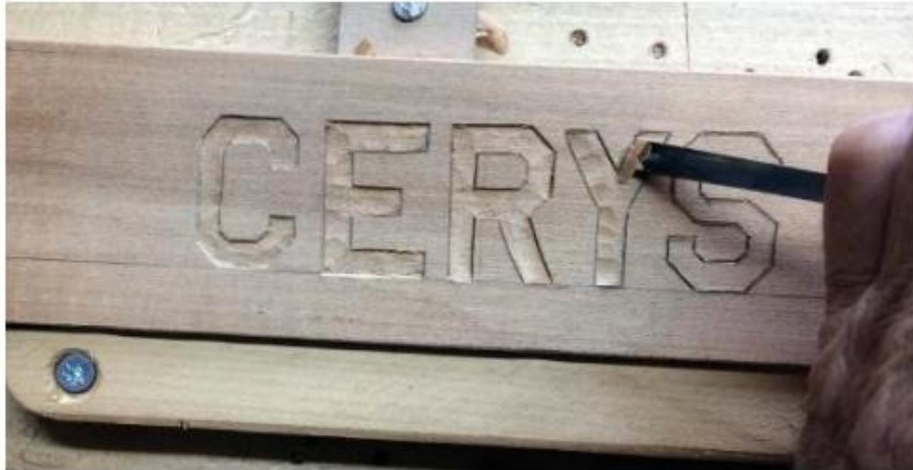
Using a very shallow gouge to start removing waste
