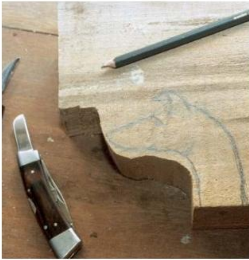
The outline is transferred to the wood, incorporating an area for a workable shank in the neck
