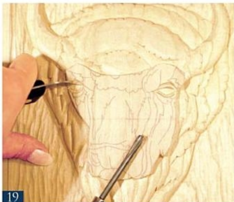
19 Make a stop cut along the joint line of the upper eyelid and the top of the eyeball.
