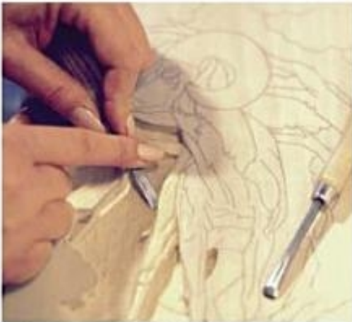
Undercut 3: Use a bench knife, back bent gouge, or dogleg chisel to reach into the cut and clean out the wedge-shaped area.
