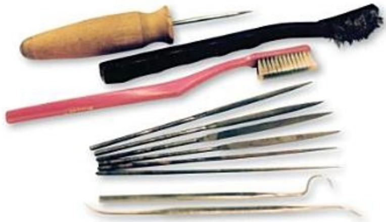
Cleaning tools often include rasps, small files, dental picks, and wire brushes.
