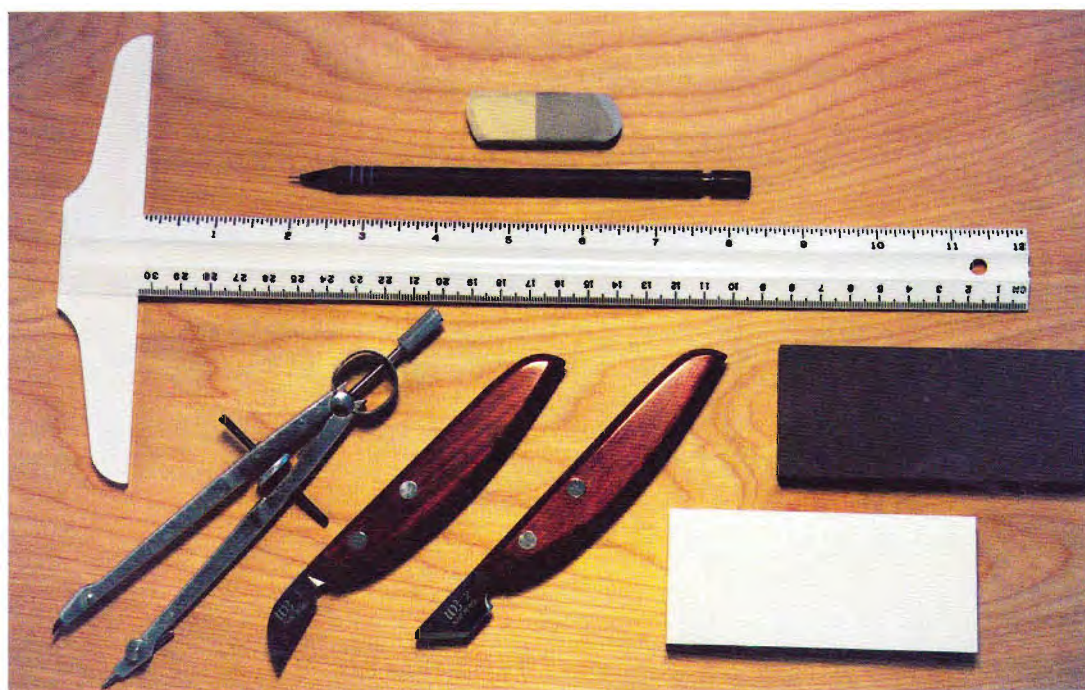
Tools needed for chip carving: T-square, pencil, cutting and stab Premier chip carving knives, draftsman's compass, eraser, and ceramic sharpening and polishing stones.
