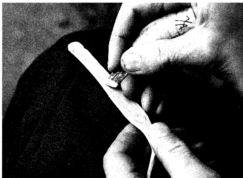
A short-handled, straight-edged engraving knife. The butt can be nestled in the web of the thumb and index finger.
