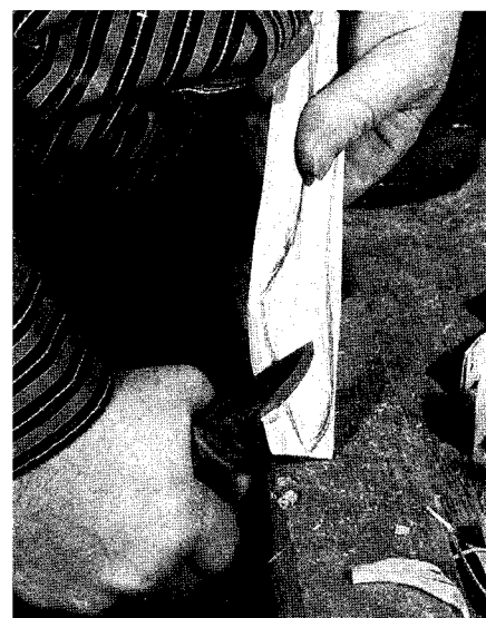
Power can be added to the stroke if you carve against a stop.
