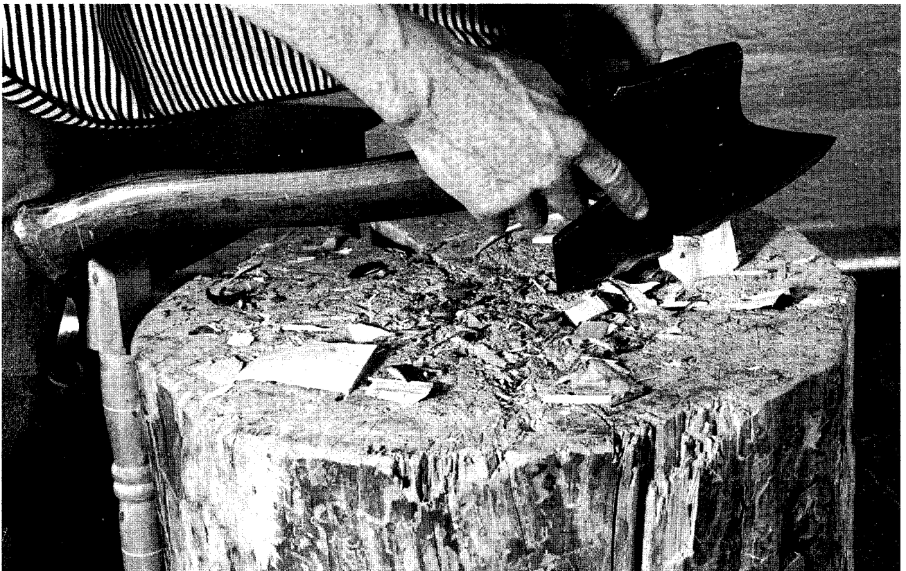
Hewing hatchets have short handles because you usually choke up on the handle for fine work. The narrow throat lets you grasp the tool directly behind the edge.
