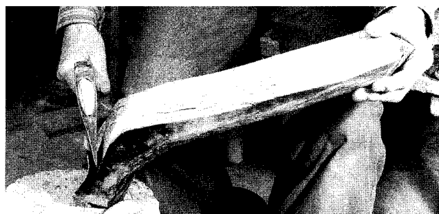
Cleaning up the split on the inner half of a crook. Notice how close the ax hand is to the chopping block.
