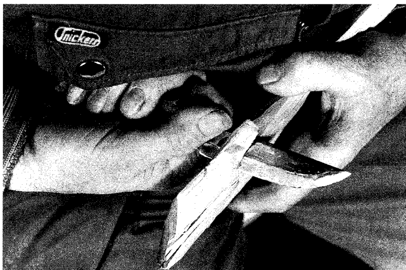
Rough out the spoon handle with the forehand grip (above left) and the chest-lever grip (left).
