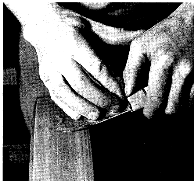
Grinding the blade's tip. The handle is raised and pulled slightly backward, following the curve of the blade.
