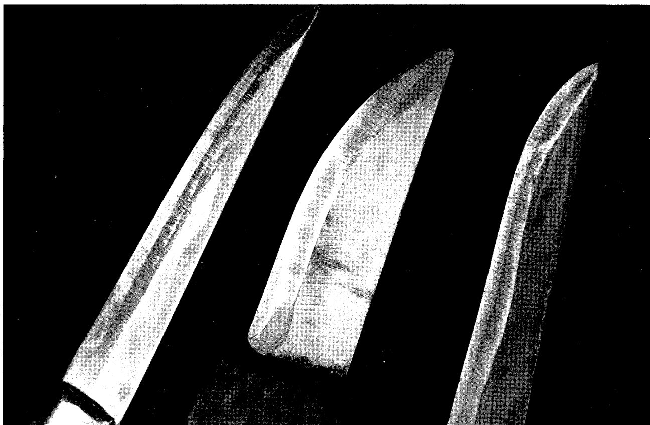
A seam on the bevel reveals a laminated blade. The knife in the middle, with no seam, is of solid steel.
