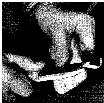
A thumb-push stroke smooths the back of the bowl toward the leading edge. Long strokes will leave a smooth surface.
