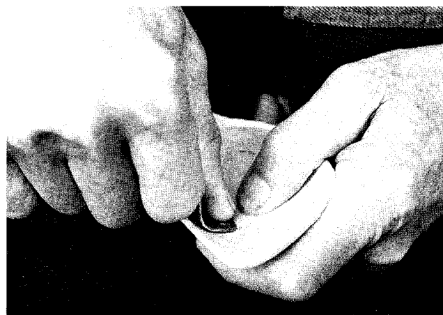
When sanding the bowl's inside, the edge of the sandpaper must be lifted slightly to avoid rounding the rim.
