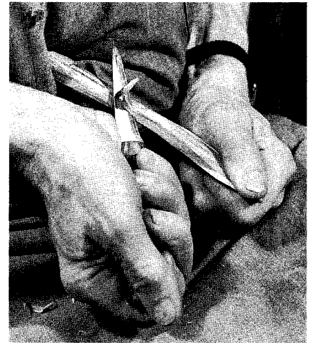
The forearms are pressed against the body and the hands are locked in a cocked position.
