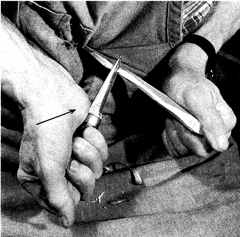
The wrist grip powered toward the body looks dangerous, but it isn't if the correct technique is used.
