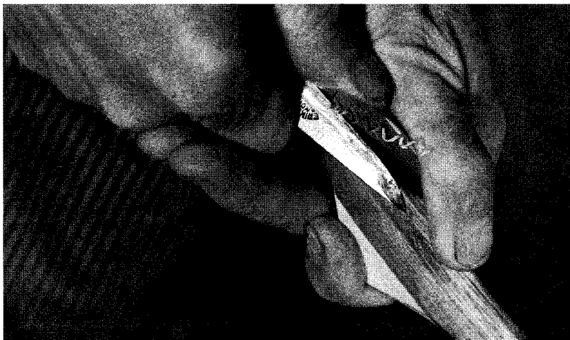
Finish carving requires control that comes from pressing the bevel flat on the work.
