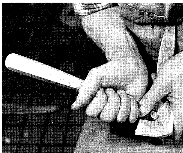
With your arms pressed to your sides and your opposite thumb in the gouge flute, scooping strokes are made easy.
