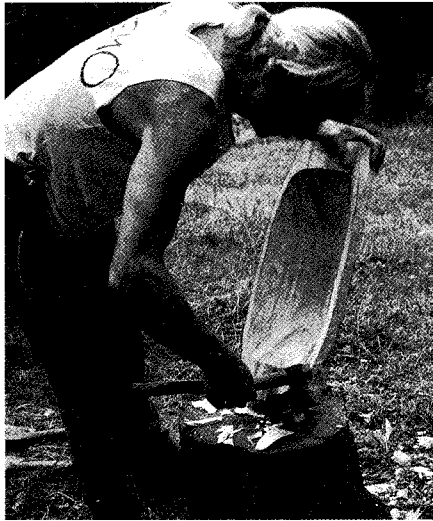
With the inside roughed out, begin shaping the outside of the bowl by hewing to the layout line.
