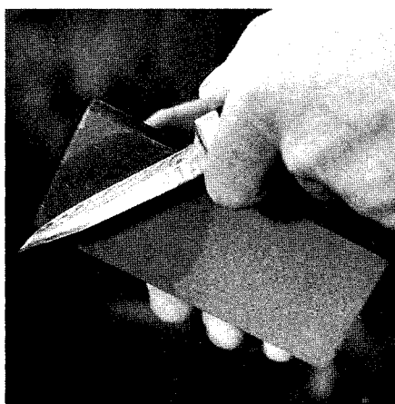
A circular motion is best when honing a knife on an unmounted stone. You can move the stone or the knife, whichever is more comfortable for you.
