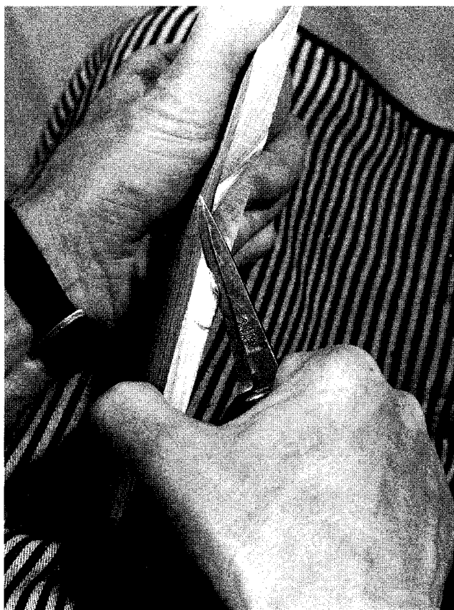
The blank is turned slightly away from the knife to start the stroke near the blade's tip (left). The blank is then rotated into the knife (right), and the stroke is completed when the knife handle and index finger contact the blank.
