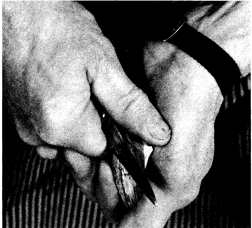
Two hands are better than one. Reinforcing the draw grip with the opposite hand adds control and power.
