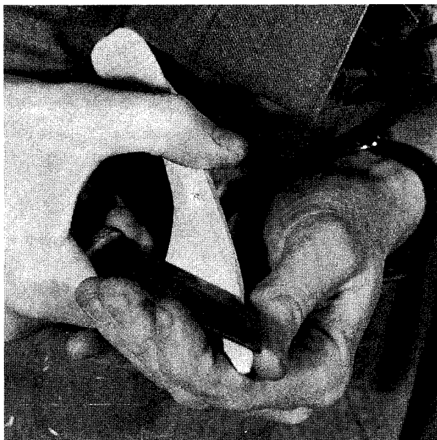
Three fingers of the opposite hand help power the back of the blade. The little finger presses on the knife hand.
