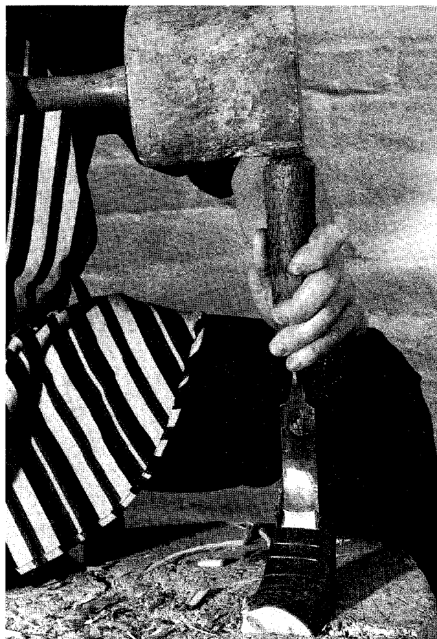
Relief cuts make it easier to hew to a line without splitting wood that should be saved. The chisel shown here is an alternative to the hewing hatchet.
