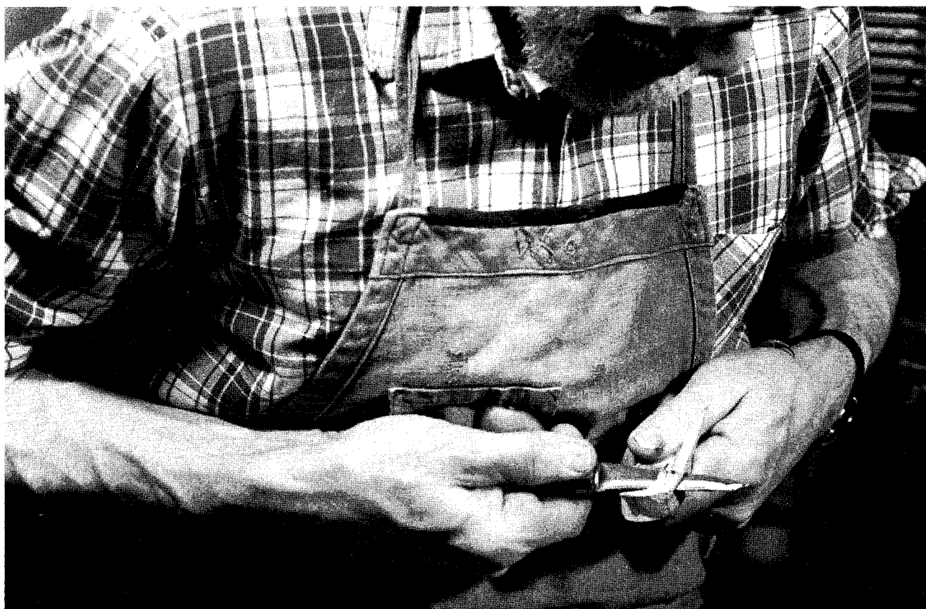
Start the chest-lever grip with your elbows almost straight out from the sides, and your hands in contact with your chest. Your forearms, hands and wrists act as levers and your chest as the fulcrum.
