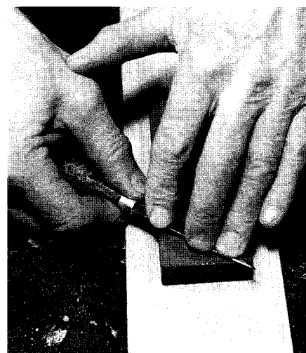
On the opposite bevel, the thumb replaces the index finger to keep the bevel flat on the stone. The left thumb still braces the hands.
