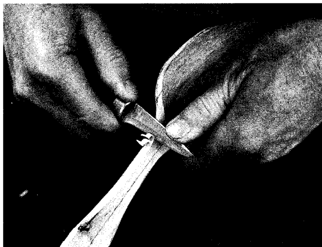
Where grain direction changes, smooth the surface with thumb-push strokes, alternating directions.
