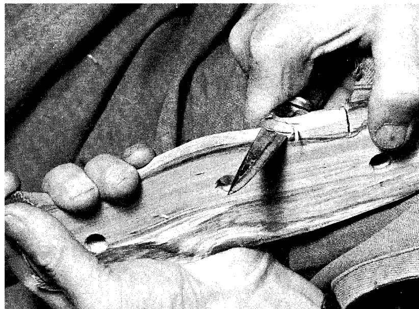
To shape the edge of the board blank, you can saw relief cuts, then use a modified thumb-joint grip and shear from blade tip to hilt.
