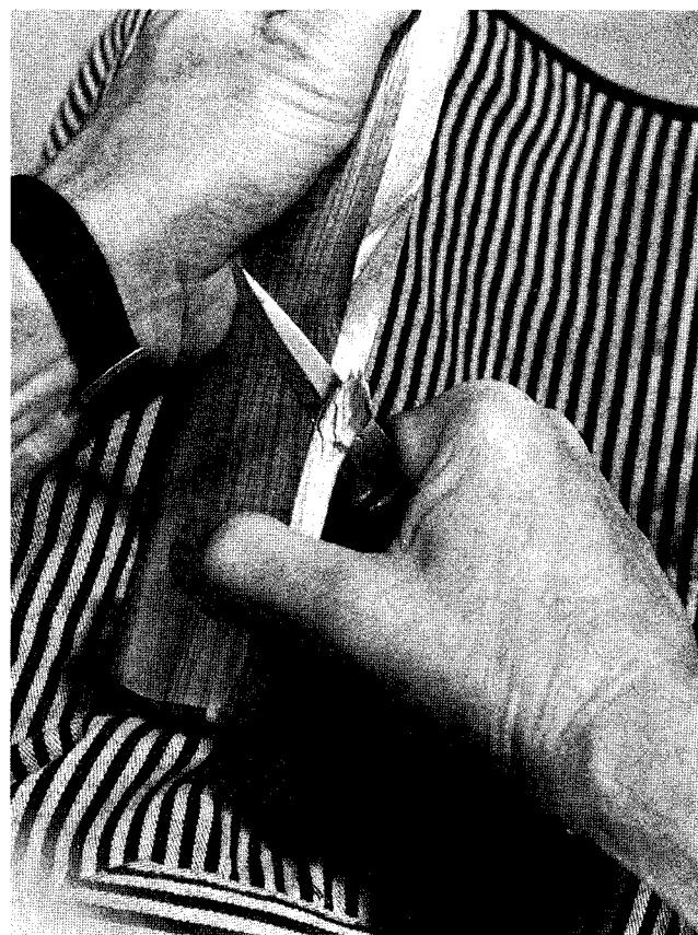
The blank is turned slightly away from the knife to start the stroke near the blade's tip (left). The blank is then rotated into the knife (right), and the stroke is completed when the knife handle and index finger contact the blank.
