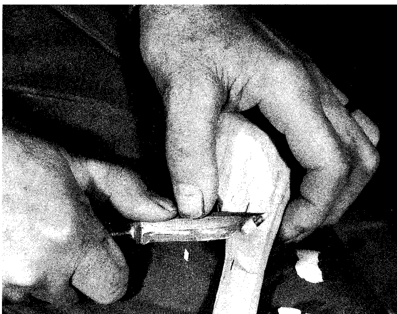
The blank is on the left knee and a thumb-push stroke smooths the transition from bowl to stem. Changes in grain direction in this area require frequent repositioning of the knife and blank.
