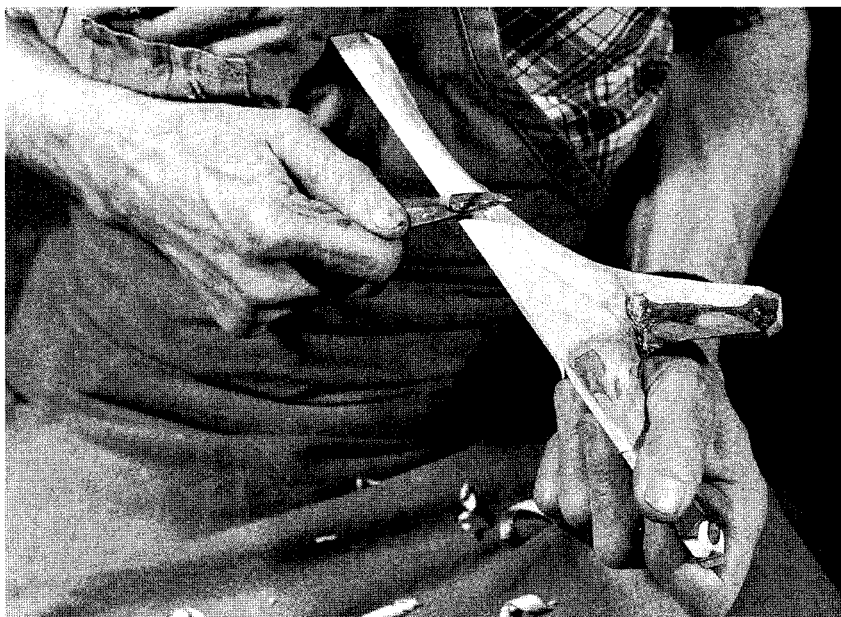
Long pull strokes are used to shape the front of the clothes hook after the back has been planed.
