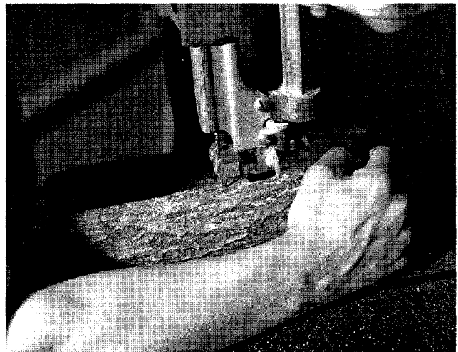
Before bandsawing the blank in half, hew a flat on one side for the blank to rest on through the cut. Then rip the blank down the pith, grasping it securely away from the blade. Note how the forearm rests on the bandsaw table for added stability.
