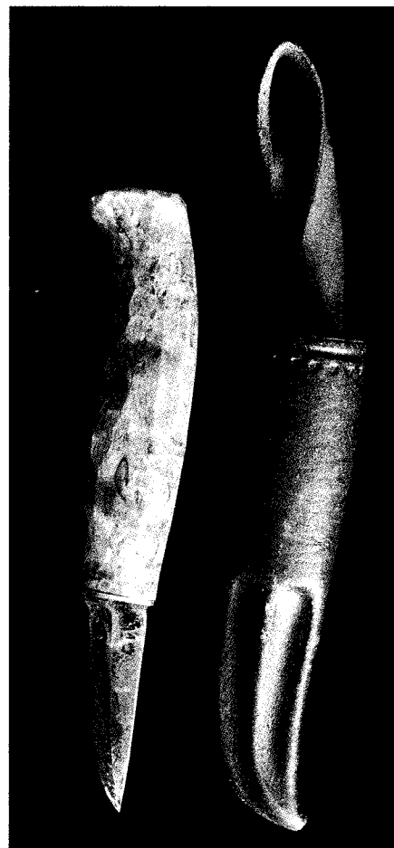
The carved surface of the handle on this knife gives it a good grip. The handle also has a dropped butt and slight flare toward the blade.
