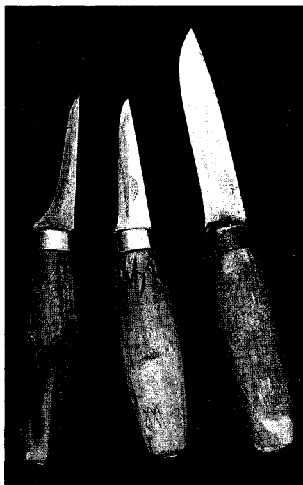
These Mora knives have been ground many times. The two knives at left have an excellent shape for carving small objects and getting into tight spots.
