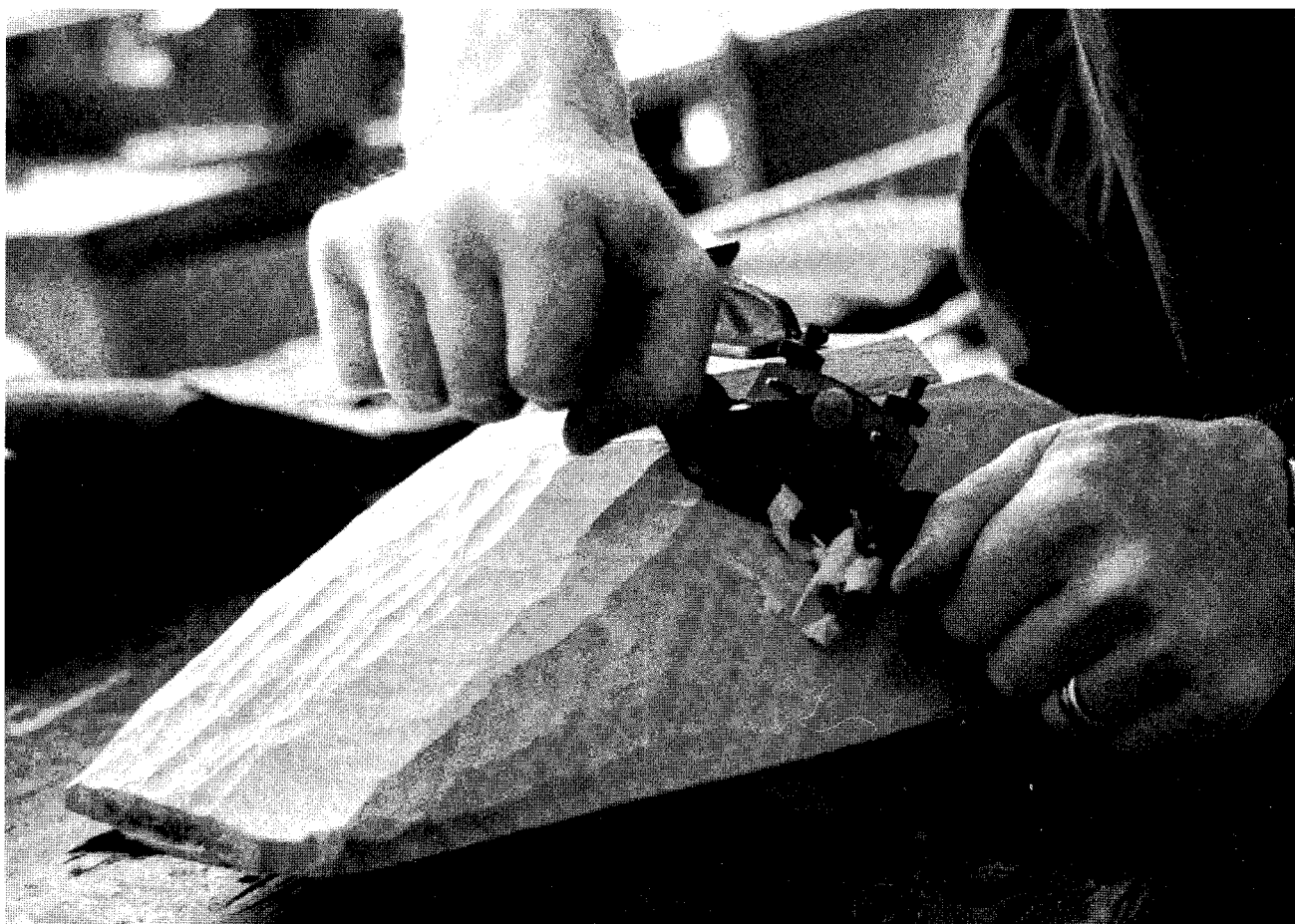
Smooth the outside shape with a splitting knife, drawknife or spokeshave.
