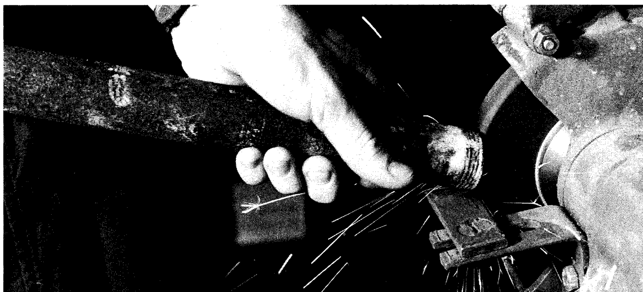
A high-speed grinder is used to sharpen the pipe.
