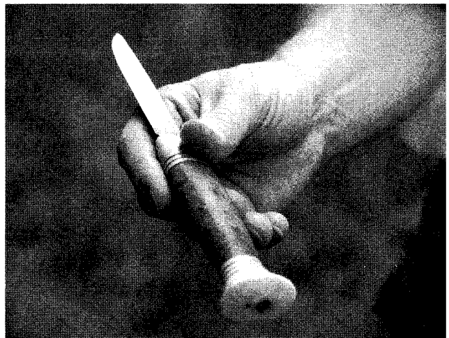
To hand a knife to another person safely, begin with a common grip. Flick the handle forward and rotate your hand. The handle is ready to take, with the back of the blade safely toward the web of your thumb.
