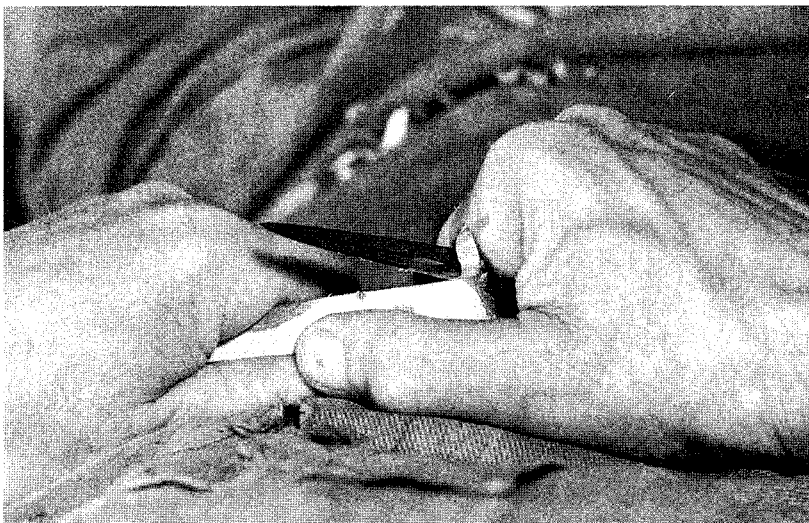
For increased power (in exchange for a somewhat shorter stroke), you can position the blank all the way under the second thumb joint.
