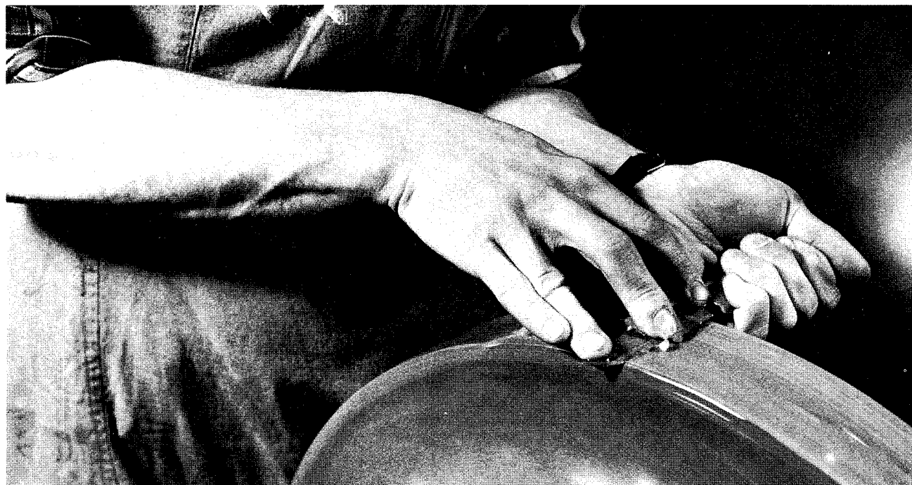
When a palm-up grip is used, the elbows gain support from the sides of the body and the hips.
