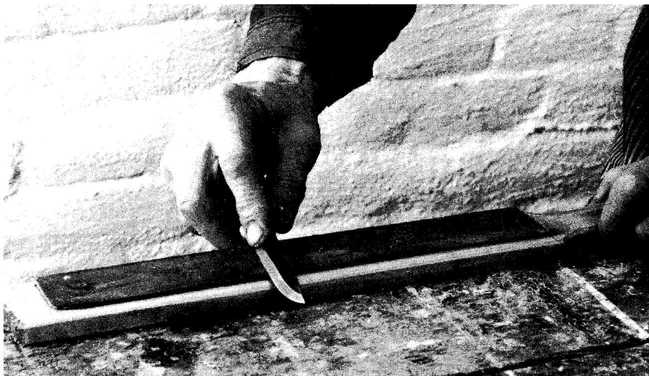
Strop on a piece of leather glued to a flat board. Draw the knife away from the edge. To strop the other bevel, roll the knife over the back of the blade, not the edge.
