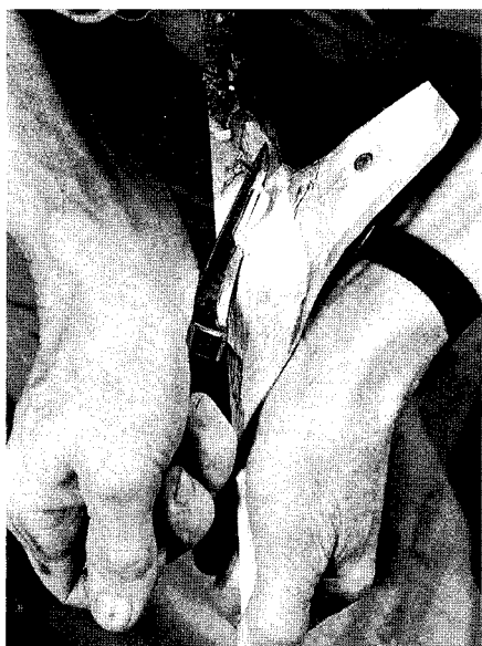
This wrist grip uses the ball of the wrist as a fulcrum, levering the knife through its stroke.
