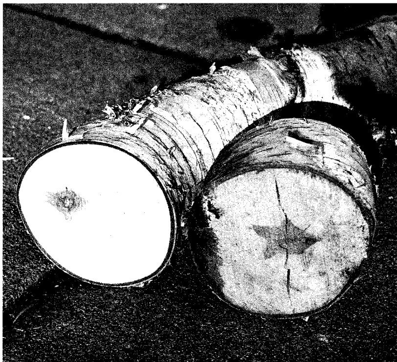
The pith usually follows the middle of a pine crook, but in birch it tends toward the outer part of the elbow.
