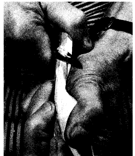
The stop for the thumb-joint grip is your index finger contacting the blank.
