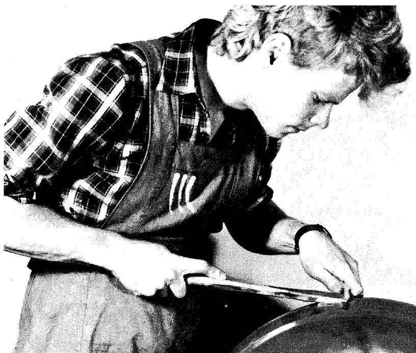
Grinding with the aid of a grinding stick.
