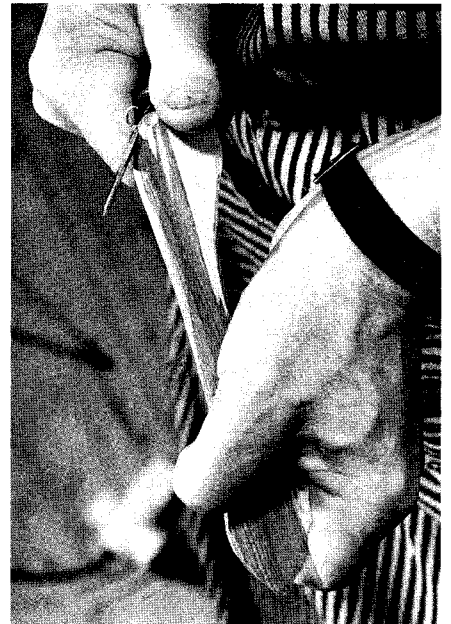
The draw grip cuts smoothest when it's used to shear from the tip of the blade to the hilt (top), or from the hilt to the tip (bottom).
