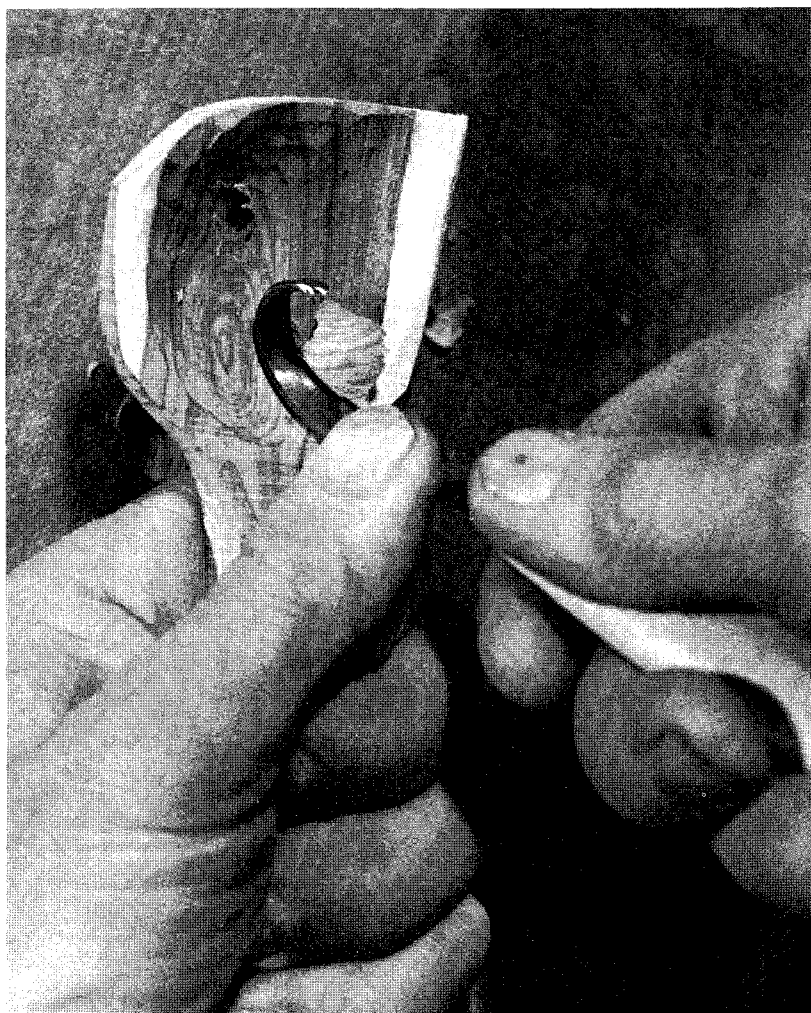
A single-edged carving hook makes it possible for the thumb to push, or be a fulcrum, for sweeping strokes that smoothly hollow a spoon bowl.
