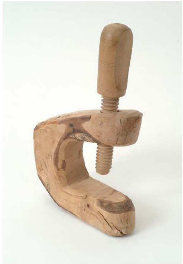
C-clamp, made from a naturally formed piece of birch. Rauland, Norway.
